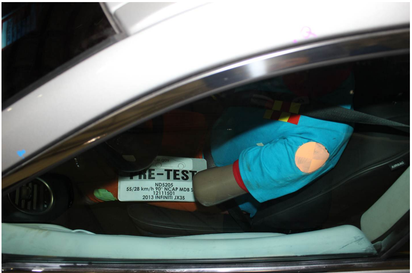
Pre-Test Driver Dummy and Door Clearance View
