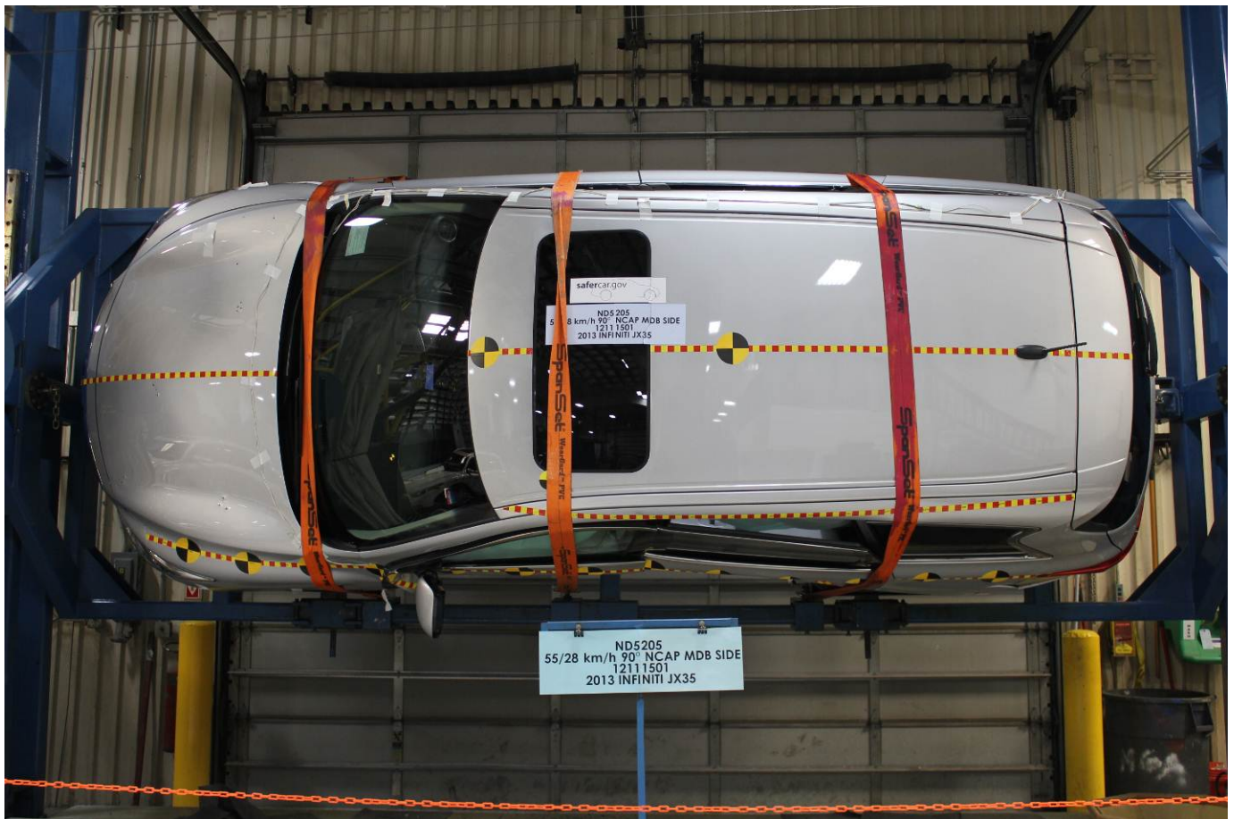
FMVSS No. 301 Static Rollover 90 Degrees
