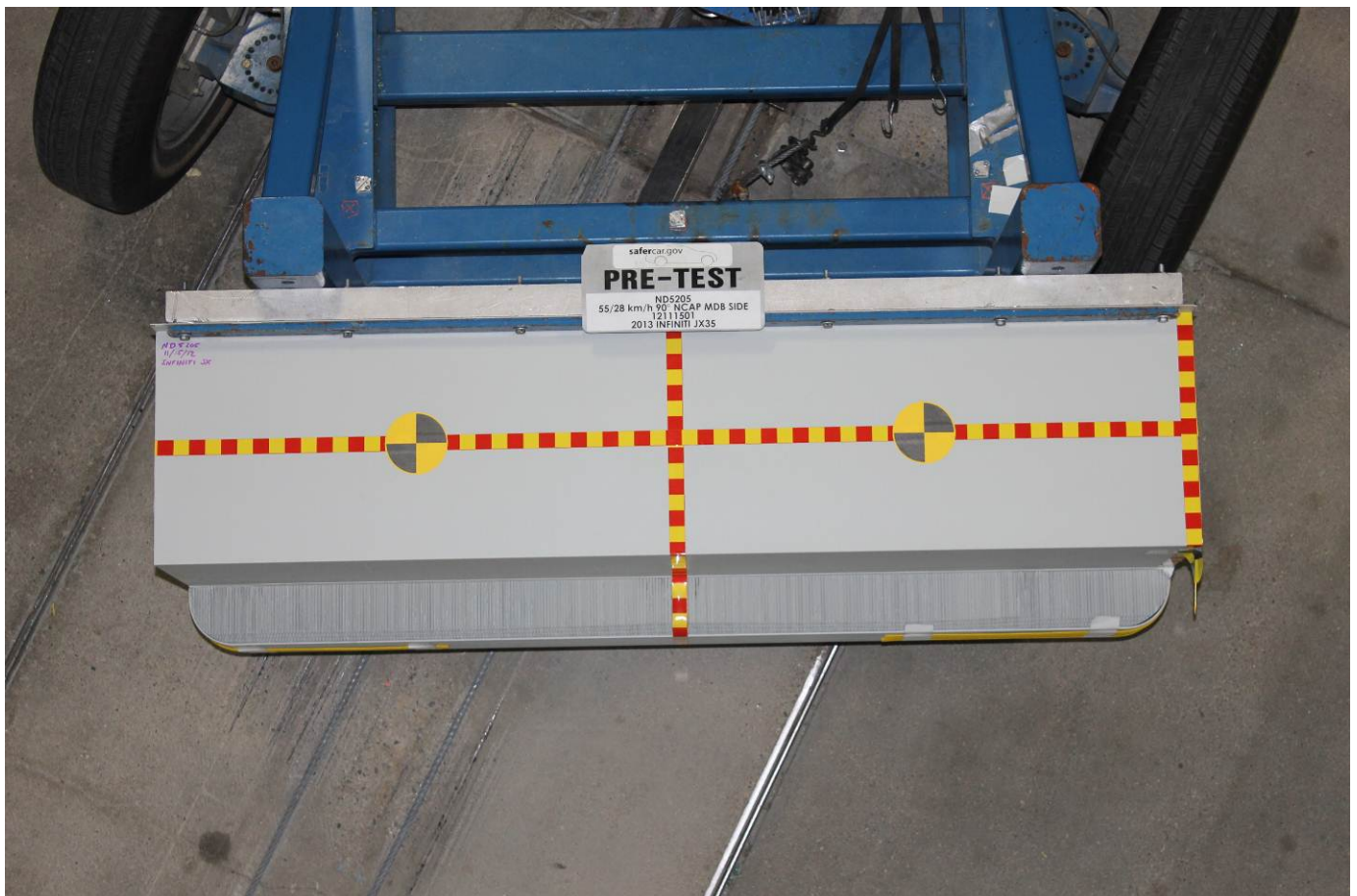
Pre-Test Top View of MDB Impactor Face
