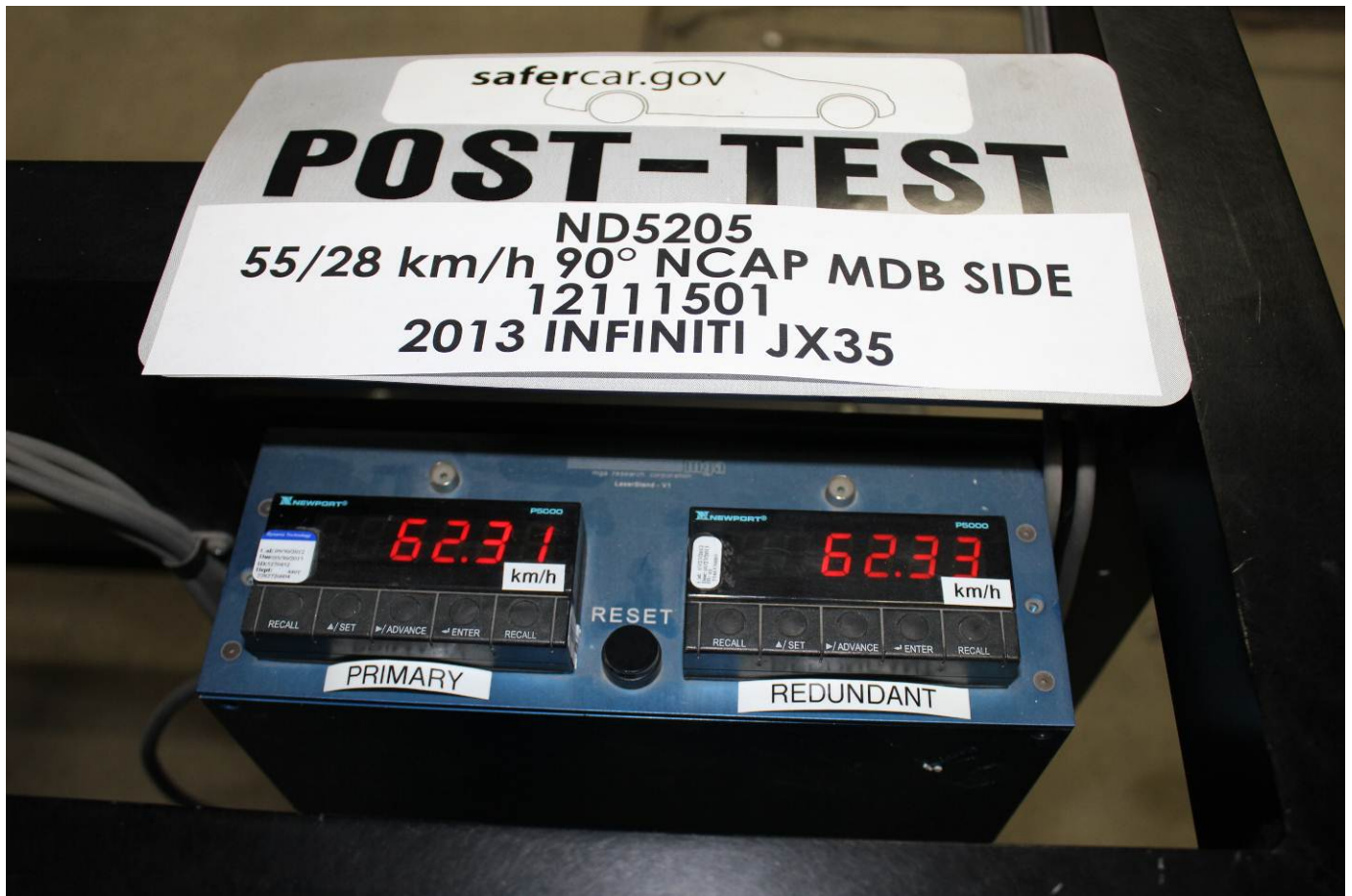
Post-Test Primary and Redundant Speed Trap Read-Out
