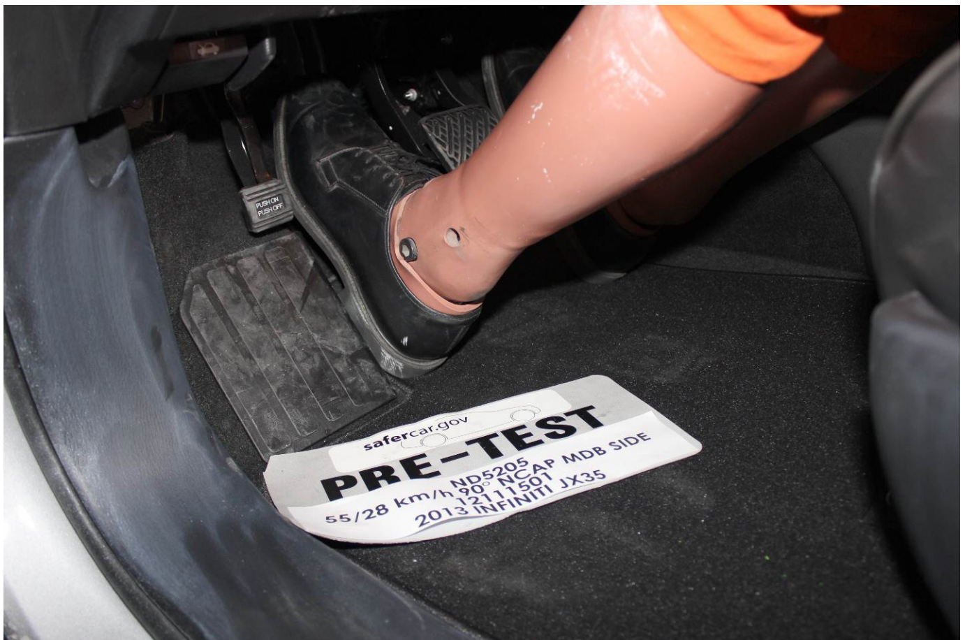
Pre-Test Placement of Driver Dummy's Feet
