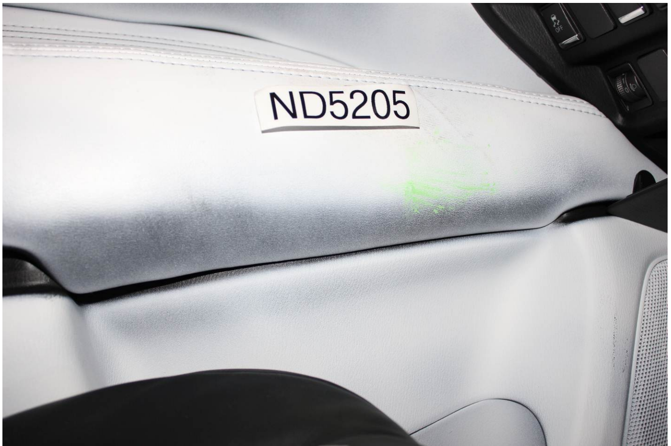
Post-Test Driver Dummy Close-up Knee Contact View
