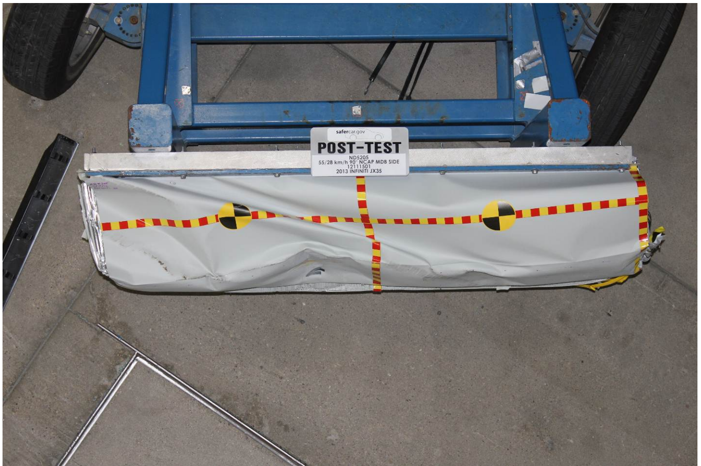
Post-Test Top View of MDB Impactor Face
