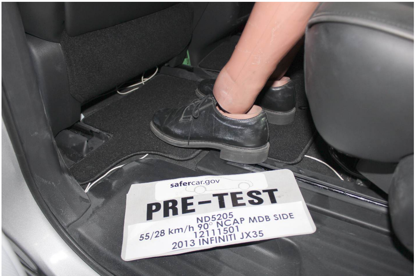
Pre-Test Placement of Rear Passenger Dummy's Feet
