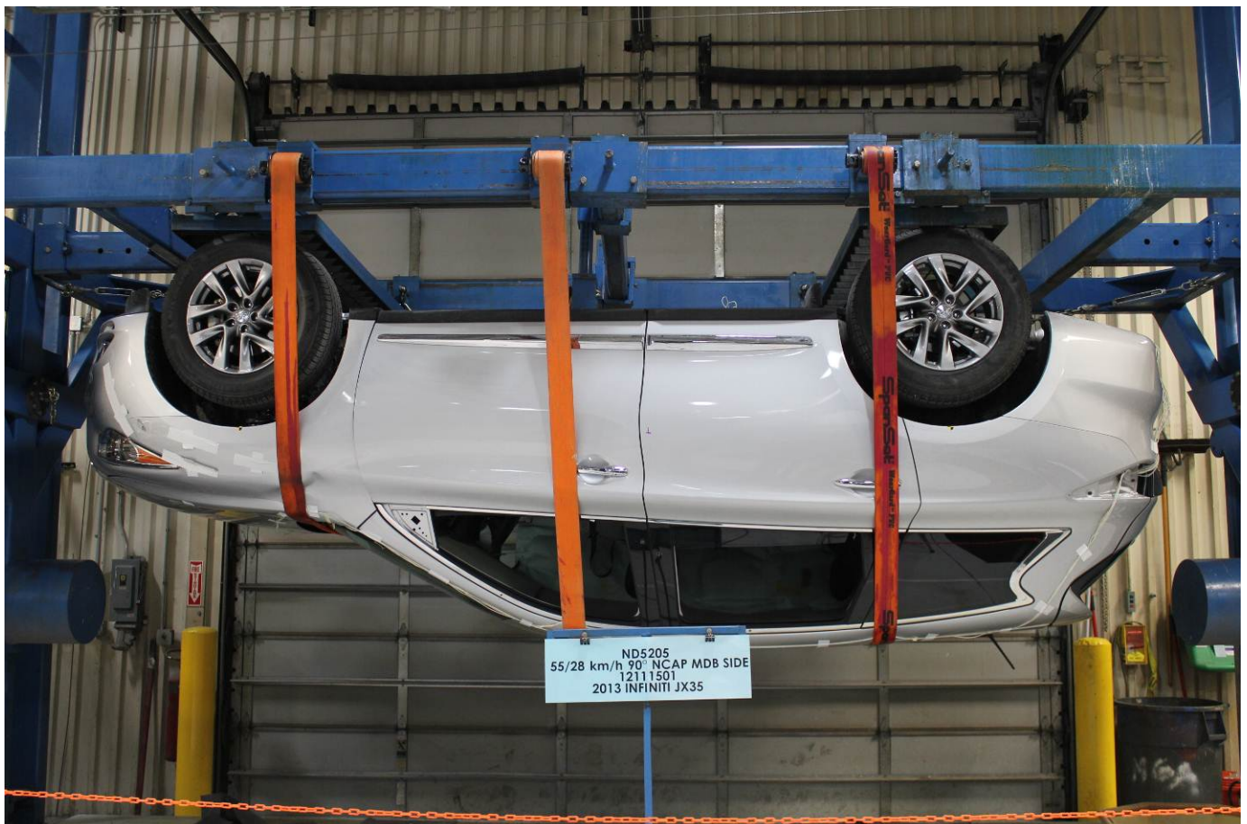
FMVSS No. 301 Static Rollover 180 Degrees
