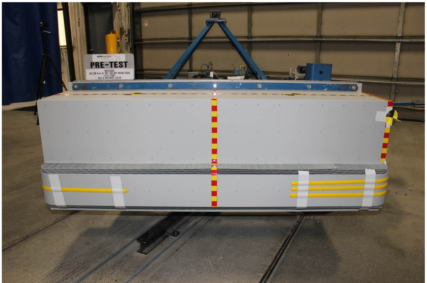
Pre-Test Front View of MDB Impactor Face
