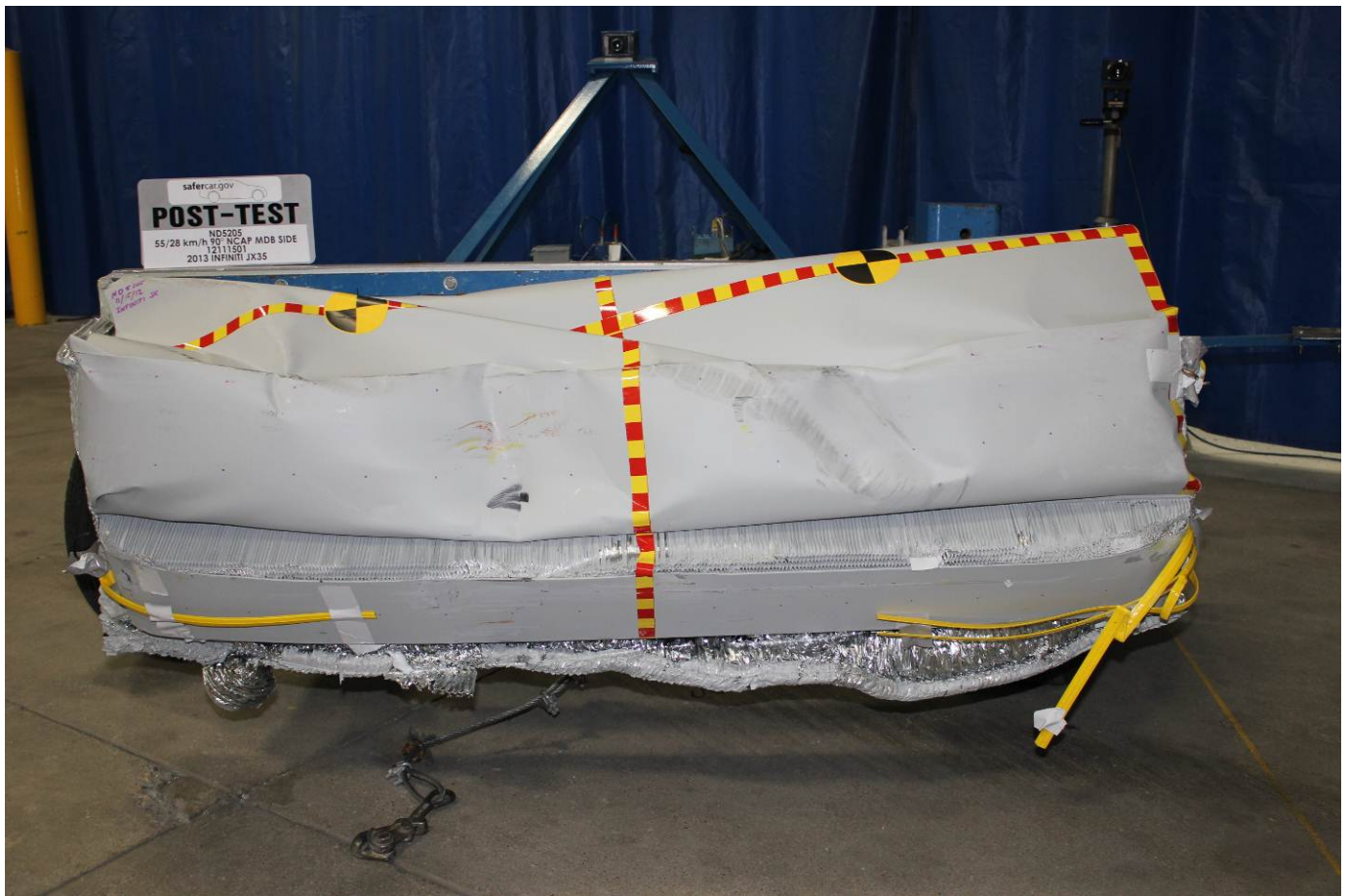
Post-Test Front View of MDB Impactor Face
