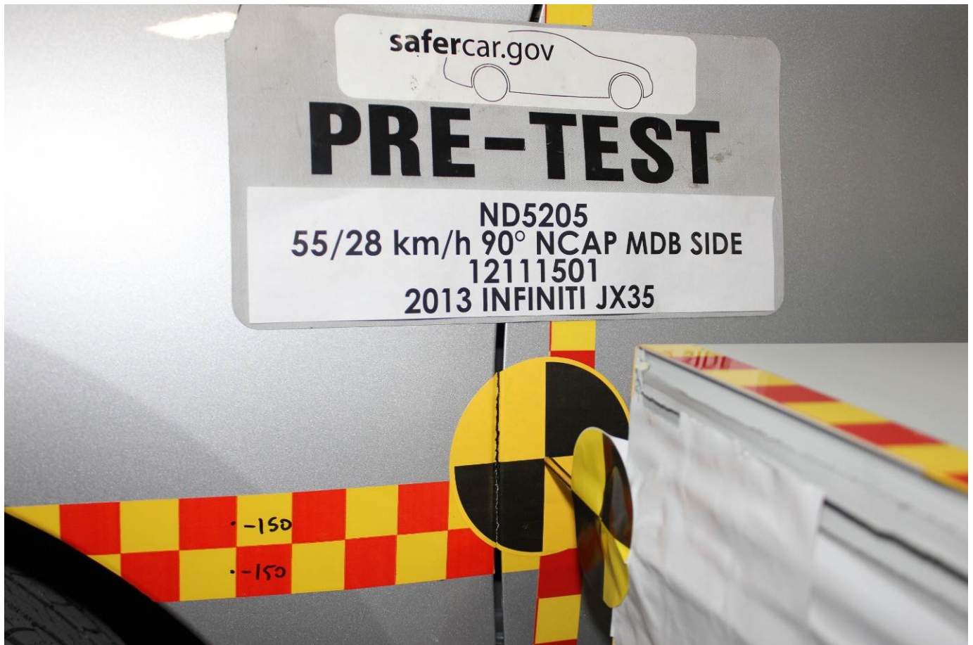
Pre-Test Close-Up View of Impact Point Target
