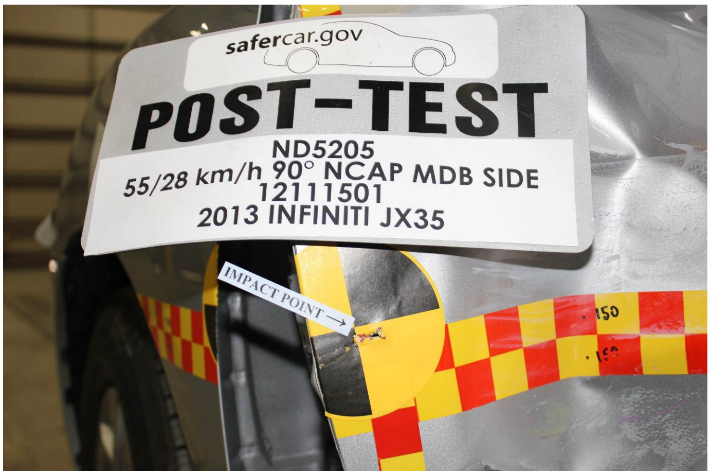
Post-Test Close-Up View of Impact Point Target
