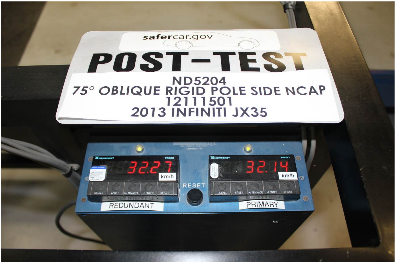
Post-Test Primary and Redundant Speed Trap Read-Out
