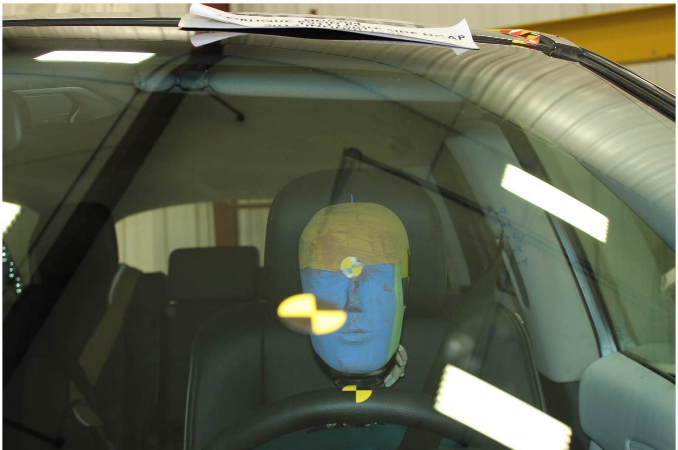
Pre-Test Front Close-Up View of Dummy Head and Shoulders in Relation to Head Restraint
