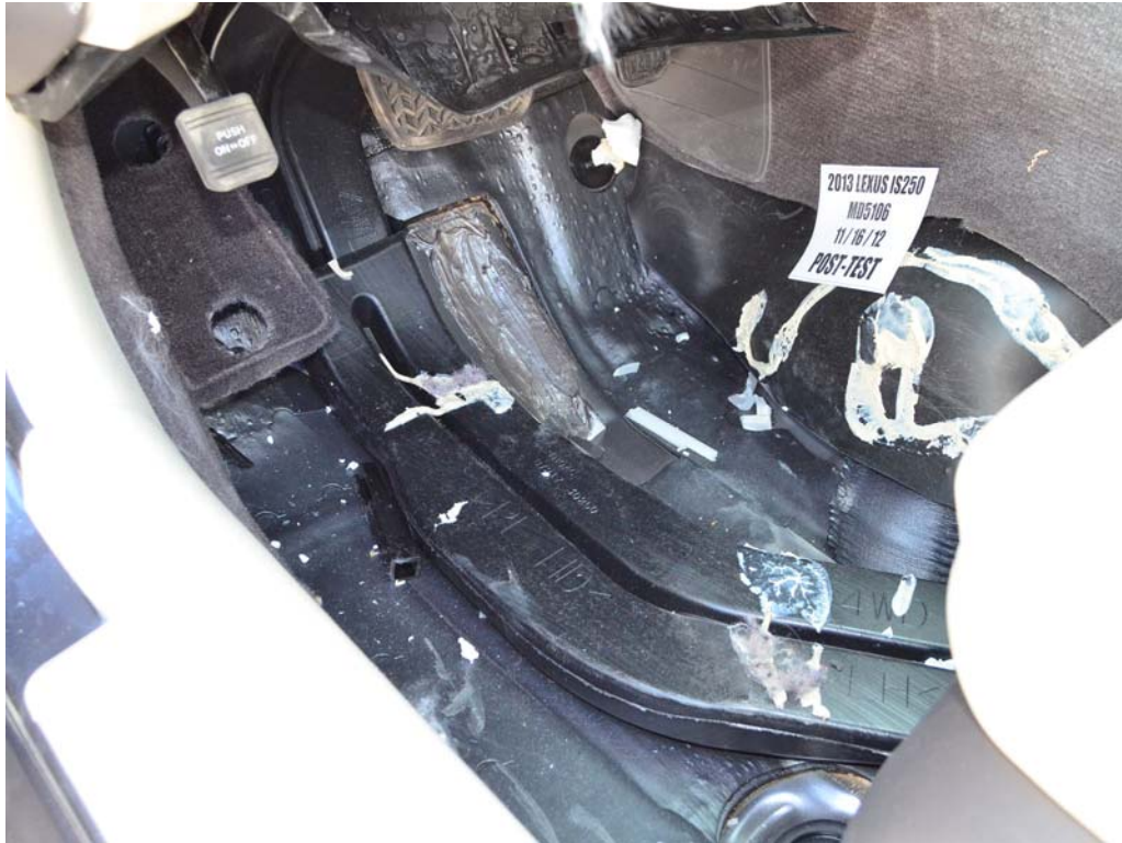
FIGURE 44. Post-Test Driver's Side Floorpan
