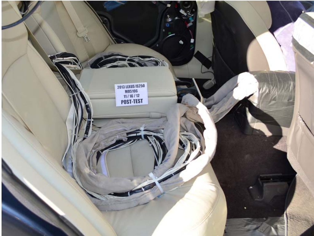
FIGURE 28. Post-Test Dummy Cable Routing
