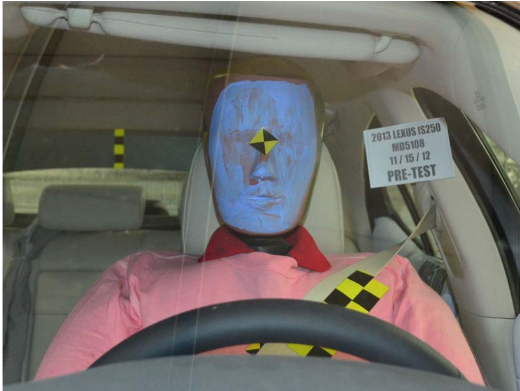
FIGURE 25. Pre-Test Front Close-Up View of Driver Dummy
