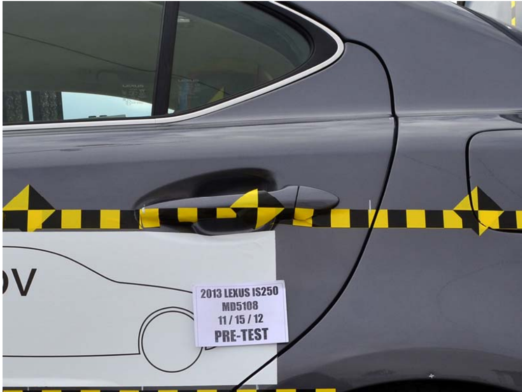
FIGURE 23. Pre-Test Left Rear Door Latch Close-Up
