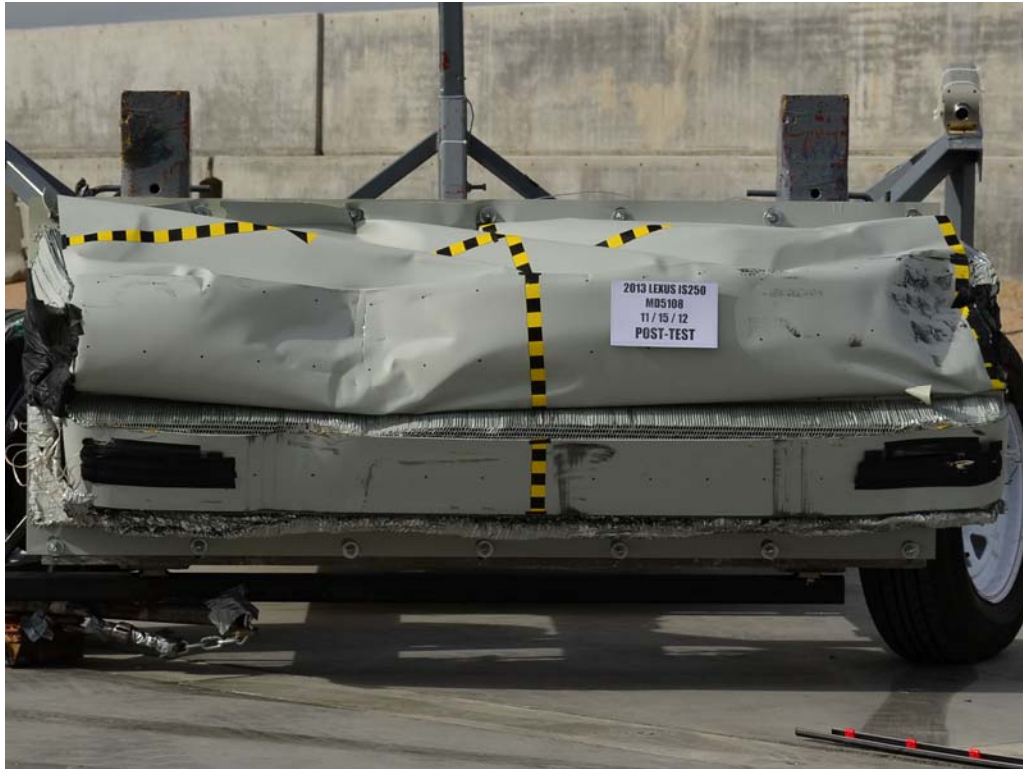
FIGURE 85. Post-Test Front View of MDB Impactor Face
