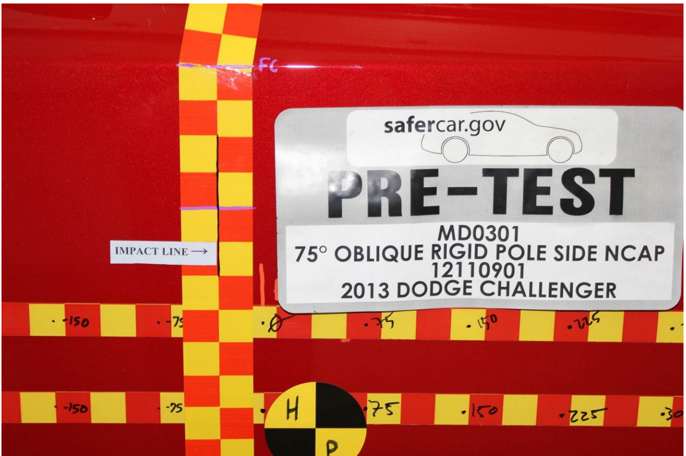
Pre-Test Close-Up View of Impact Point Target
