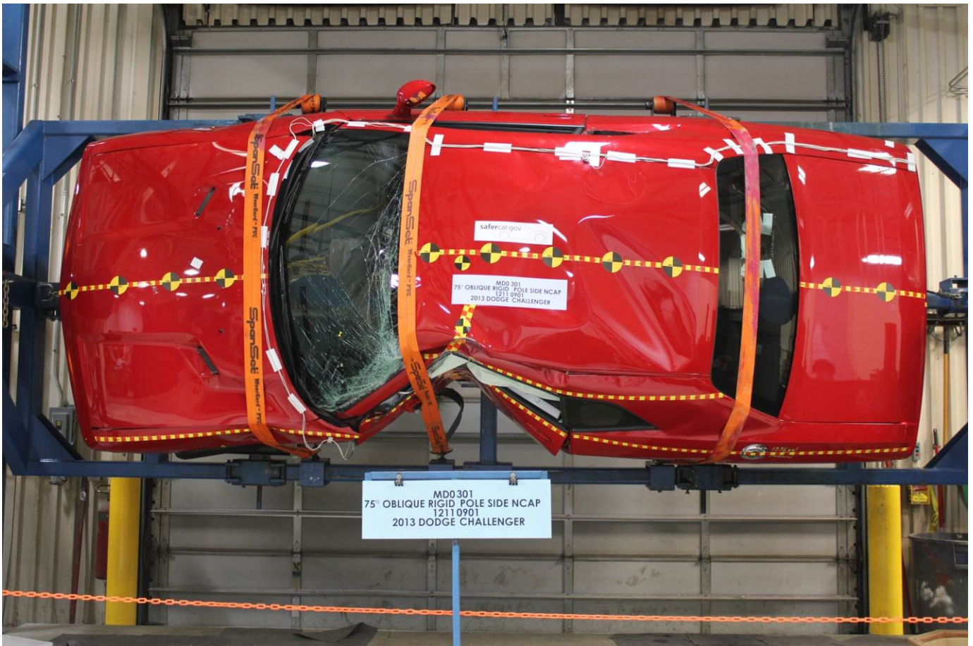
FMVSS No. 301 Static Rollover 90 Degrees
