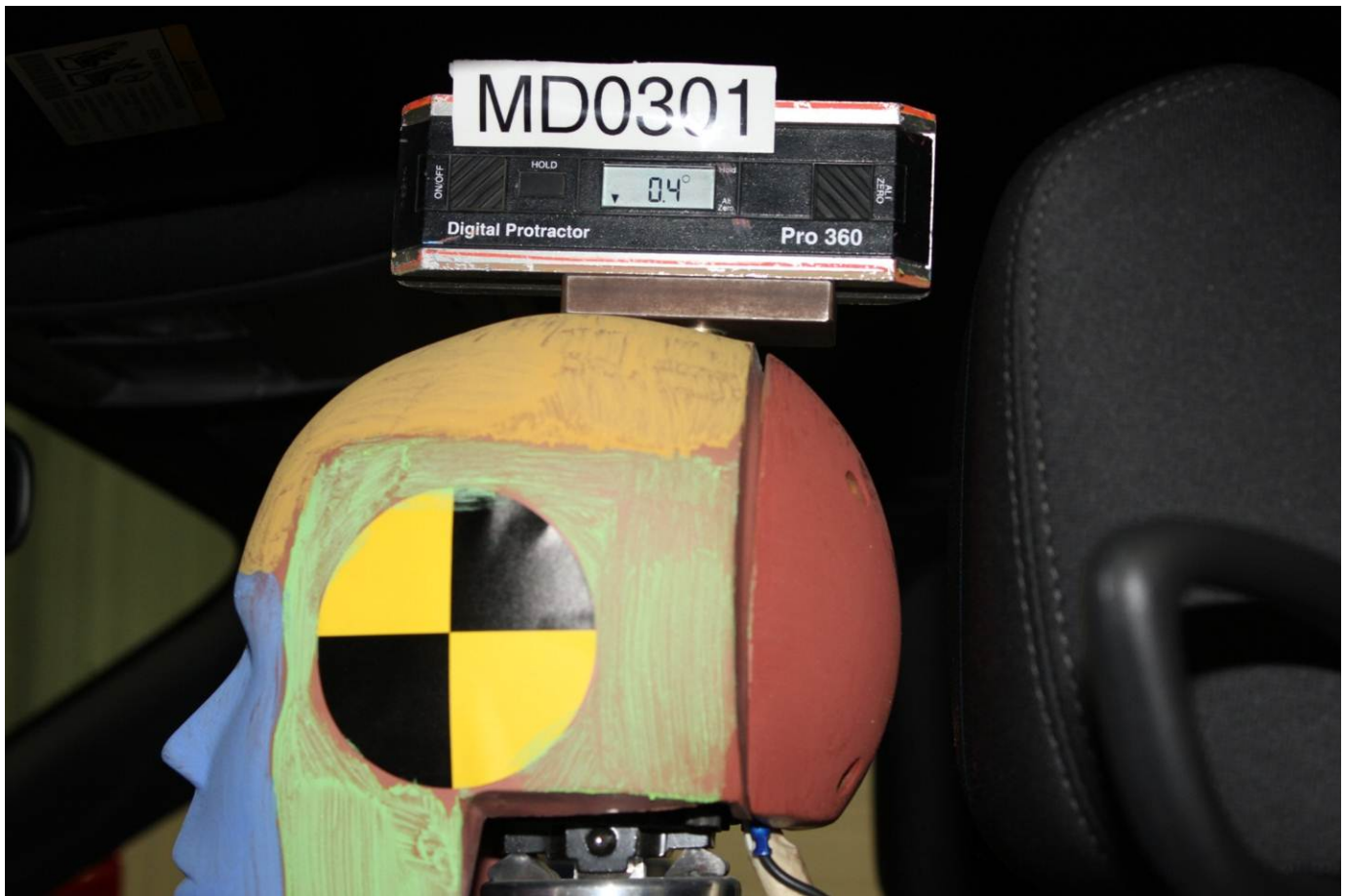
Pre-Test Left Side View of Dummy's Head Showing Dummy's Head is Level
