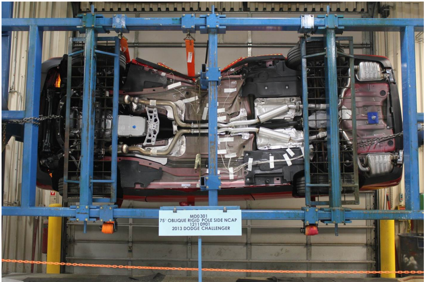
FMVSS No. 301 Static Rollover 270 Degrees
