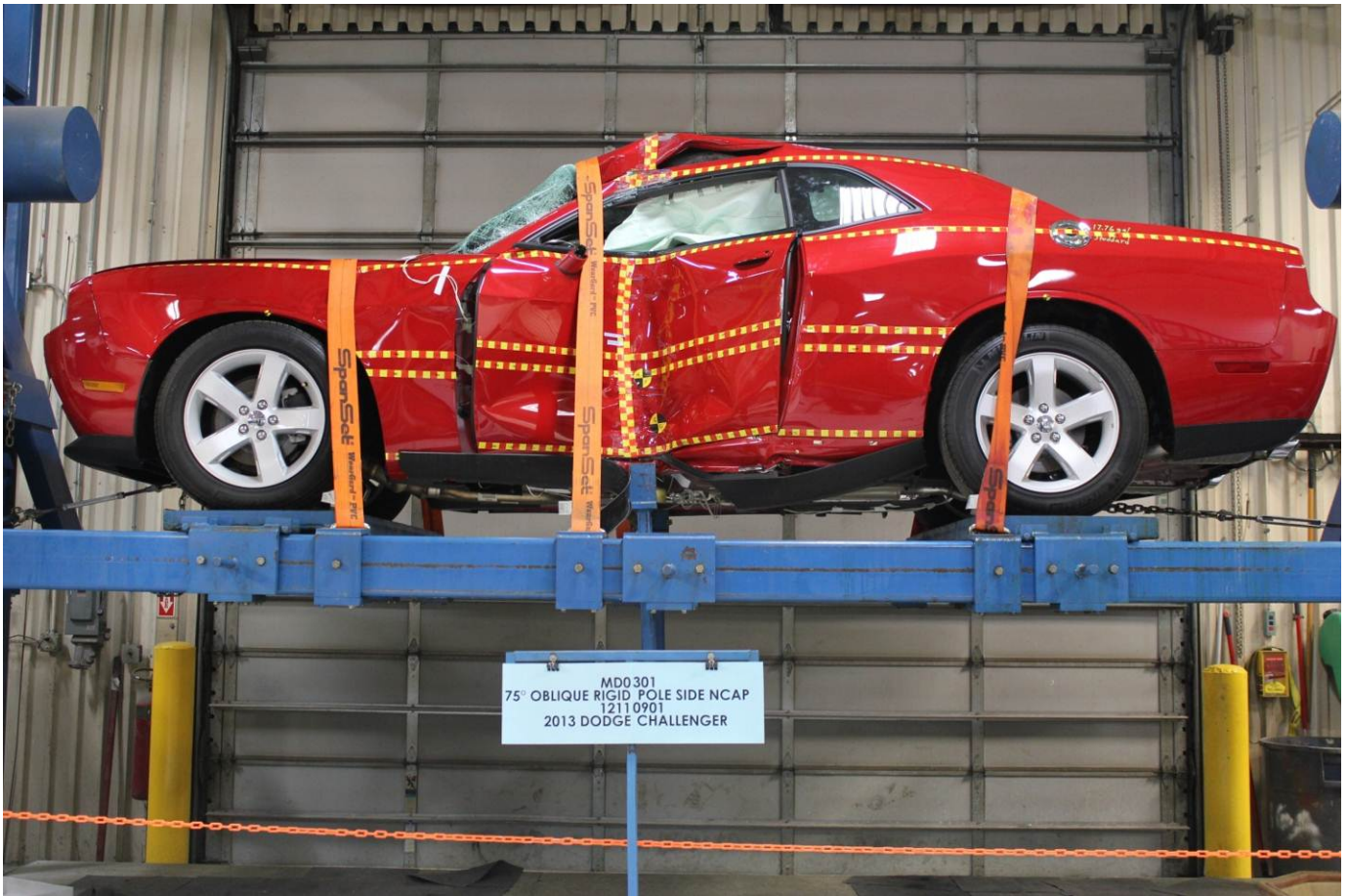
FMVSS No. 301 Static Rollover 0 Degrees
