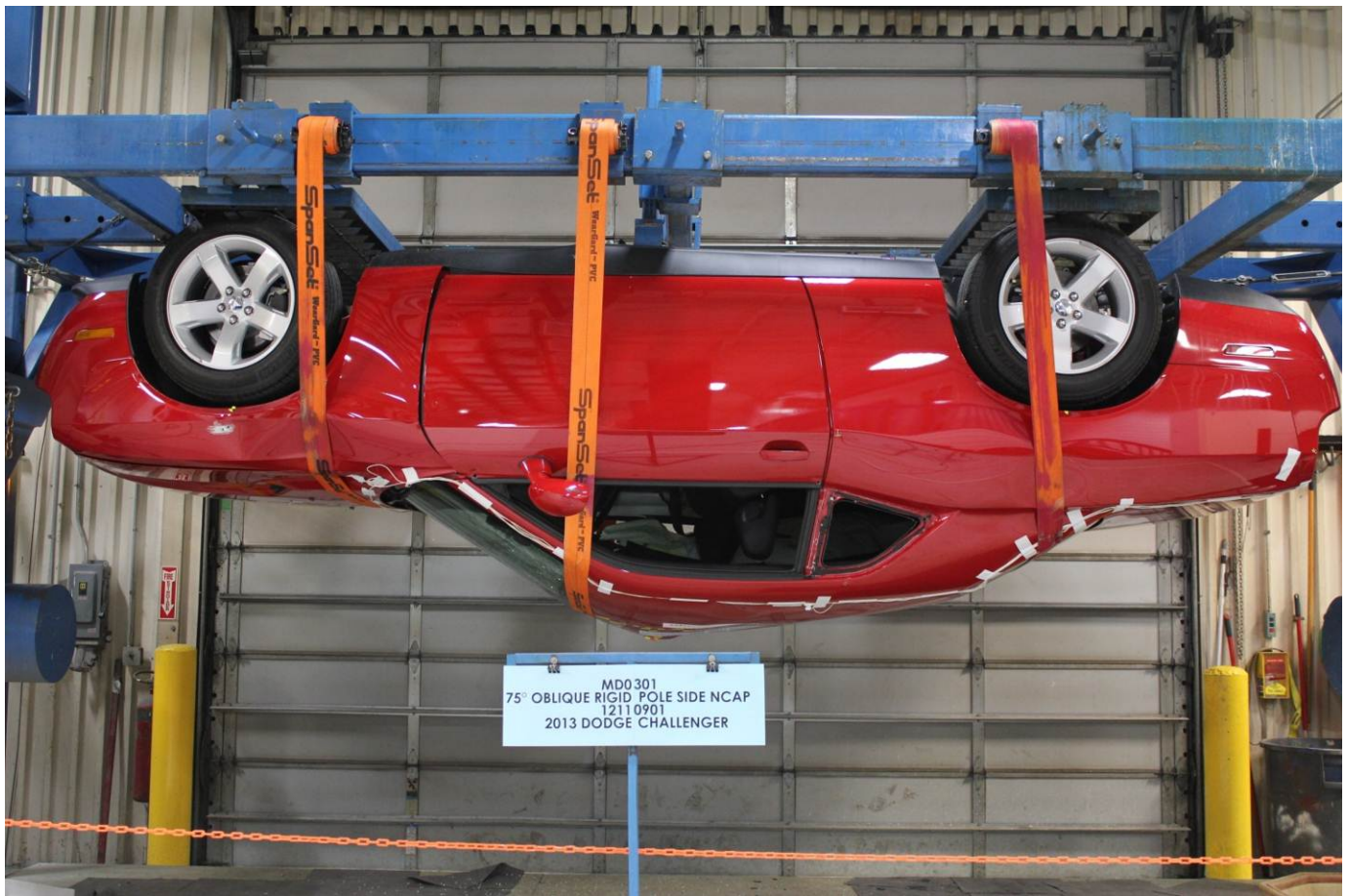
FMVSS No. 301 Static Rollover 180 Degrees
