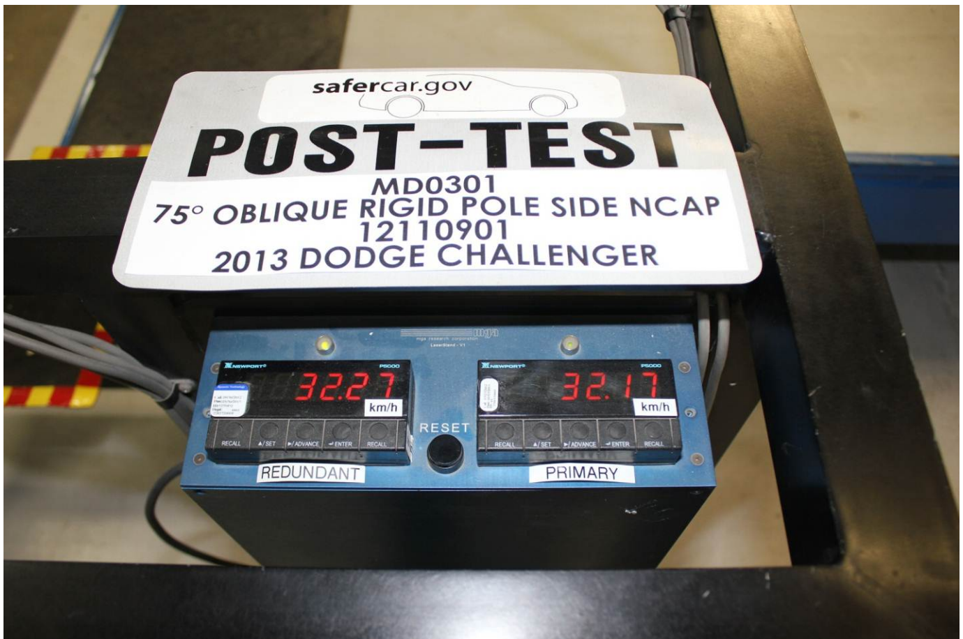
Post-Test Primary and Redundant Speed Trap Read-Out
