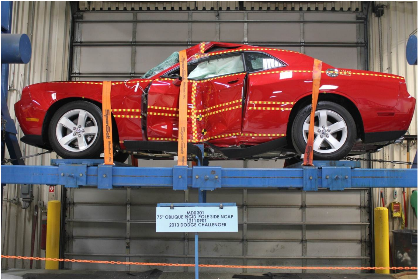
FMVSS No. 301 Static Rollover 360 Degrees
