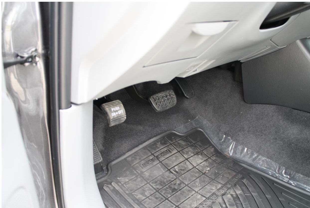
Figure A-37: View of Disengaged Parking Brake
