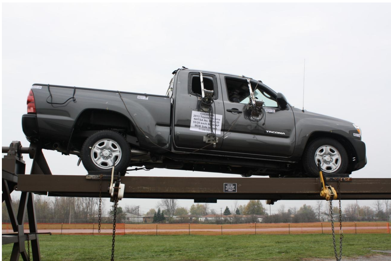
Figure A-100: FMVSS No. 301 Static Rollover 360 Degrees
