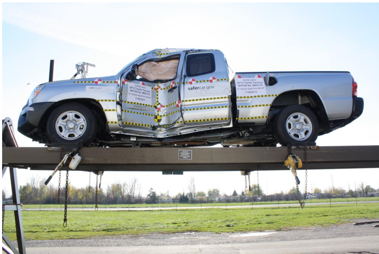
Figure A-63: FMVSS No. 301 Static Rollover 0 Degrees
