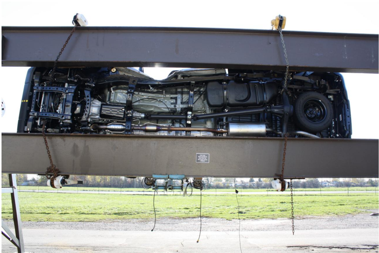
Figure A-66: FMVSS No. 301 Static Rollover 270 Degrees
