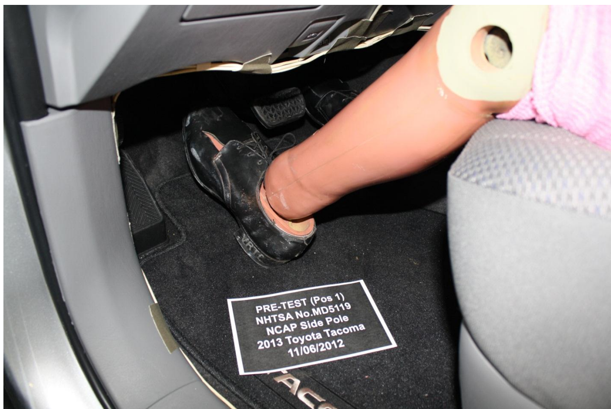
Figure A-32: Pre-Test Placement of Dummy's Feet
