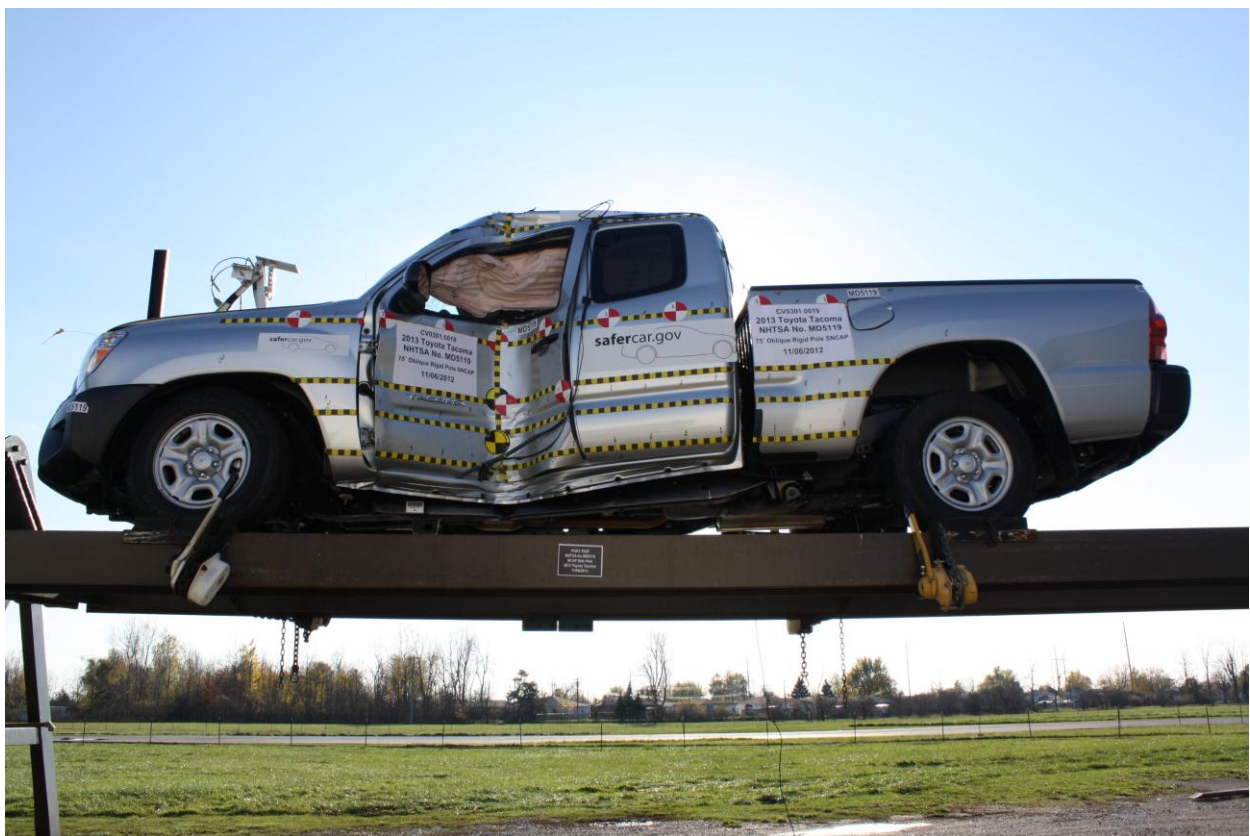
Figure A-67: FMVSS No. 301 Static Rollover 360 Degrees
