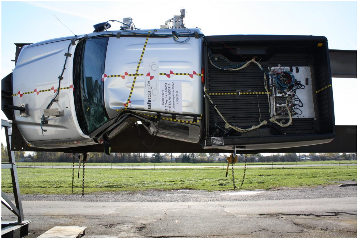
Figure A-64: FMVSS No. 301 Static Rollover 90 Degrees
