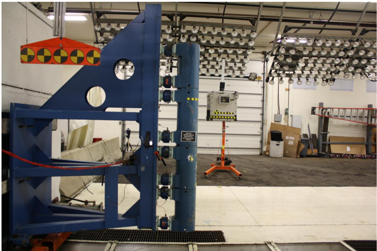
Figure A-59: Pre-Test Pole Barrier Side View
