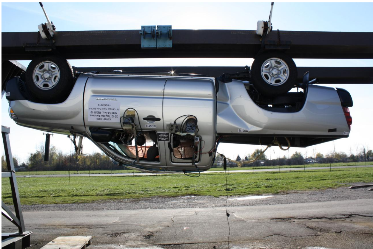
Figure A-65: FMVSS No. 301 Static Rollover 180 Degrees
