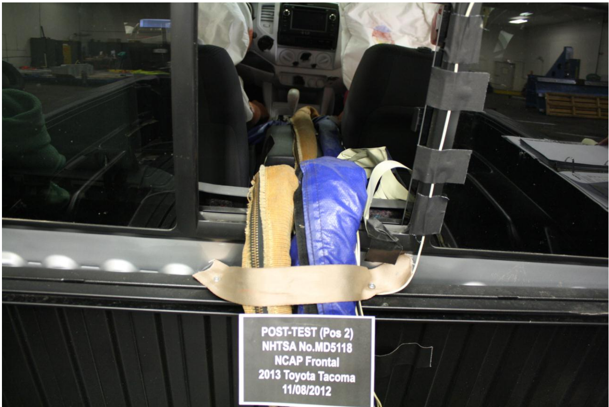
Figure A-28: Post-Test Dummy Cable Routing
