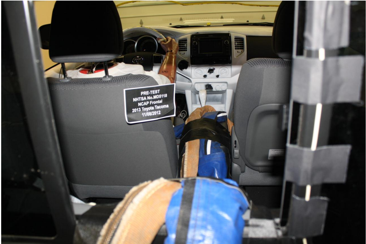
Figure A-27: Pre-Test Dummy Cable Routing
