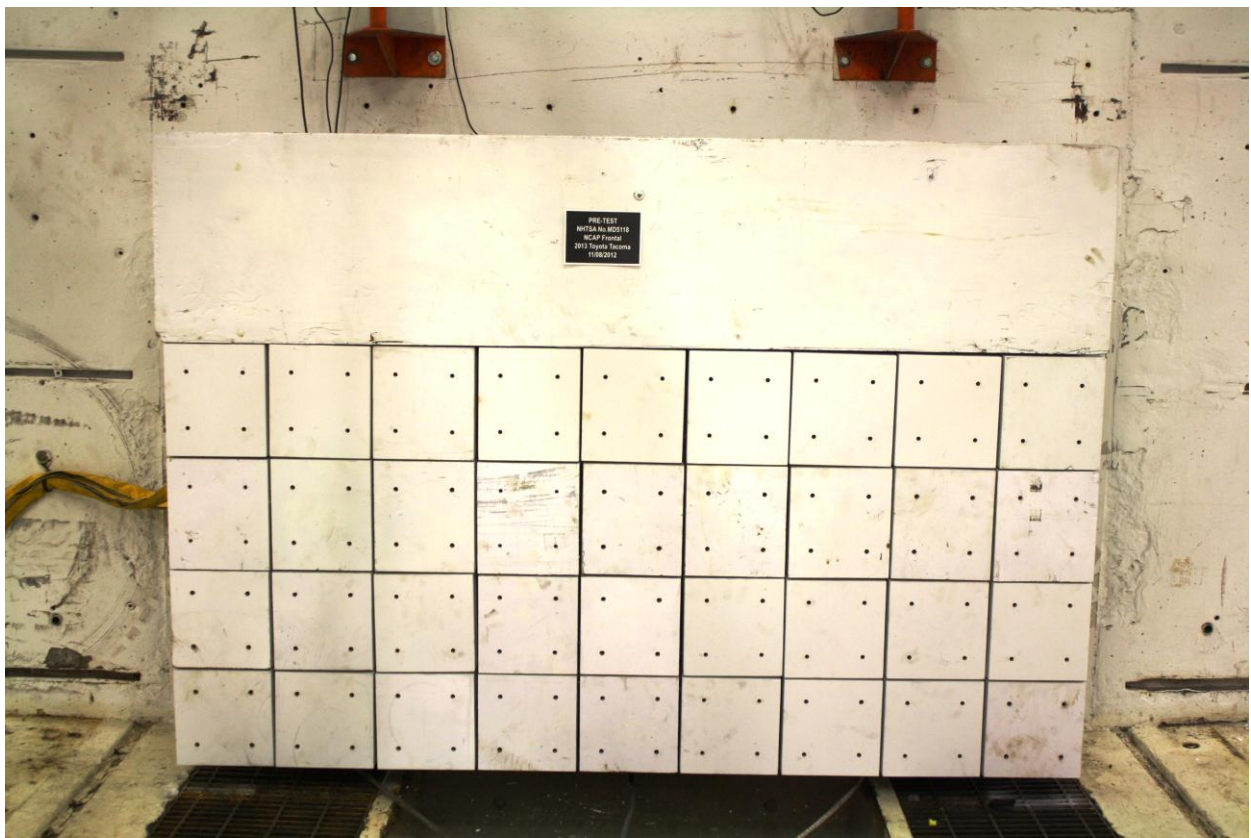
Figure A-2: Load Cell Wall
