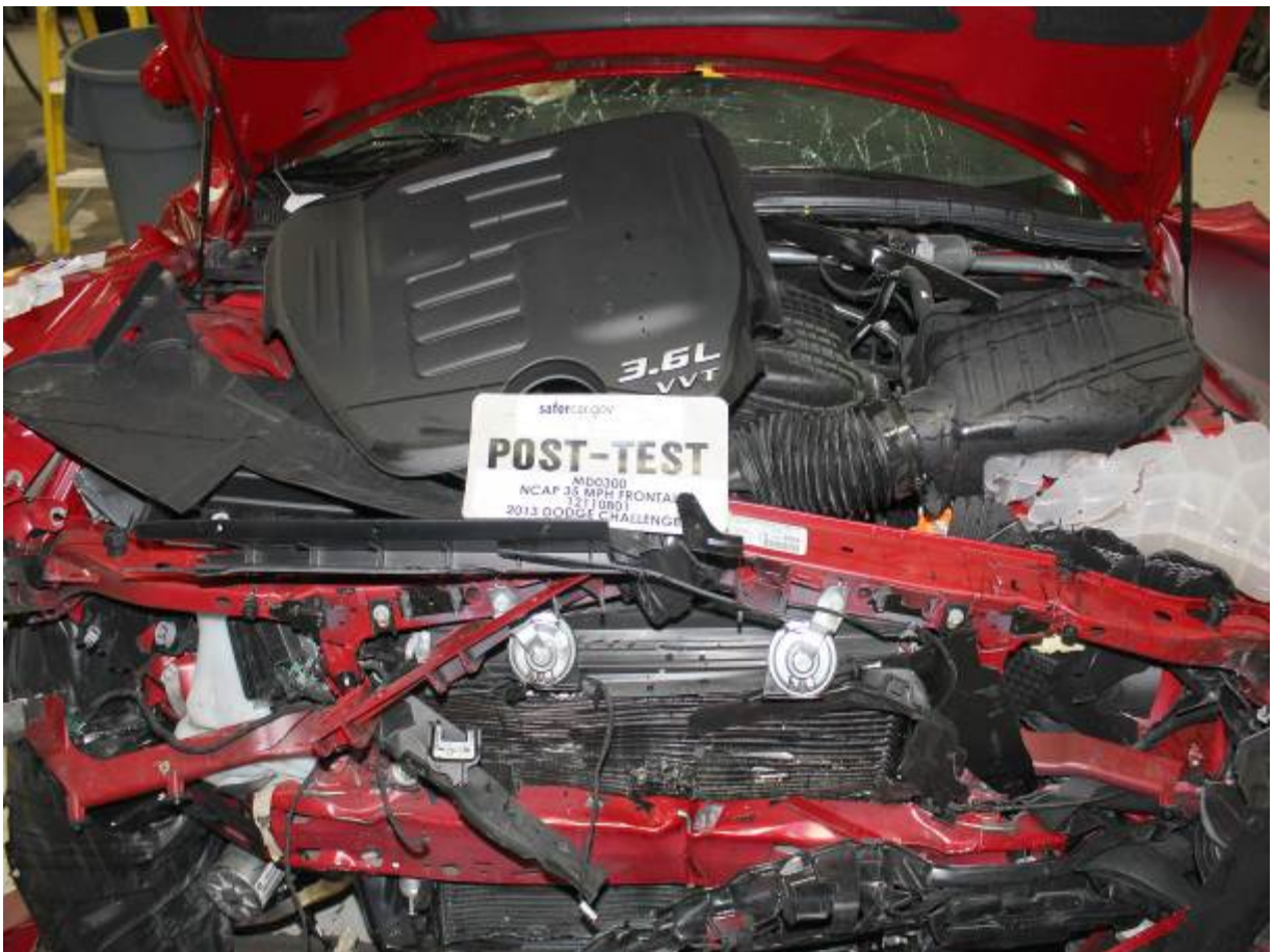
Post-Test Engine Compartment View
