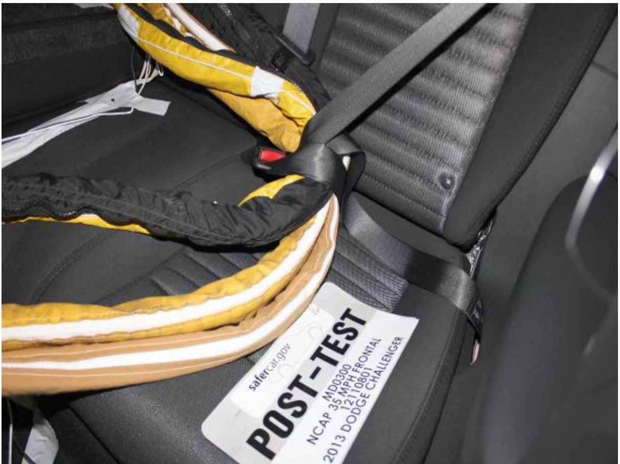
Post-Test Dummy Cable Routing
