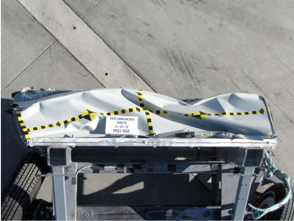
FIGURE 87. Post-Test Top View of MDB Impactor Face
