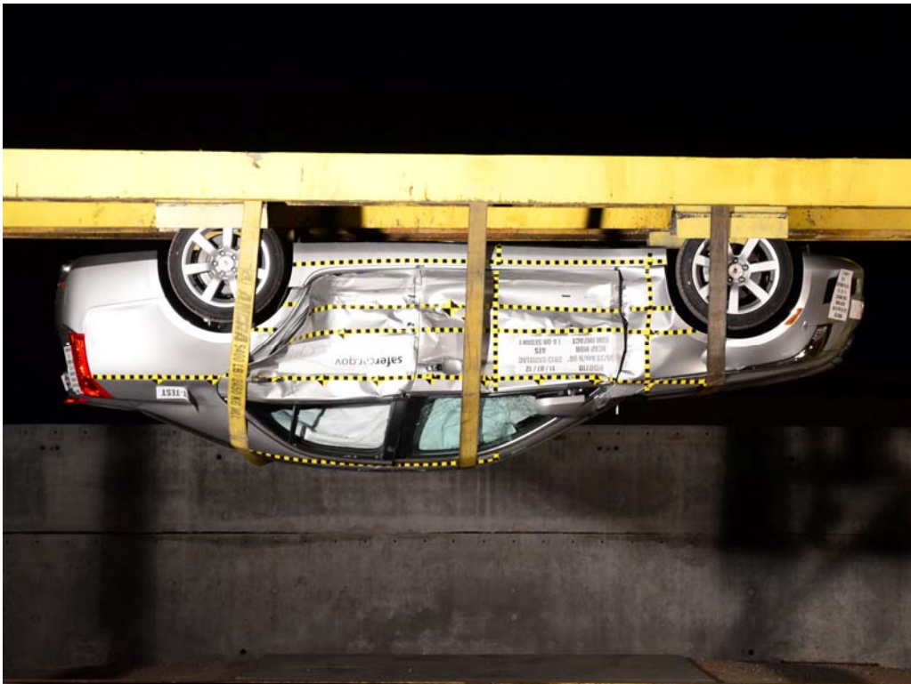
FIGURE 98. FMVSS No. 301 Static Rollover 180 Degrees
