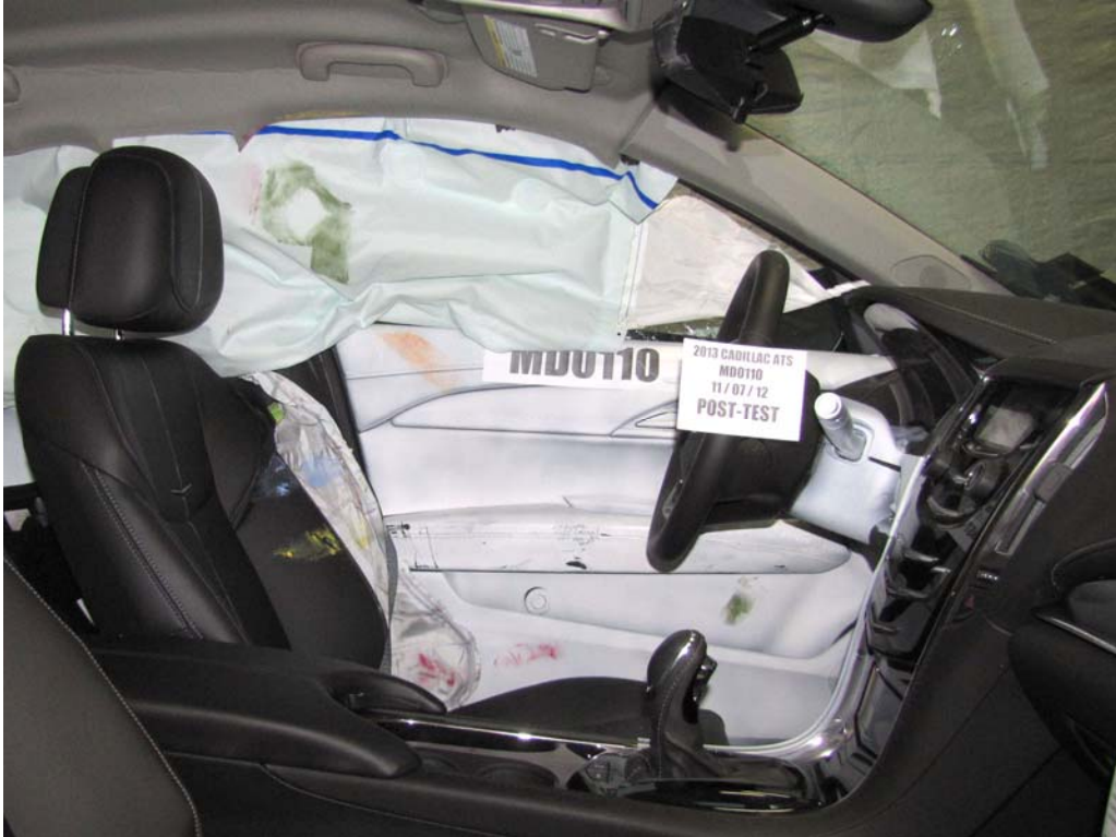
FIGURE 47. Post-Test Driver Inner Door Panel View
