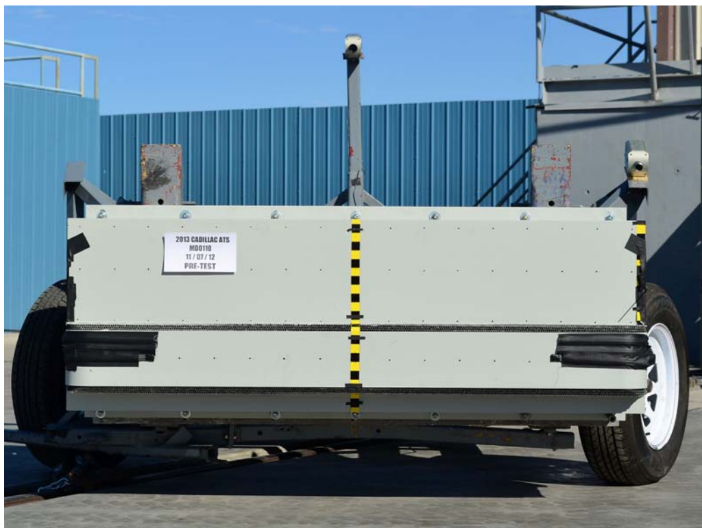
FIGURE 84. Pre-Test Front View of MDB Impactor Face
