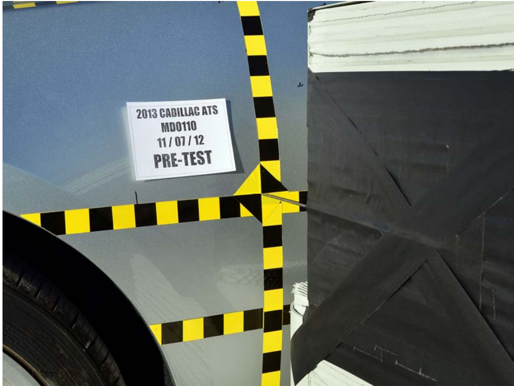
FIGURE 19. Pre-Test Close-Up View of Impact Point Target
