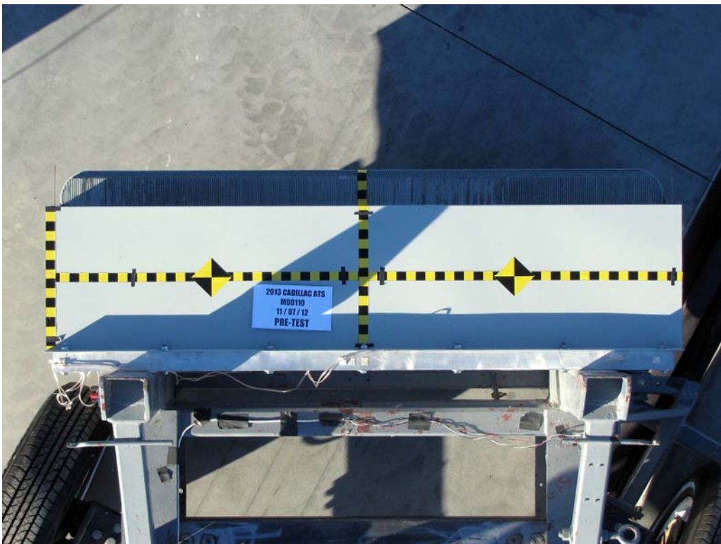
FIGURE 86. Pre-Test Top View of MDB Impactor Face
