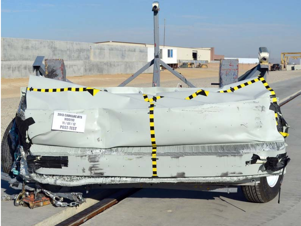
FIGURE 85. Post-Test Front View of MDB Impactor Face
