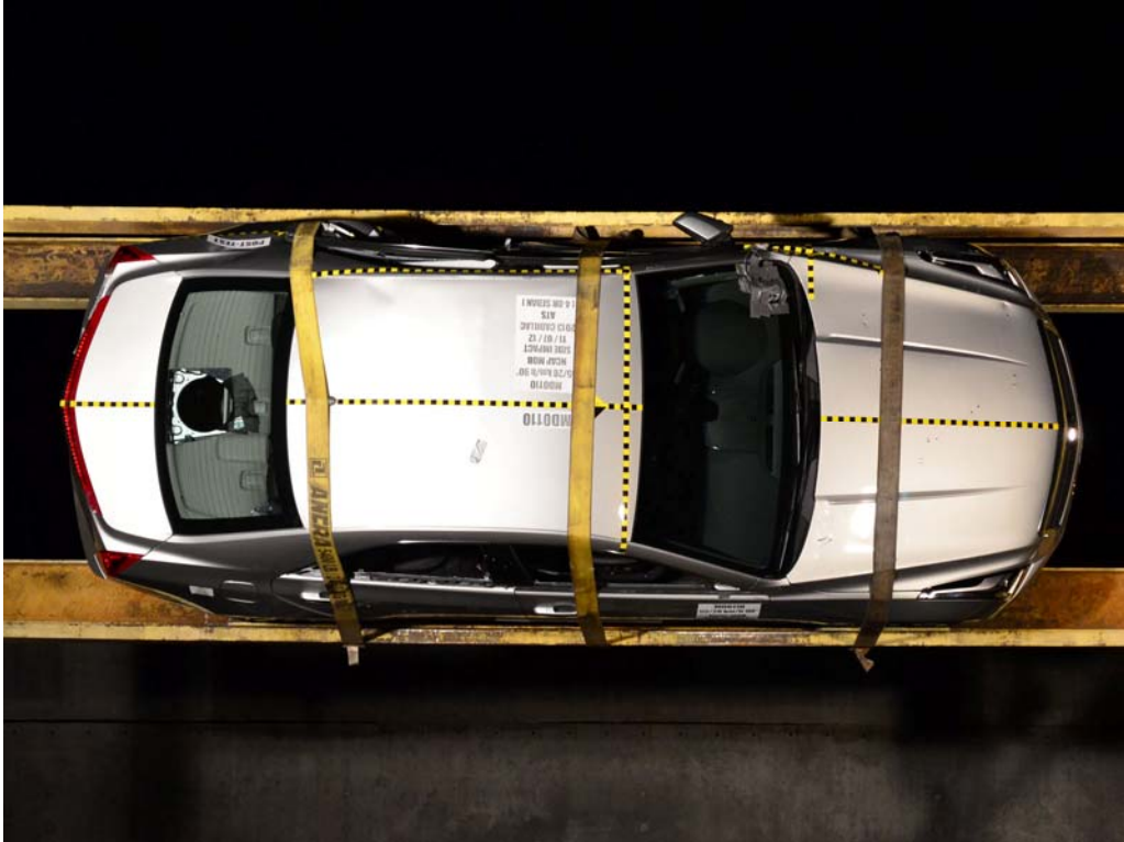
FIGURE 97. FMVSS No. 301 Static Rollover 90 Degrees
