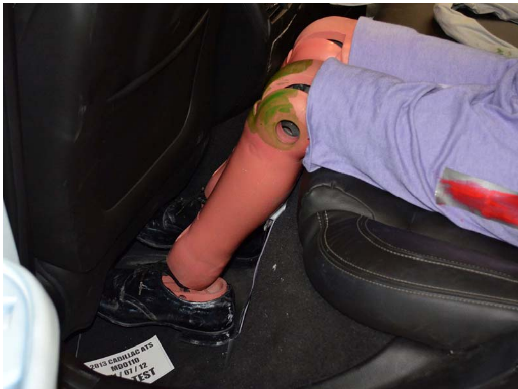
FIGURE 64. Pre-Test Placement of Rear Passenger Dummy's Feet
