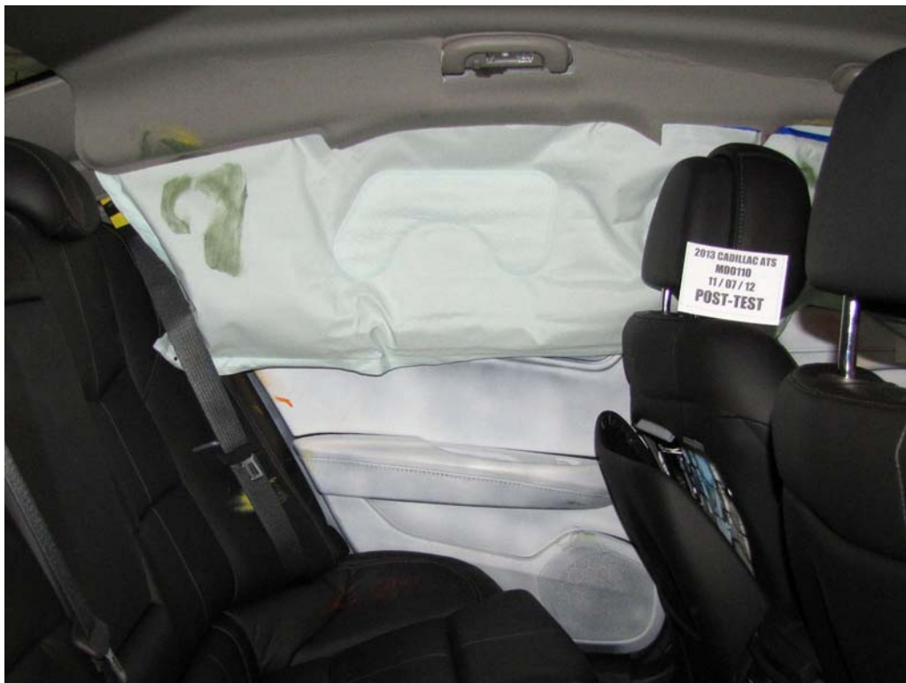
FIGURE 74. Post-Test Rear Passenger Inner Door Panel View
