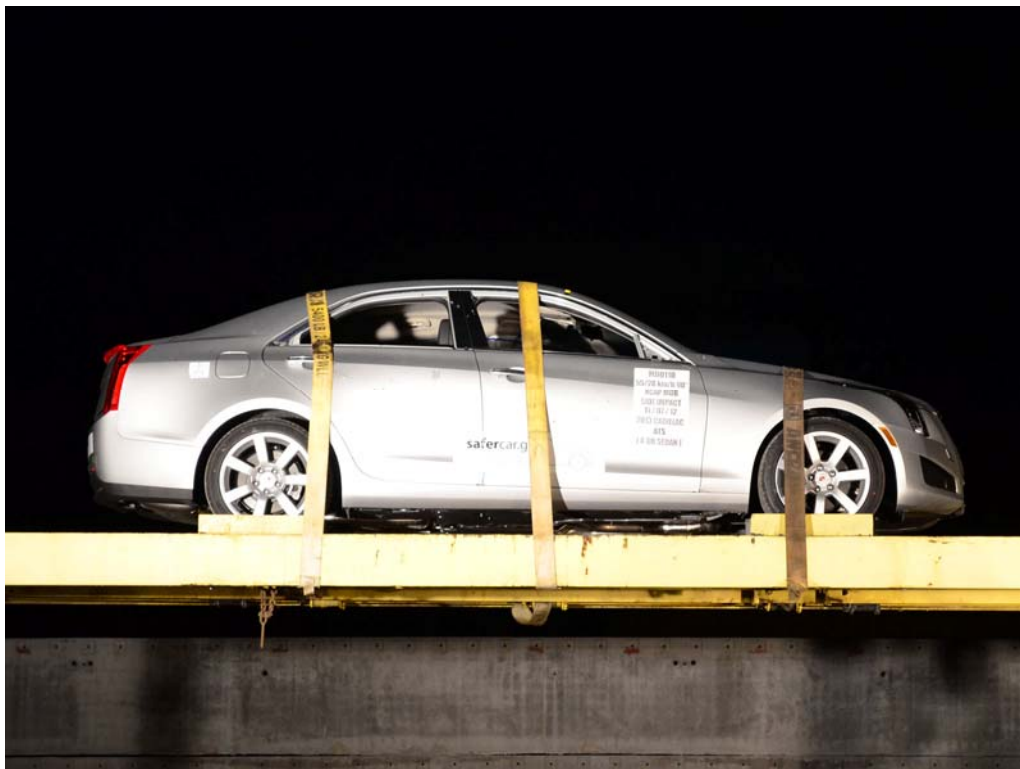
FIGURE 96. FMVSS No. 301 Static Rollover 0 Degrees
