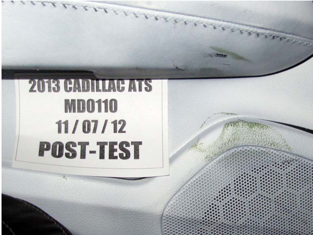
FIGURE 81. Post-Test Rear Passenger Dummy Knee Close-Up View
