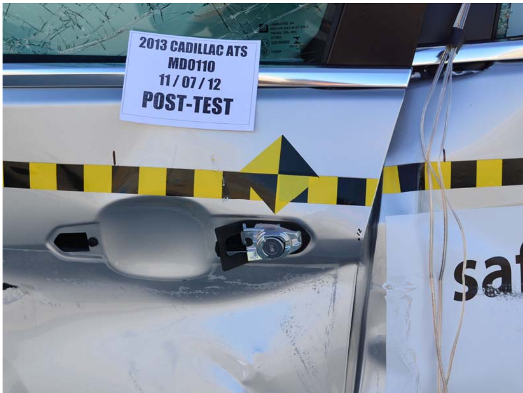
FIGURE 22. Post-Test Left Front Door Latch Close-Up
