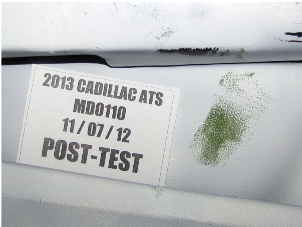
FIGURE 54. Post-Test Driver Dummy Close-Up Knee Contact View
