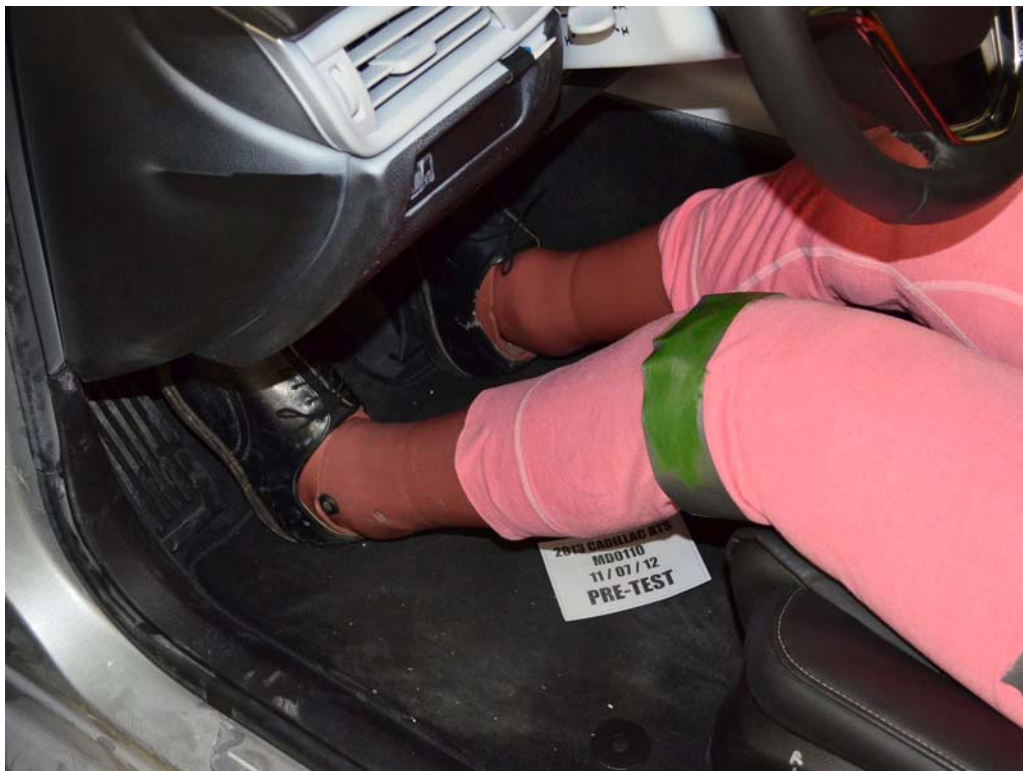
FIGURE 34. Pre-Test Placement of Driver Dummy's Feet
