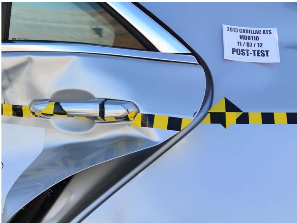
FIGURE 24. Post-Test Left Rear Door Latch Close-Up
