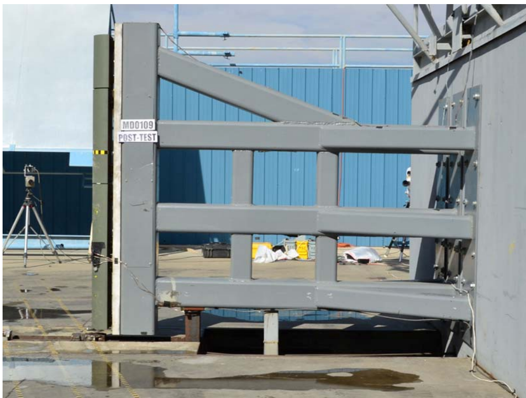
FIGURE 60. Post-Test Pole Barrier Side View
