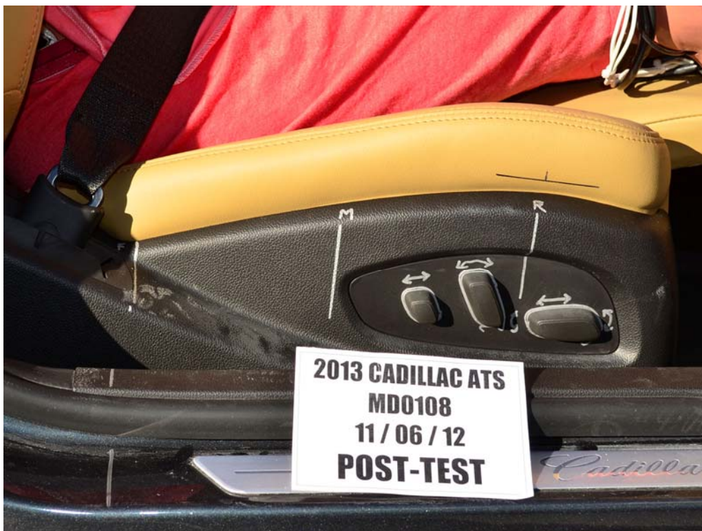
FIGURE 57. Post-Test Passenger's Seat Fore-Aft Markings
