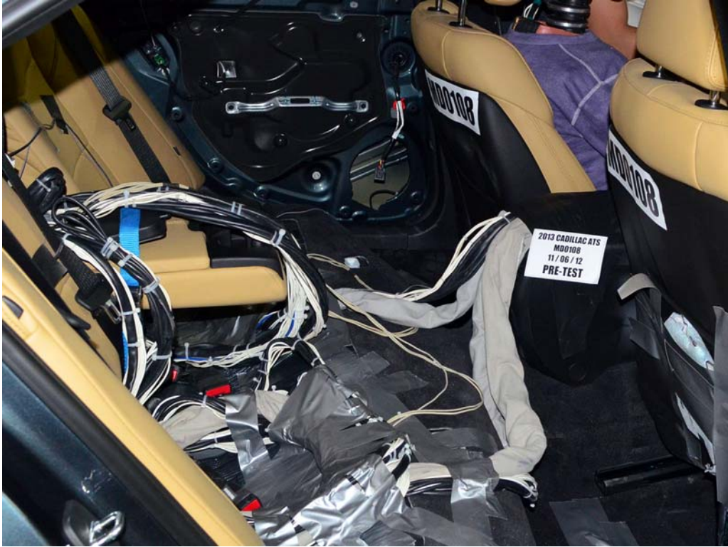
FIGURE 27. Pre-Test Dummy Cable Routing
