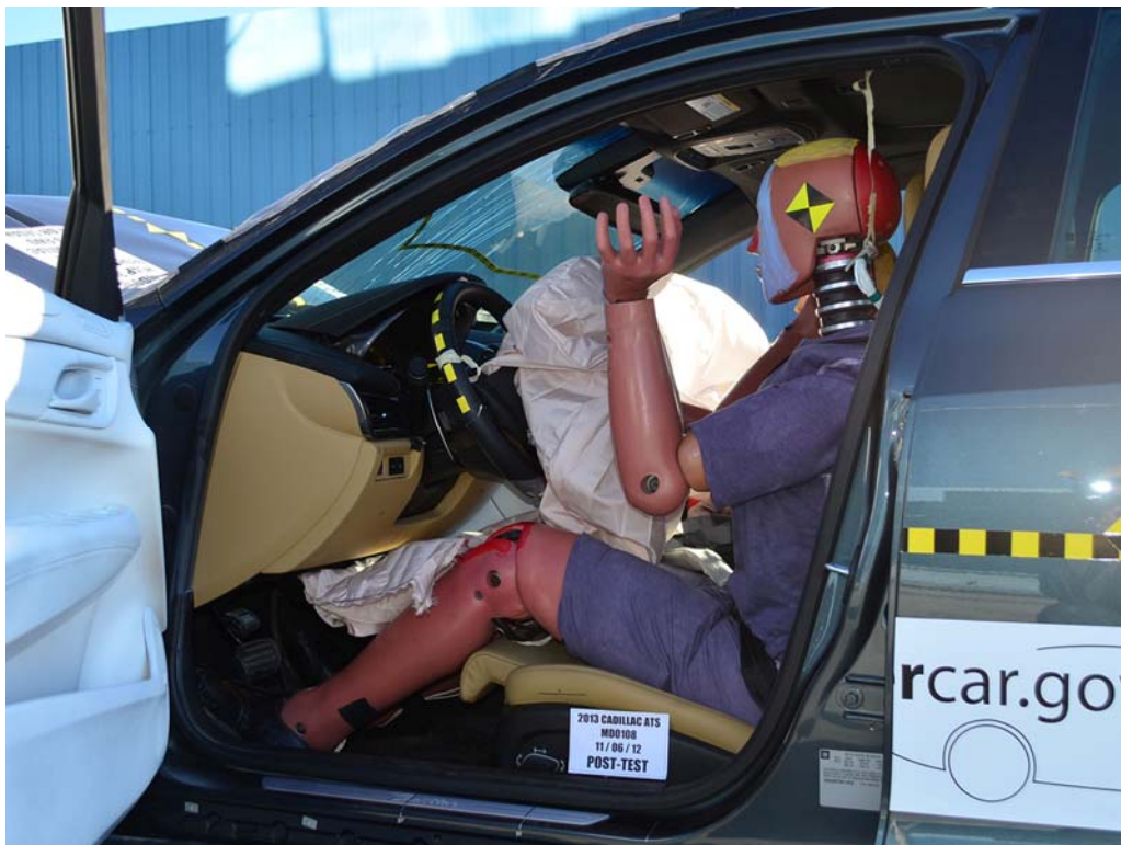
FIGURE 34. Post-Test Driver Dummy and Vehicle Interior View
