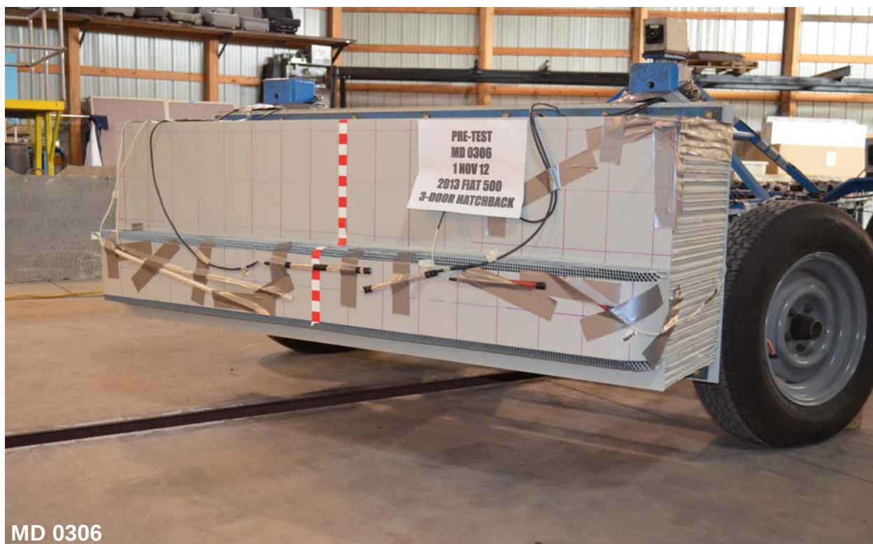
Figure A-88: Pre-Test Left Side View of MDB Impactor Face
