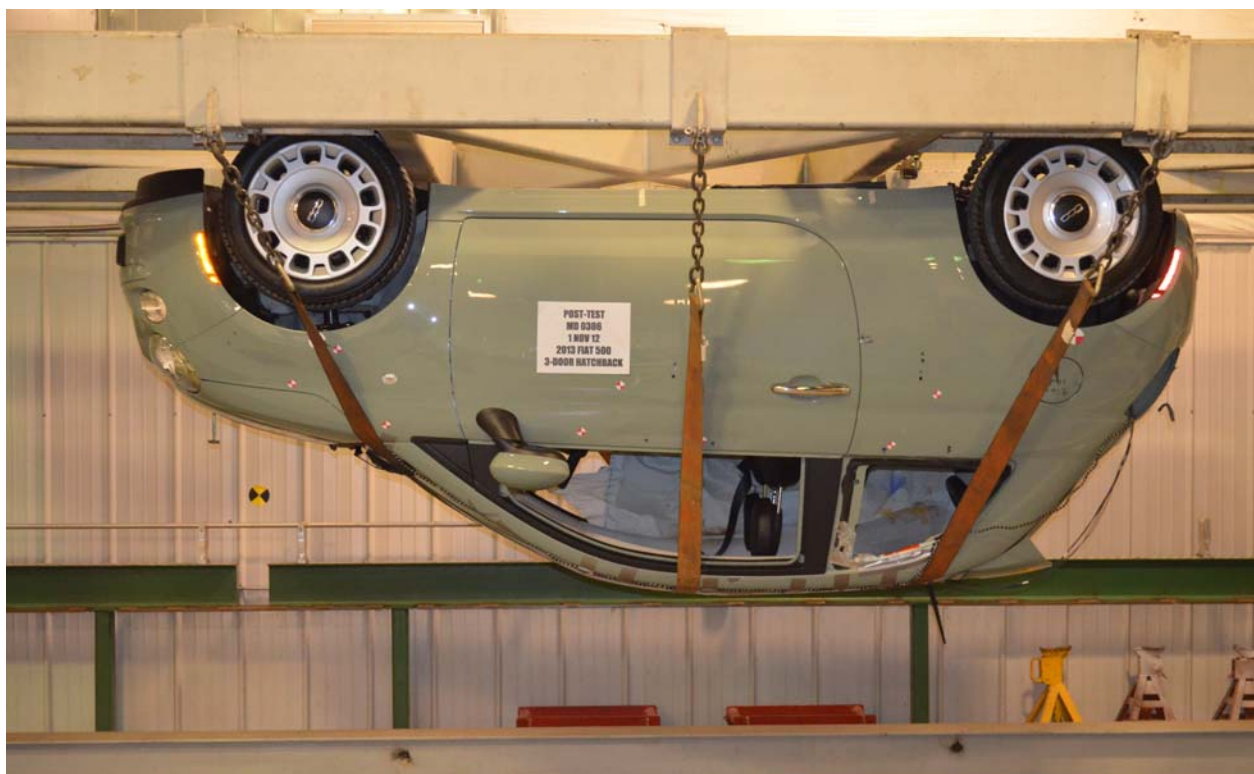
Figure A-98: FMVSS No. 301 Static Rollover 180 Degrees
