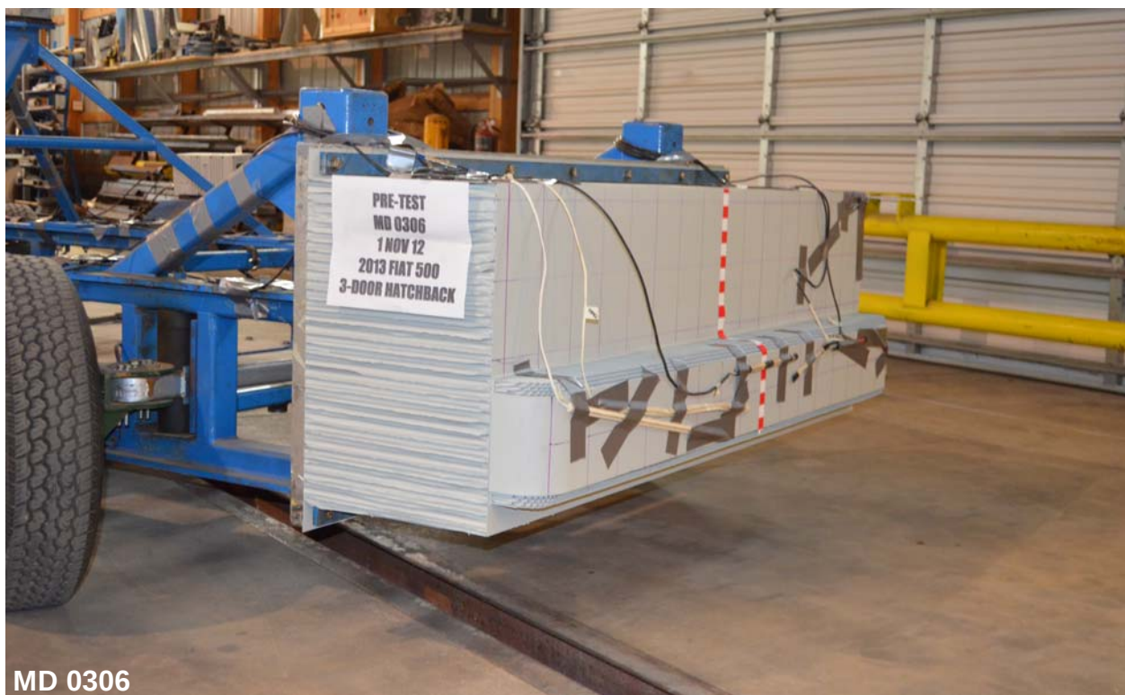
Figure A-90: Pre-Test Right Side View of MDB Impactor Face
