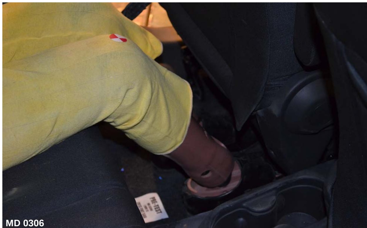
Figure A-64: Pre-Test Placement of Rear Passenger Dummy's Feet
