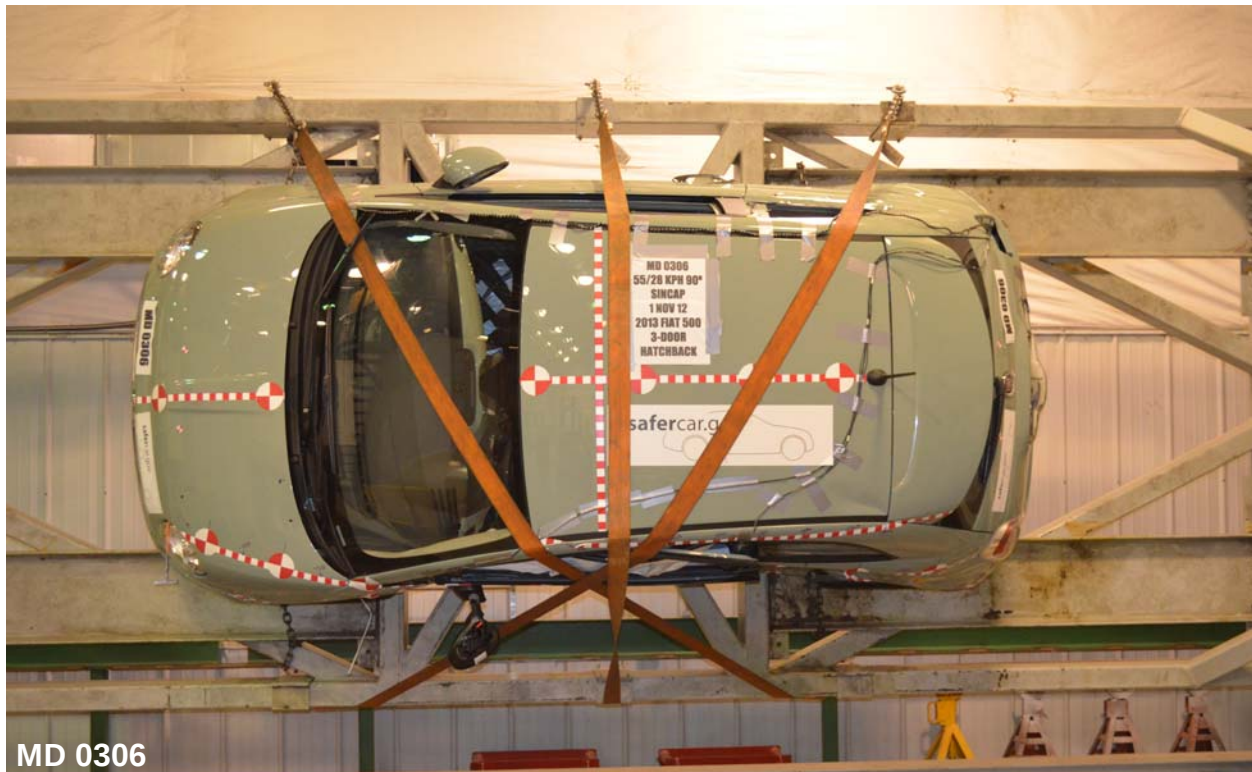
Figure A-99: FMVSS No. 301 Static Rollover 270 Degrees
