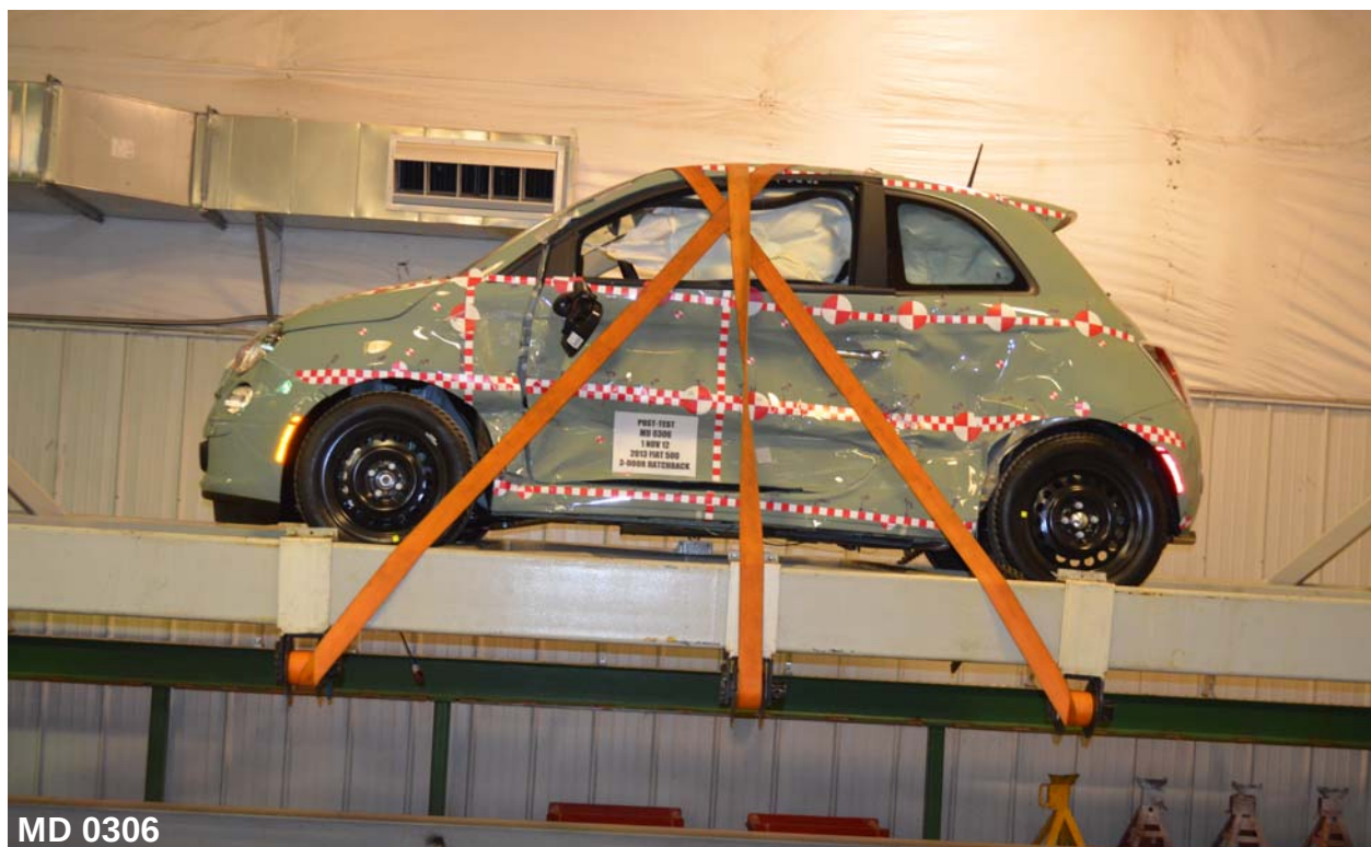
Figure A-96: FMVSS No. 301 Static Rollover 0 Degrees
