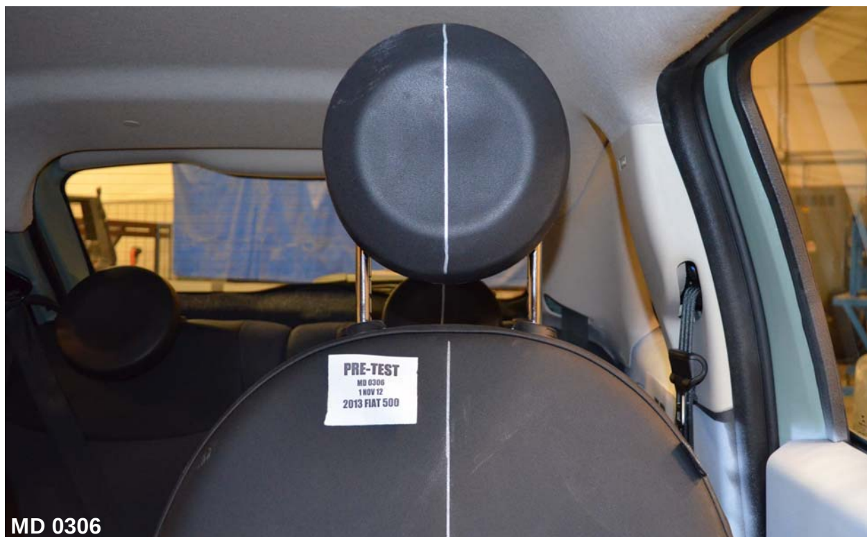
Figure A-30: Pre-Test Frontal View of Driver Seat Back Prior to Dummy Positioning
