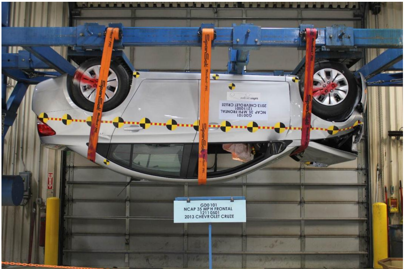
Vehicle at 180° on Static Rollover Device
