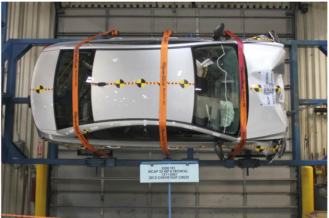
Vehicle at 90° on Static Rollover Device
