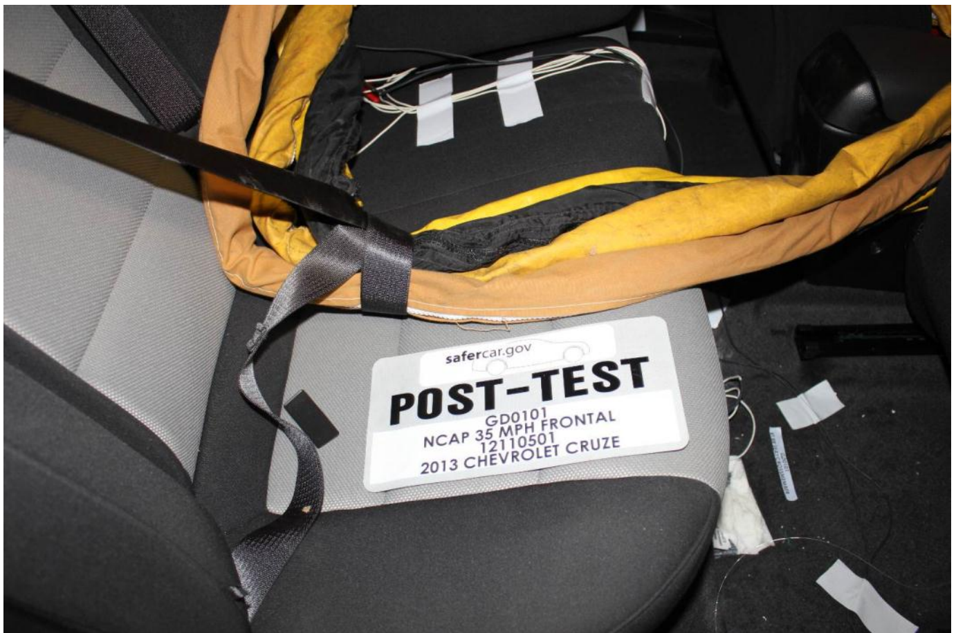
Post-Test Dummy Cable Routing
