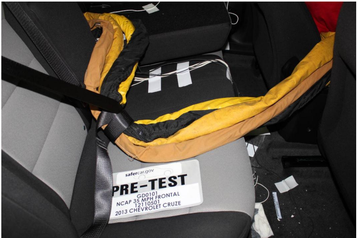
Pre-Test Dummy Cable Routing
