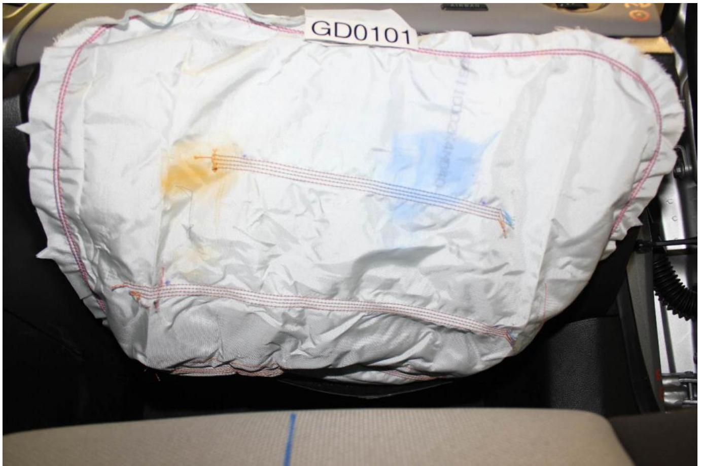
Post-Test Passenger Dummy Contact with Knee Airbag
