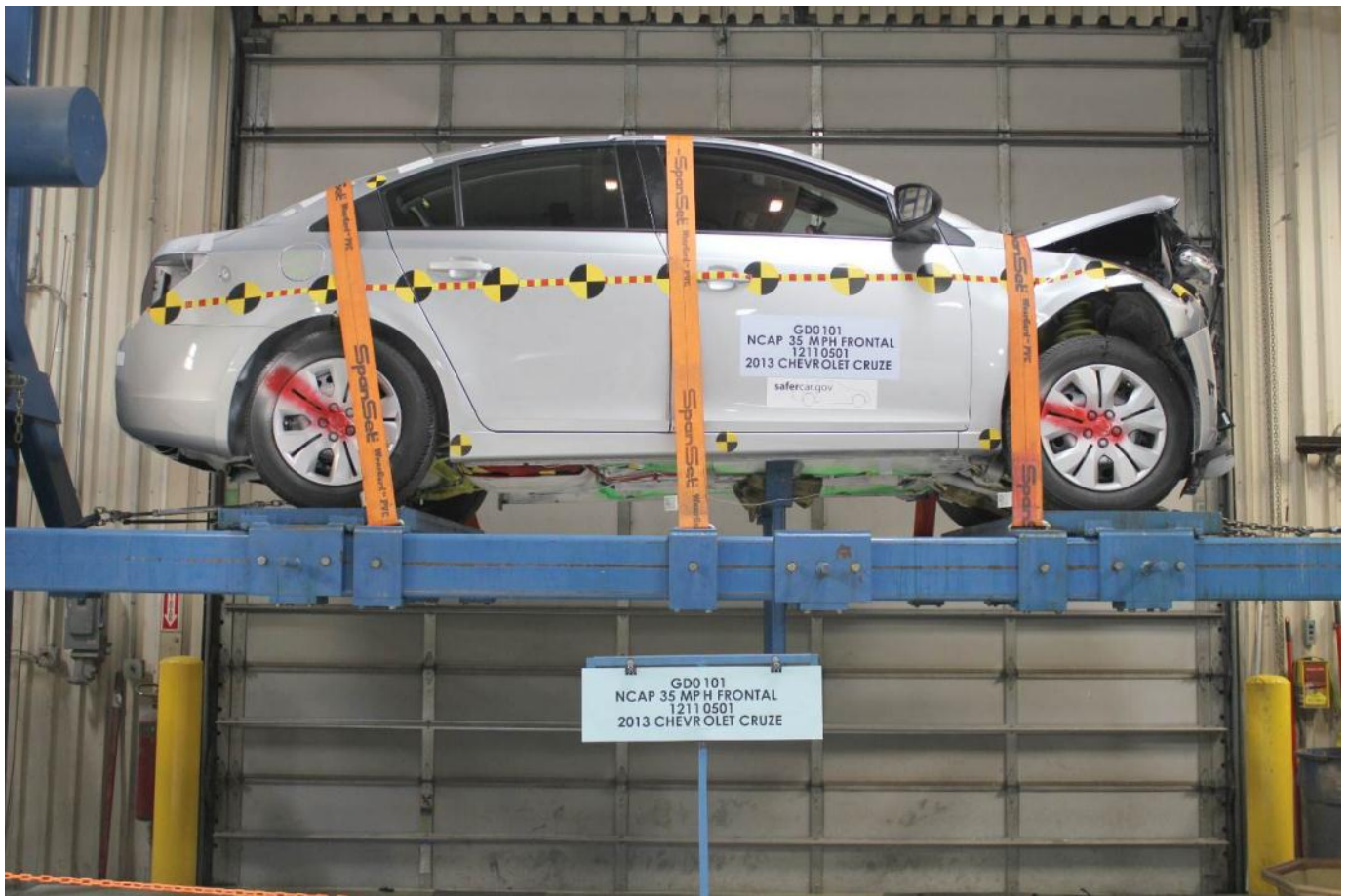
Vehicle at 360° on Static Rollover Device
