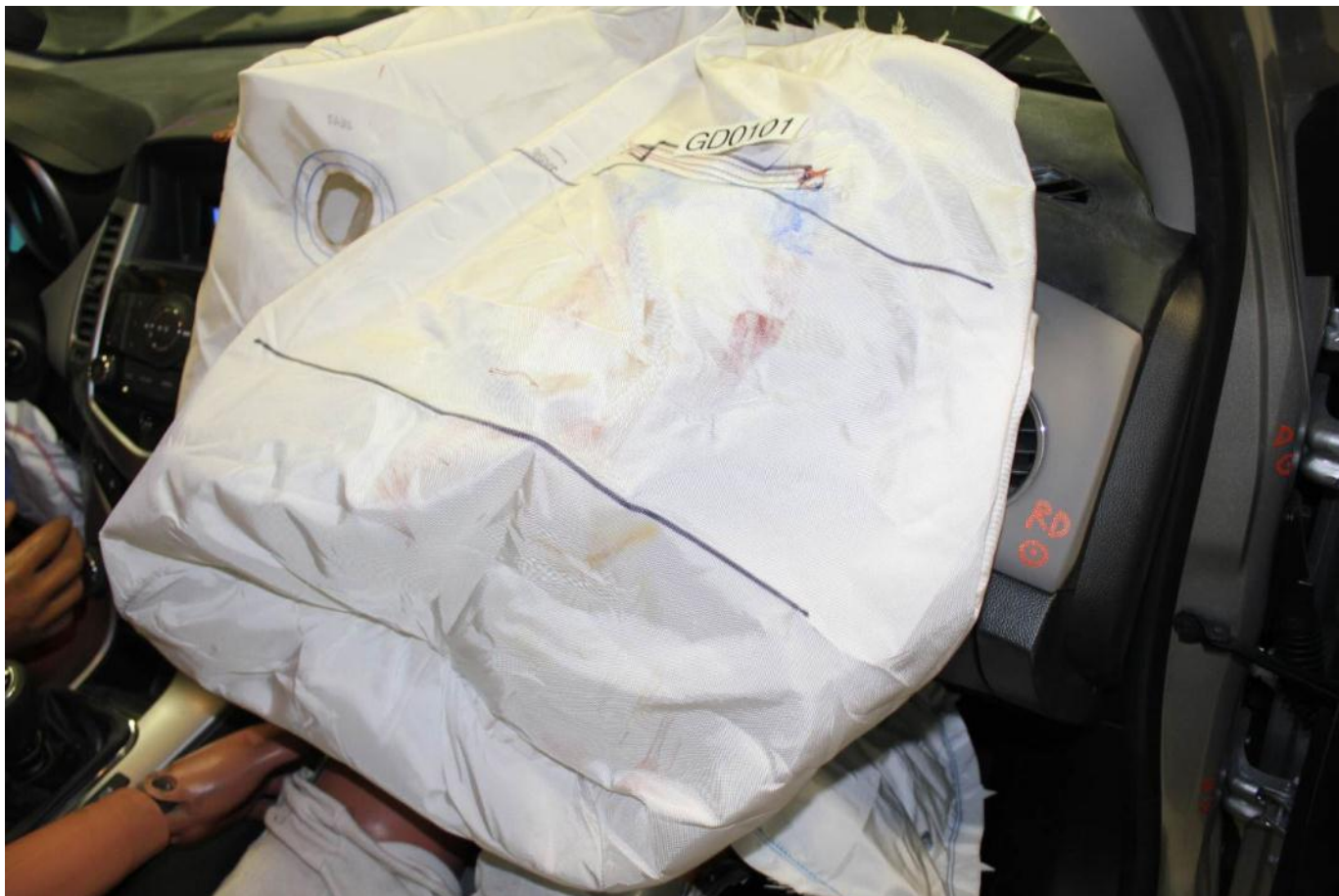
Post-Test Passenger Dummy Contact with Airbag
