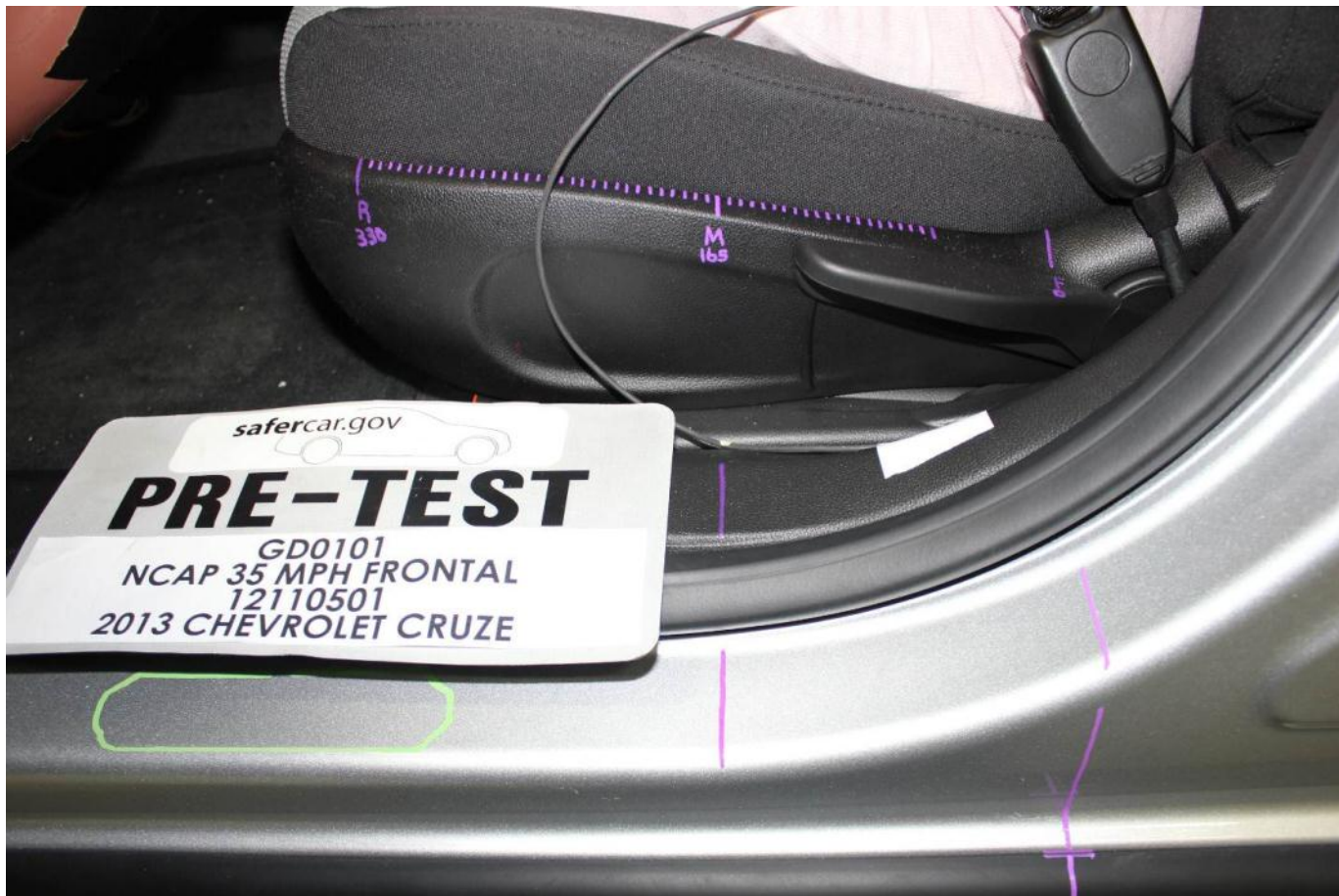
Pre-Test Driver's Seat Fore-Aft Markings
