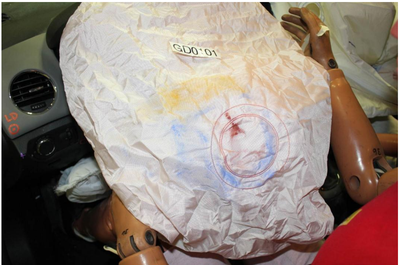
Post-Test Driver Dummy Contact with Airbag
