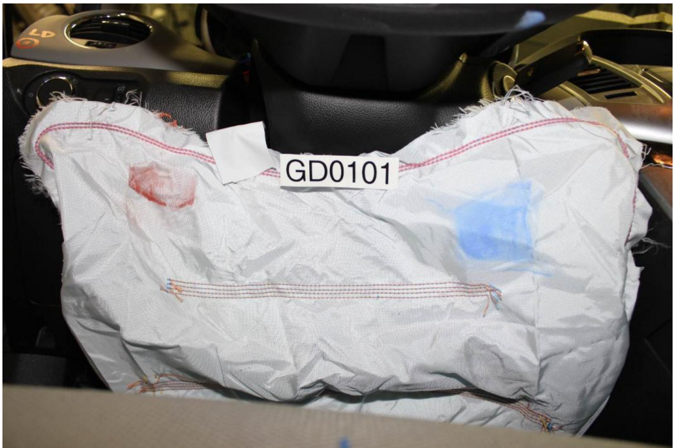
Post-Test Driver Dummy Contact with Knee Airbag
