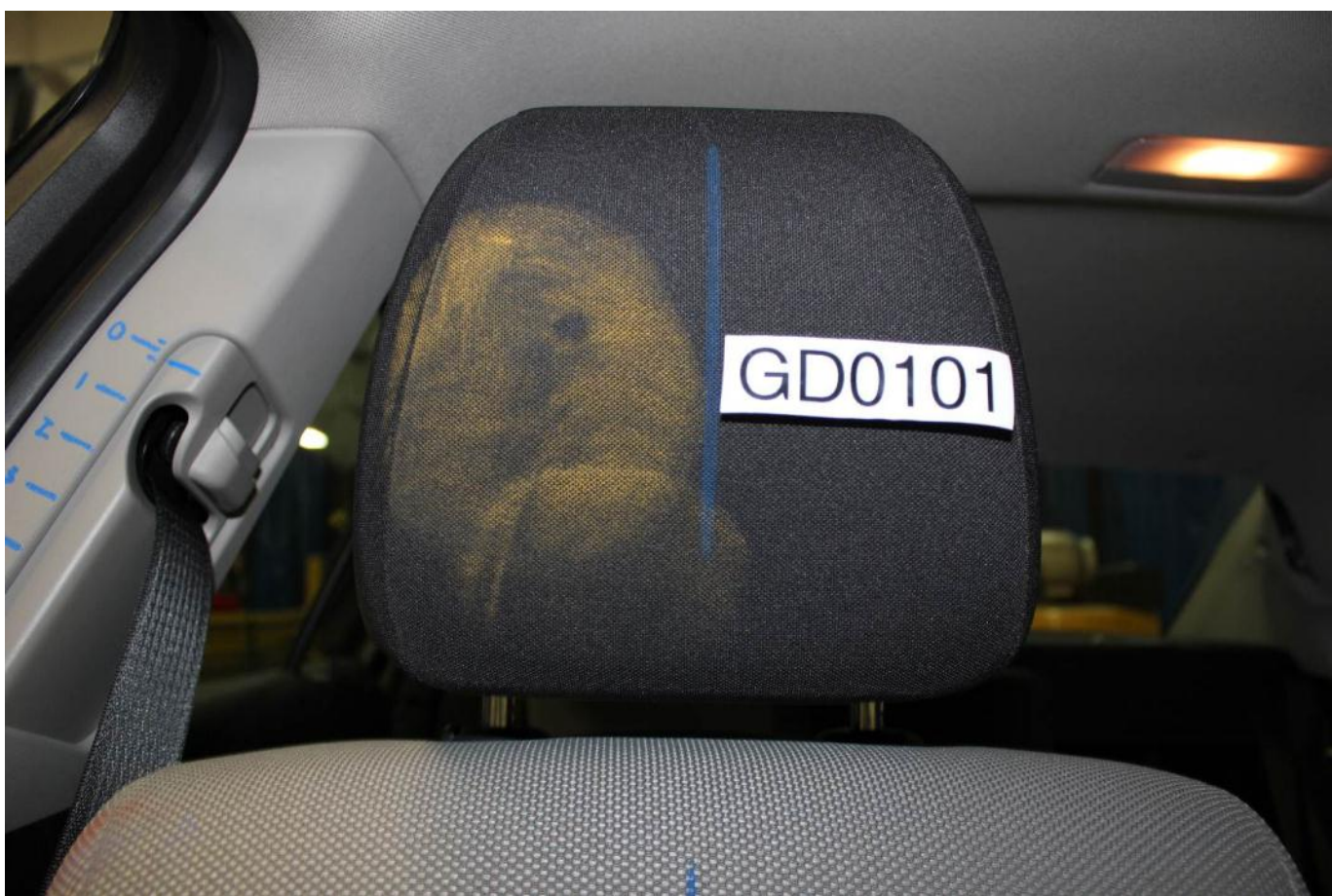
Post-Test Passenger Dummy Contact with Headrest
