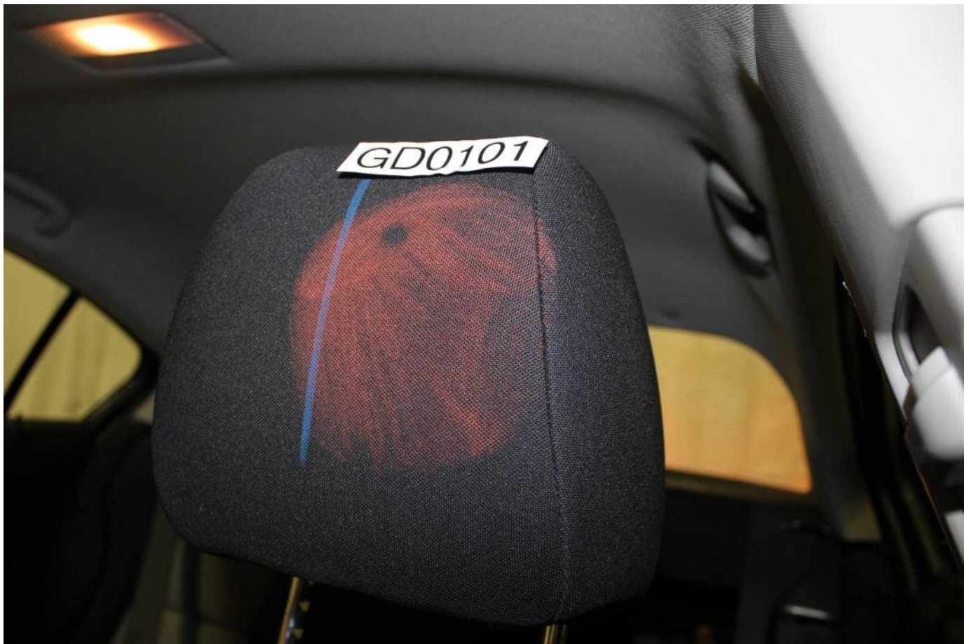
Post-Test Driver Dummy Contact with Headrest
