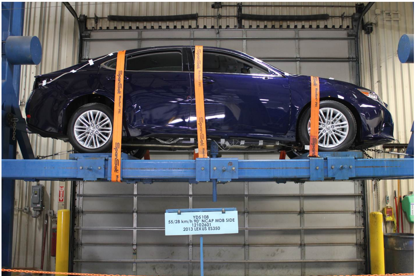
FMVSS No. 301 Static Rollover 0 Degrees
