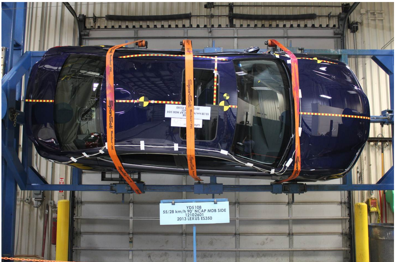
FMVSS No. 301 Static Rollover 270 Degrees
