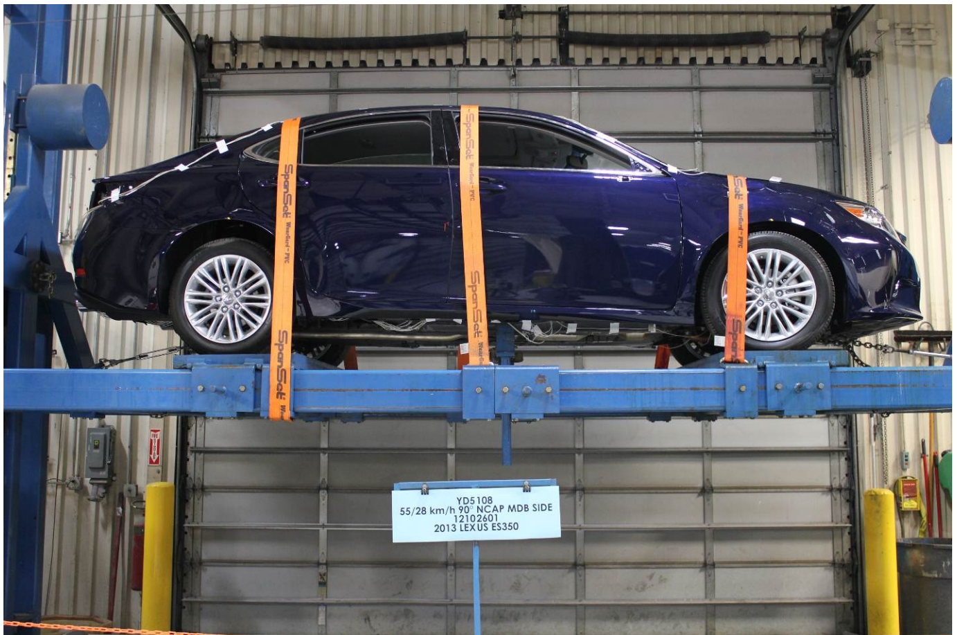
FMVSS No. 301 Static Rollover 360 Degrees
