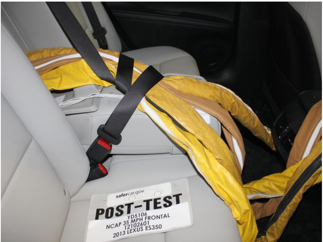
Post-Test Dummy Cable Routing
