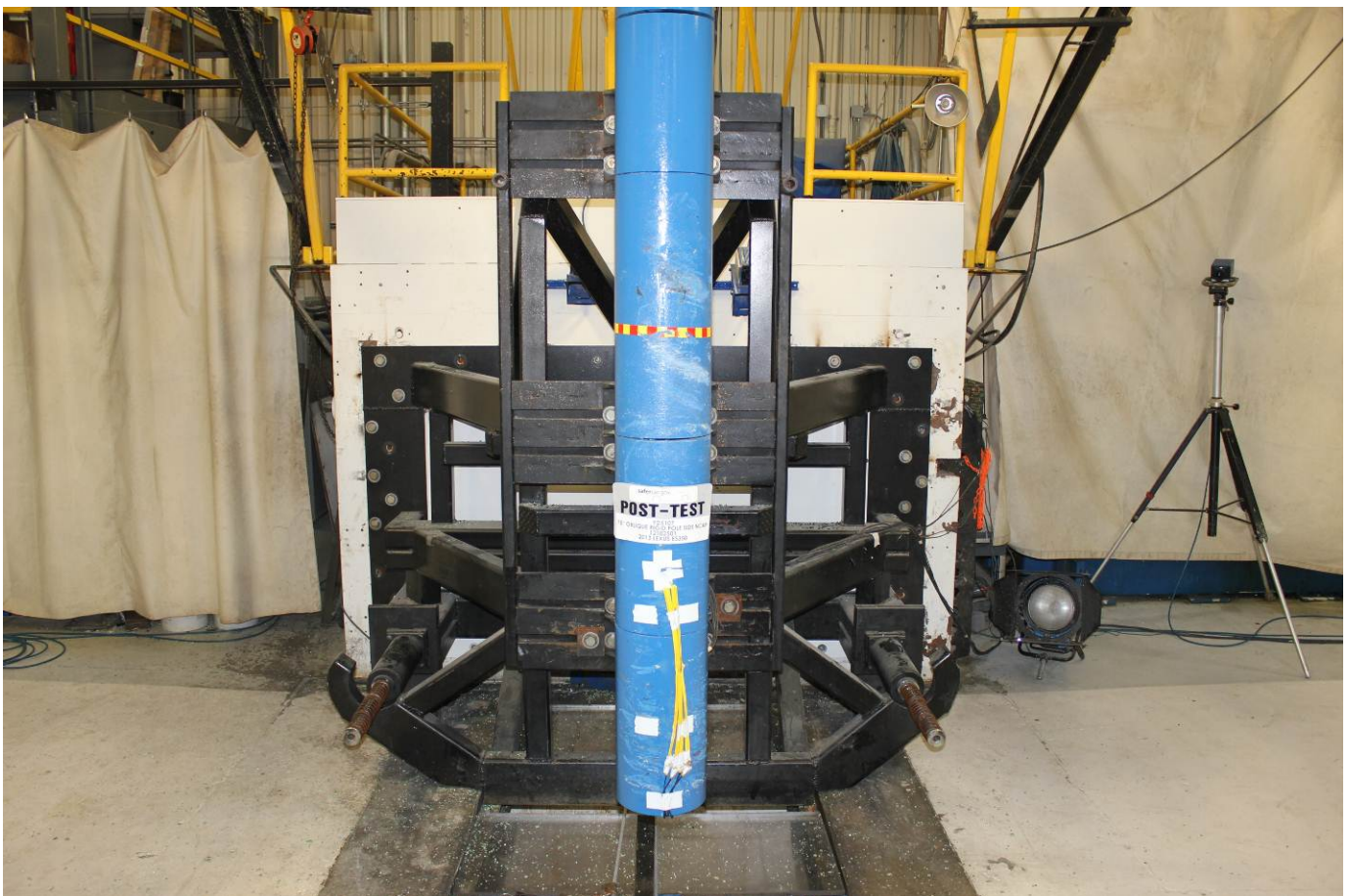
Post-Test Pole Barrier Front View
