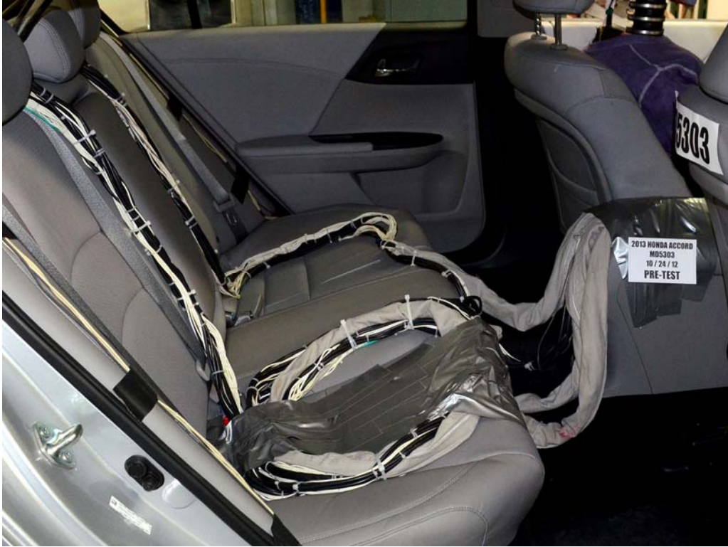
FIGURE 27. Pre-Test Dummy Cable Routing
