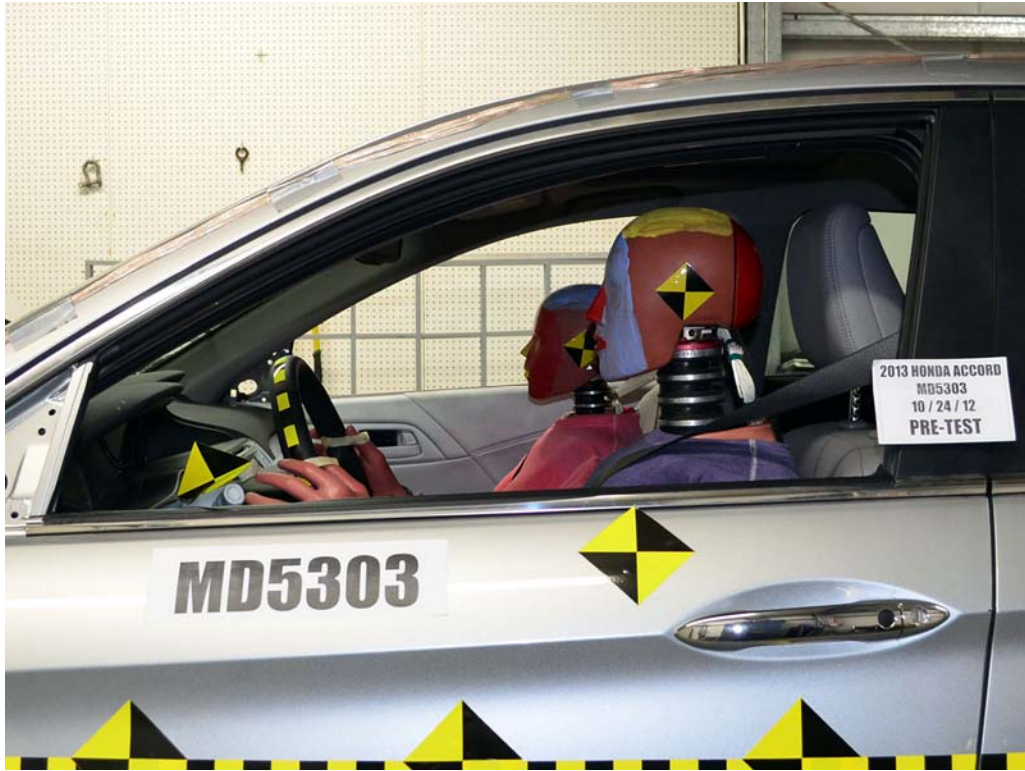
FIGURE 31. Pre-Test Driver Dummy Window View
