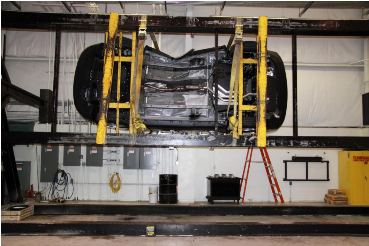
066 FMVSS No. 301 Static Rollover 270 Degrees
