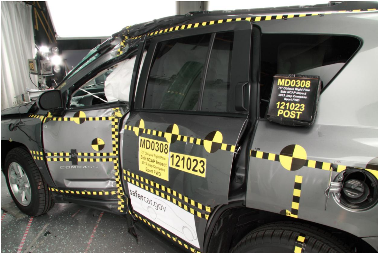
018a Post-Test Right Side View of Pole Positioned Against Side of Vehicle
