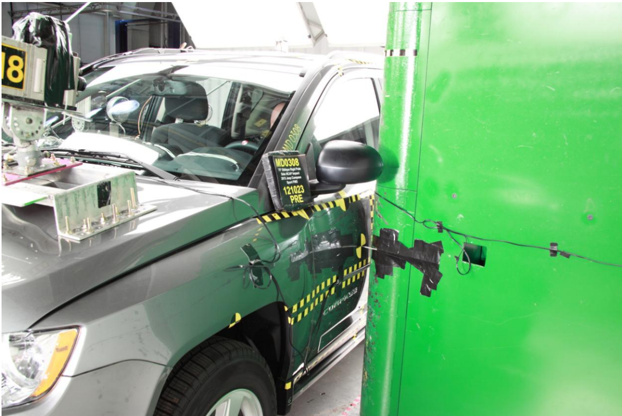
017 Pre-Test Left Side View of Pole Positioned Against Side of Vehicle
