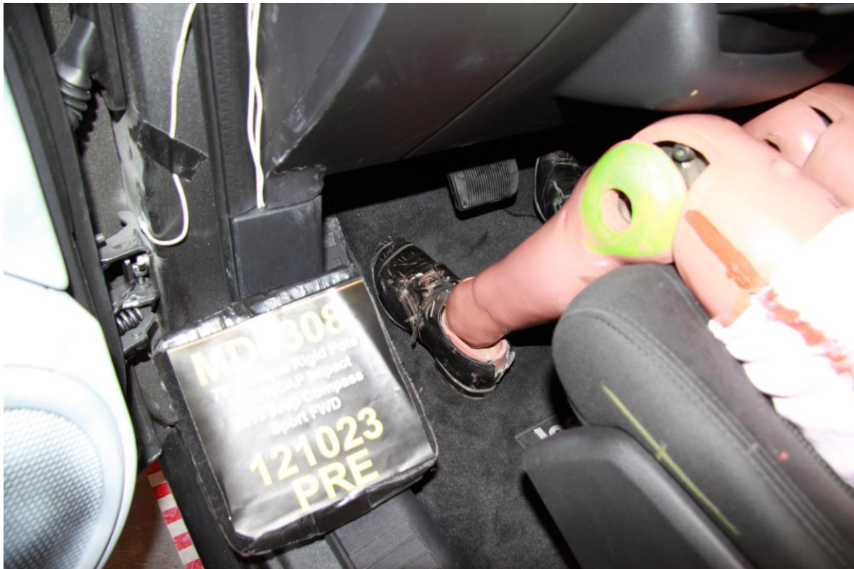
032 Pre-Test Placement of Dummy Feet
