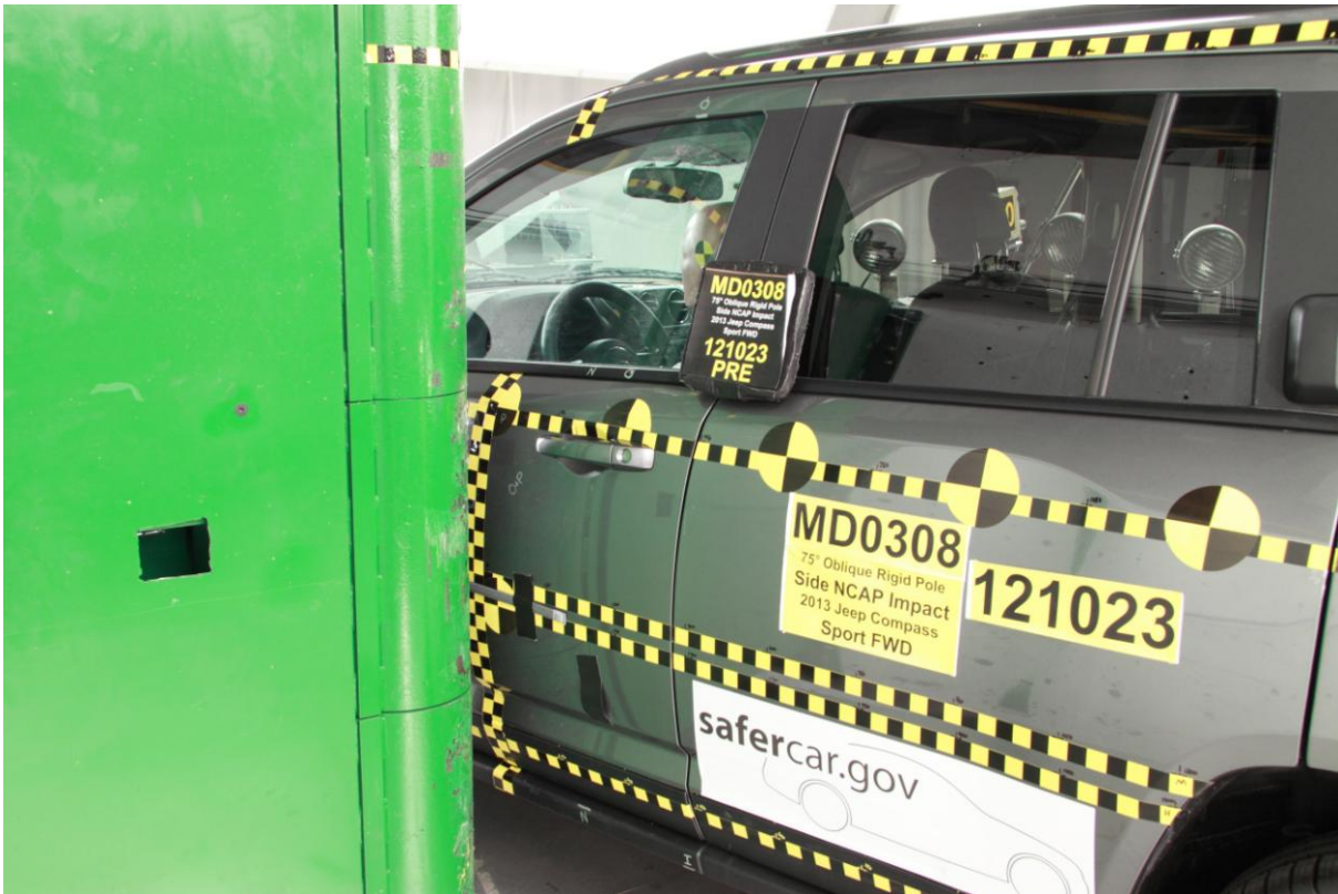
018 Pre-Test Right Side View of Pole Positioned Against Side of Vehicle
