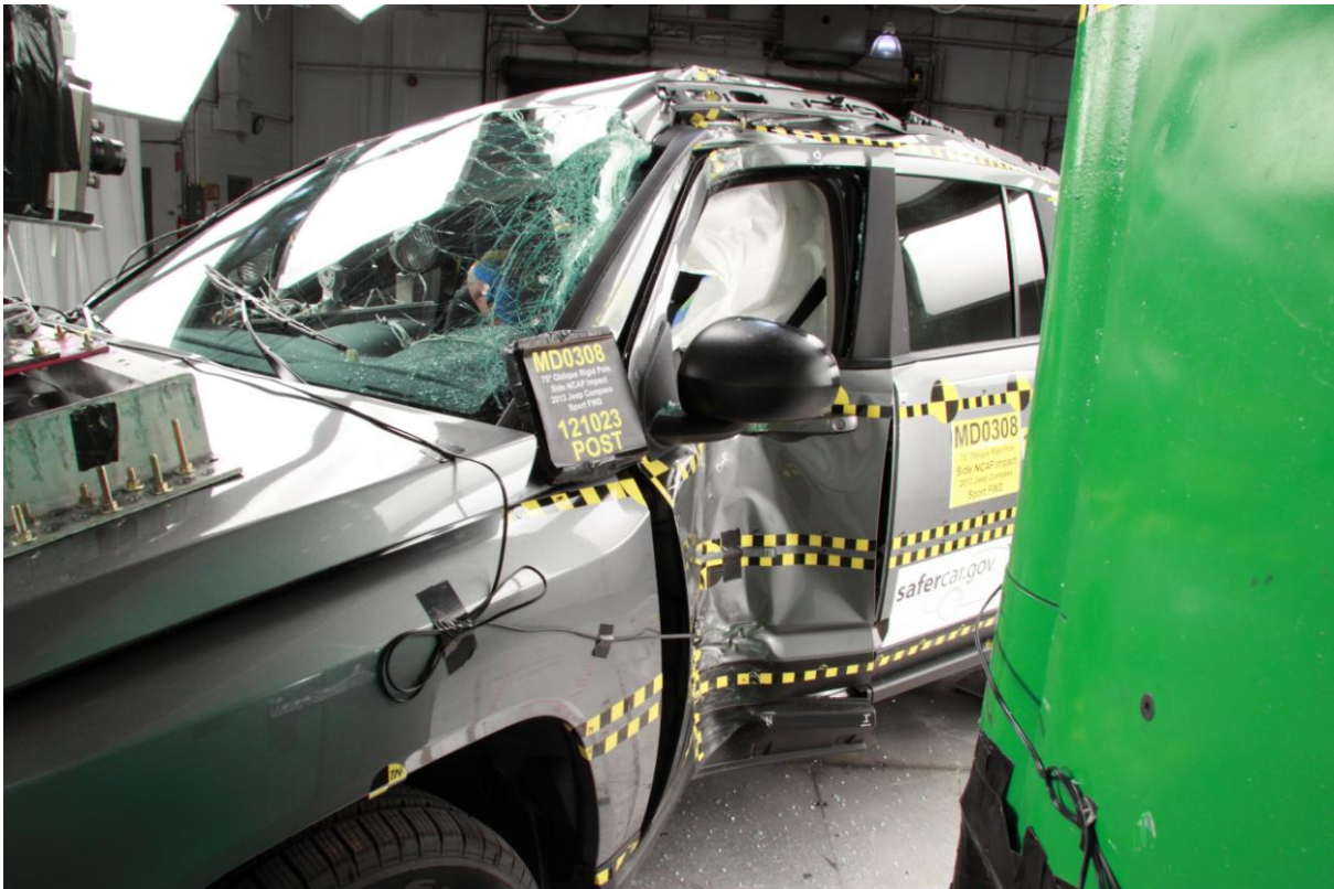
017a Post-Test Left Side View of Pole Positioned Against Side of Vehicle
