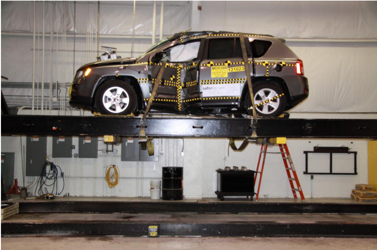
063 FMVSS No. 301 Static Rollover 0 Degrees
