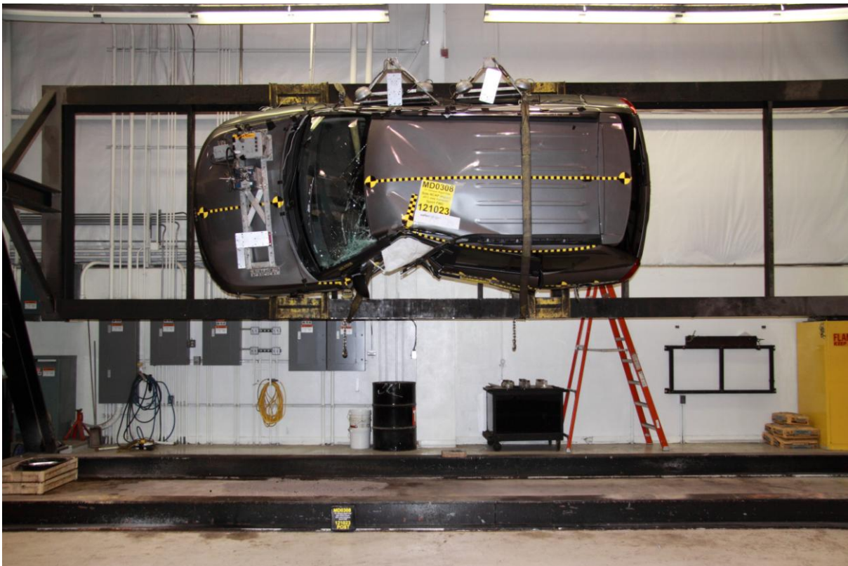
064 FMVSS No. 301 Static Rollover 90 Degrees
