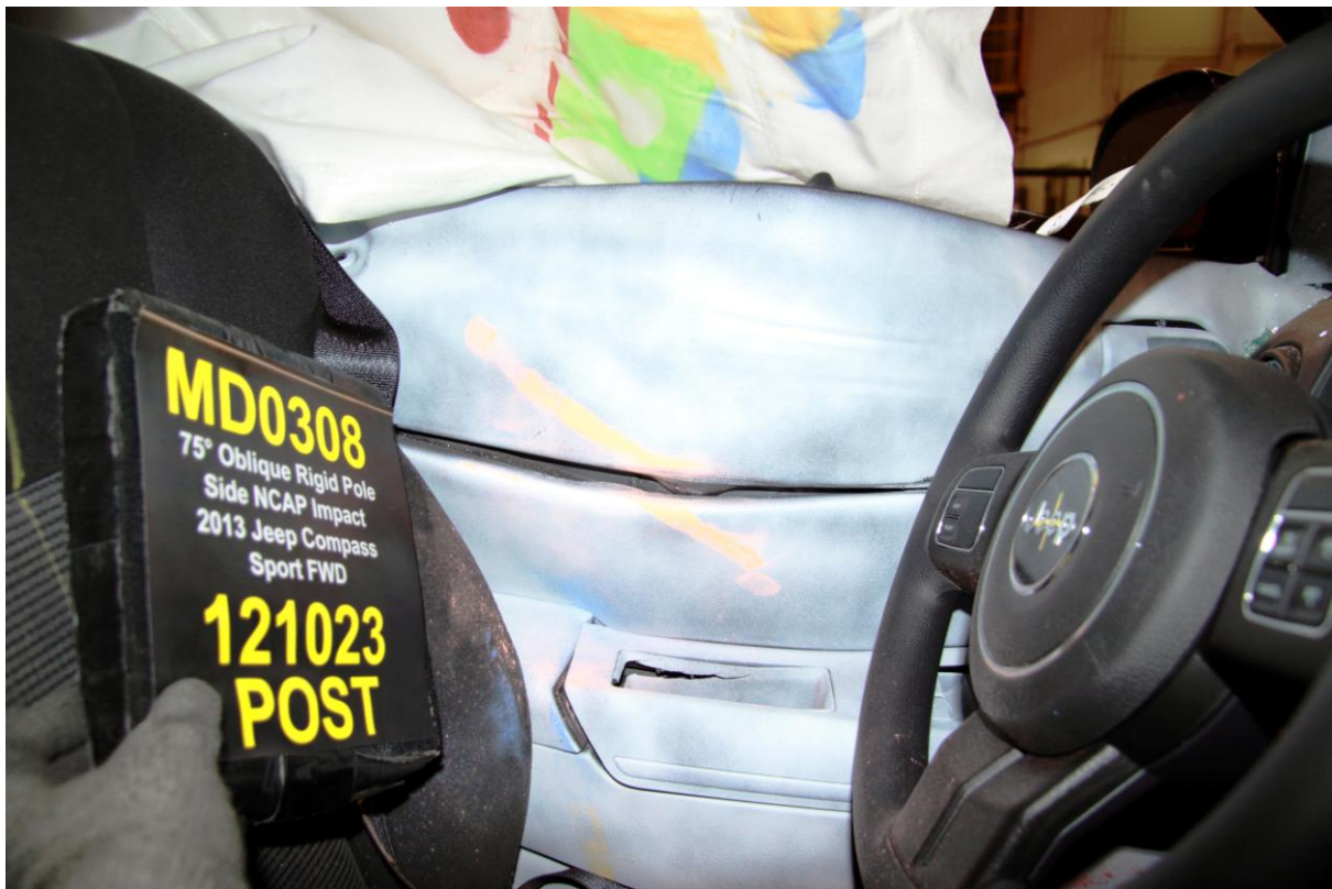
048 Post-Test Dummy Close-Up Torso Contact with Vehicle Interior View
