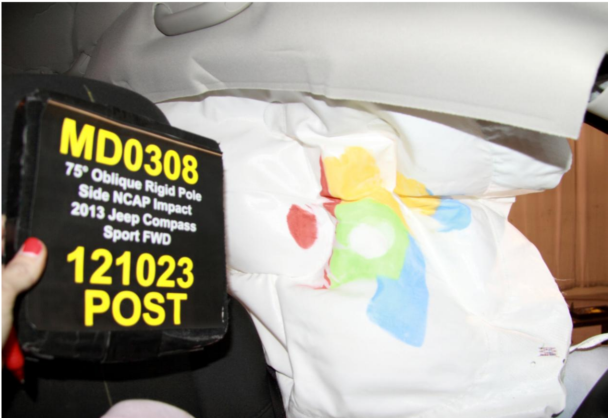
046 Post-Test Dummy Close-Up Head Contact with Vehicle View
