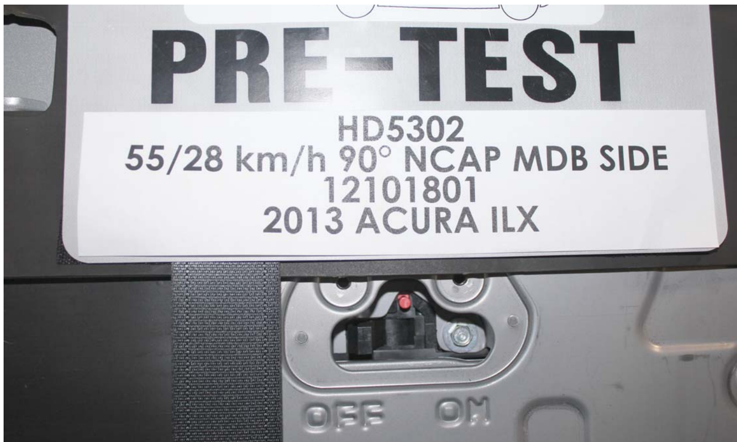
No. 007 Manual High Voltage Service Disconnect Removed
