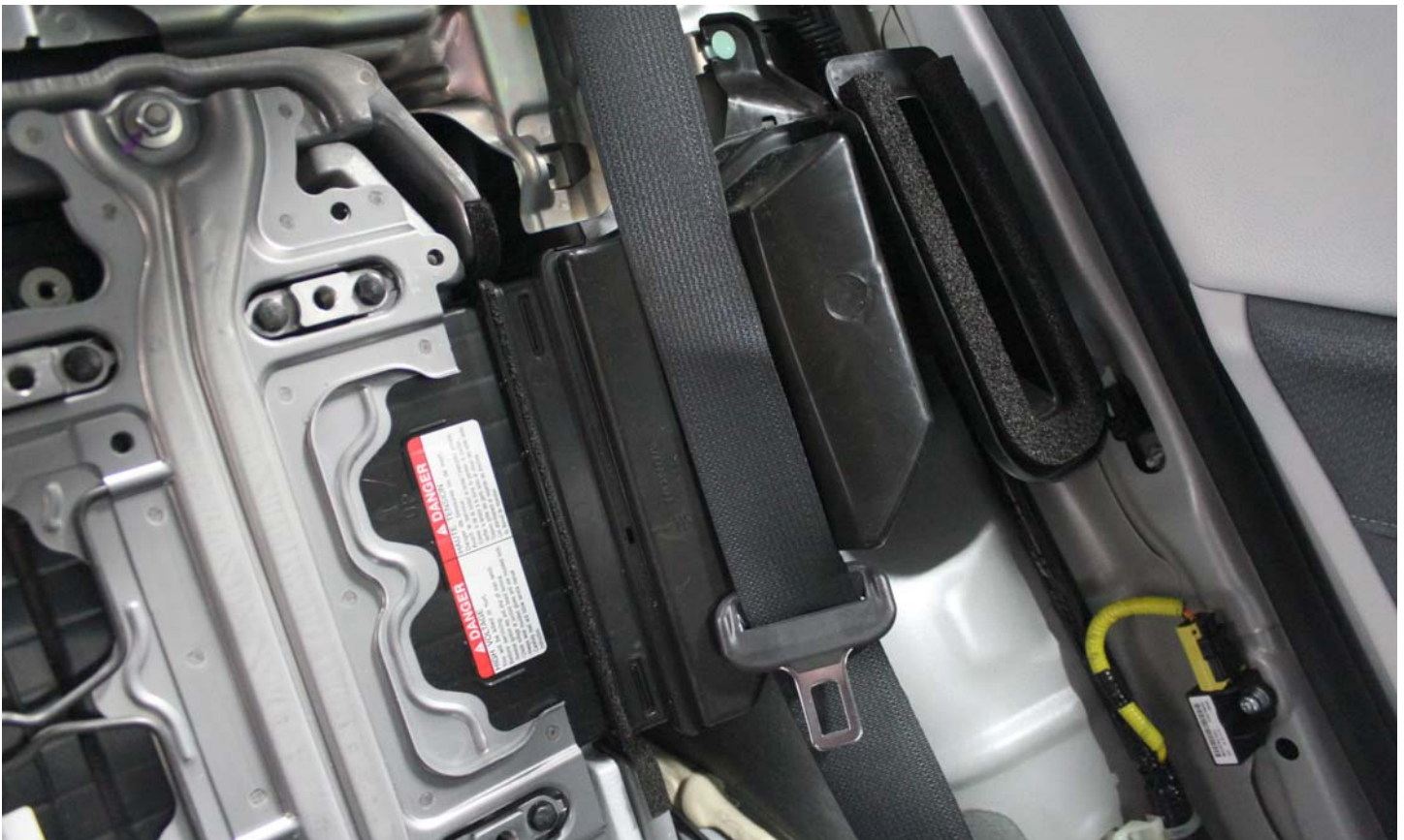
No. 019 Pre-Impact View Propulsion Battery Venting System(s)
