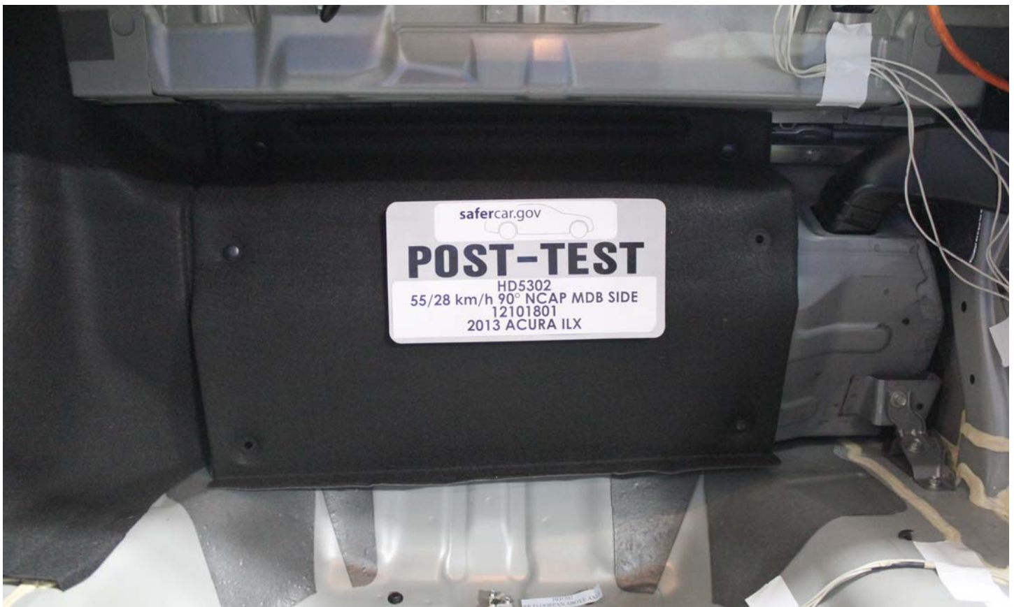
No. 011 Post-Impact Rear View of Propulsion Battery
