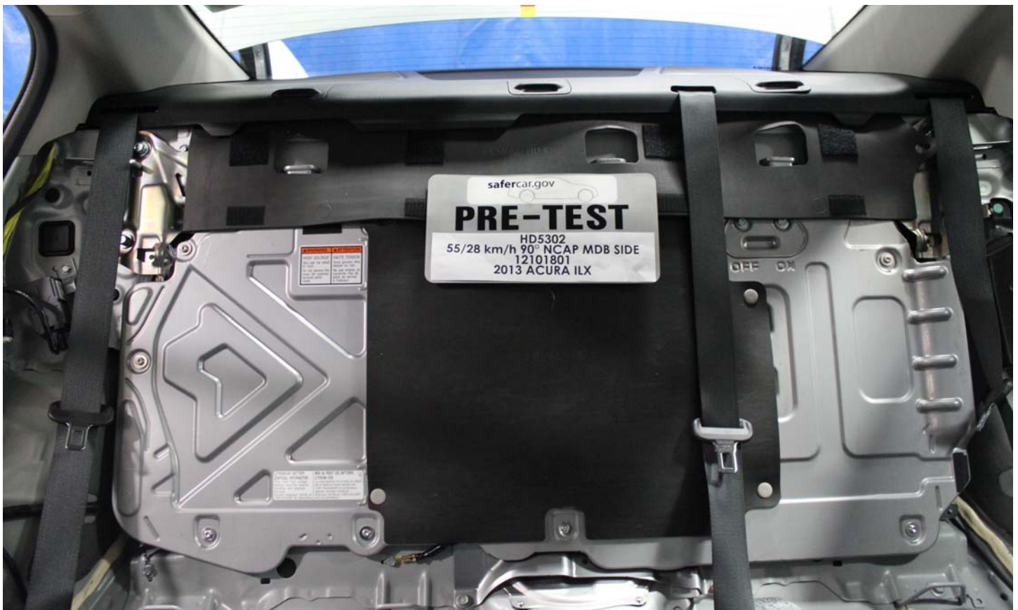
No. 009 Pre-Impact View of Propulsion Battery
