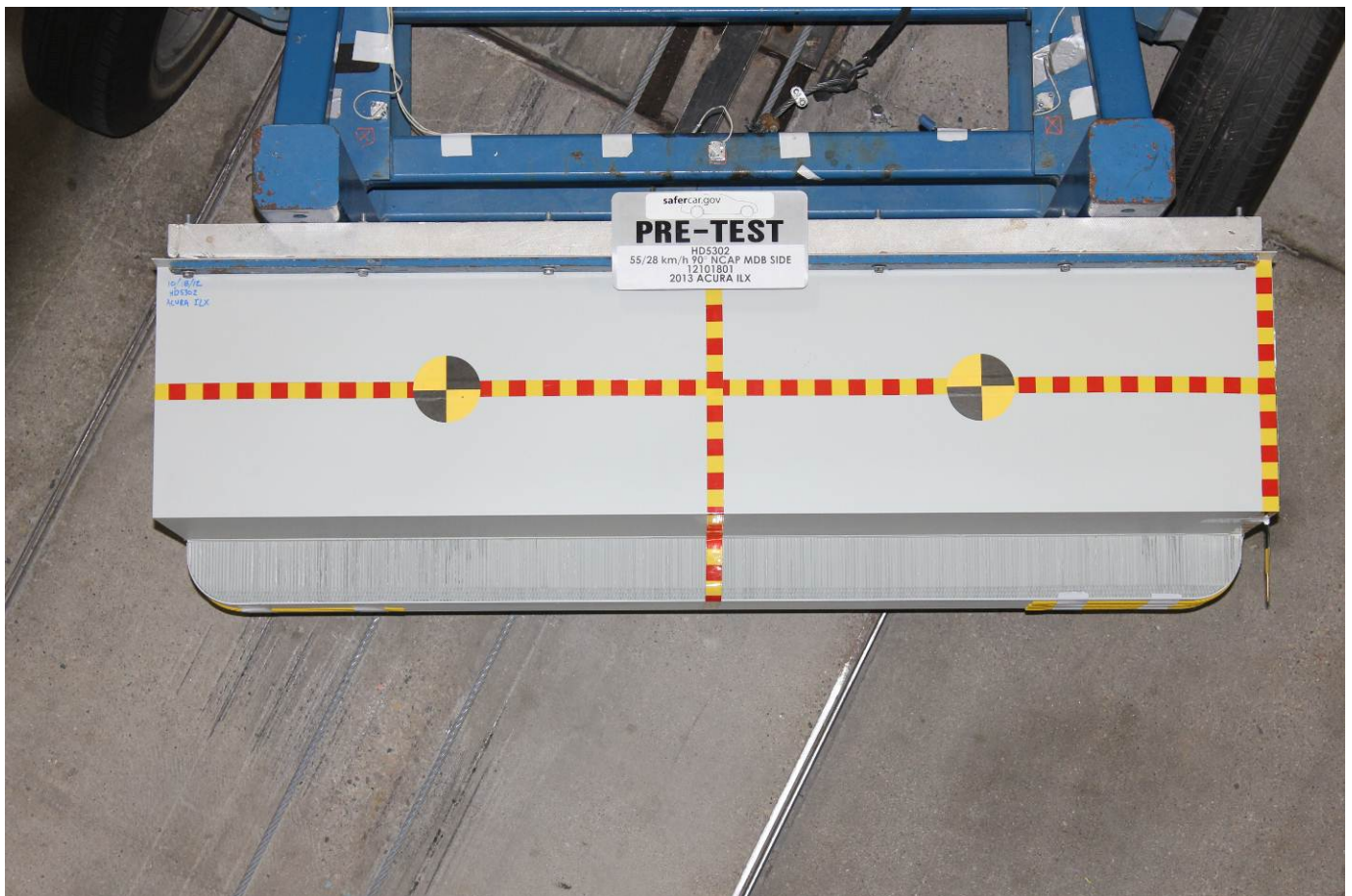
Pre-Test Top View of MDB Impactor Face
