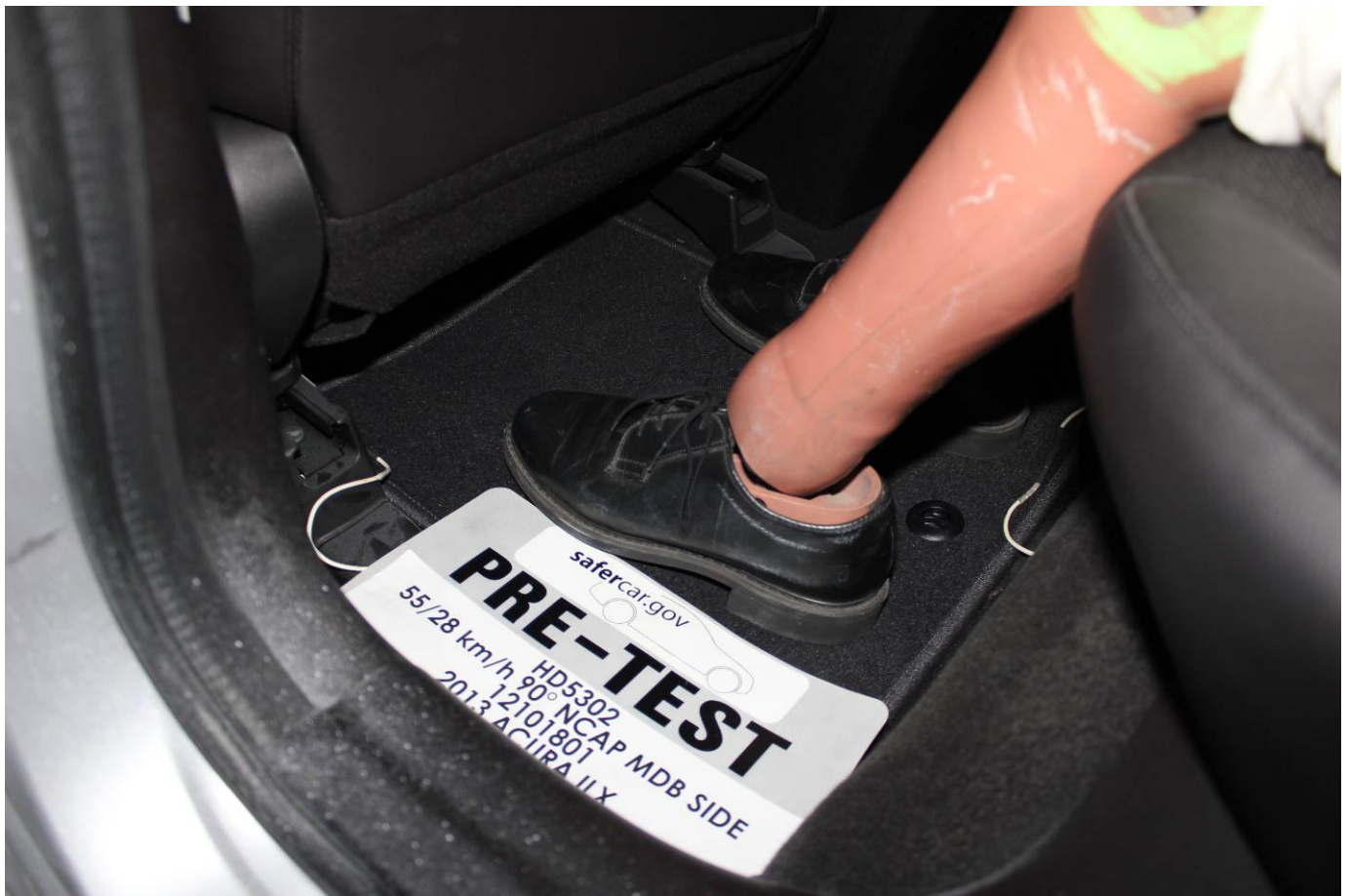
Pre-Test Placement of Rear Passenger Dummy's Feet
