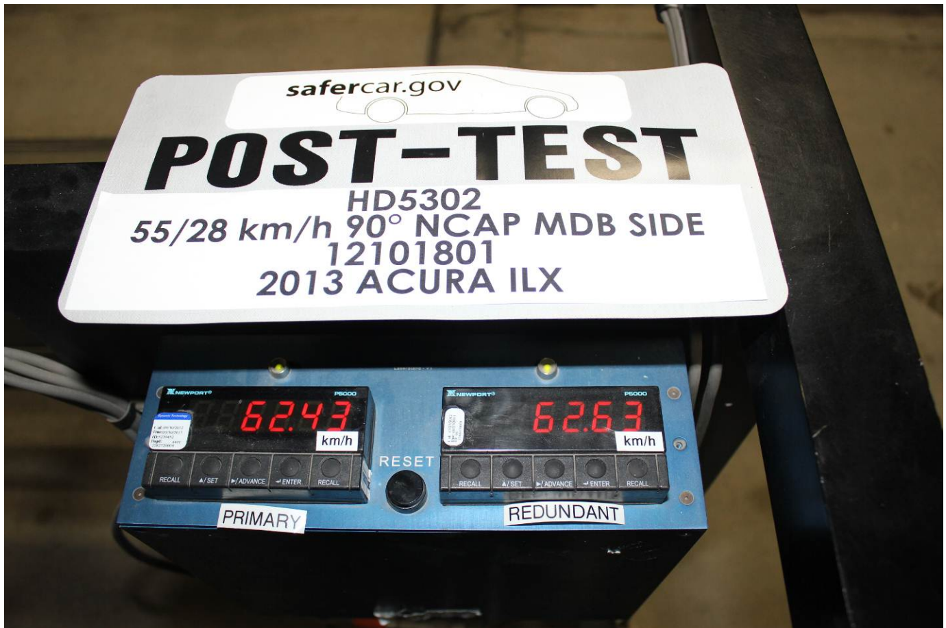
Post-Test Primary and Redundant Speed Trap Read-Out
