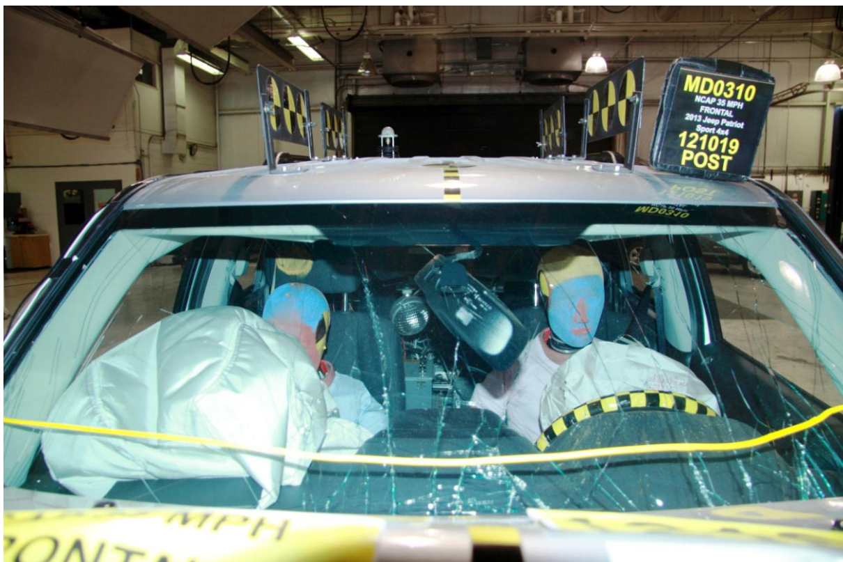
018 Post-test Windshield View
