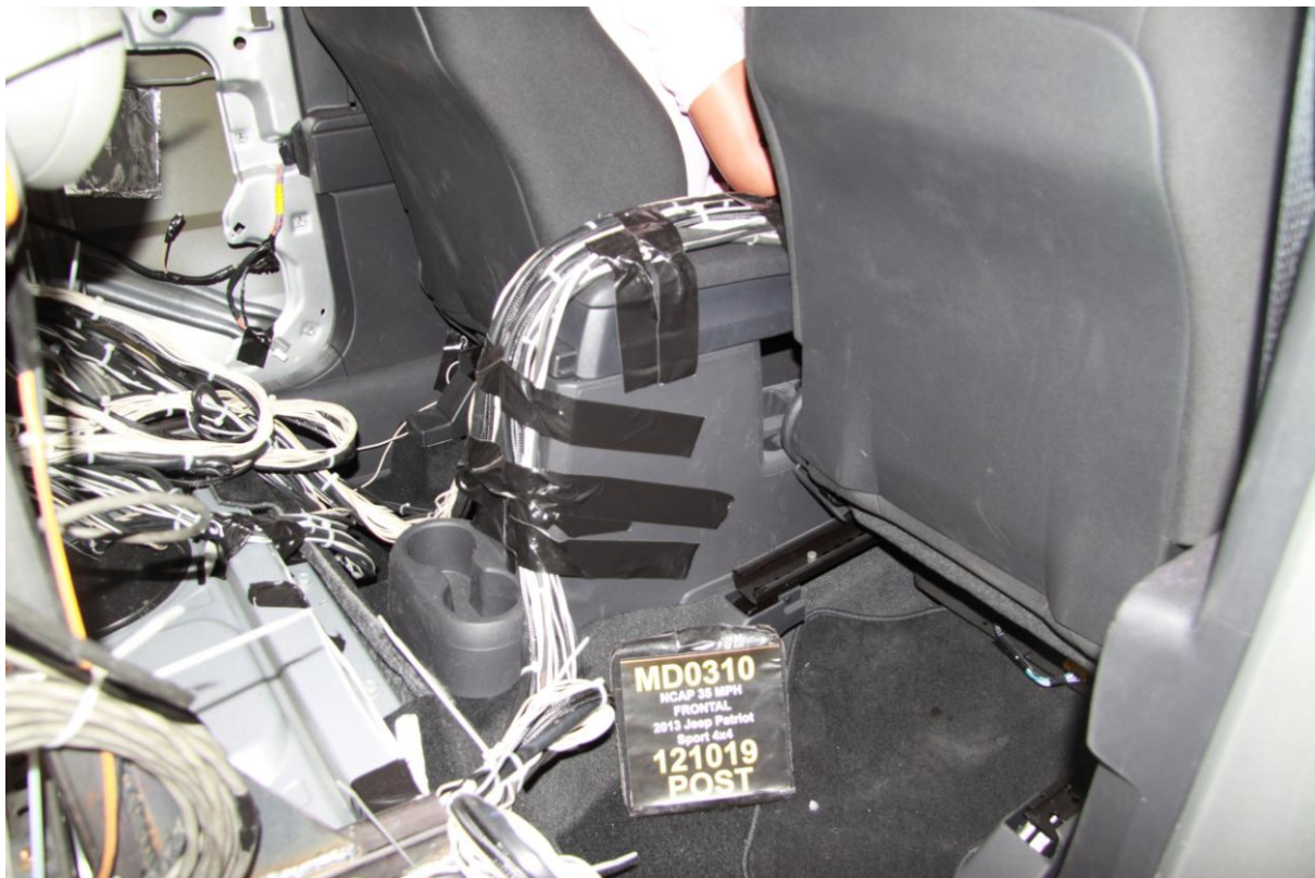
028 Post-test Dummy Cable Routing
