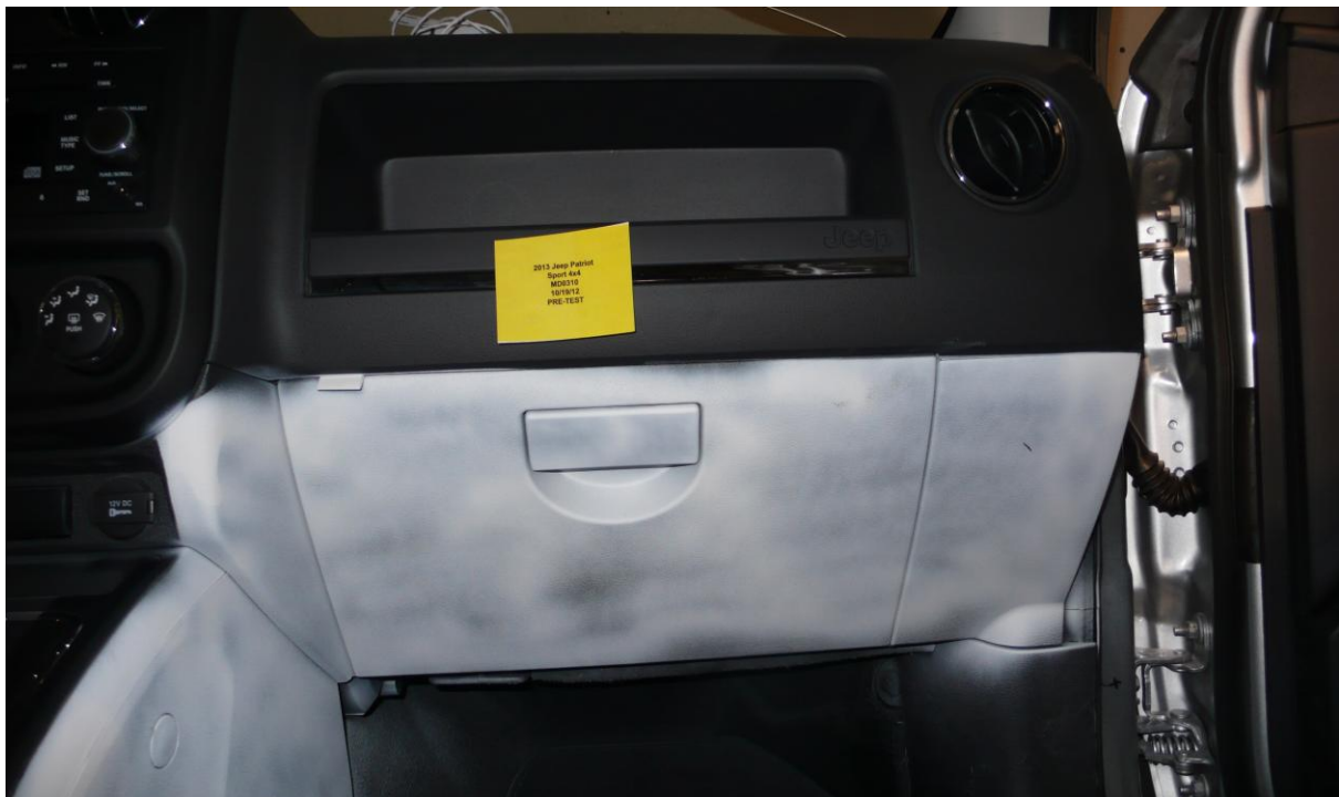
062 Pre-test Passenger's Side Knee Bolster
