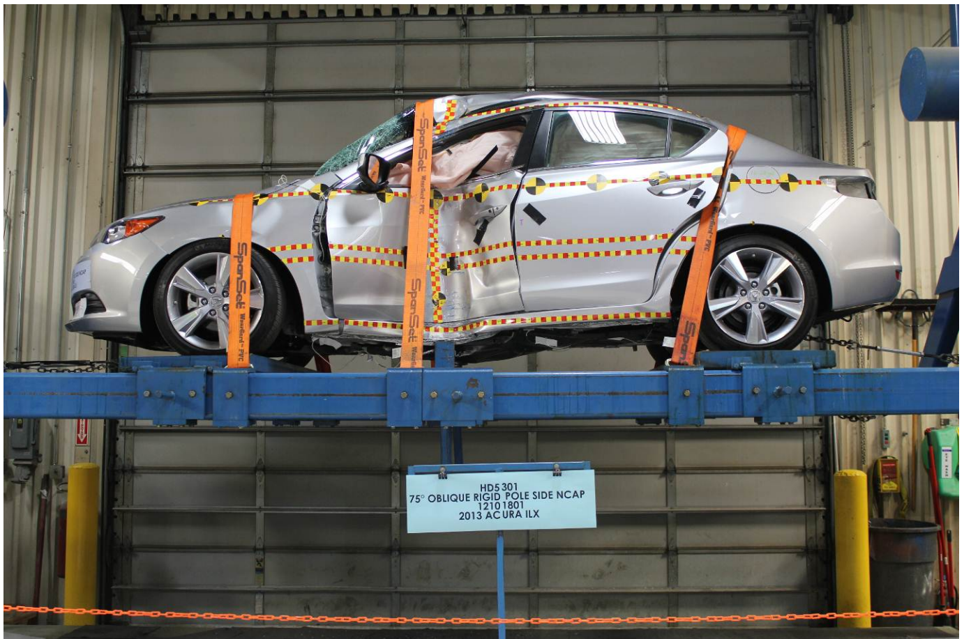
FMVSS No. 301 Static Rollover 360 Degrees
