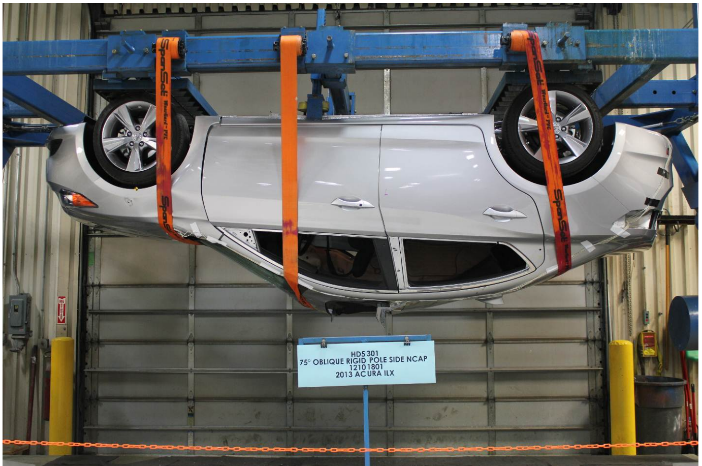
FMVSS No. 301 Static Rollover 180 Degrees
