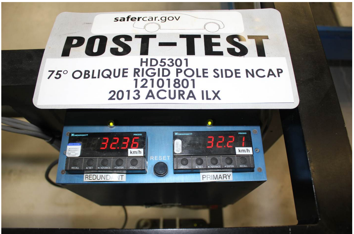
Post-Test Primary and Redundant Speed Trap Read-Out
