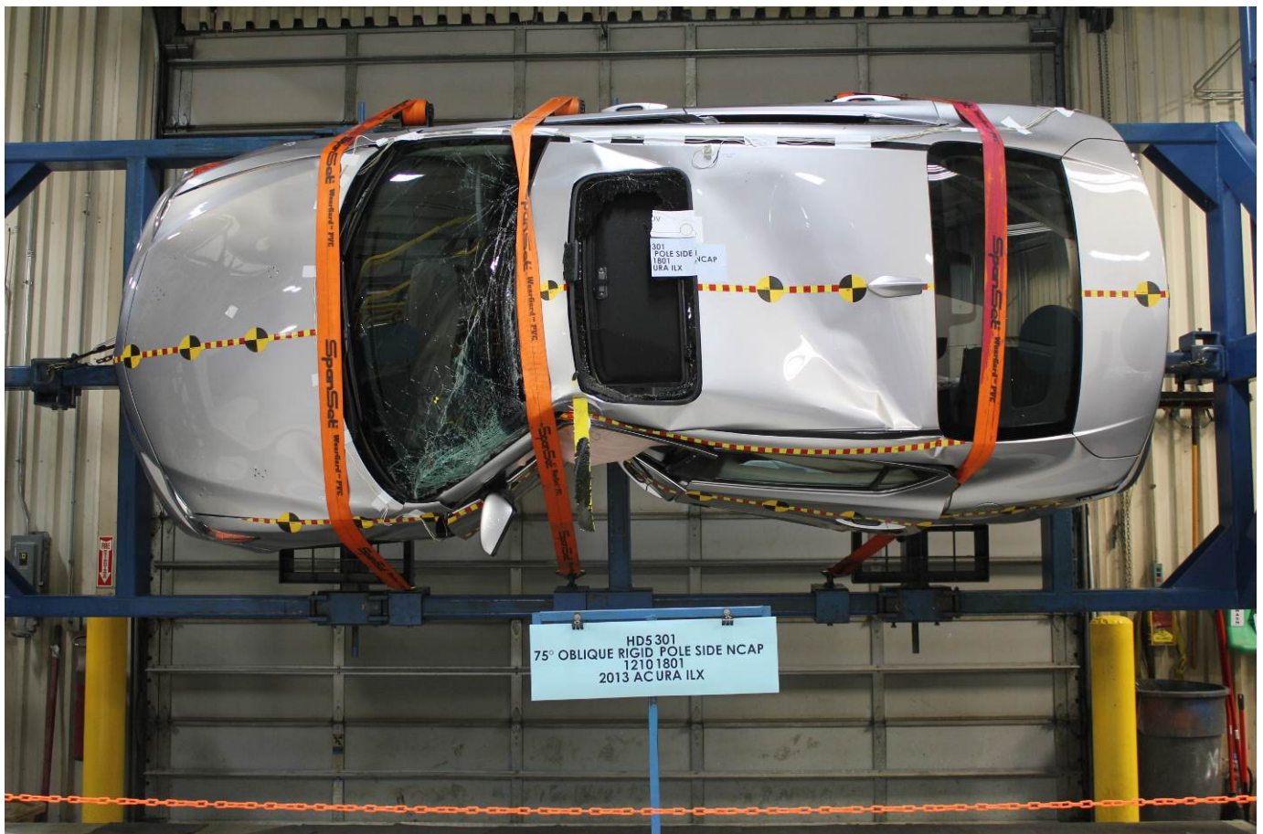
FMVSS No. 301 Static Rollover 90 Degrees
