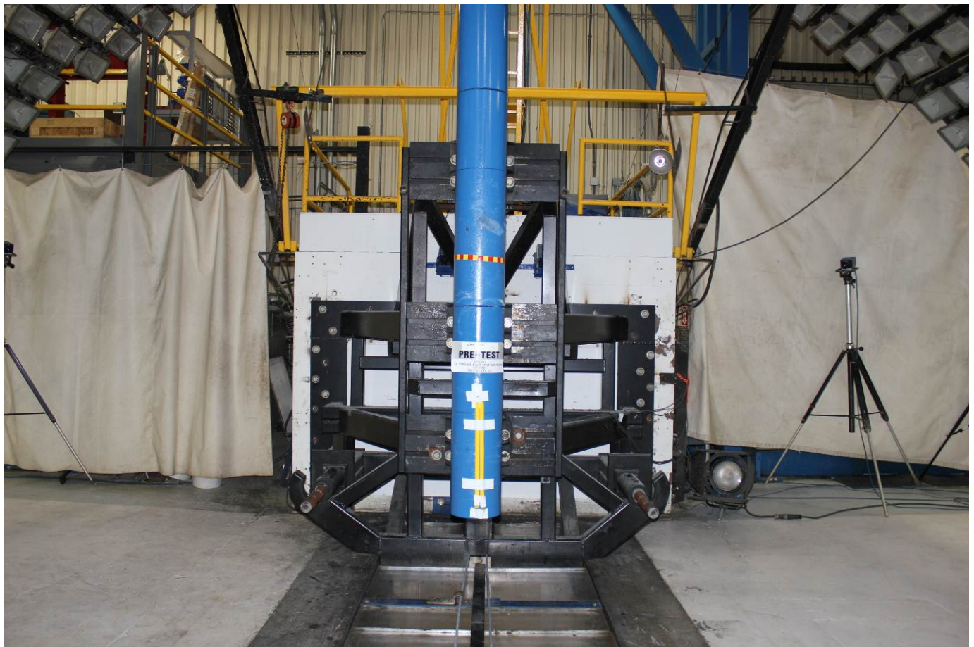
Pre-Test Pole Barrier Front View
