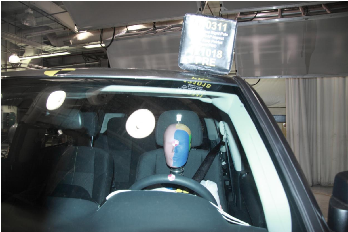
027 Pre-Test Front View of Dummy Head and Shoulders in Relation to Head Restraint
