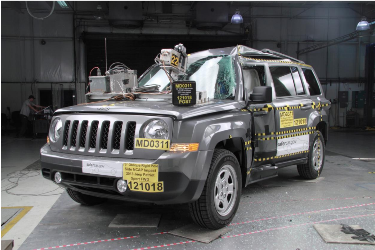
006 Post-Test Left Front 3/4 View of Test Vehicle
