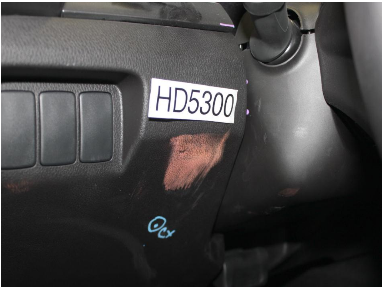
Post-Test Driver Dummy Contact with Knee Bolster
