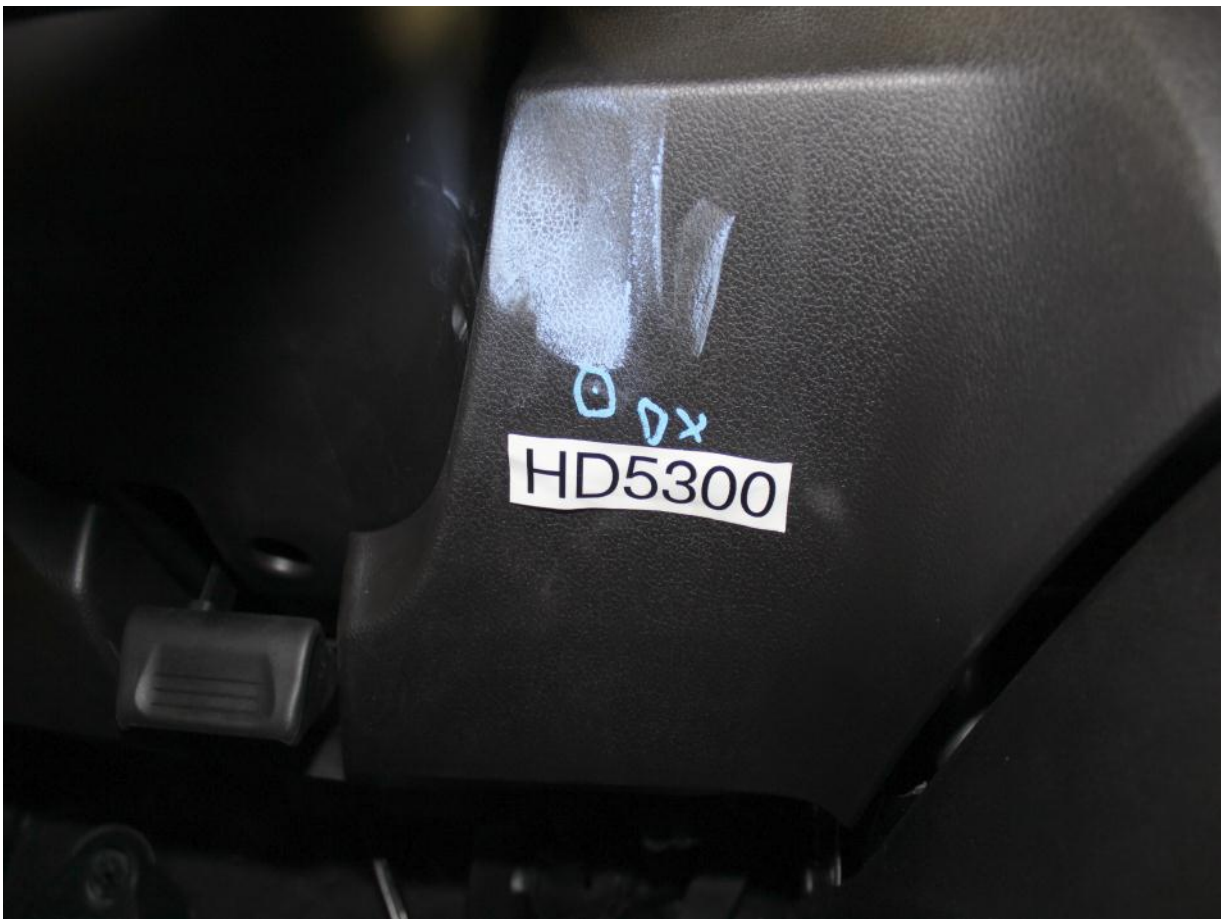
Post-Test Driver Dummy Contact with Knee Bolster
