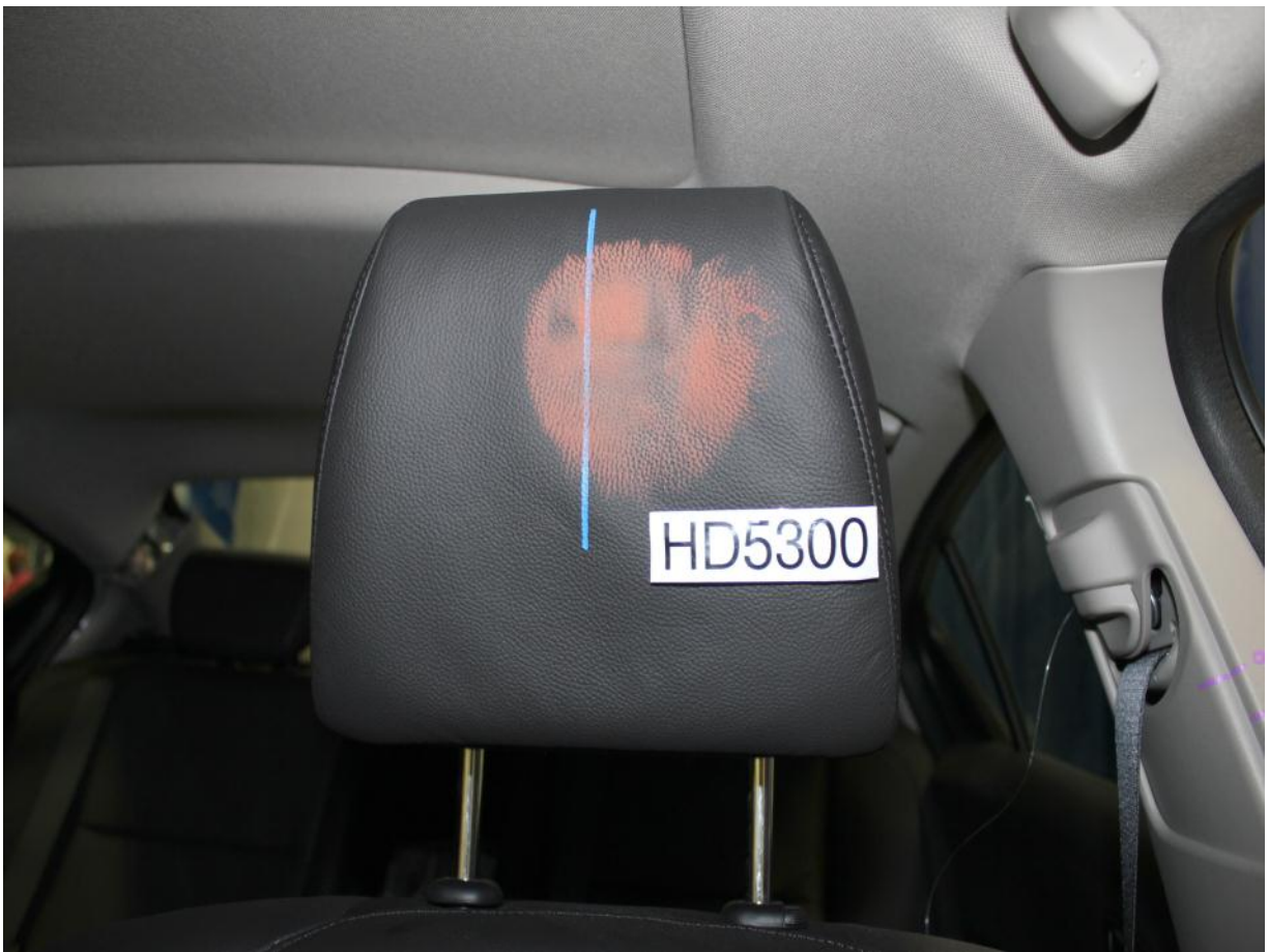
Post-Test Driver Dummy Contact with Headrest
