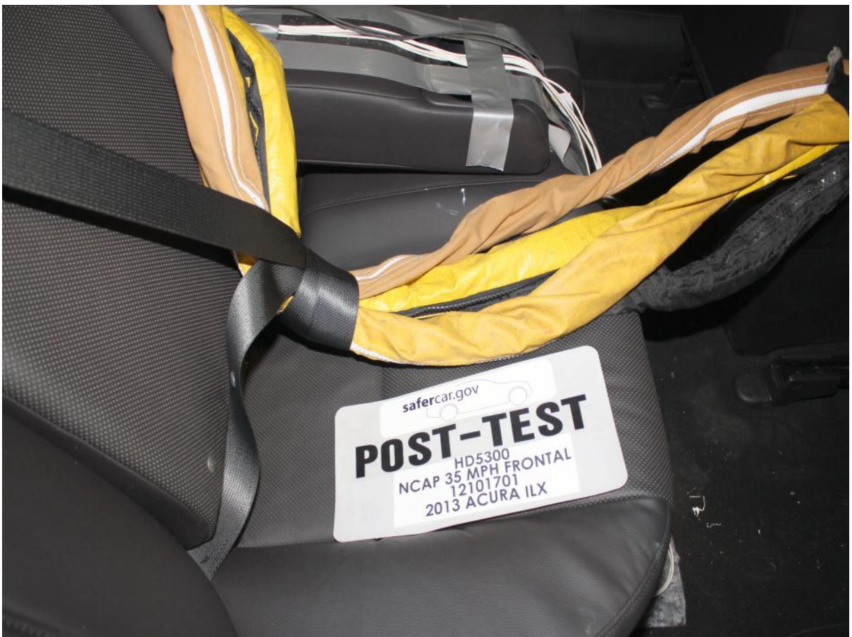
Post-Test Dummy Cable Routing
