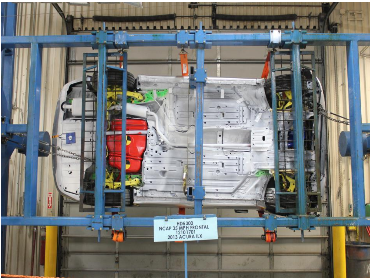
Vehicle at 90° on Static Rollover Device
