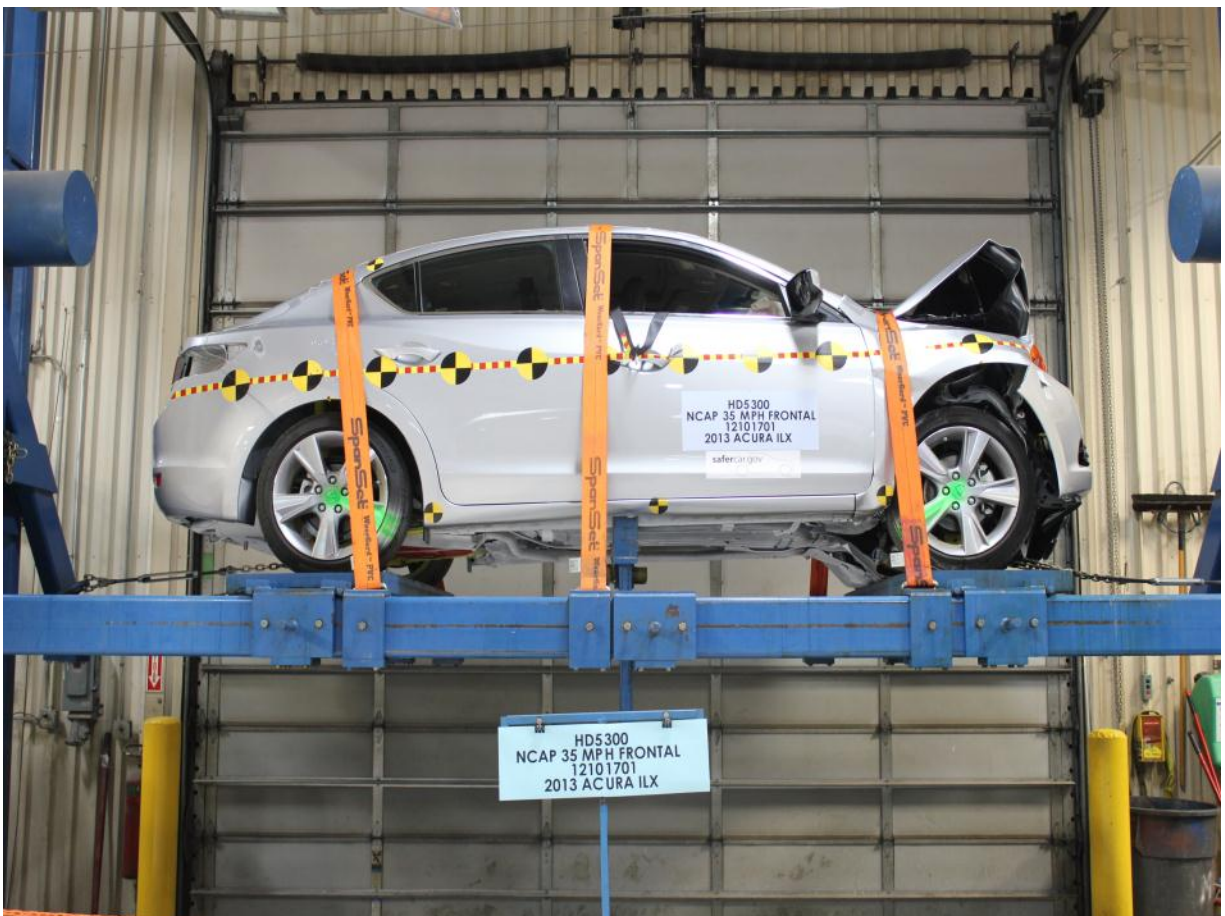
Vehicle at 360° on Static Rollover Device
