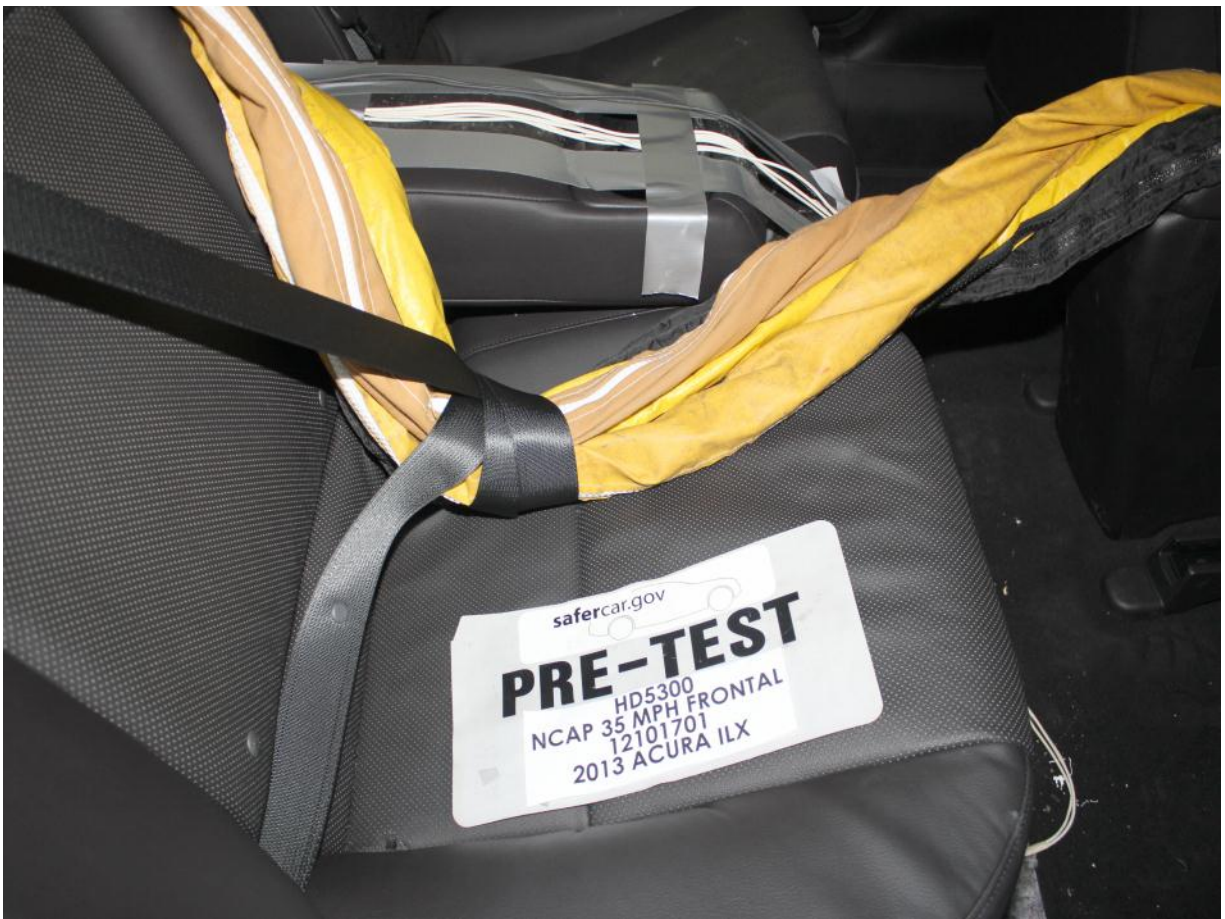
Pre-Test Dummy Cable Routing
