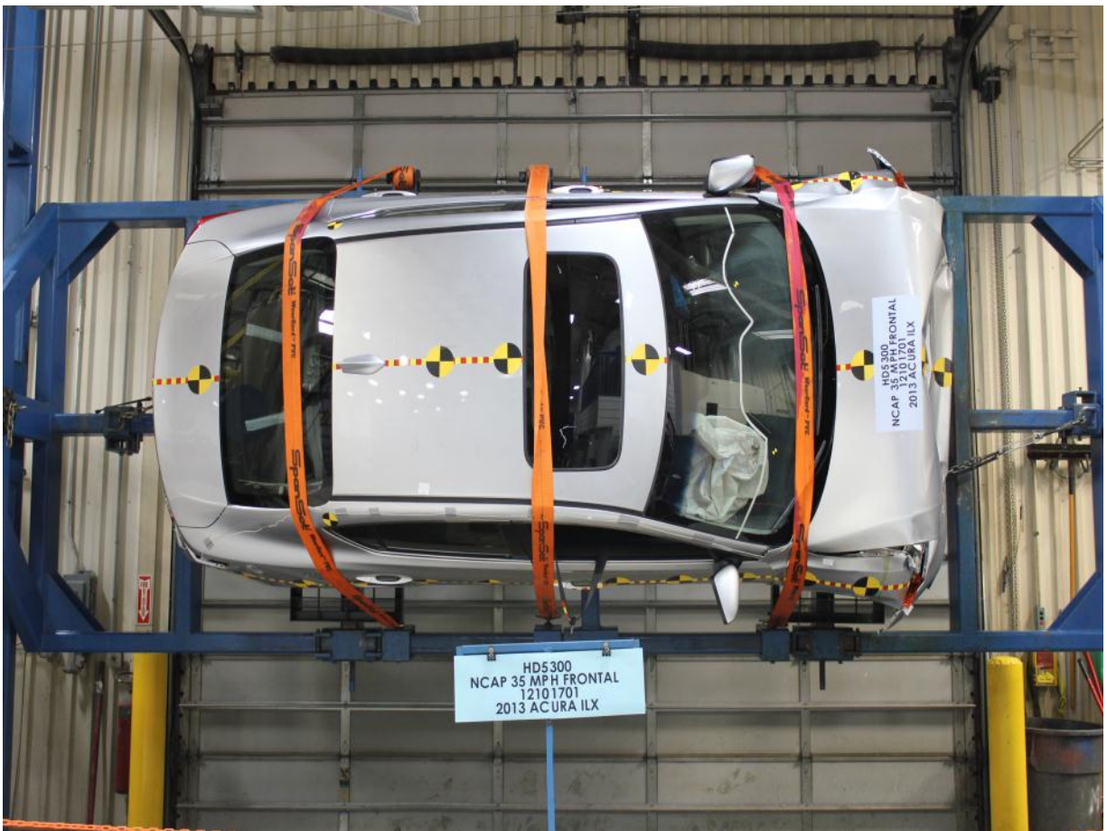
Vehicle at 270° on Static Rollover Device
