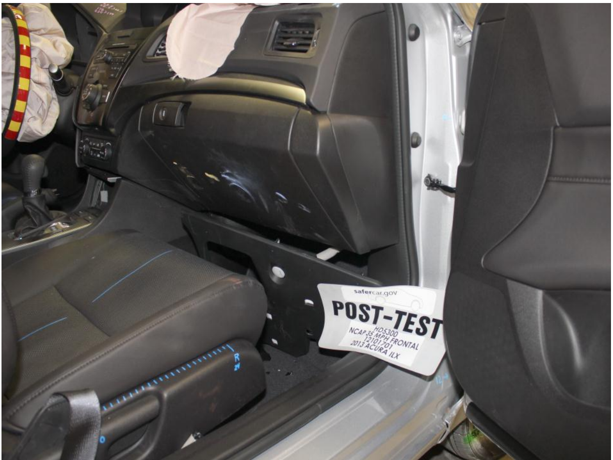
Post-Test Passenger's Side Knee Bolster (without dummy)
