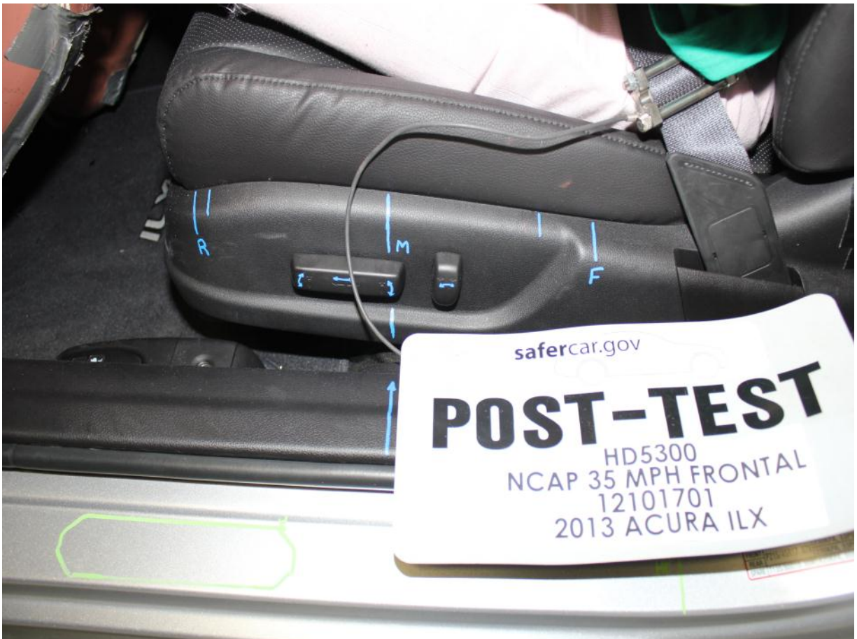
Post-Test Driver's Seat Fore-Aft Markings
