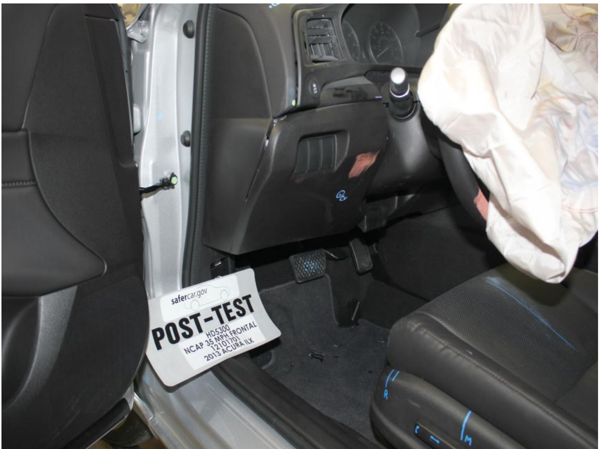
Post-Test Driver's Side Knee Bolster (without dummy)
