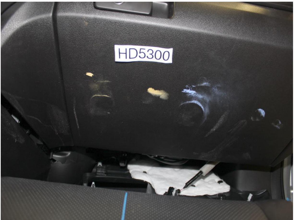
Post-Test Passenger Dummy Contact with Glove Box
