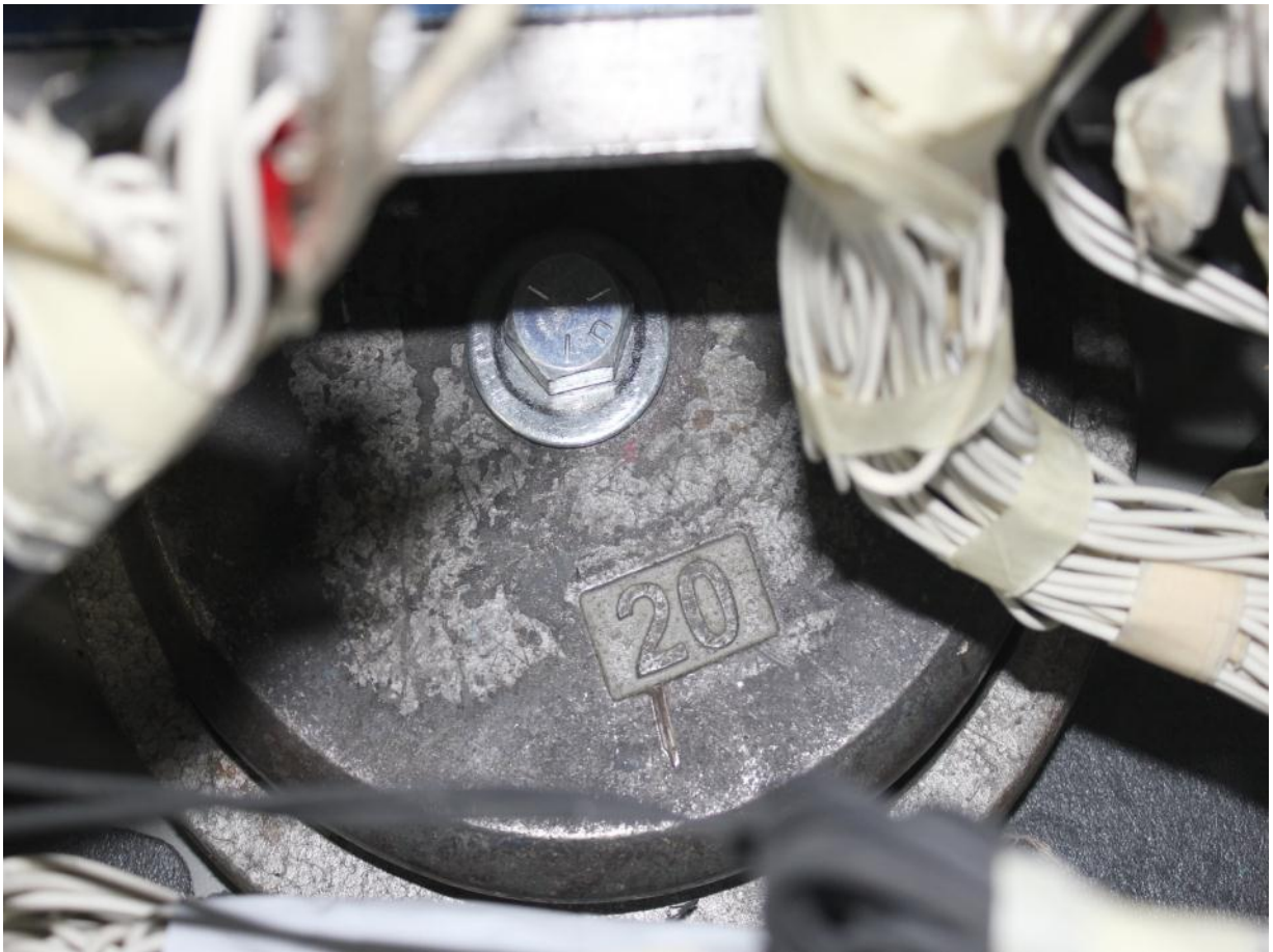
Ballast Installed in Vehicle
