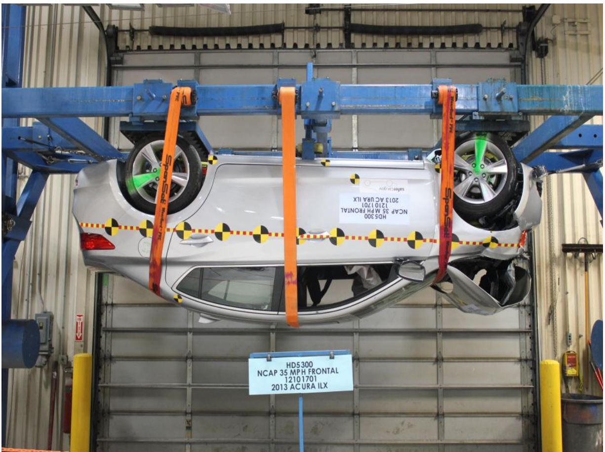
Vehicle at 180° on Static Rollover Device
