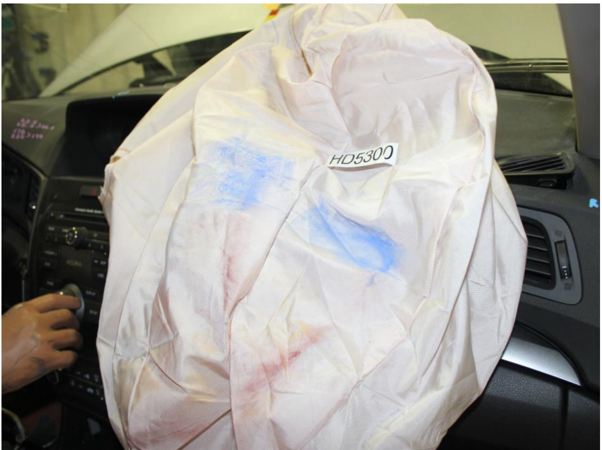
Post-Test Passenger Dummy Contact with Airbag
