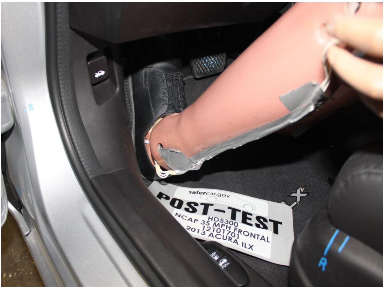
Post-Test Driver Dummy Feet
