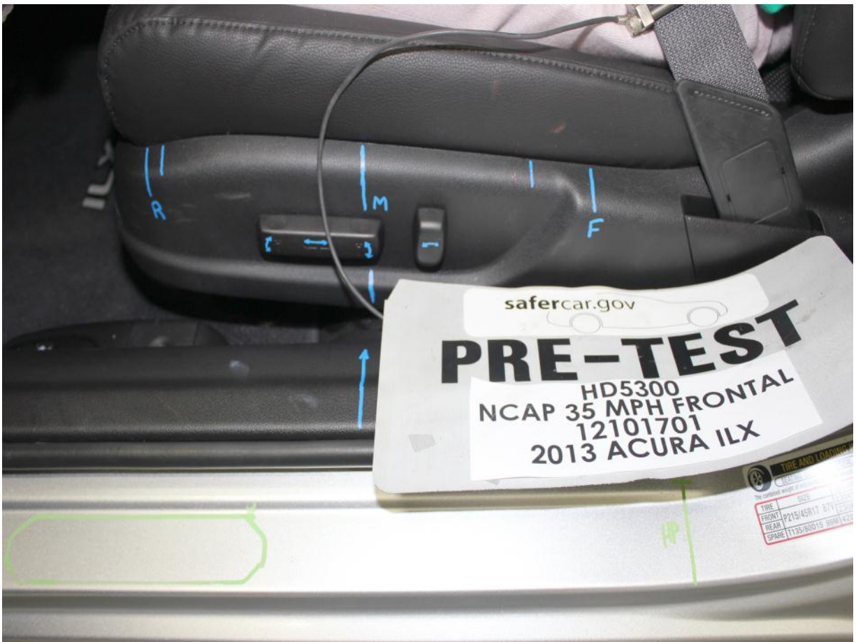
Pre-Test Driver's Seat Fore-Aft Markings
