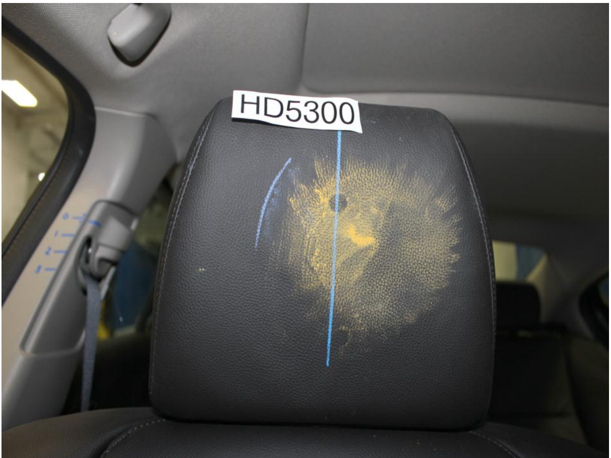
Post-Test Passenger Dummy Contact with Headrest
