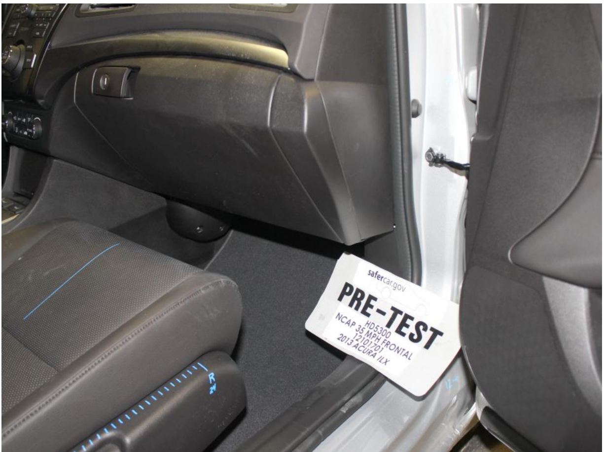
Pre-Test Passenger's Side Knee Bolster (without dummy)
