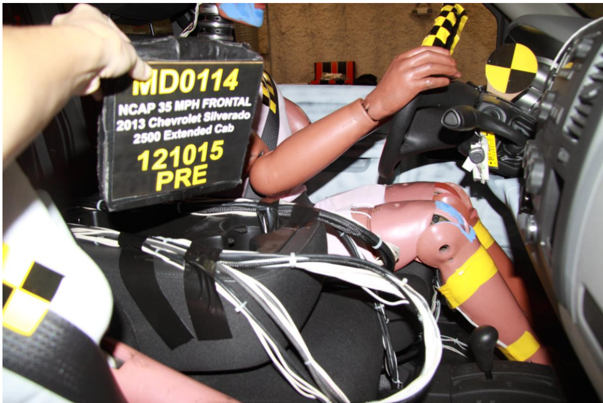
027 Pre-test Dummy Cable Routing
