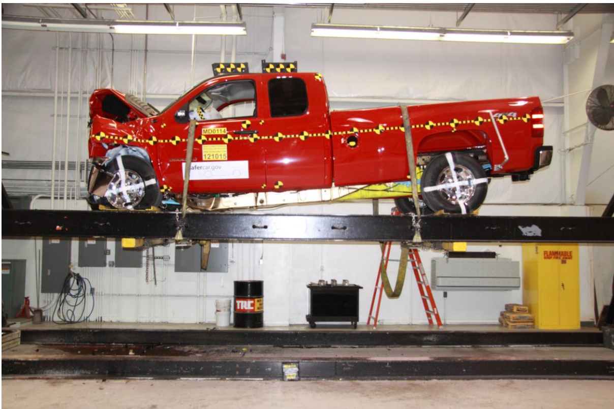
074 Vehicle at 360° on Static Rollover Device
