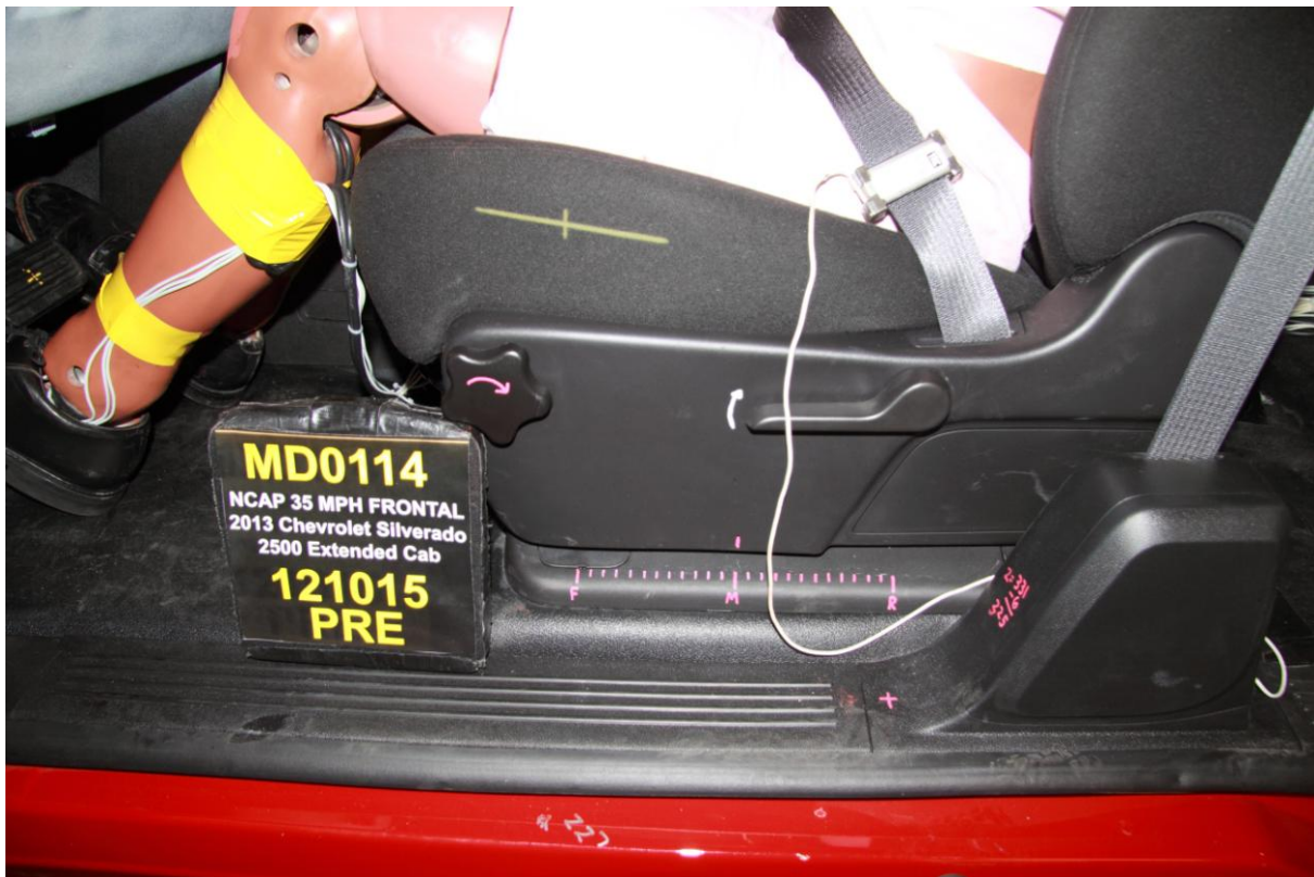
035 Pre-test Driver's Seat Fore-Aft Markings
