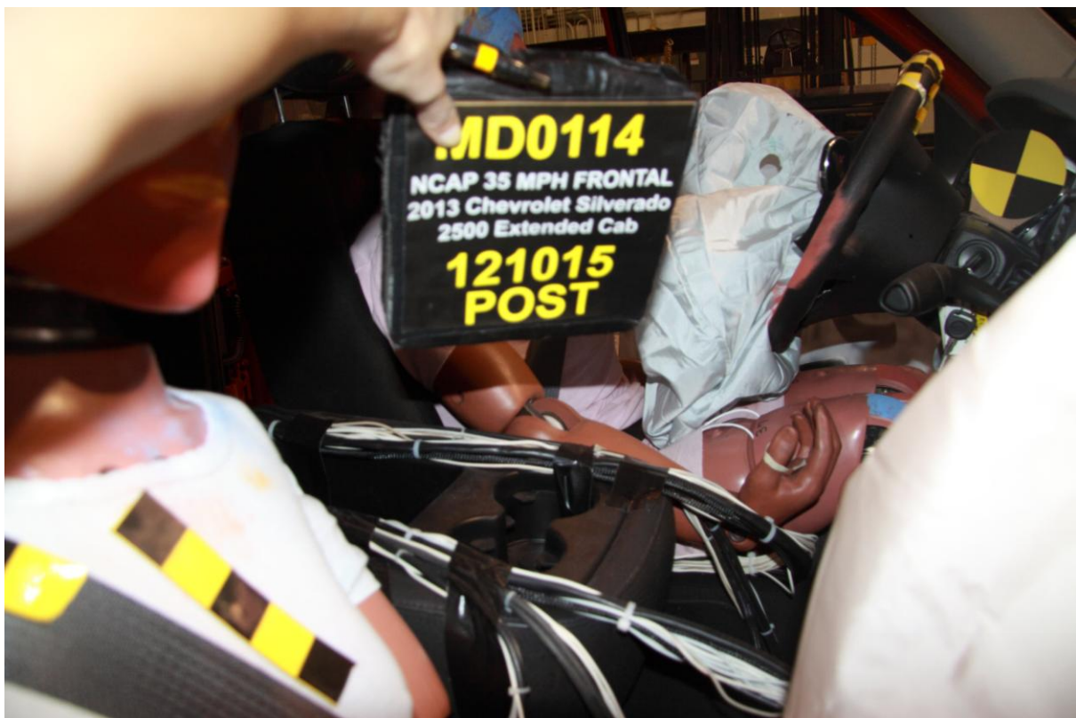
028 Post-test Dummy Cable Routing
