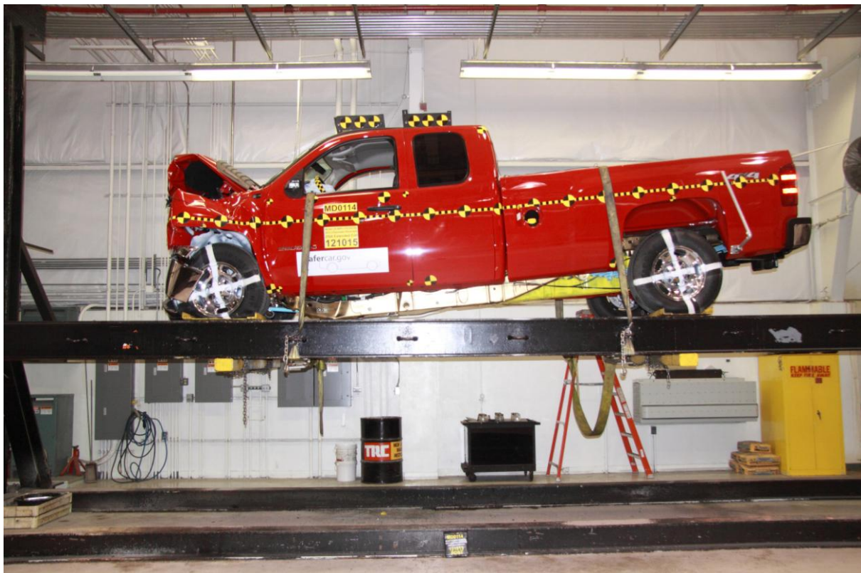
070 Vehicle at 0° on Static Rollover Device
