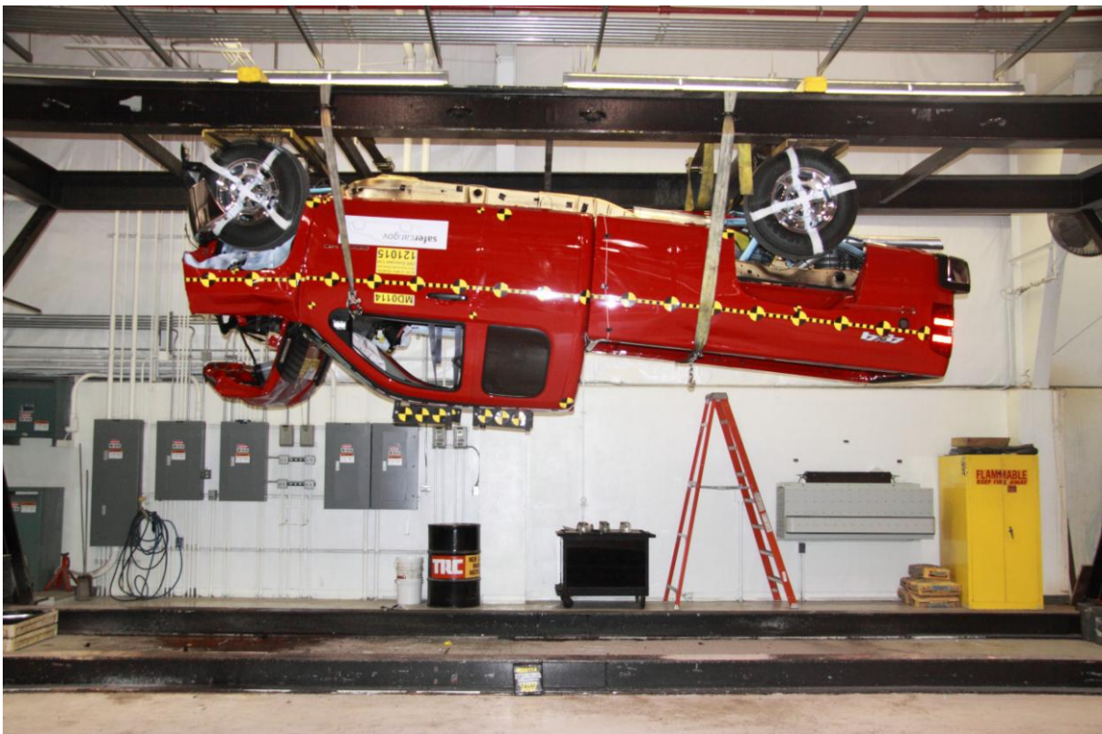
072 Vehicle at 180° on Static Rollover Device
