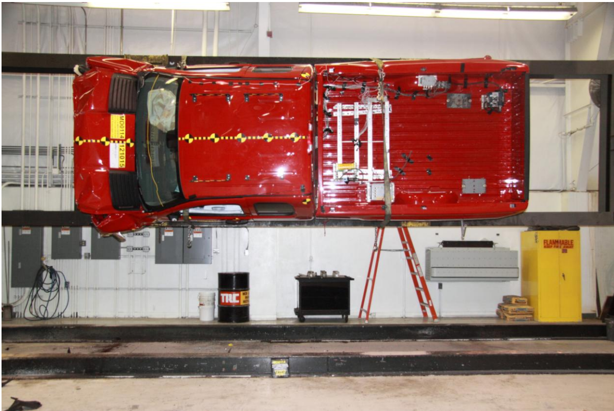
071 Vehicle at 90° on Static Rollover Device
