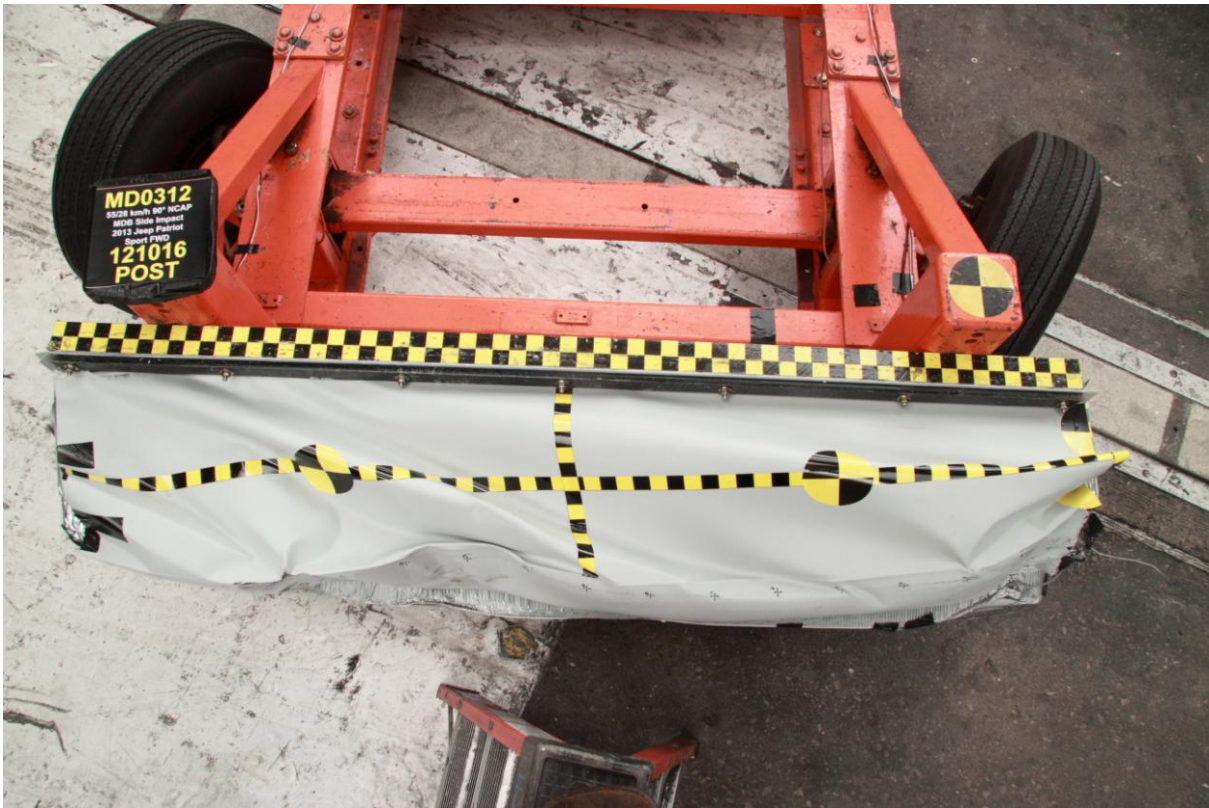
087 Post-Test Top View of MDB Impactor Face
