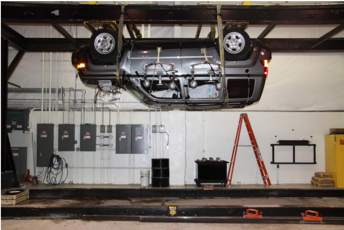
098 FMVSS No. 301 Static Rollover 180 Degrees
