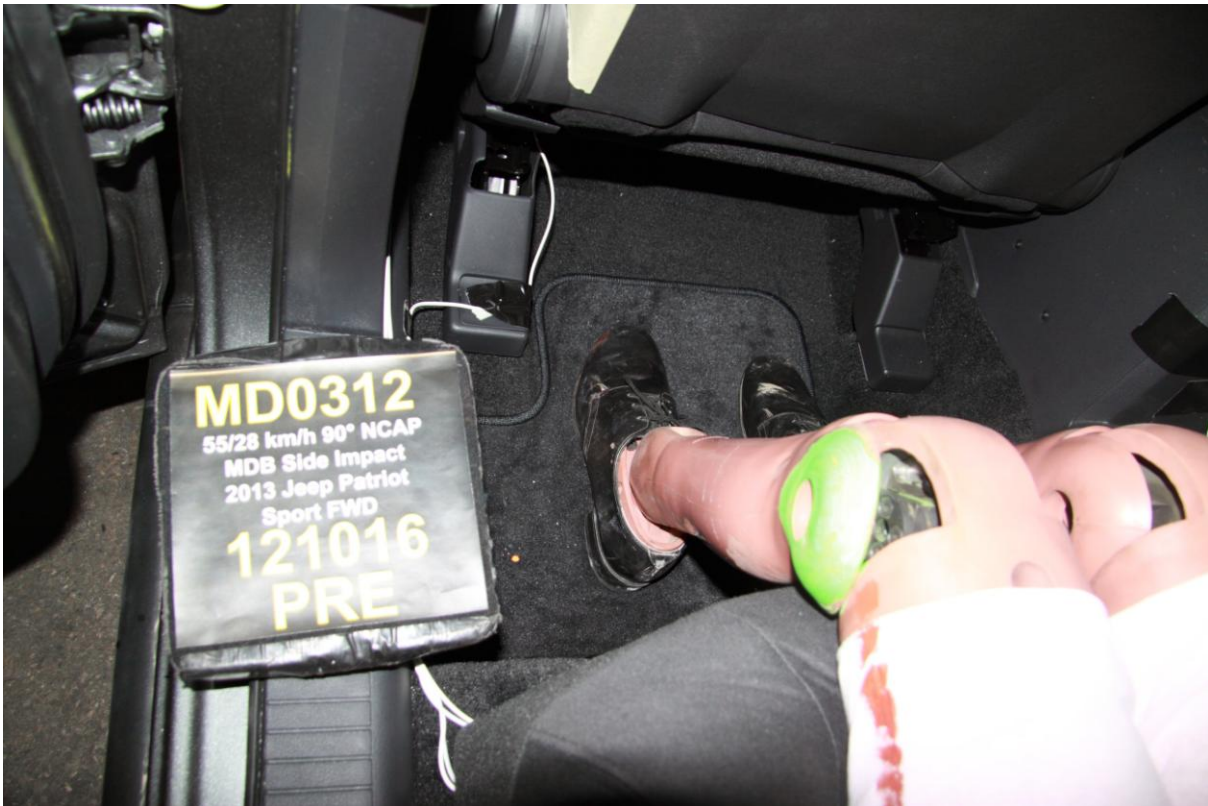
064 Pre-Test Placement of Rear Passenger Dummy Feet
