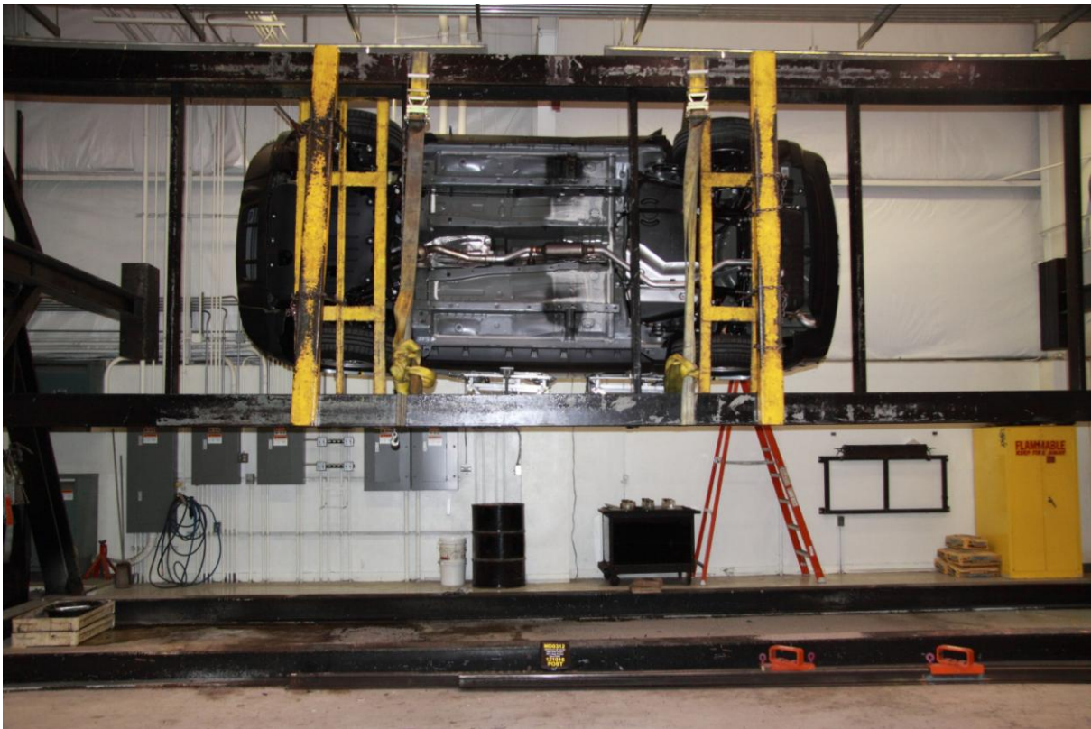
099 FMVSS No. 301 Static Rollover 270 Degrees
