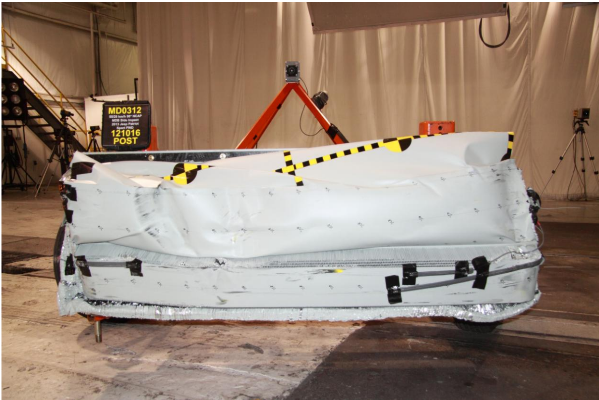
085 Post-Test Front View of MDB Impactor Face
