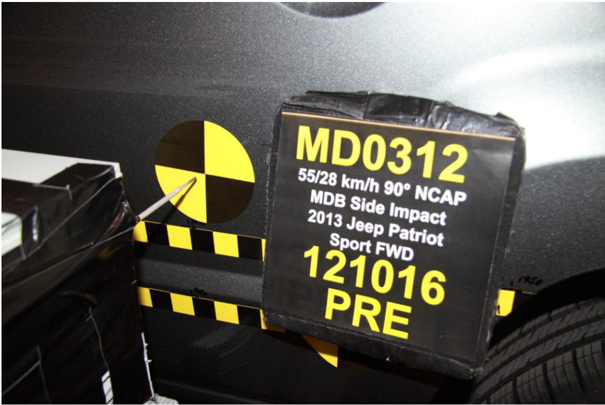
019 Pre-Test Close-up View of Impact Point Target
