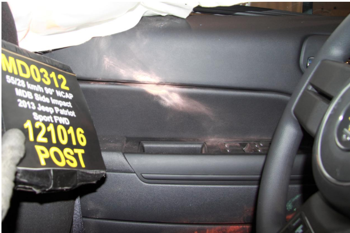
054 Post-Test Driver Dummy Close-Up Knee Contact View
