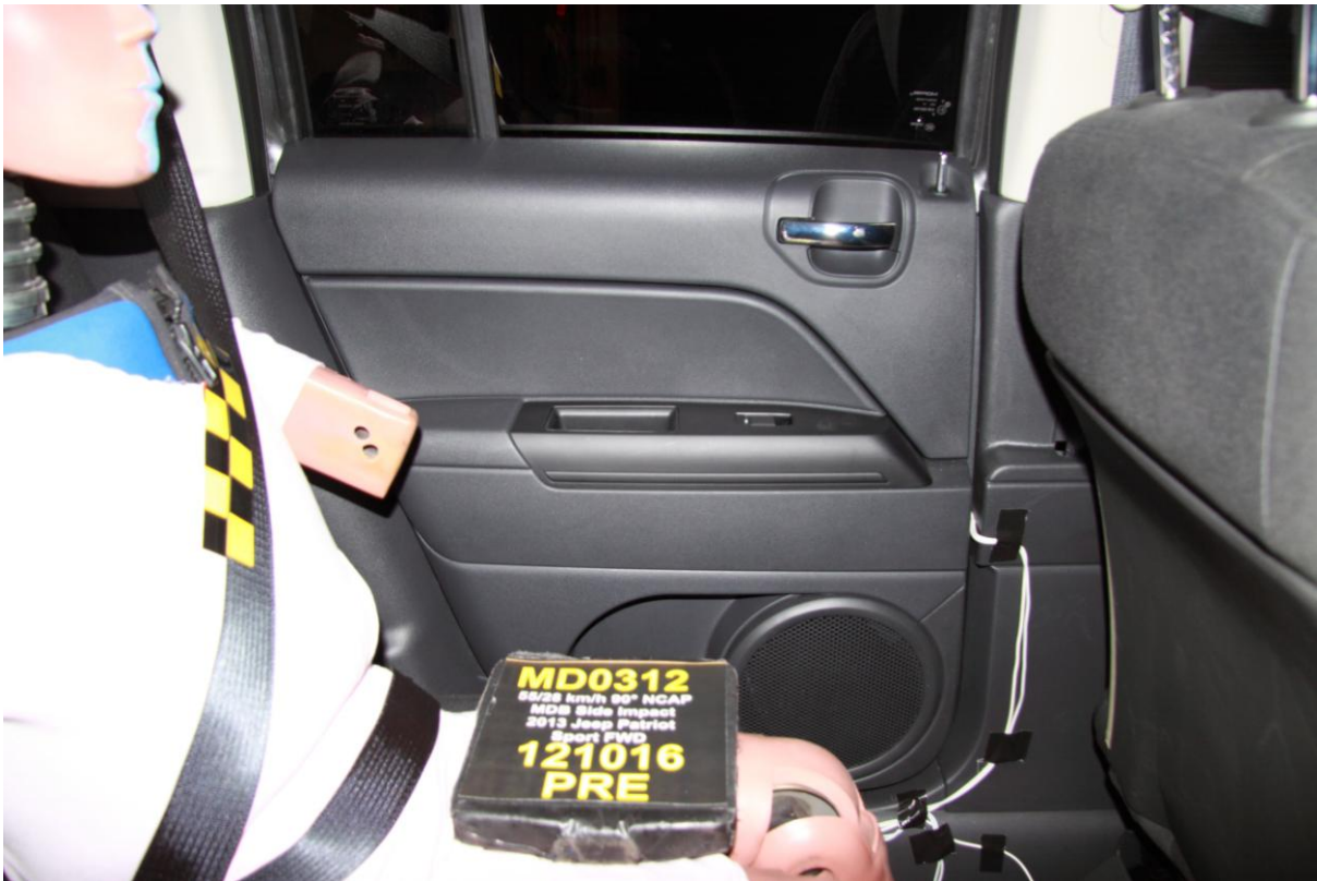
073 Pre-Test Passenger Inner Door Panel View
