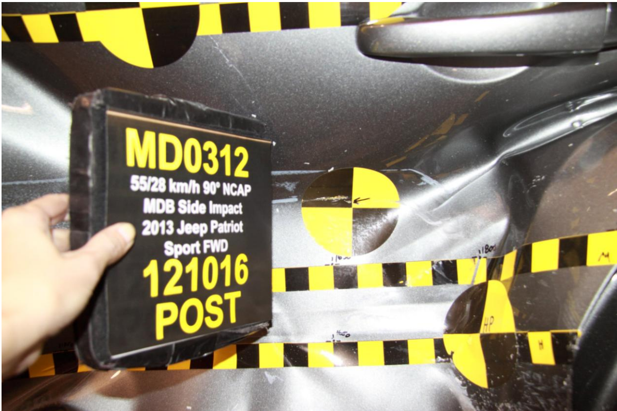
020 Post-Test Close-up View of Impact Point Target
