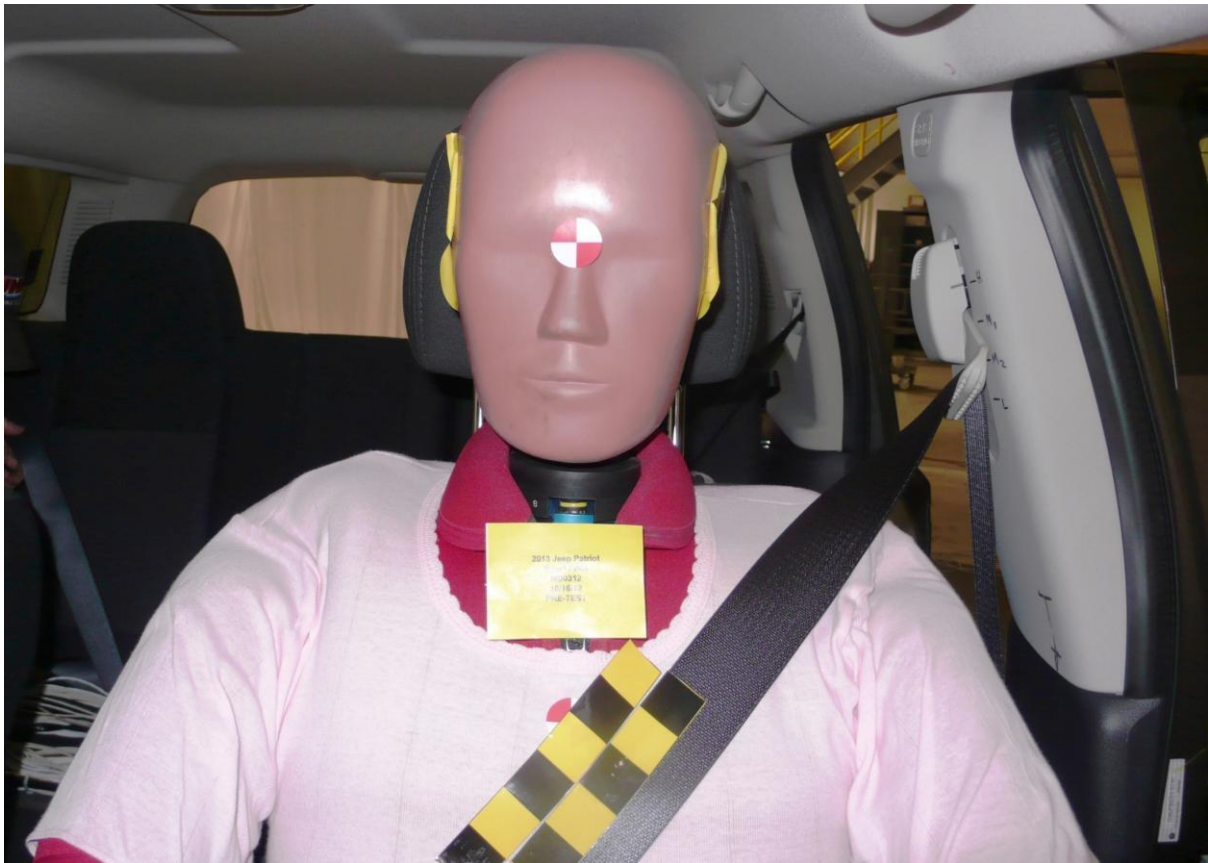
031 Pre-Test Frontal View of Driver Dummy Head and Shoulders in Relation to Head Restraint
