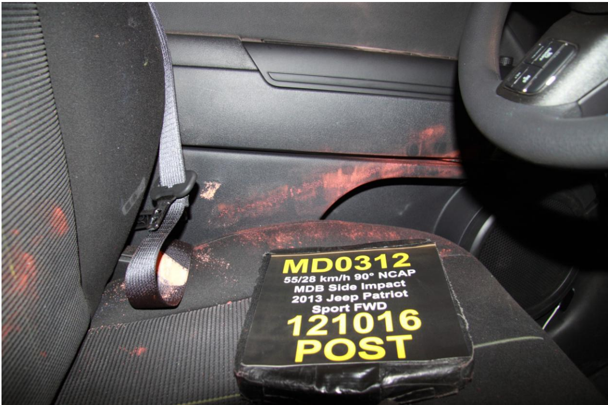
052 Post-Test Driver Dummy Close-Up Pelvis Contact View
