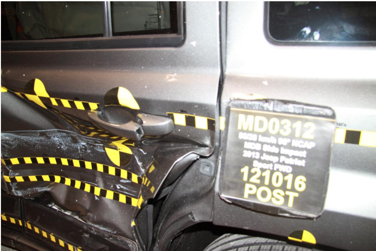
024 Post-Test Left Rear Door Latch Close-up
