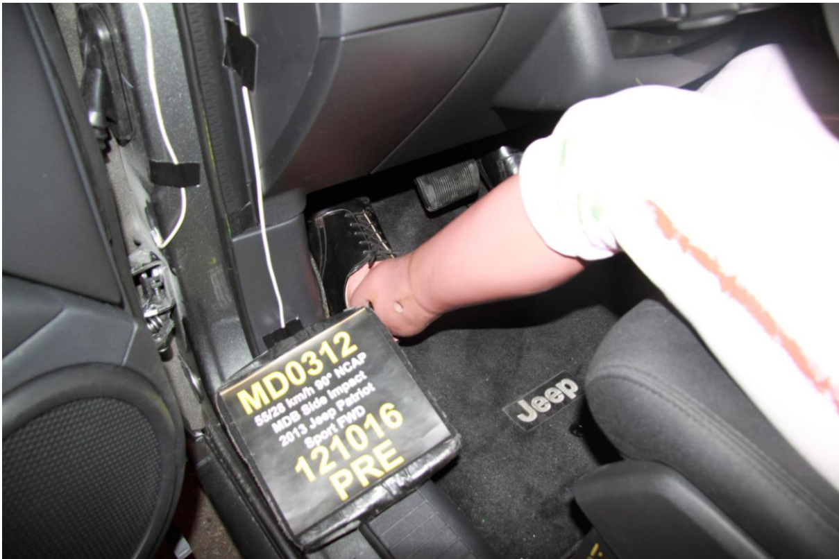
034 Pre-Test Placement of Driver Dummy Feet
