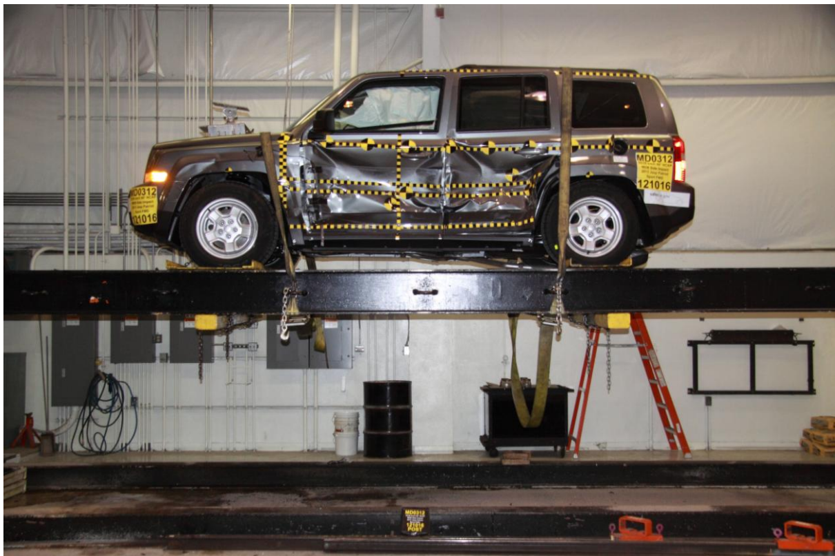
096 FMVSS No. 301 Static Rollover 0 Degrees
