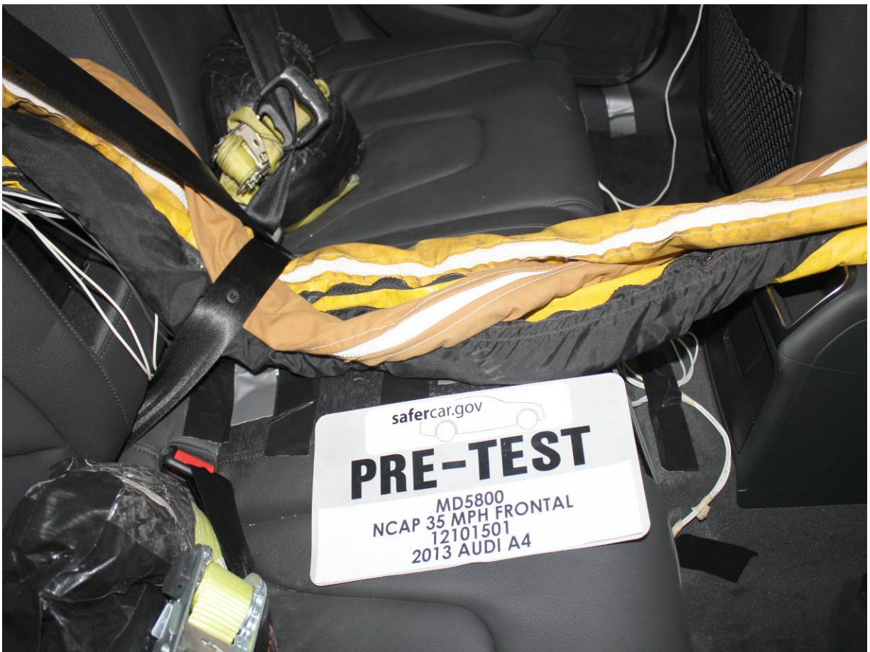
Pre-Test Dummy Cable Routing
