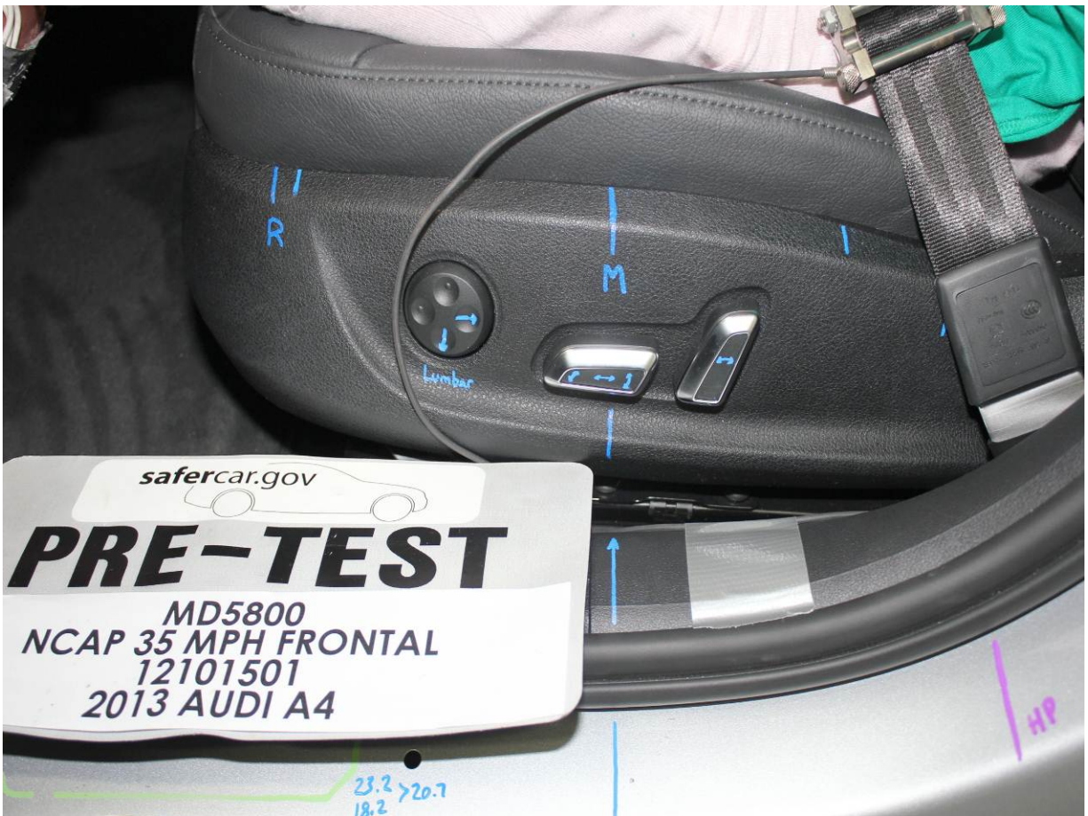
Pre-Test Driver's Seat Fore-Aft Markings
