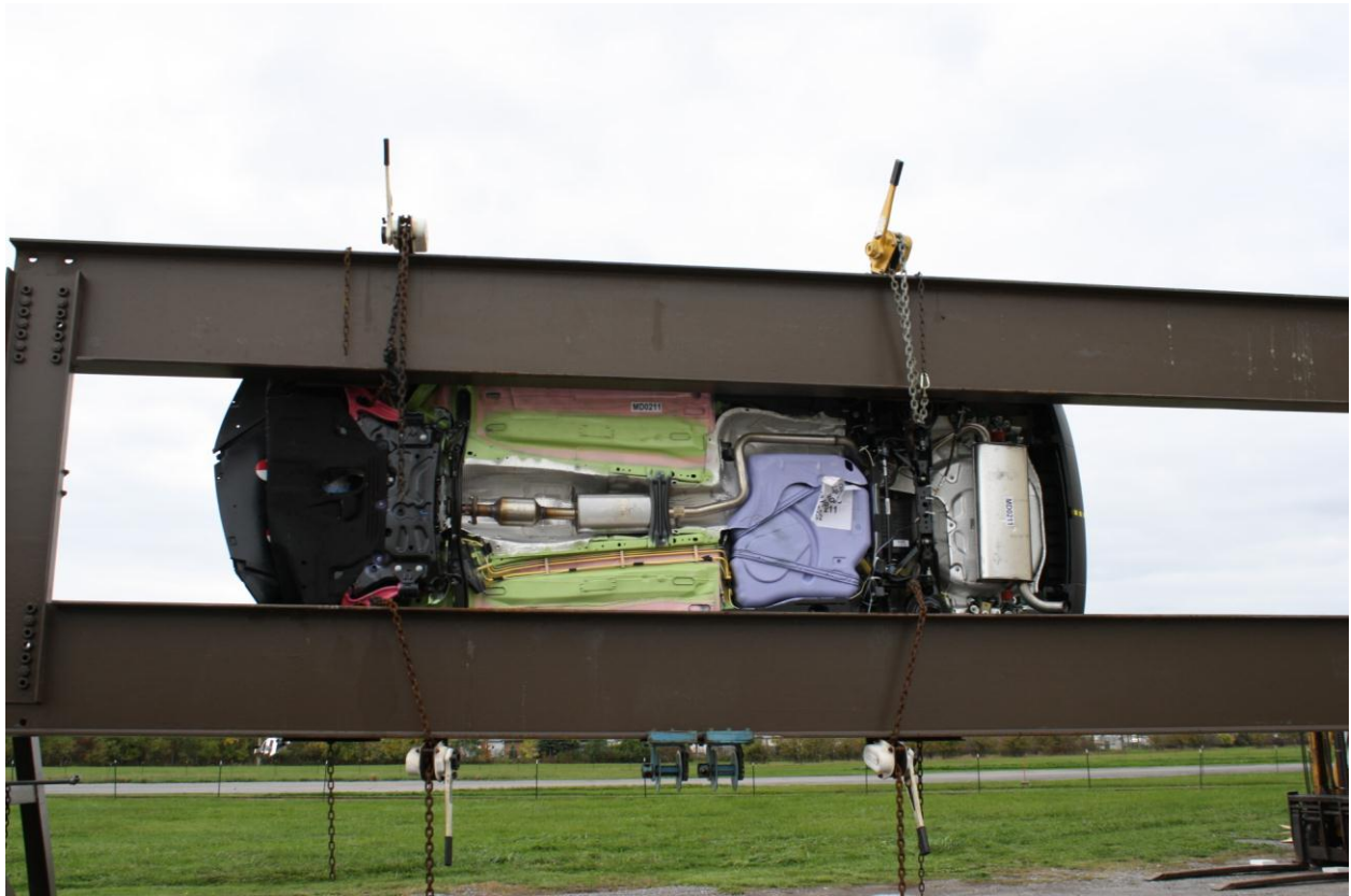
Figure A-71: Vehicle at 90° on Static Rollover Device
