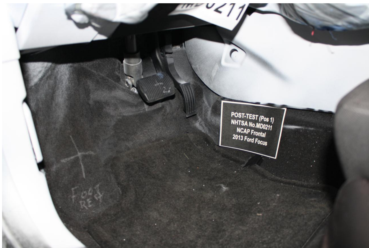
Figure A-44: Post-Test Driver's Side Floorpan
