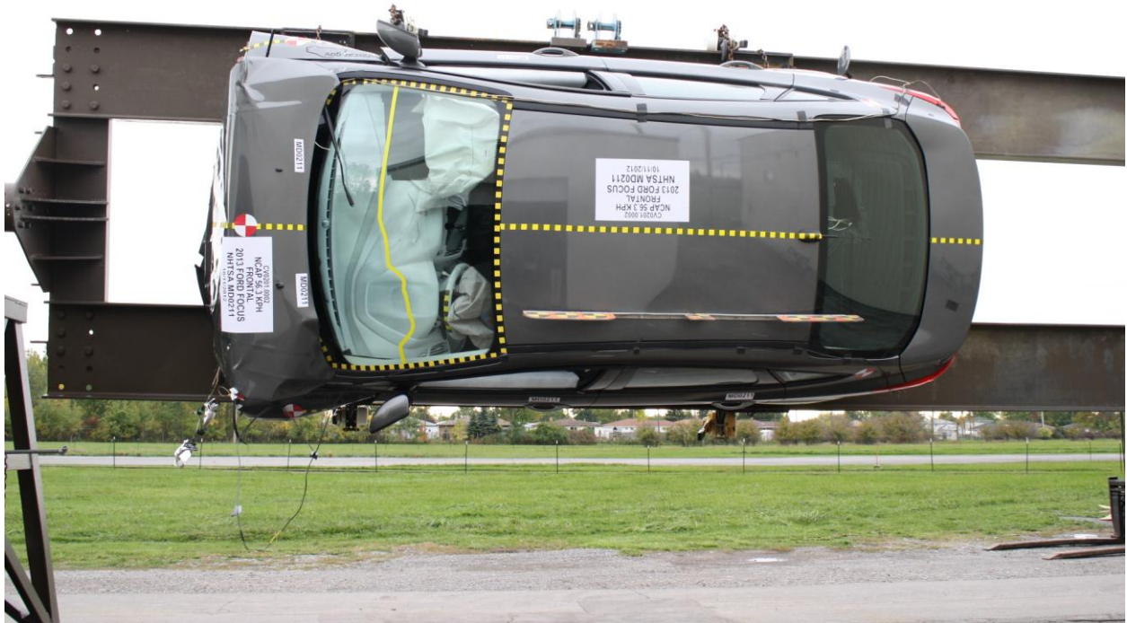
Figure A-73: Vehicle at 270° on Static Rollover Device
