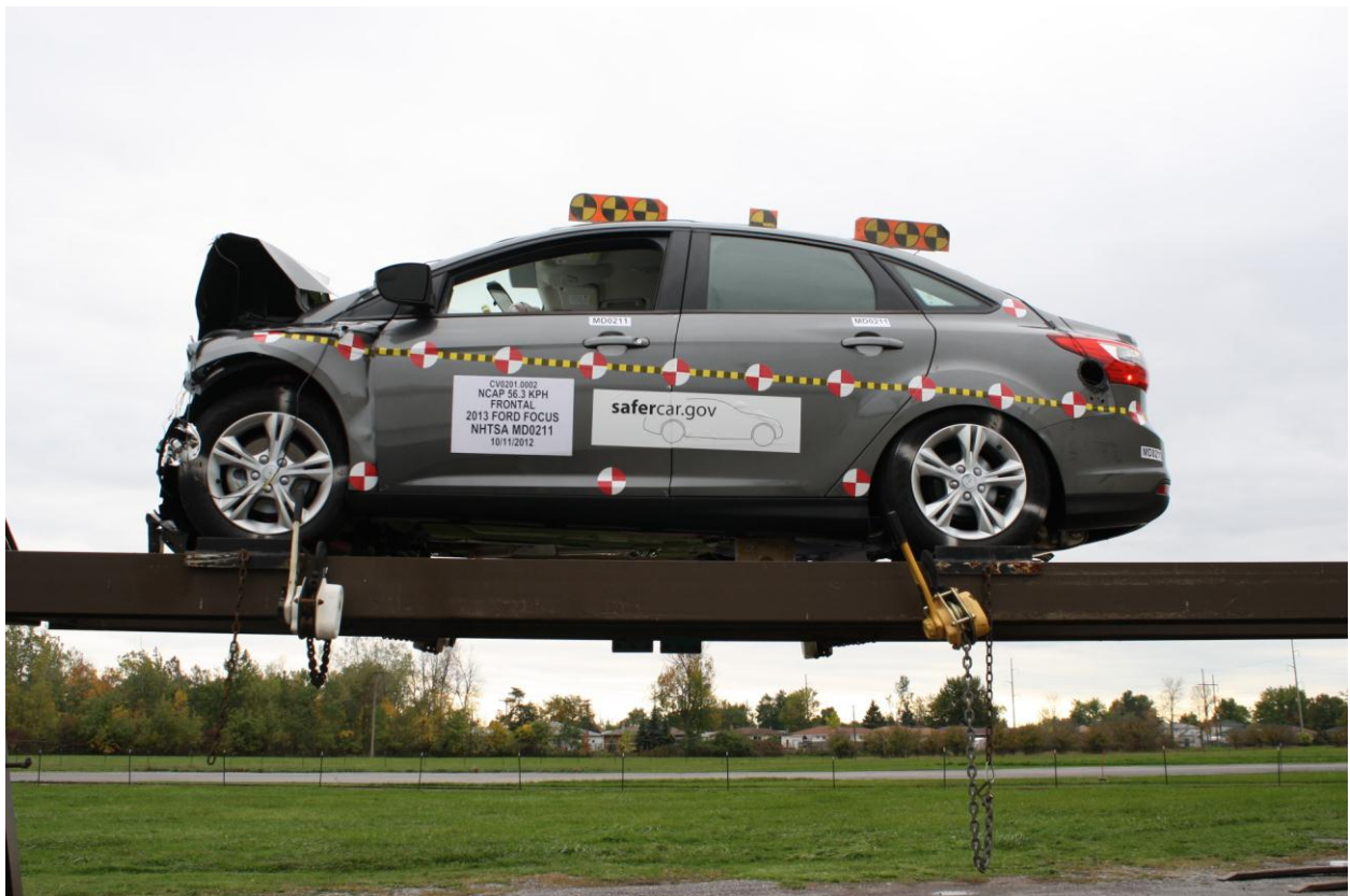
Figure A-74: Vehicle at 360° on Static Rollover Device
