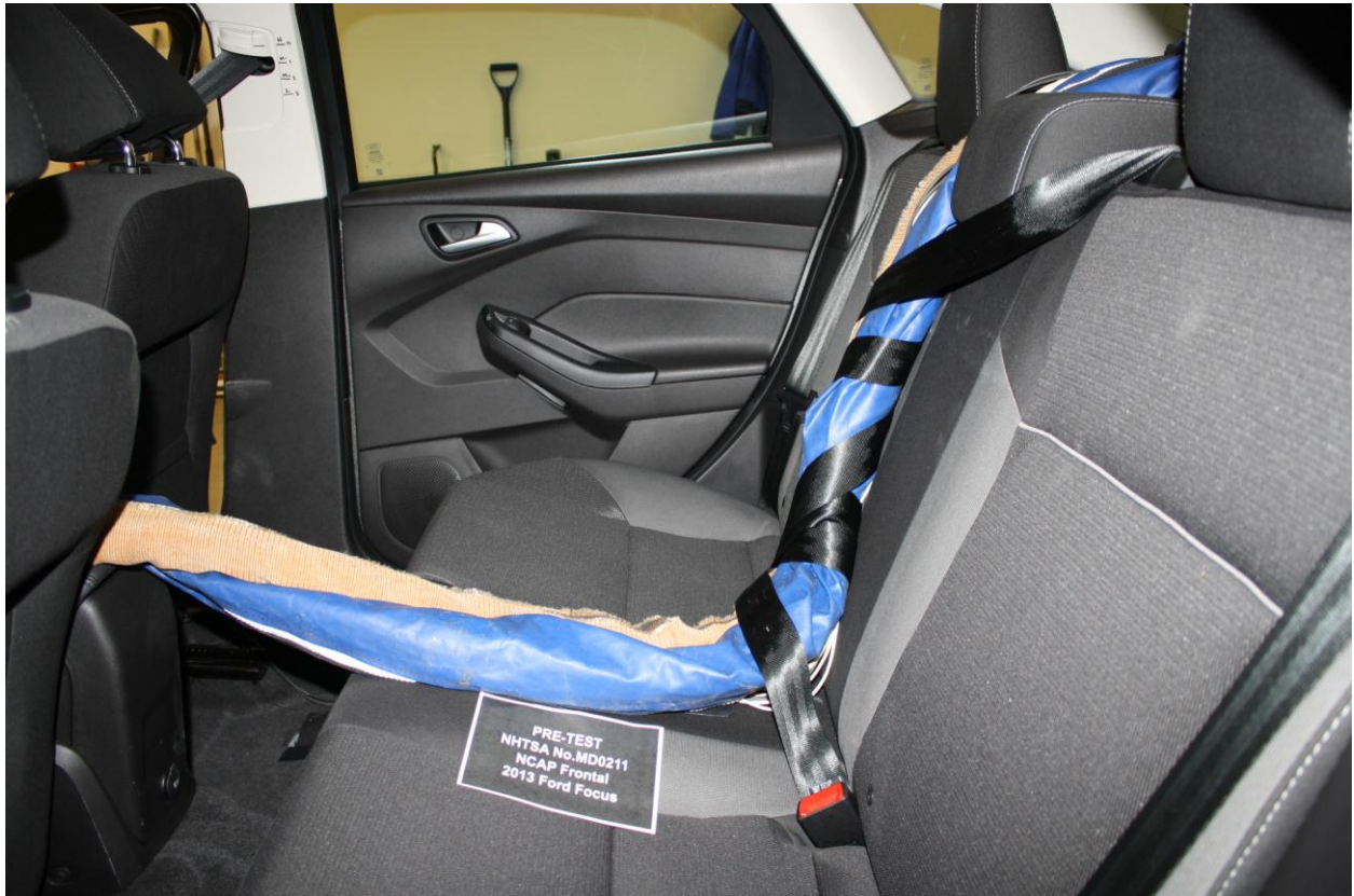
Figure A-27: Pre-Test Dummy Cable Routing
