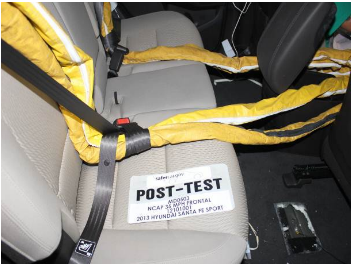
Post-Test Dummy Cable Routing
