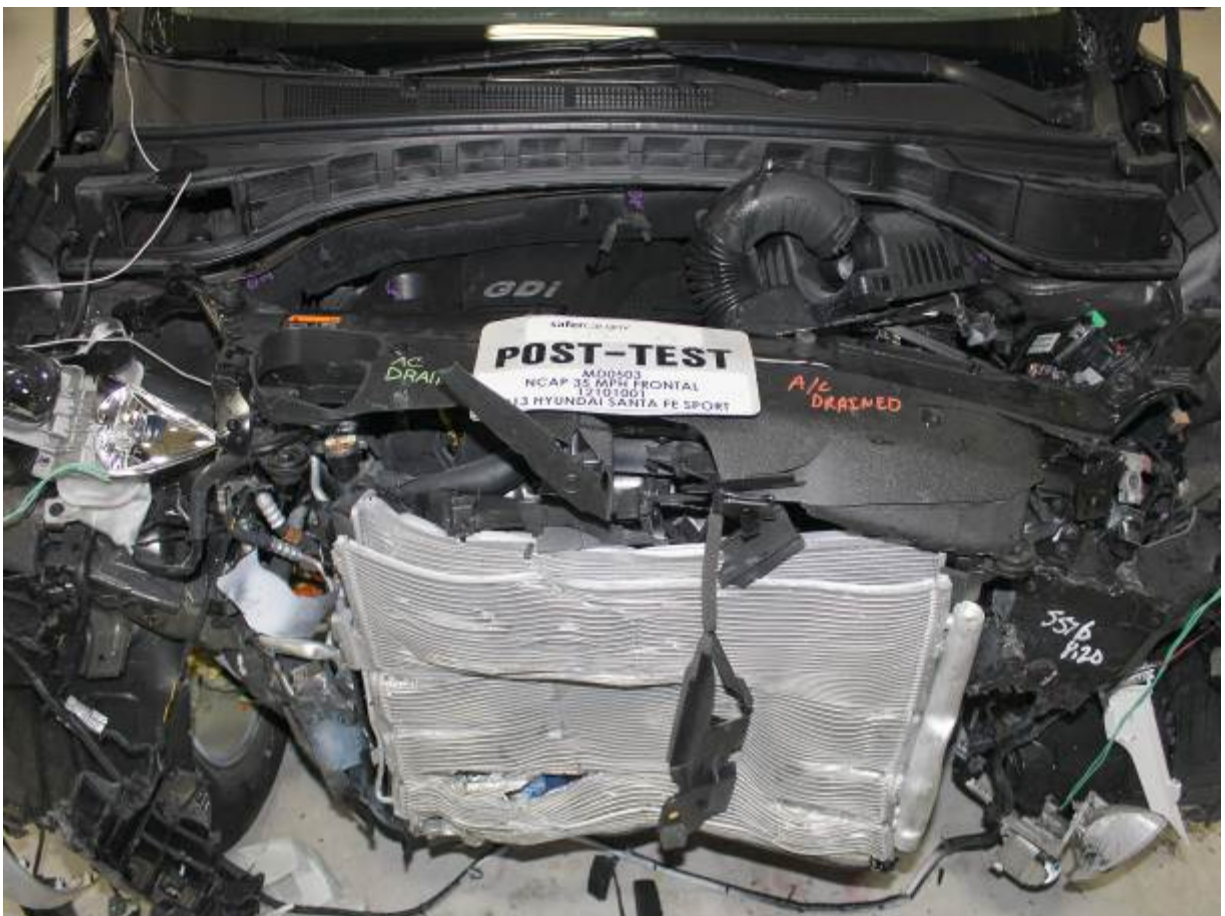
Post-Test Engine Compartment View
