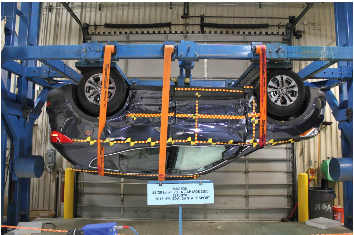
FMVSS No. 301 Static Rollover 180 Degrees
