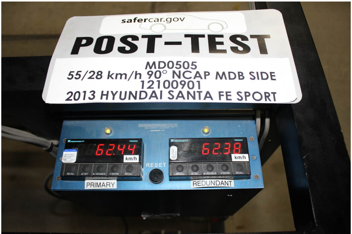
Post-Test Primary and Redundant Speed Trap Read-Out
