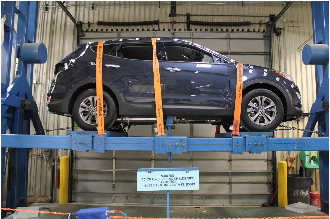
FMVSS No. 301 Static Rollover 0 Degrees
