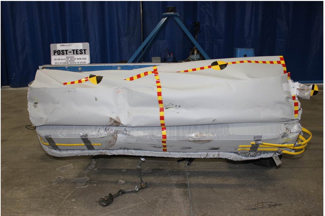
Post-Test Front View of MDB Impactor Face
