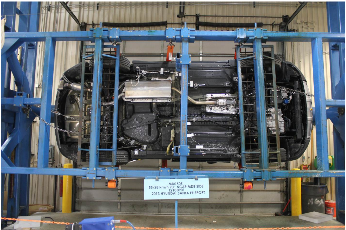
FMVSS No. 301 Static Rollover 90 Degrees
