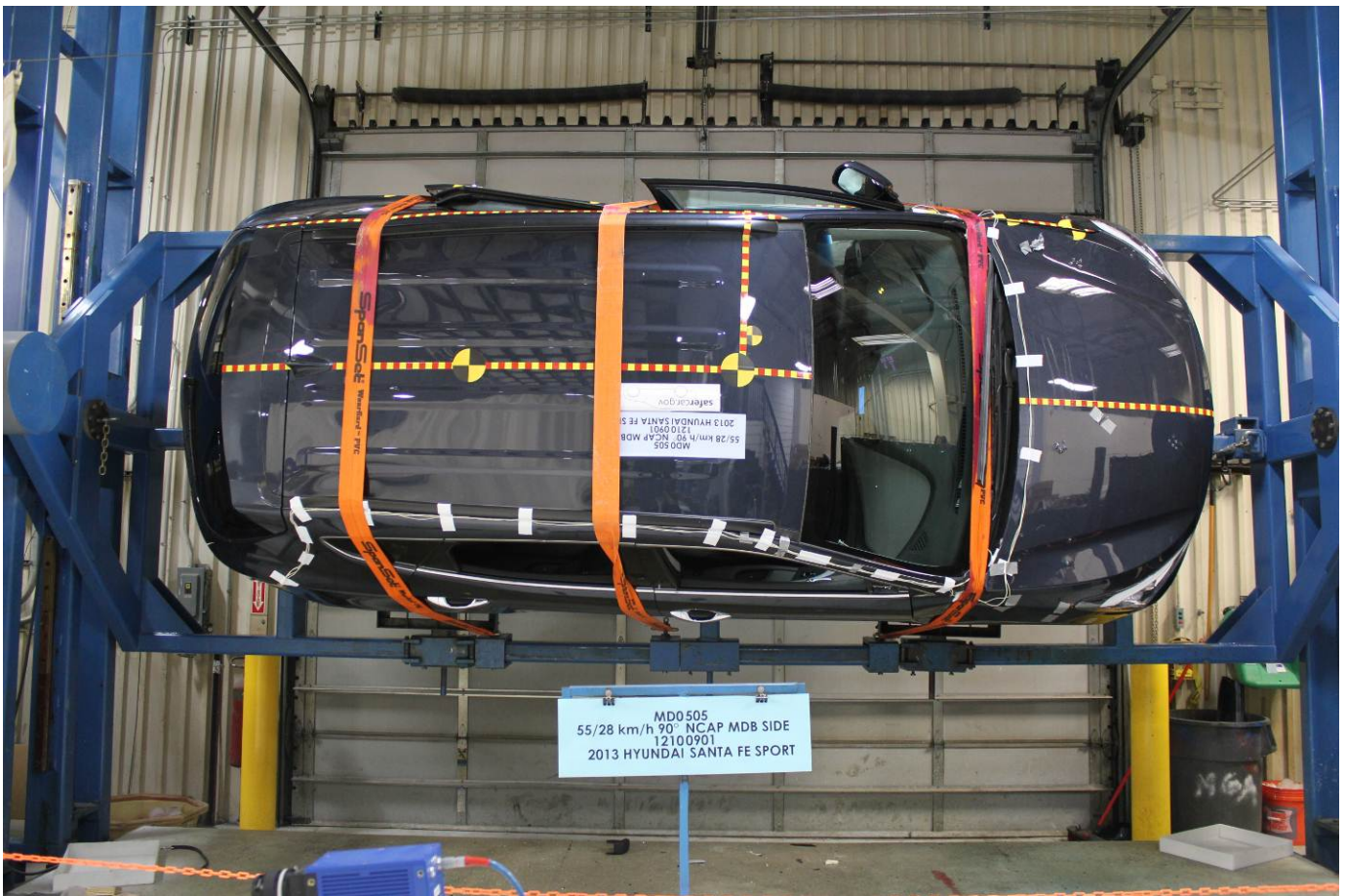
FMVSS No. 301 Static Rollover 270 Degrees
