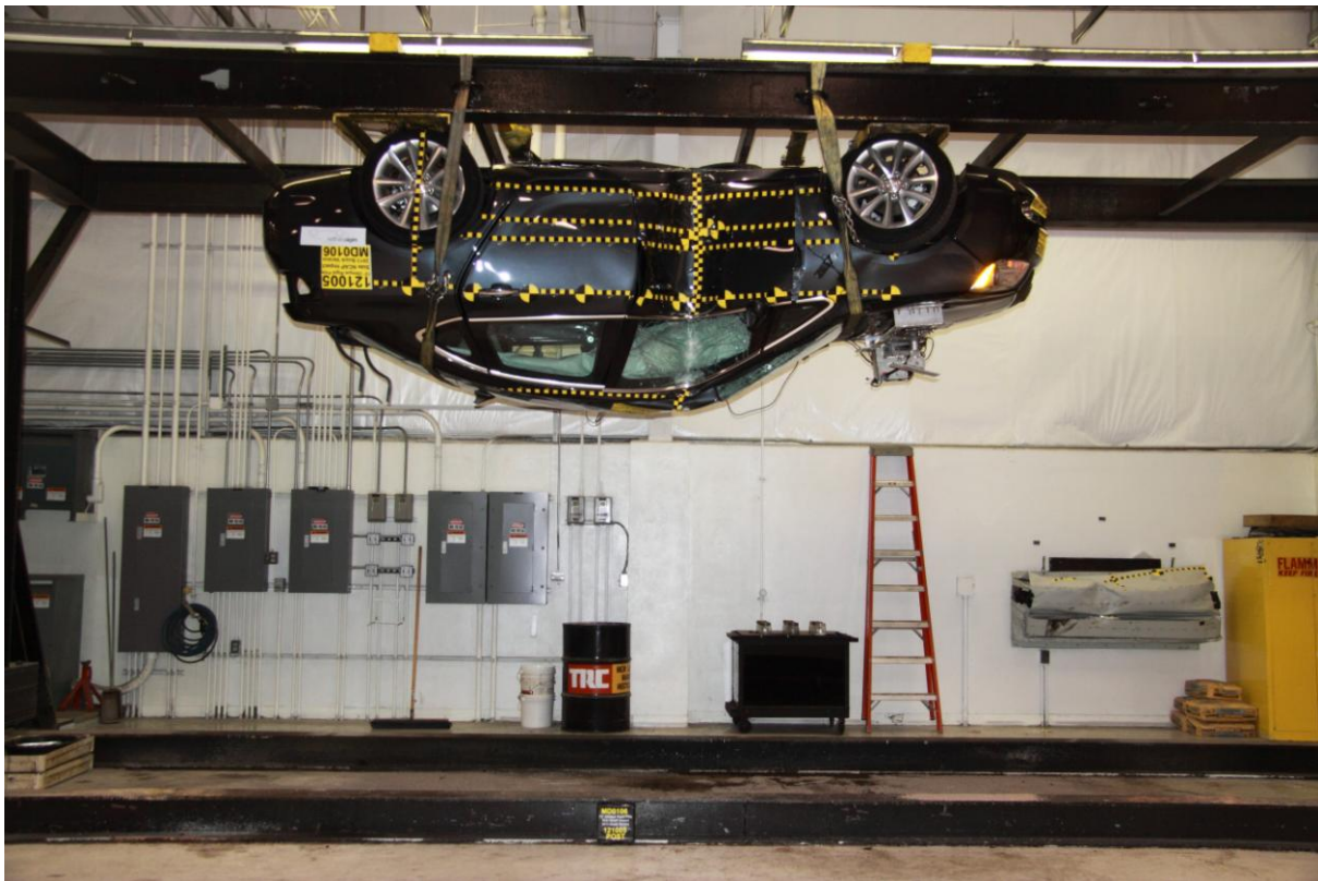
065 FMVSS No. 301 Static Rollover 180 Degrees
