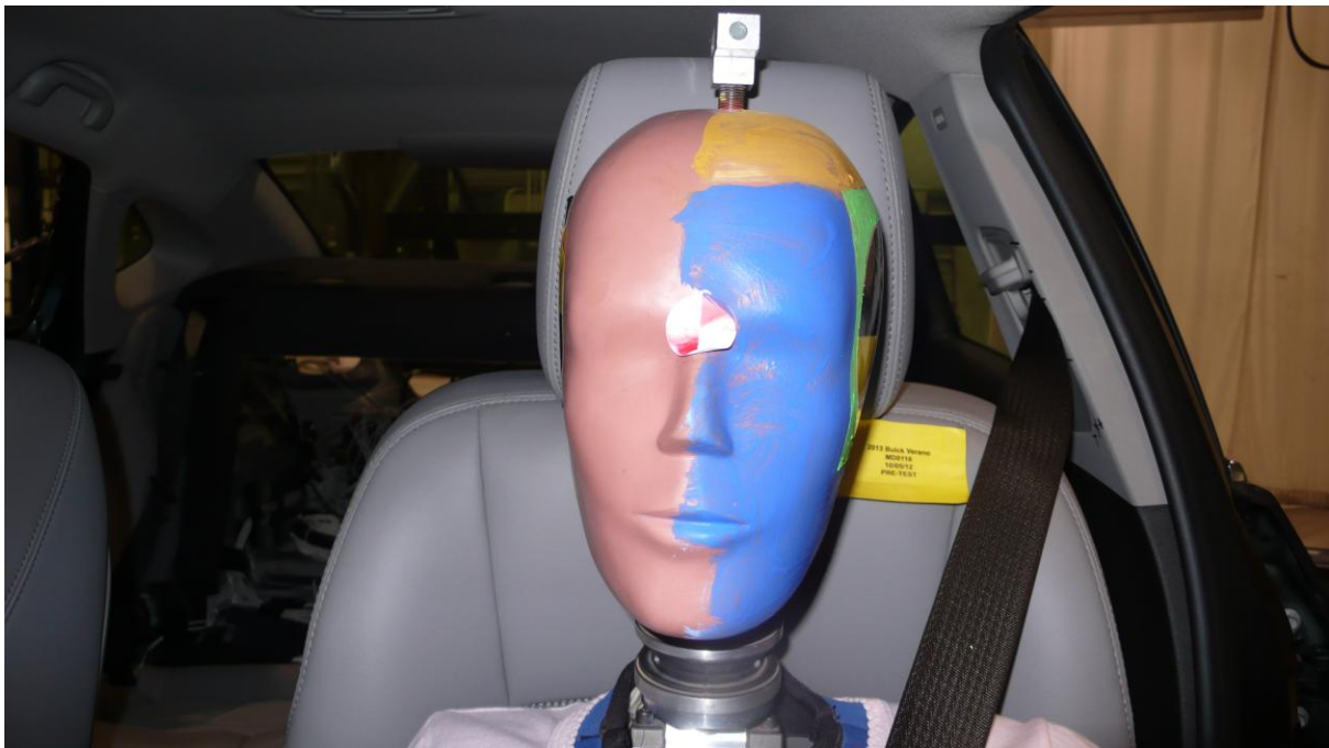
027 Pre-Test Front View of Dummy Head and Shoulders in Relation to Head Restraint
