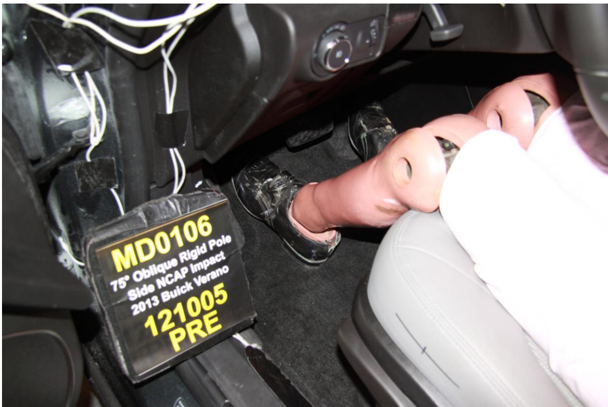
032 Pre-Test Placement of Dummy Feet
