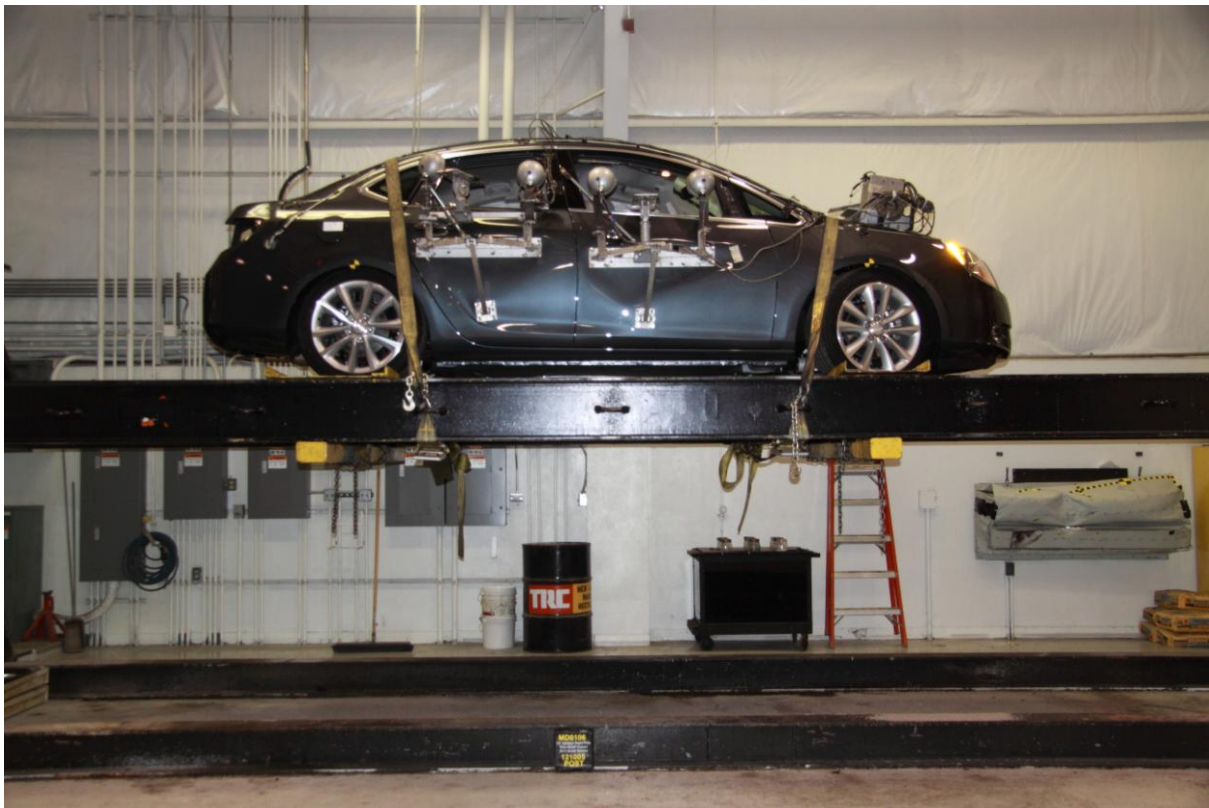
063 FMVSS No. 301 Static Rollover 0 Degrees
