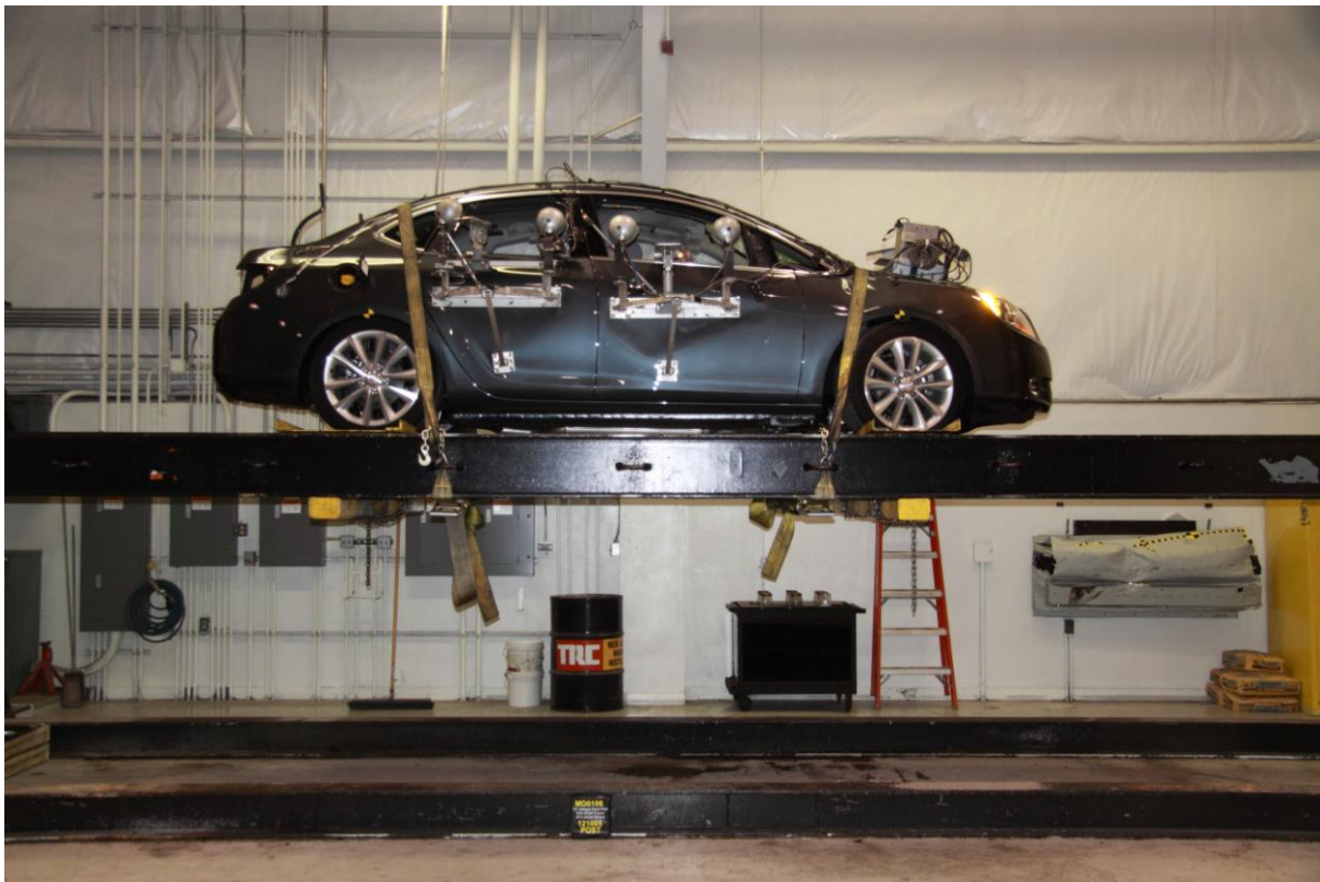
067 FMVSS No. 301 Static Rollover 360 Degrees
