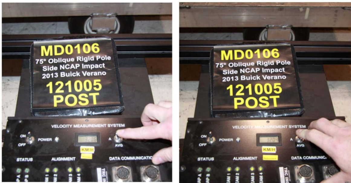
062 Post-Test Primary and Redundant Speed Trap Read-Out
