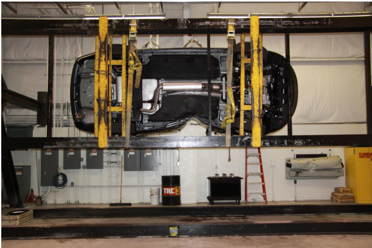
066 FMVSS No. 301 Static Rollover 270 Degrees
