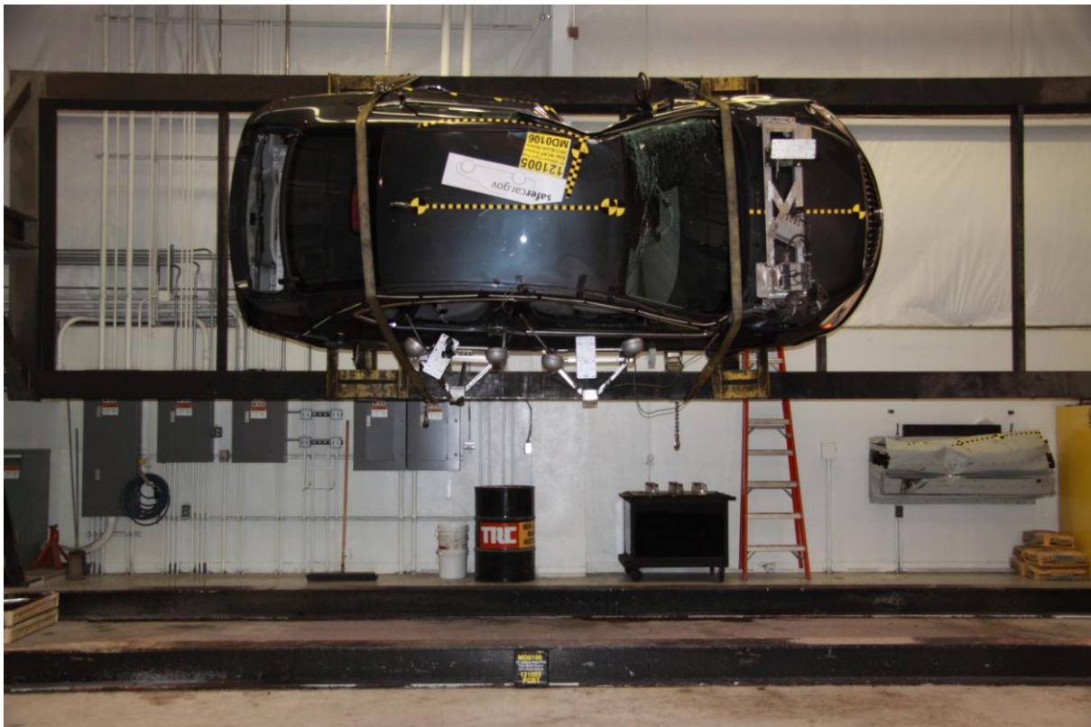
064 FMVSS No. 301 Static Rollover 90 Degrees
