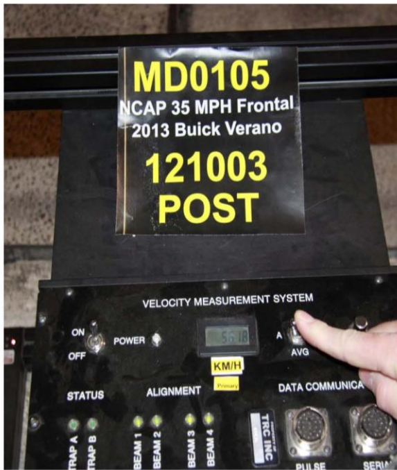
071 Post-test Speed Trap Read-out
