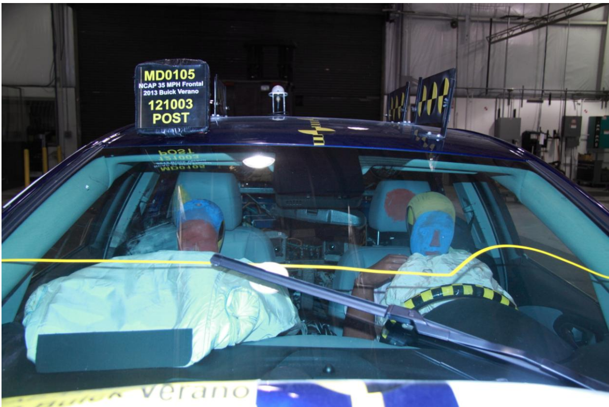
018 Post-test Windshield View
