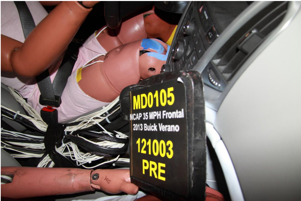
029 Pre-test Dummy Cable Routing
