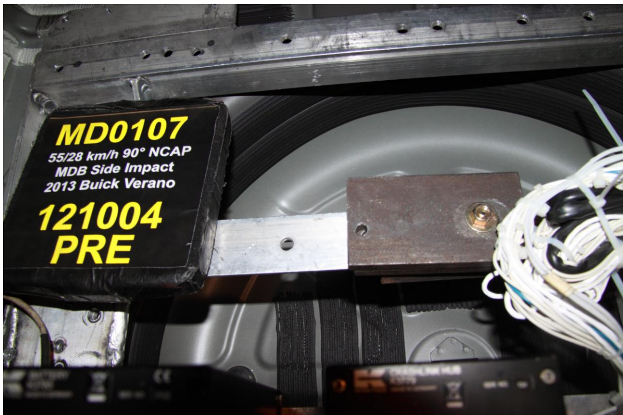
094 Pre-Test Ballast View
