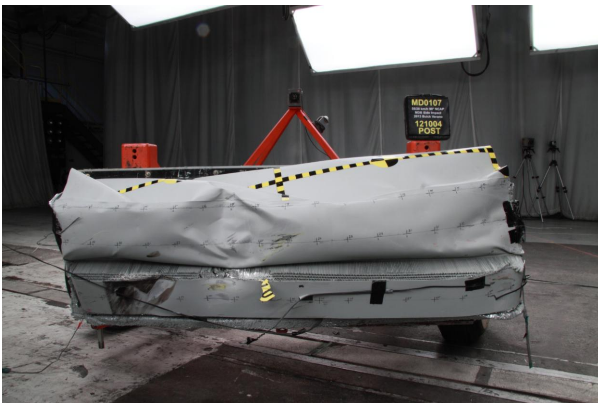
085 Post-Test Front View of MDB Impactor Face
