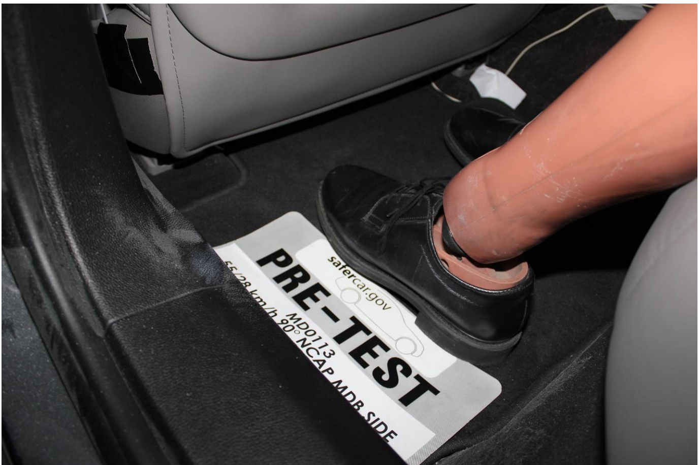
Pre-Test Placement of Rear Passenger Dummy's Feet
