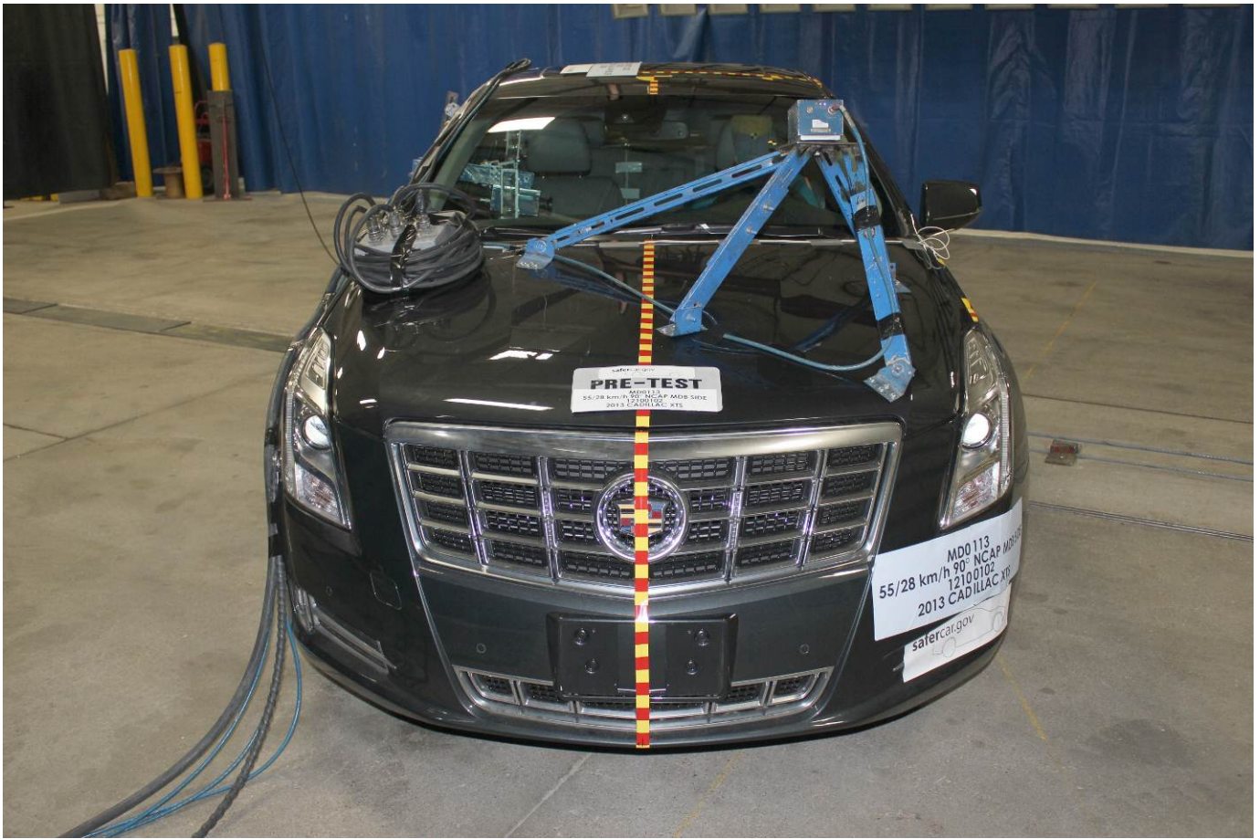
Pre-Test Frontal View of Test Vehicle
