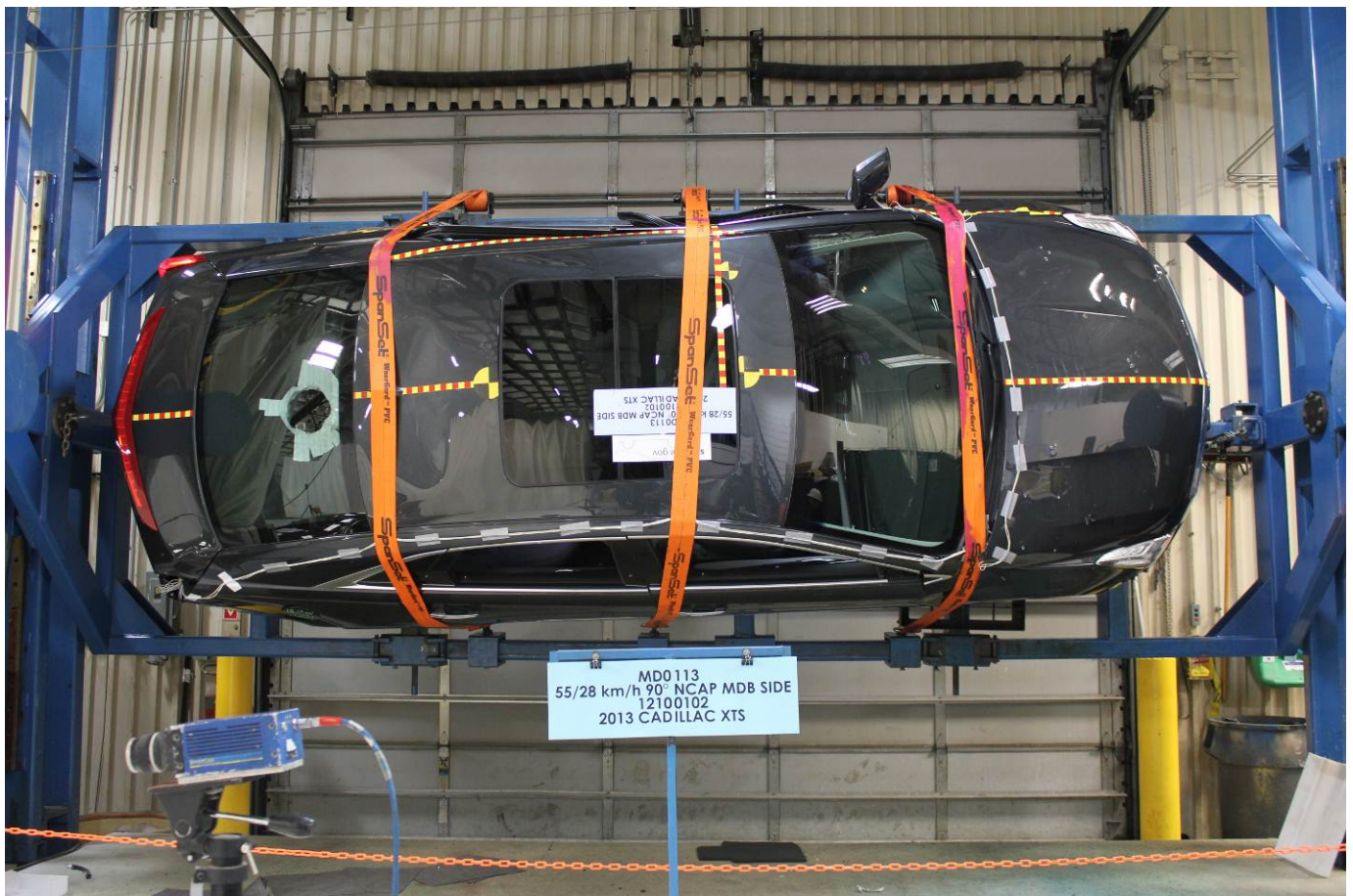
FMVSS No. 301 Static Rollover 90 Degrees
