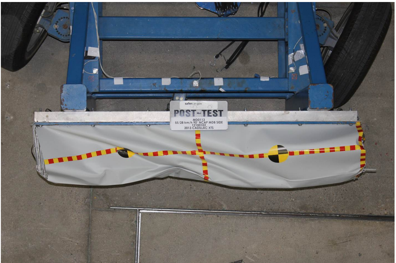
Post-Test Top View of MDB Impactor Face
