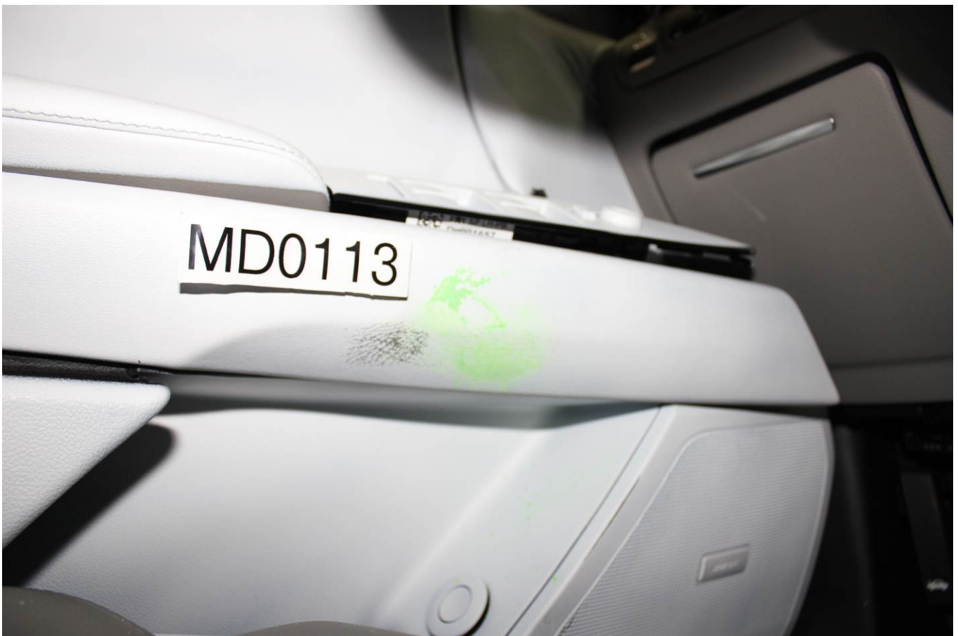
Post-Test Driver Dummy Close-up Knee Contact View
