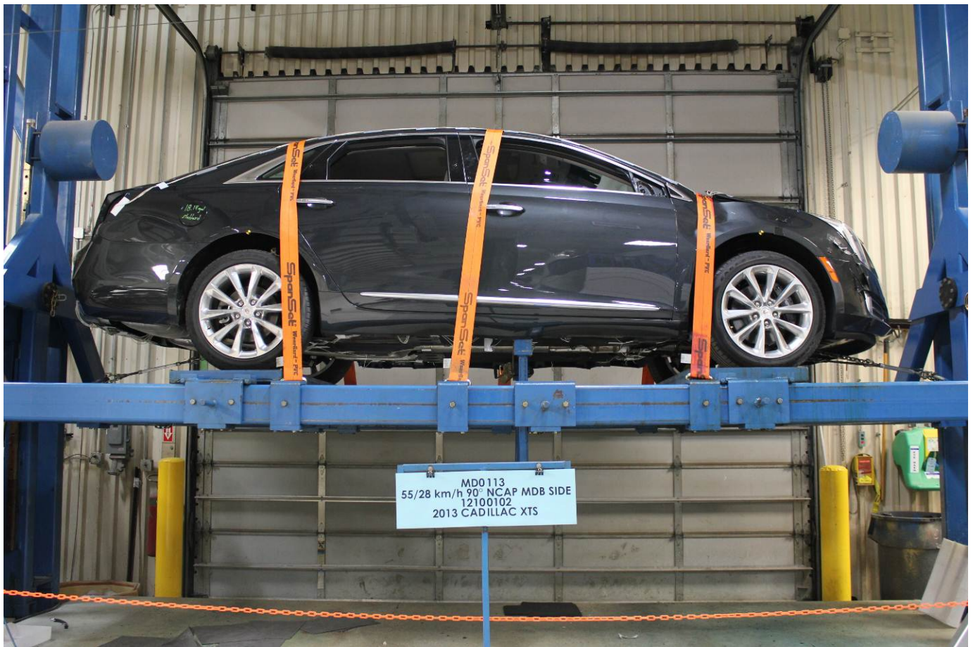
FMVSS No. 301 Static Rollover 0 Degrees
