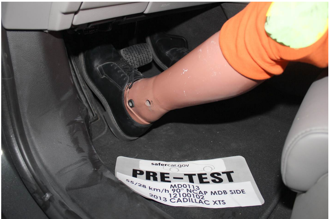
Pre-Test Placement of Driver Dummy's Feet
