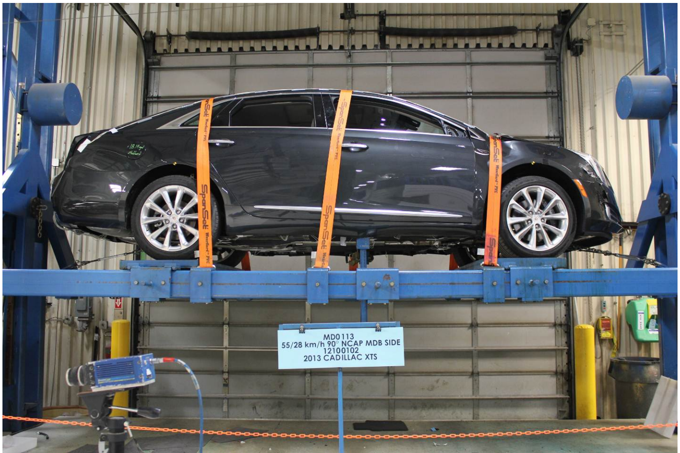
FMVSS No. 301 Static Rollover 360 Degrees
