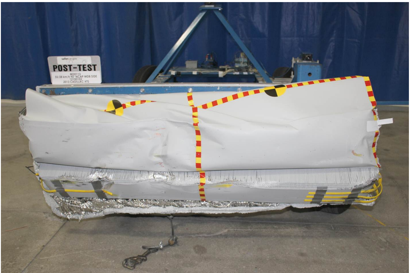
Post-Test Front View of MDB Impactor Face
