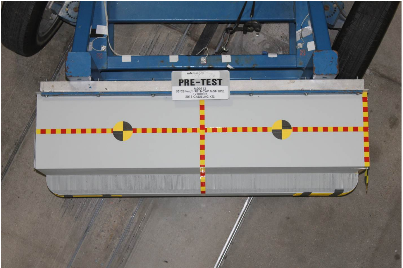
Pre-Test Top View of MDB Impactor Face
