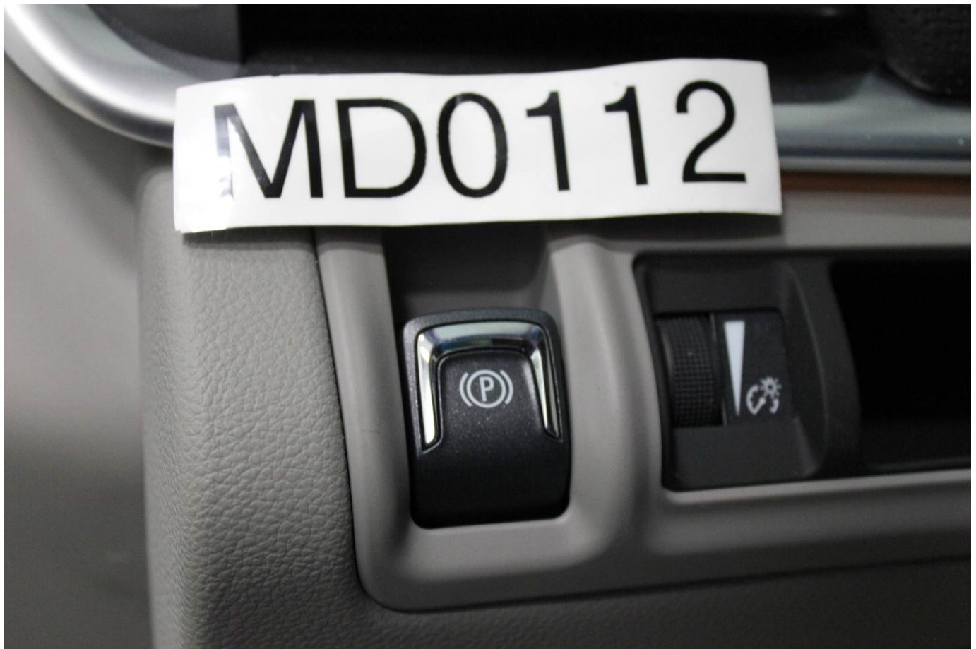
Pre-Test View of Disengaged Parking Brake
