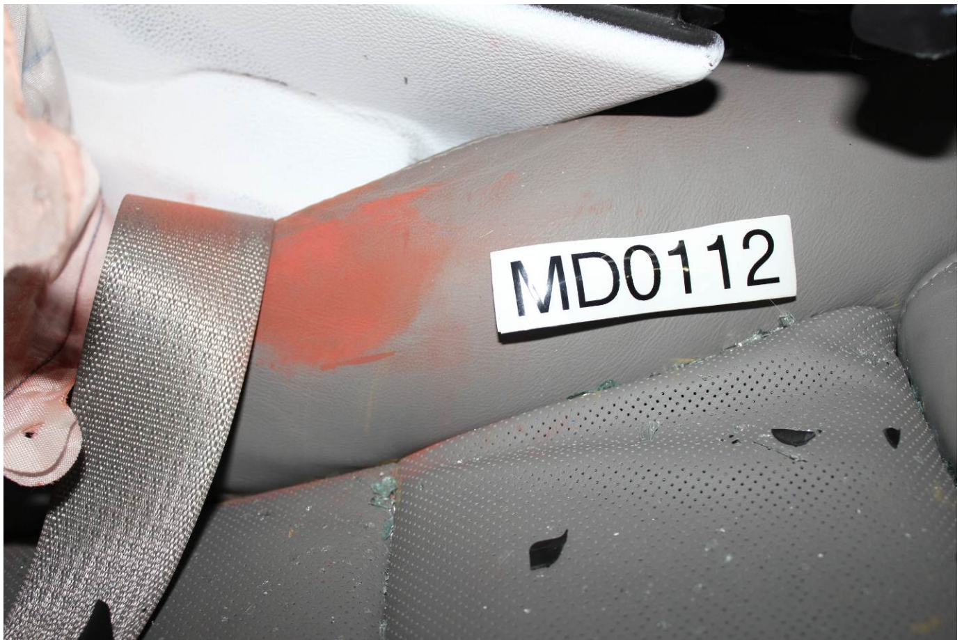
Post-Test Dummy Close-Up Pelvis Contact with Vehicle Interior View
