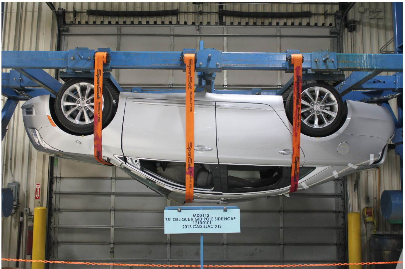
FMVSS No. 301 Static Rollover 180 Degrees
