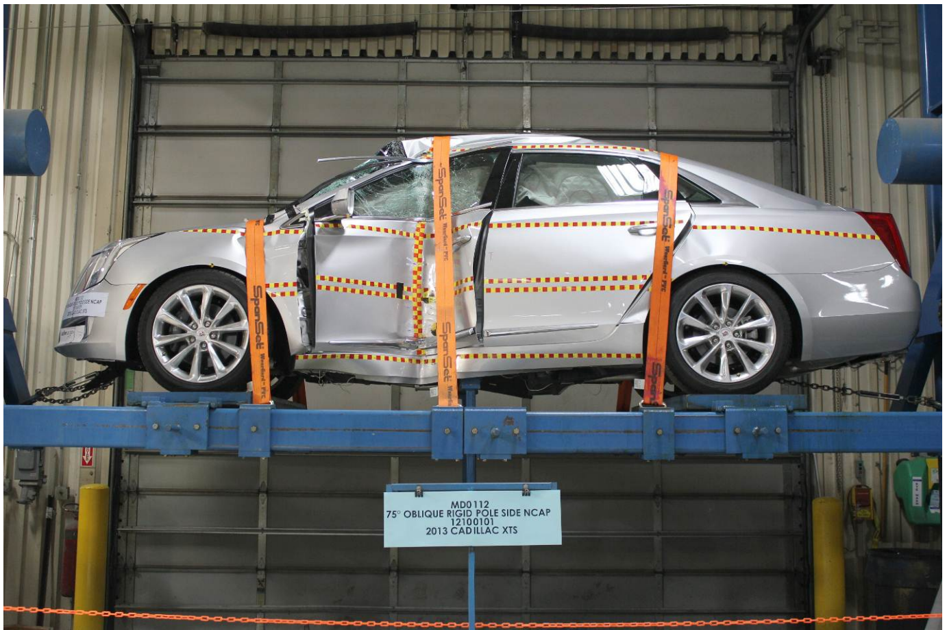
FMVSS No. 301 Static Rollover 0 Degrees
