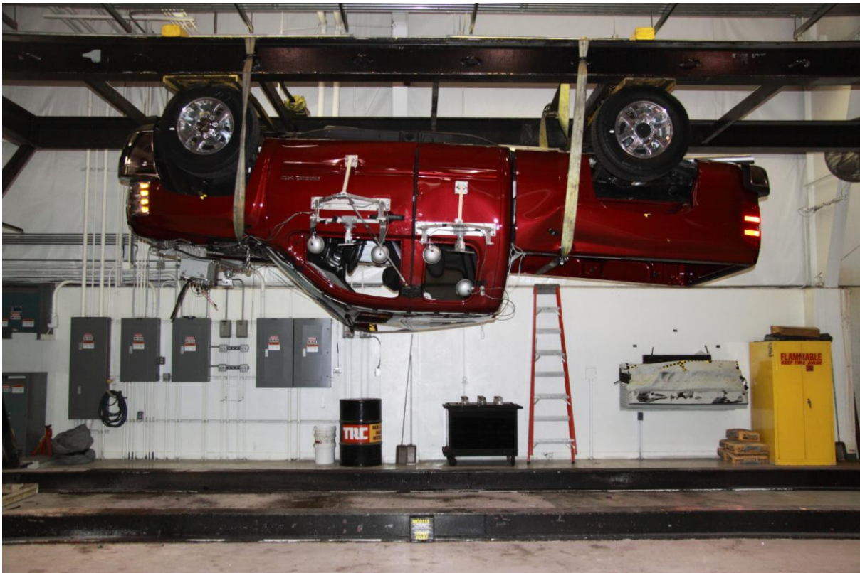
065 FMVSS No. 301 Static Rollover 180 Degrees
