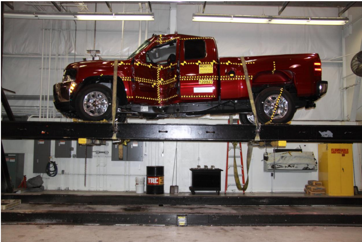
067 FMVSS No. 301 Static Rollover 360 Degrees
