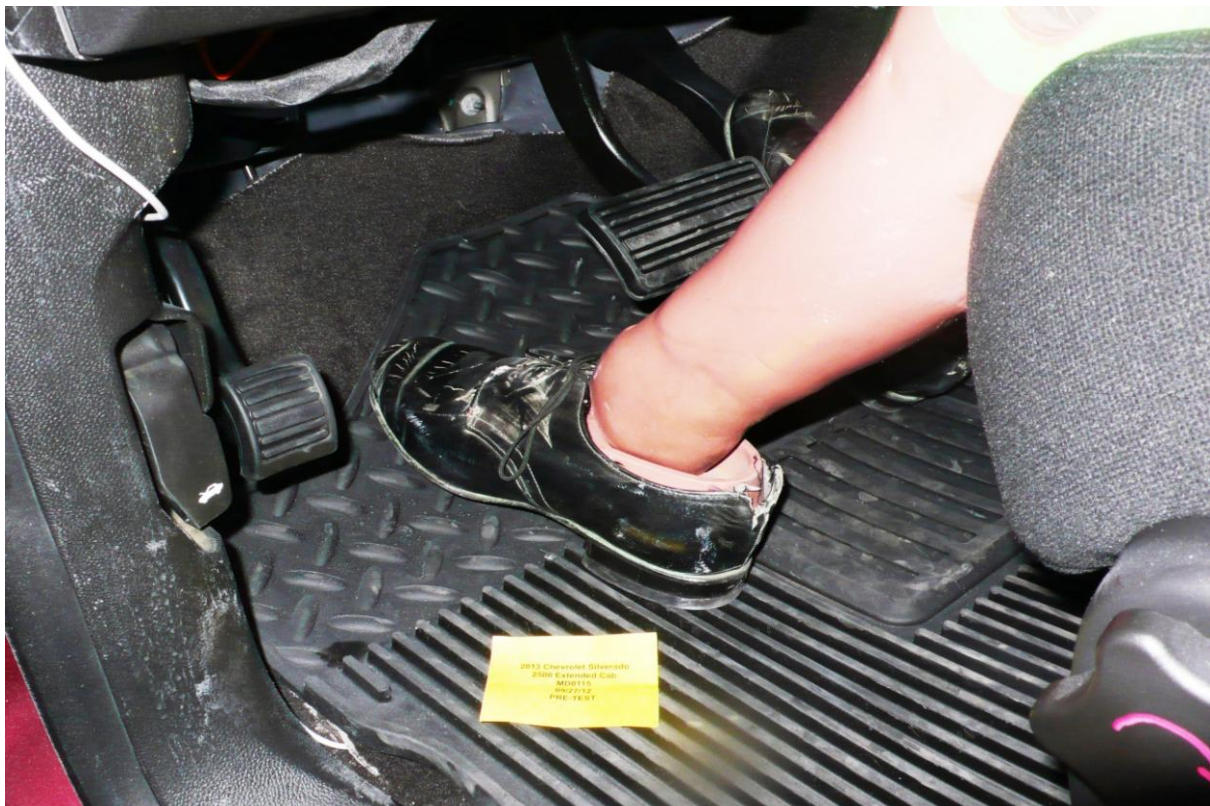
032 Pre-Test Placement of Dummy Feet
