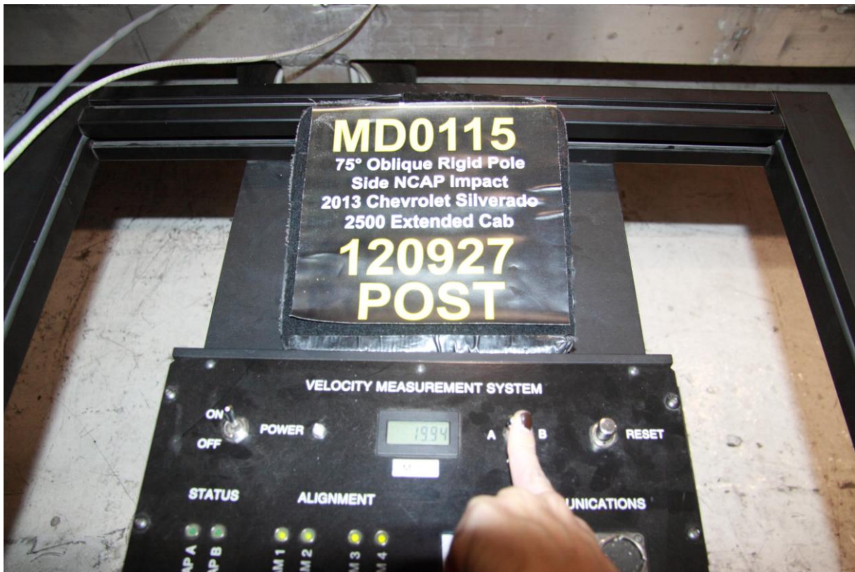
062 Post-Test Primary and Redundant Speed Trap Read-Out
