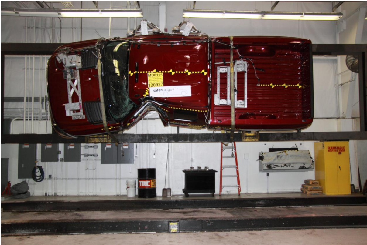
064 FMVSS No. 301 Static Rollover 90 Degrees
