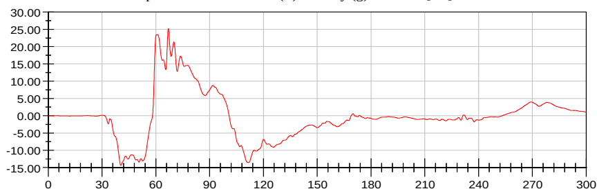
Driver Lower Spine T12 Resultant Primary (g) vs. Time [ms]
