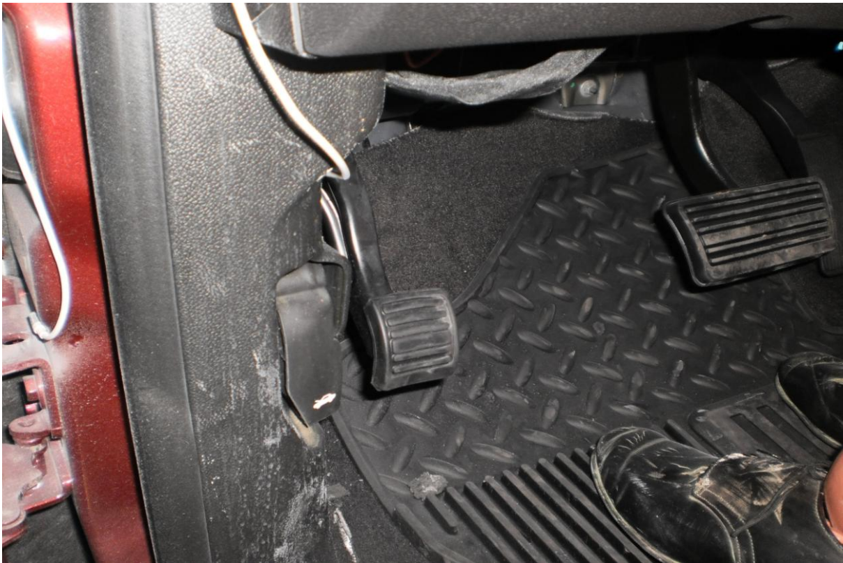
035 Pre-Test View of Disengaged Parking Brake
