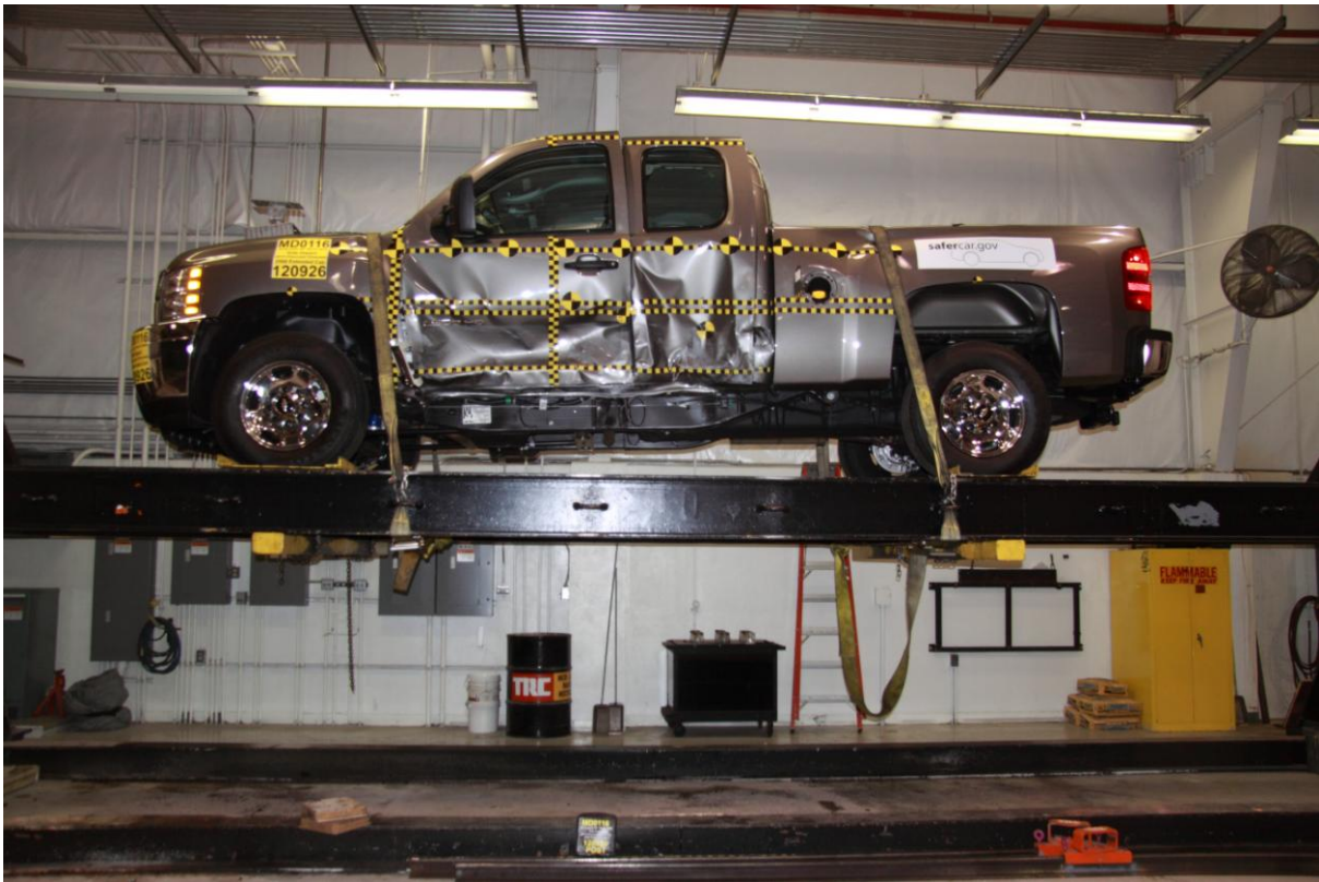
100 FMVSS No. 301 Static Rollover 360 Degrees
