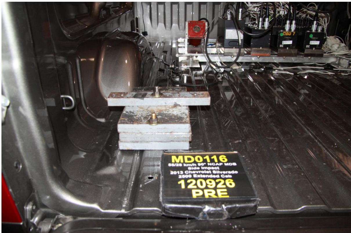
094 Pre-Test Ballast View
