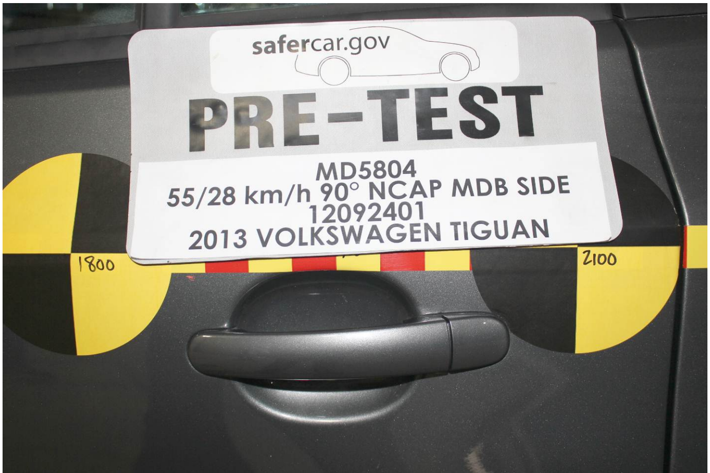
Pre-Test Left Rear Door Latch Close-Up
