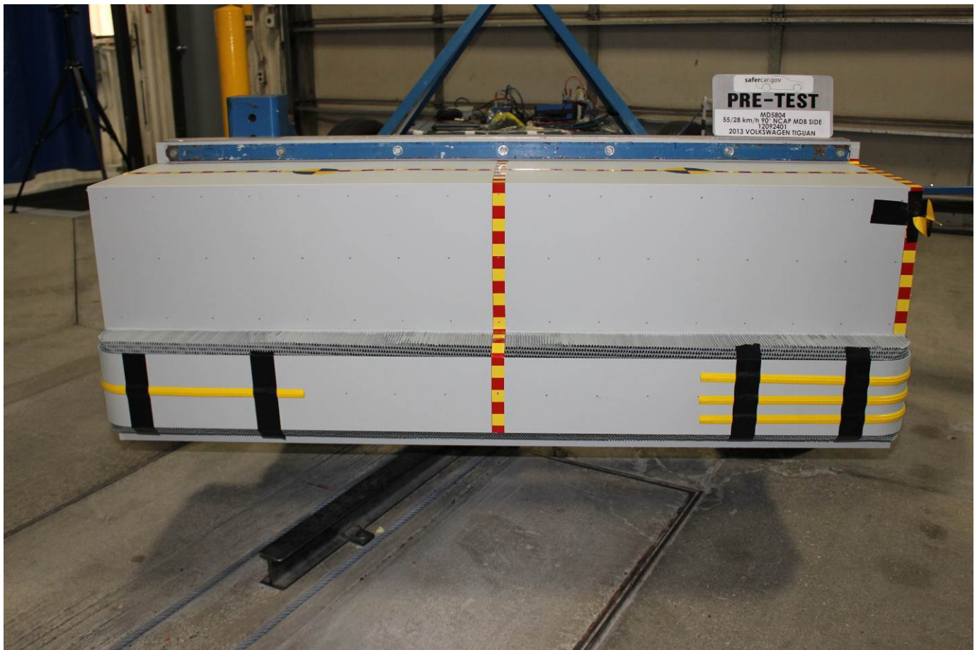
Pre-Test Front View of MDB Impactor Face
