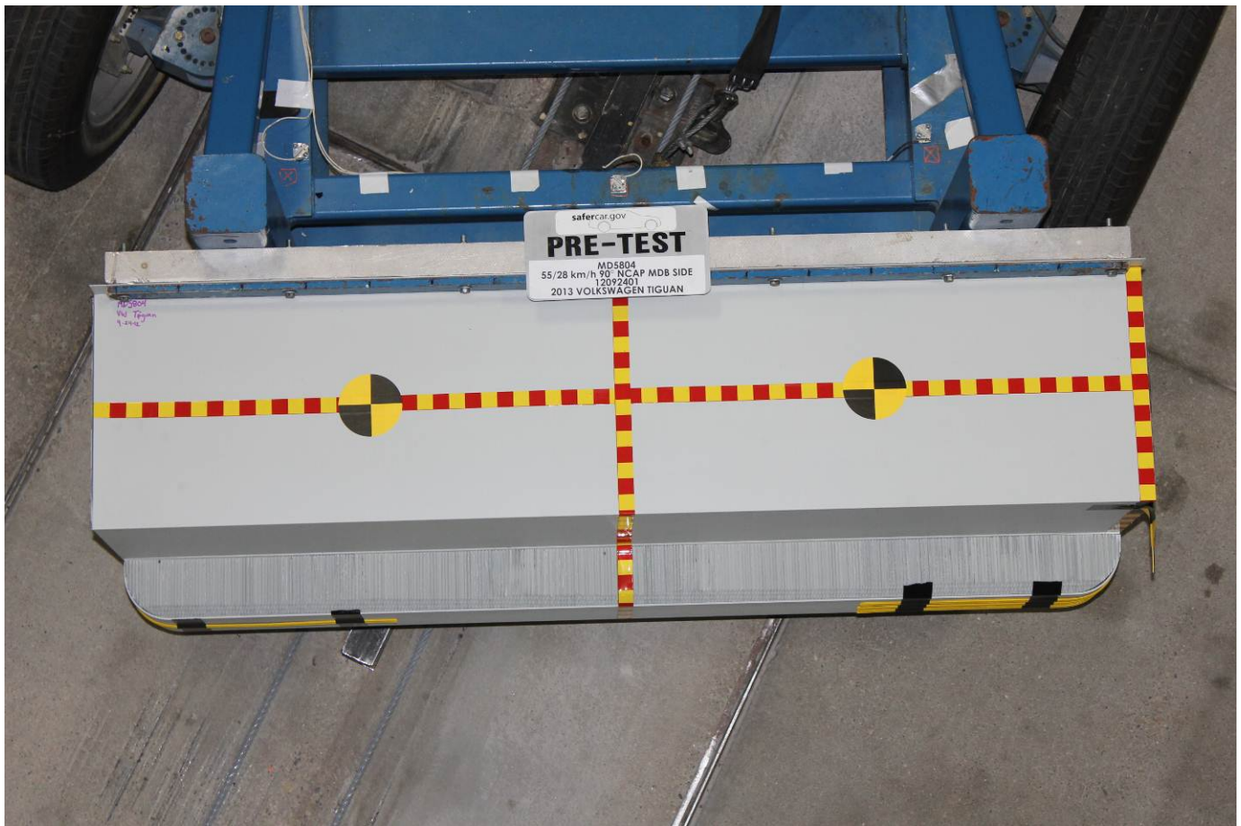
Pre-Test Top View of MDB Impactor Face
