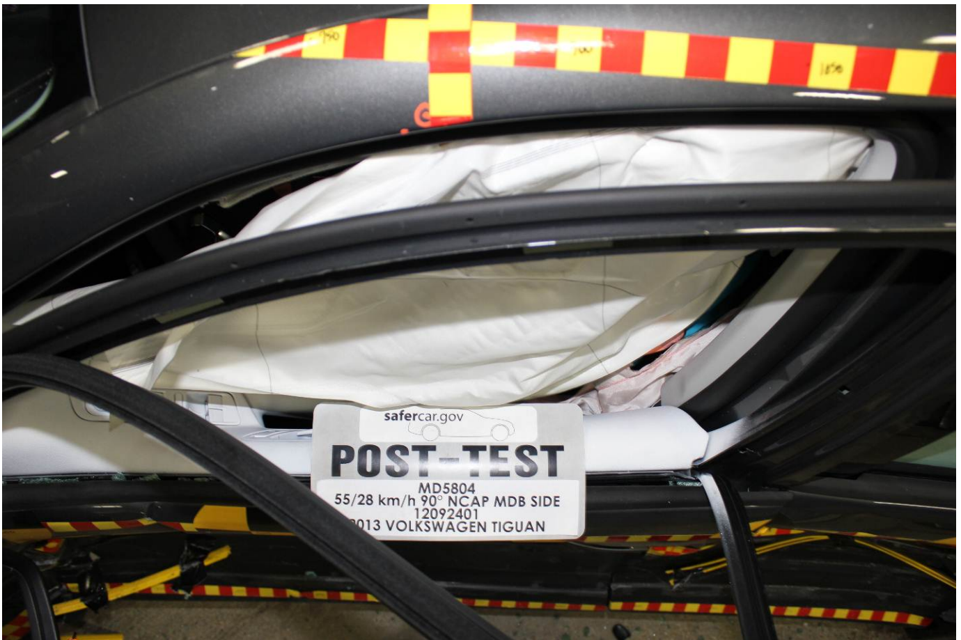
Post-Test Driver Dummy and Door Clearance View
