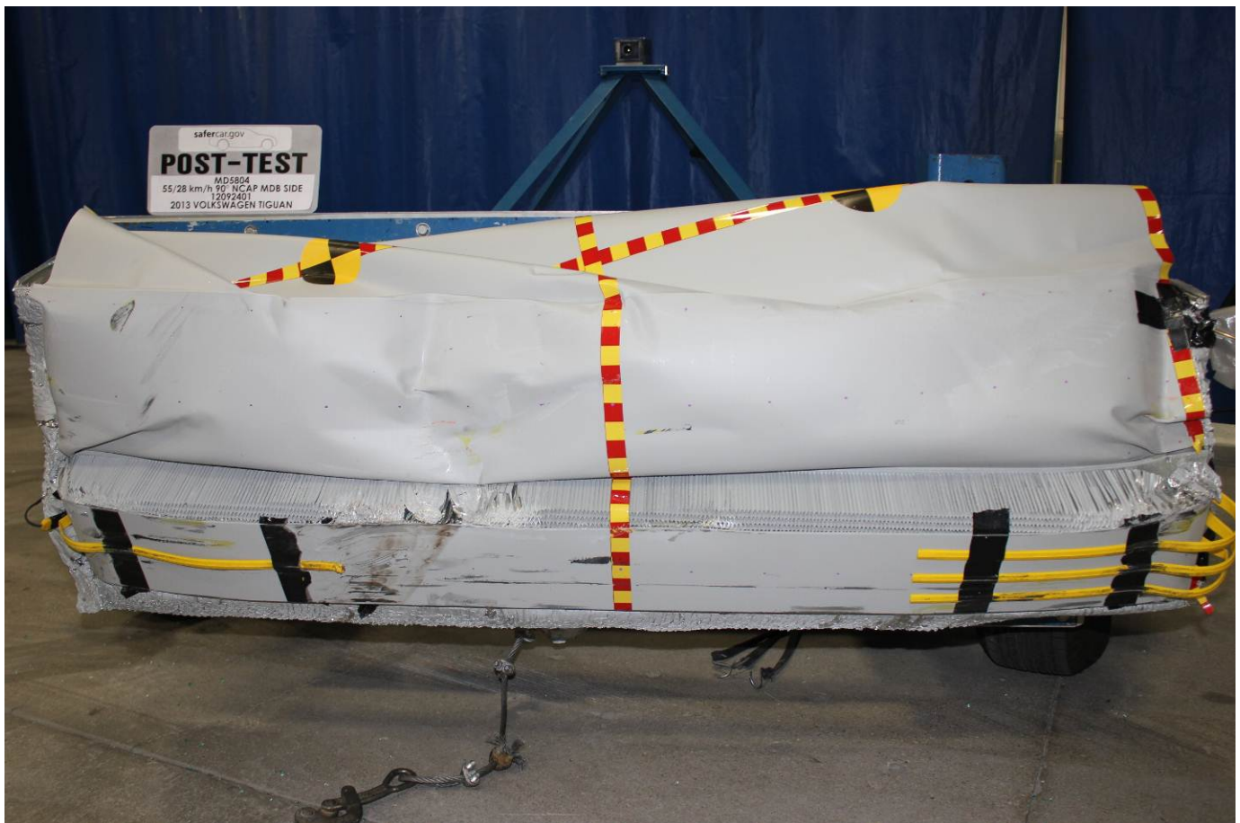
Post-Test Front View of MDB Impactor Face
