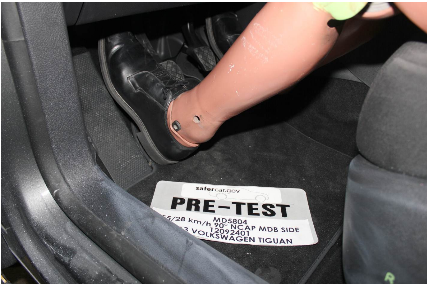
Pre-Test Placement of Driver Dummy's Feet
