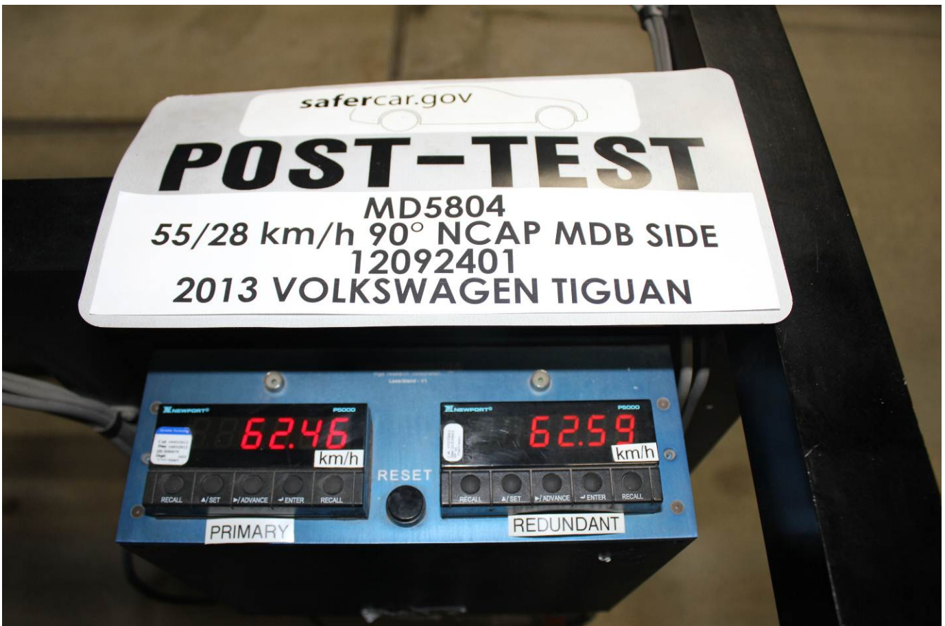
Post-Test Primary and Redundant Speed Trap Read-Out
