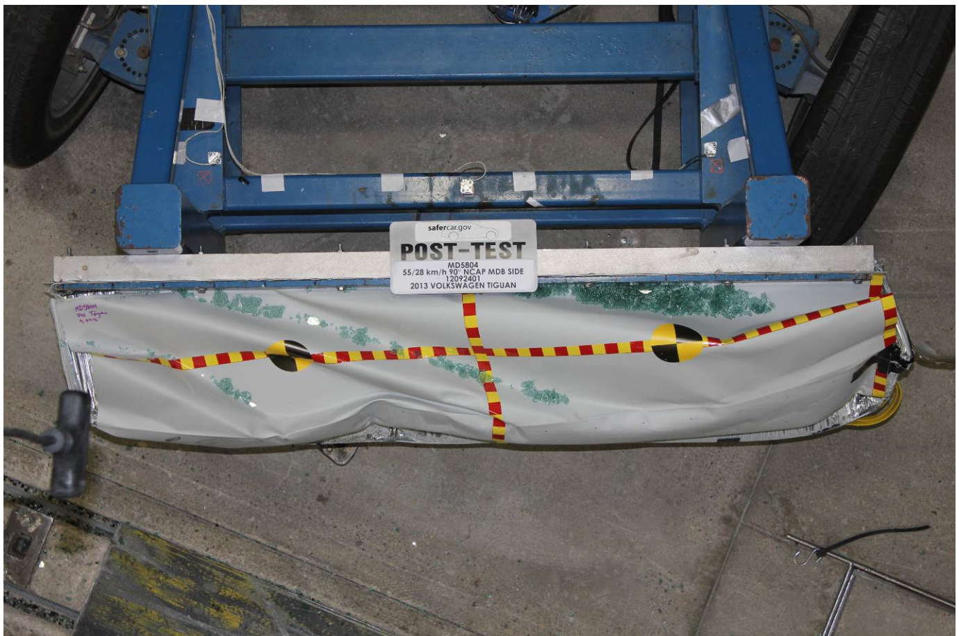
Post-Test Top View of MDB Impactor Face
