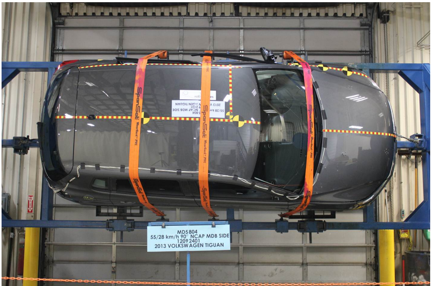
FMVSS No. 301 Static Rollover 90 Degrees
