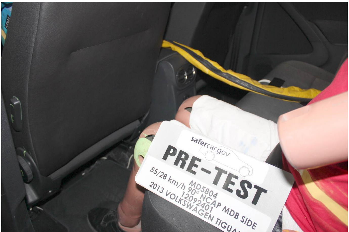
Pre-Test Placement of Rear Passenger Dummy's Feet
