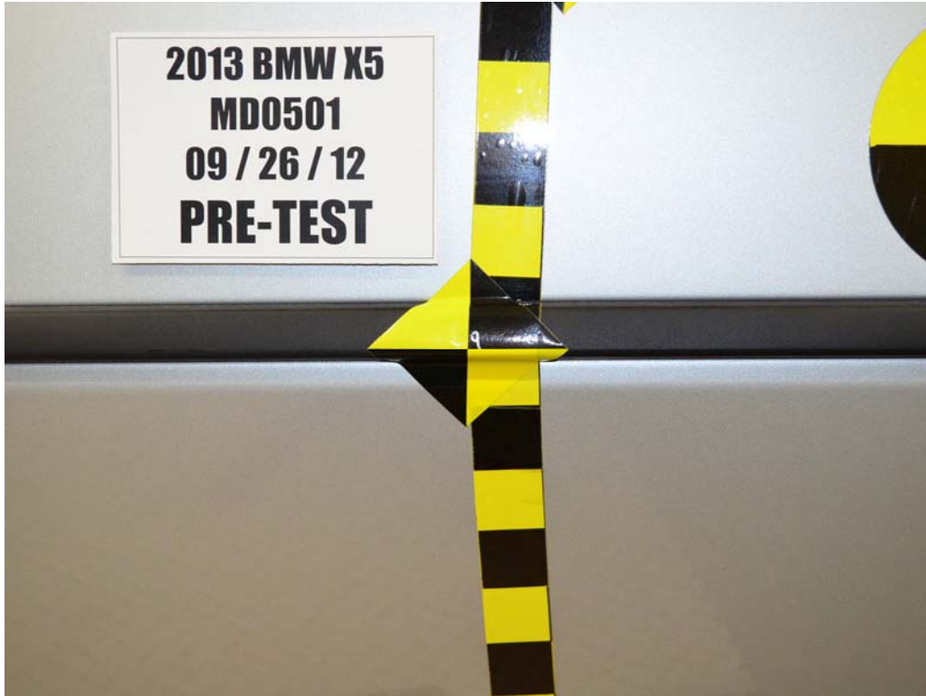
FIGURE 19. Pre-Test Close-Up View of Impact Point Target
