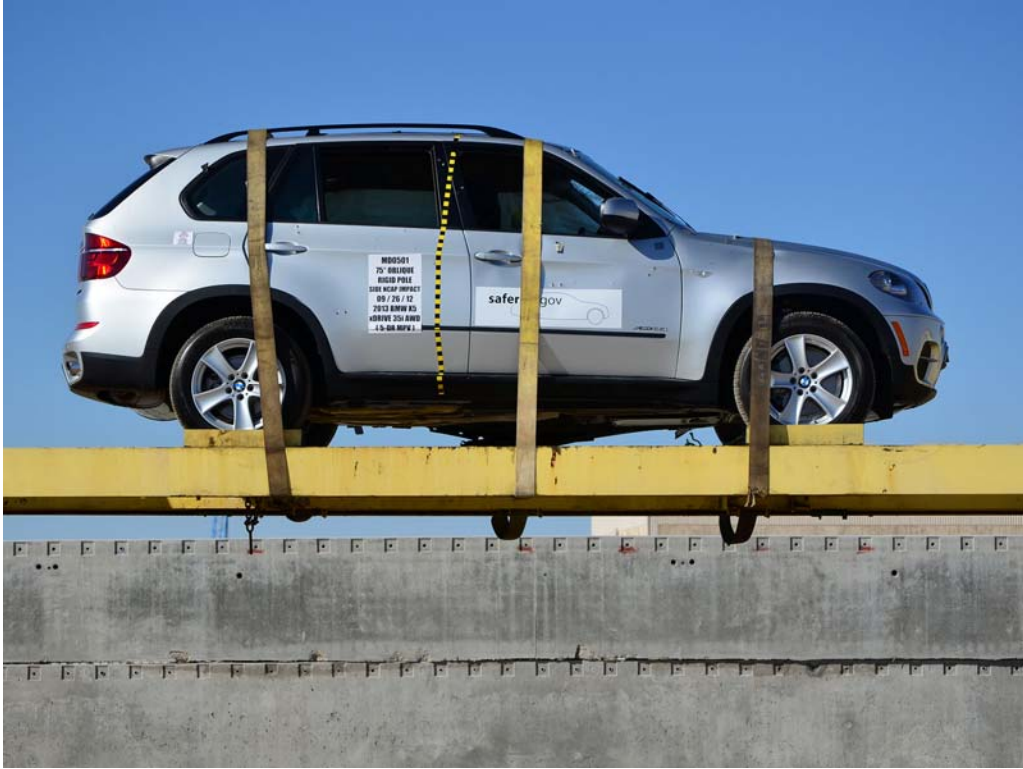
FIGURE 67. FMVSS No. 301-305 Rollover 360 Degrees
