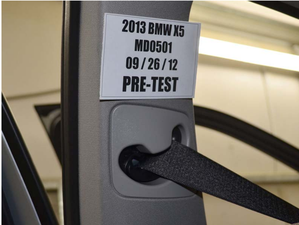
FIGURE 33. Pre-Test View of Belt Anchorage for Dummy
