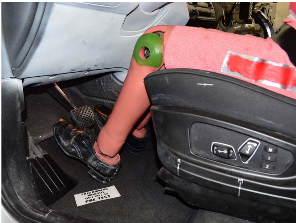
FIGURE 32. Pre-Test Placement of Dummy's Feet
