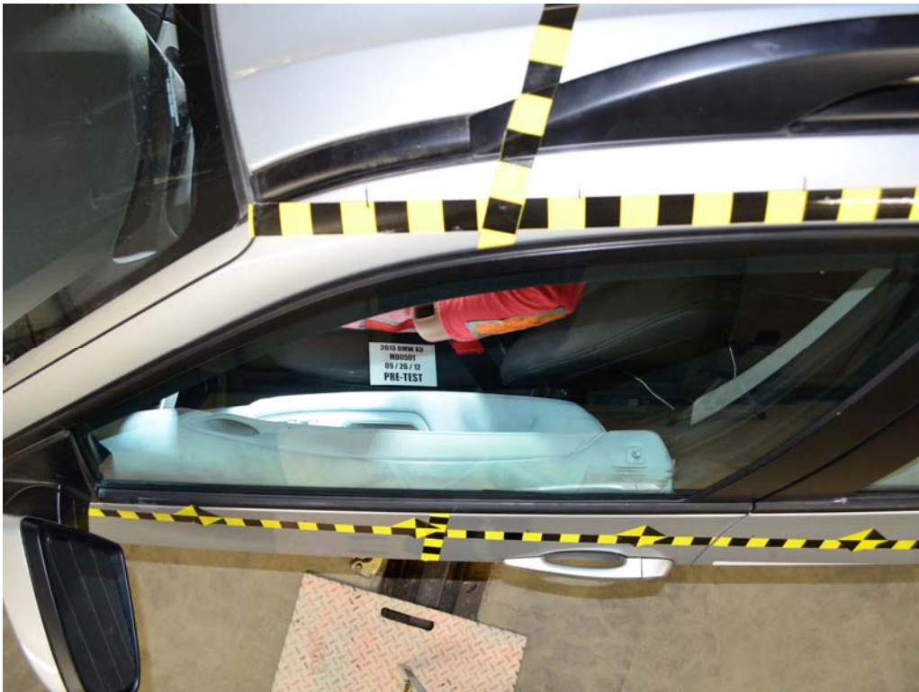
FIGURE 40. Pre-Test Dummy and Door Clearance View
