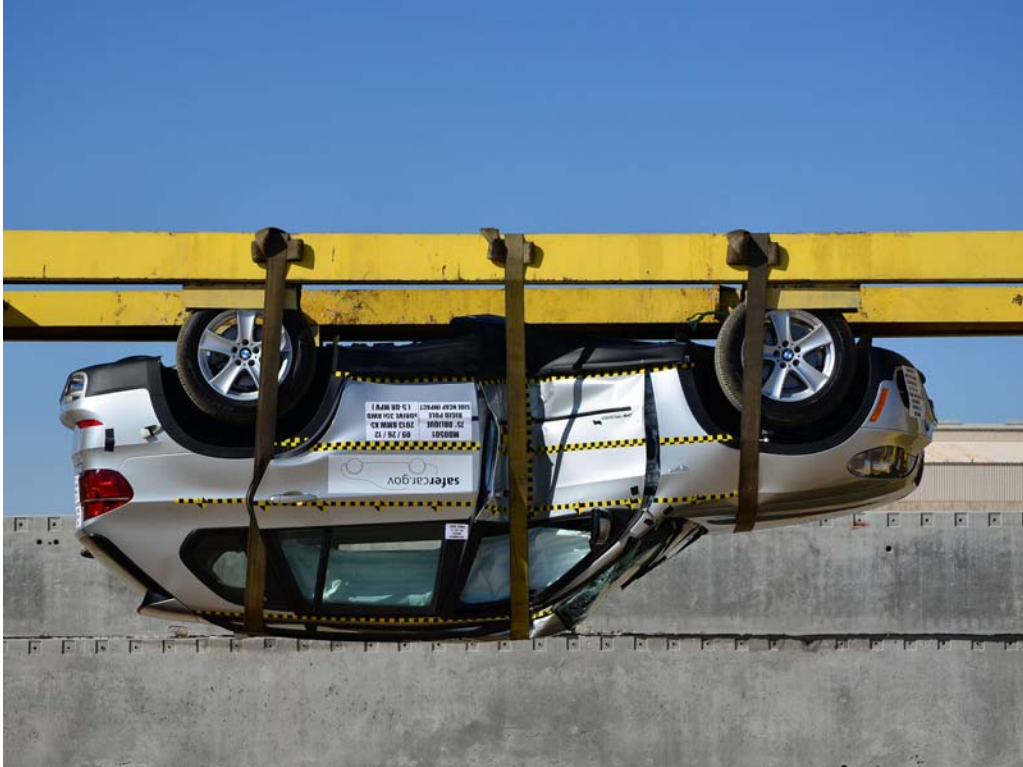
FIGURE 65. FMVSS No. 301-305 Rollover 180 Degrees
