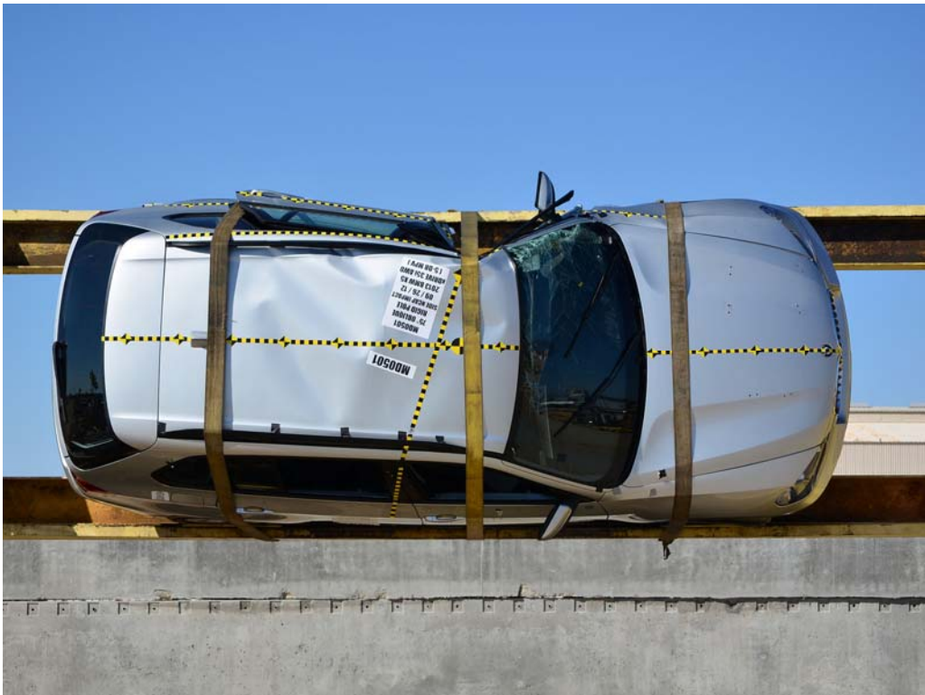
FIGURE 64. FMVSS No. 301-305 Rollover 90 Degrees
