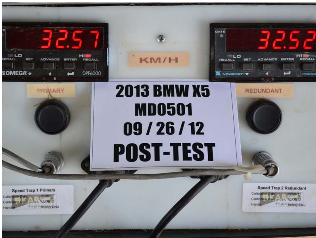
FIGURE 62. Post-Test Primary and Redundant Speed Trap Read-Out
