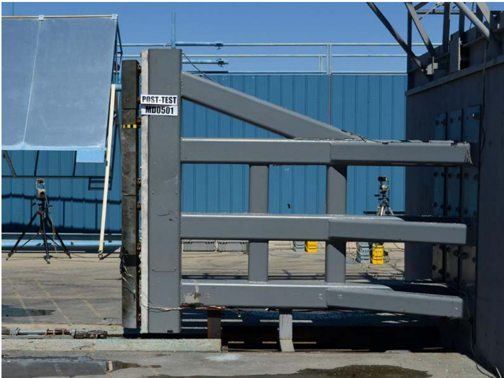
FIGURE 60. Post-Test Pole Barrier Side View
