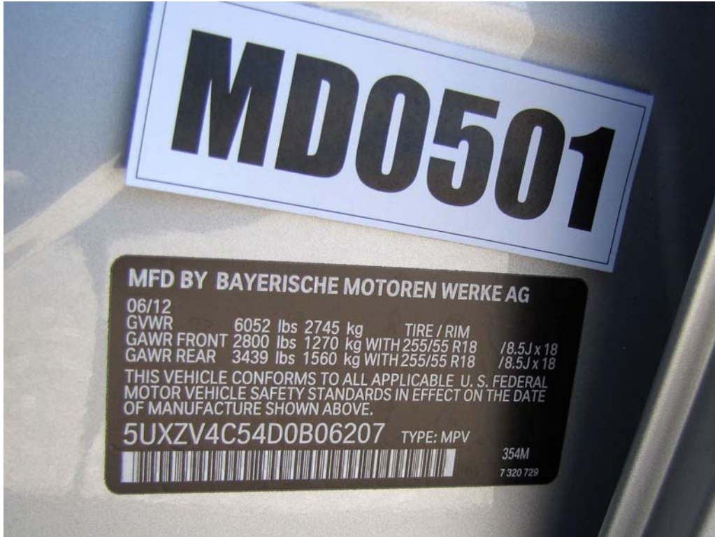
FIGURE 55. Close-Up View of Vehicle's Certification Label
