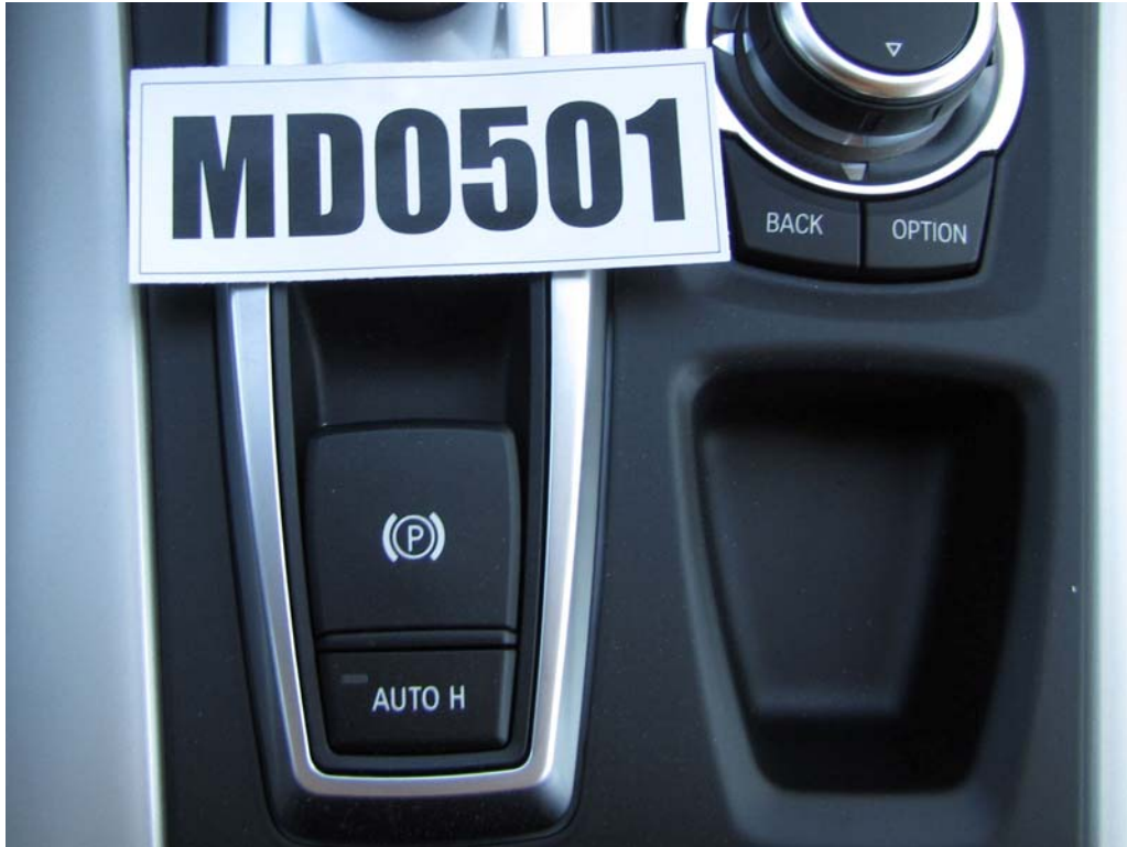
FIGURE 35. Pre-Test View of Disengaged Parking Brake
