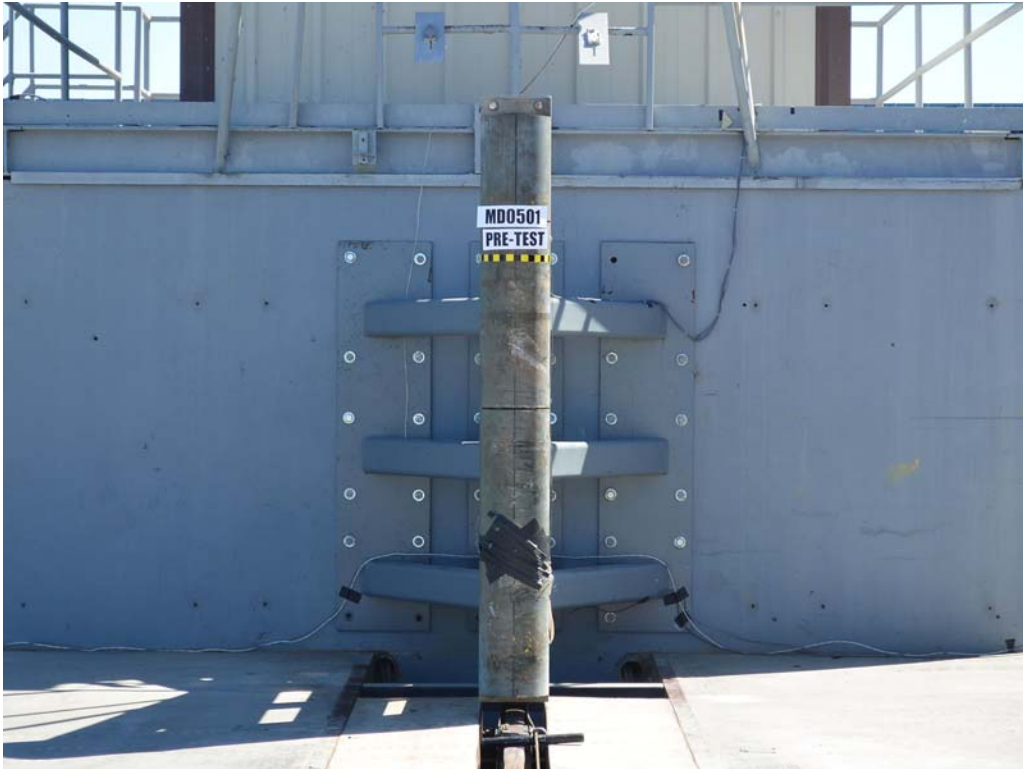
FIGURE 57. Pre-Test Pole Barrier Front View
