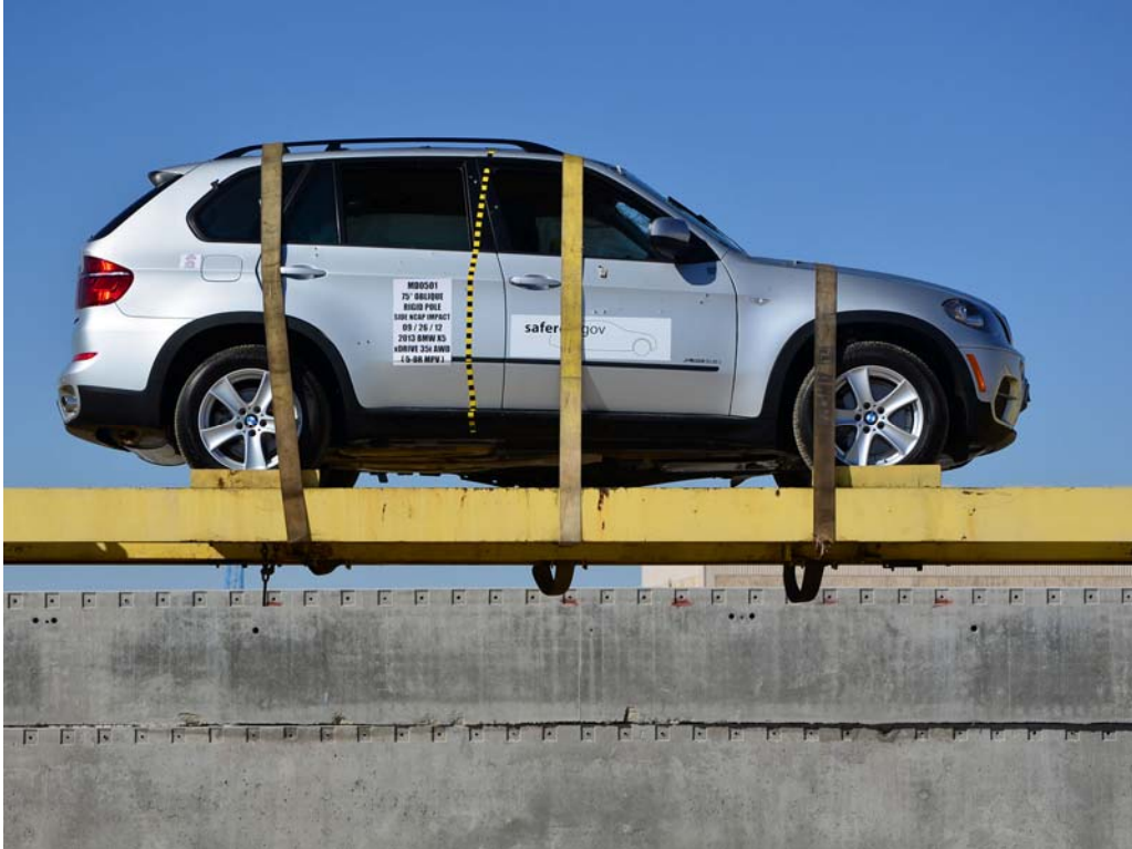
FIGURE 63. FMVSS No. 301-305 Rollover 0 Degrees
