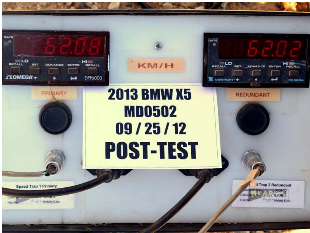
FIGURE 95. Post-Test Primary and Redundant Speed Trap Read-Out
