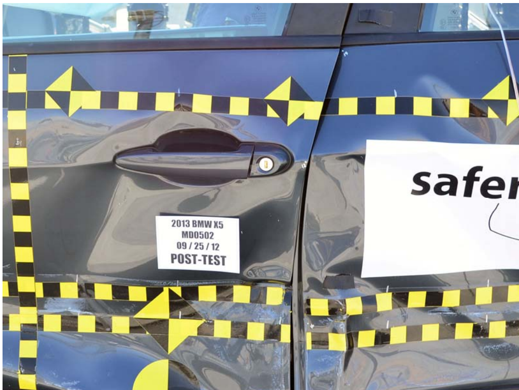
FIGURE 22. Post-Test Left Front Door Latch Close-Up
