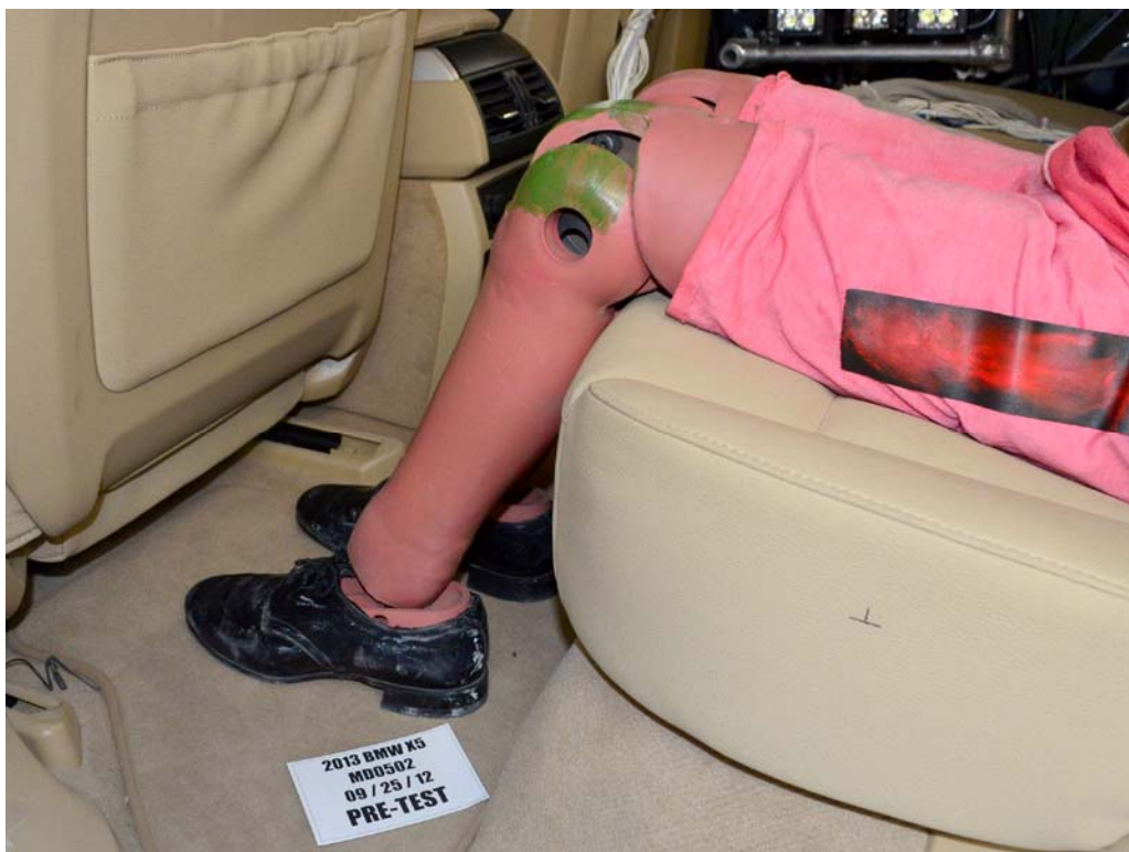
FIGURE 64. Pre-Test Placement of Rear Passenger Dummy's Feet
