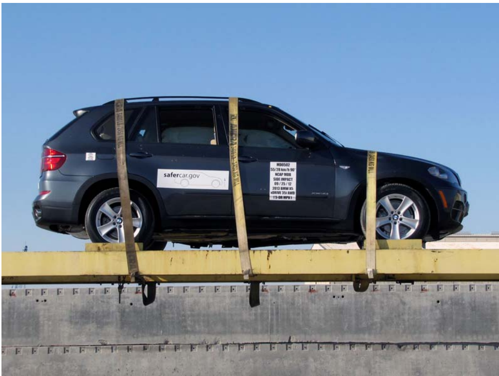
FIGURE 100. FMVSS No. 301 Static Rollover 360 Degrees
