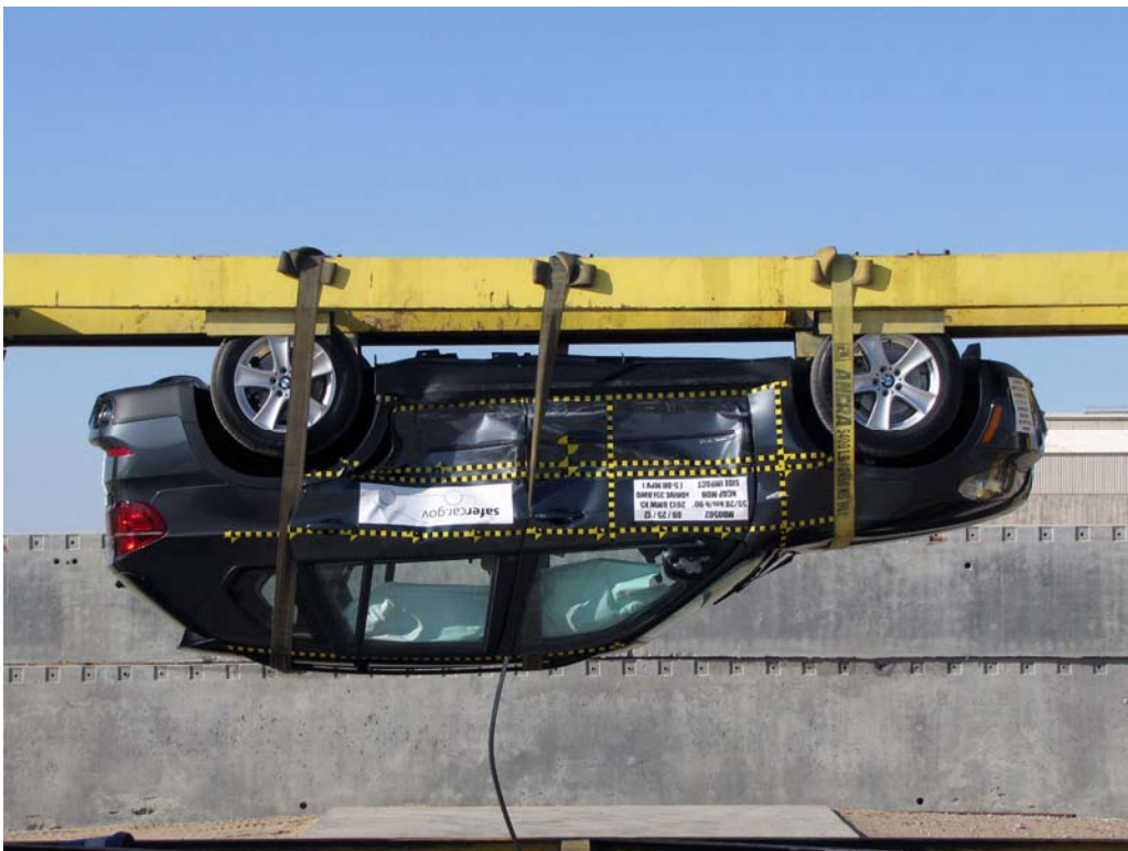
FIGURE 98. FMVSS No. 301 Static Rollover 180 Degrees
