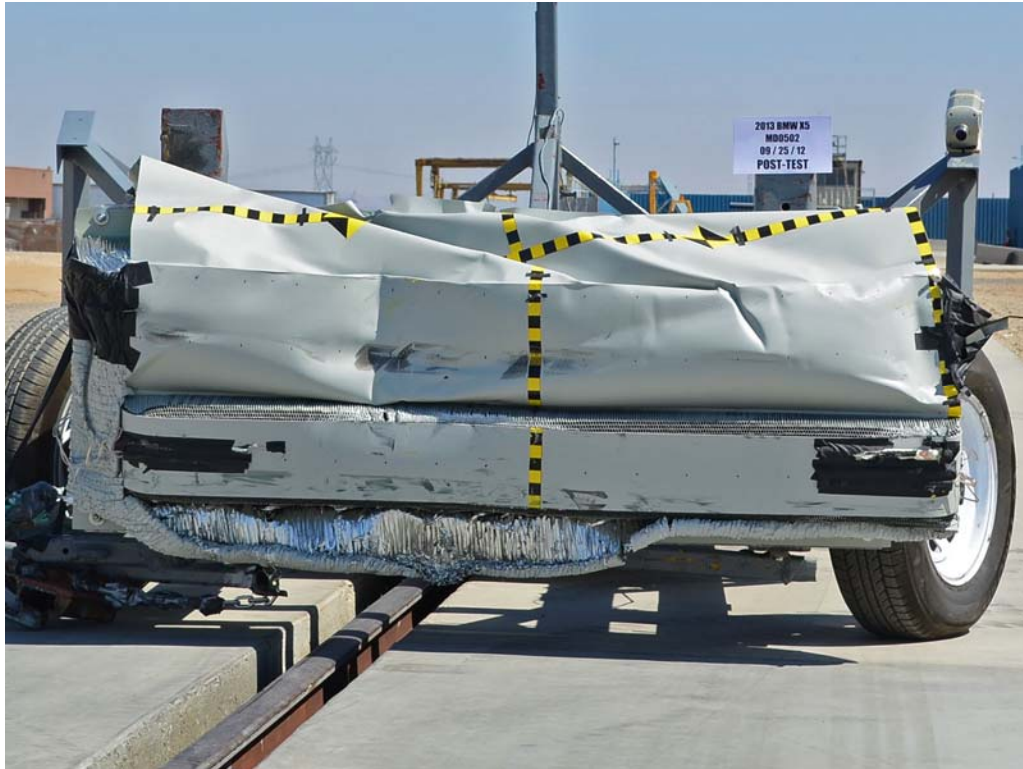
FIGURE 85. Post-Test Front View of MDB Impactor Face
