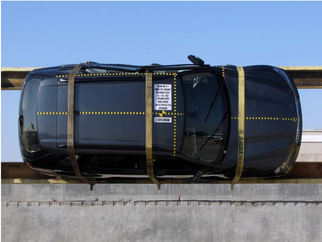
FIGURE 97. FMVSS No. 301 Static Rollover 90 Degrees
