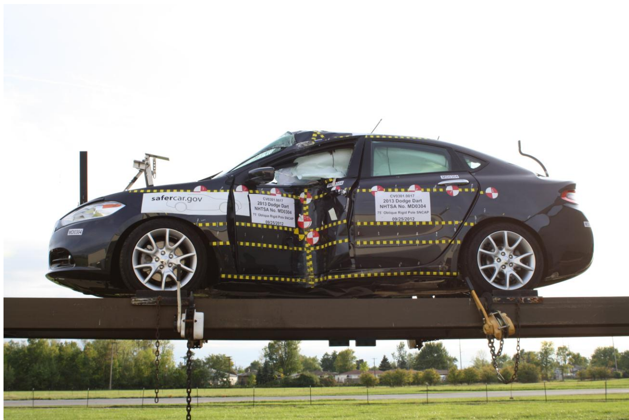
Figure A-63: FMVSS No. 301 Static Rollover 0 Degrees
