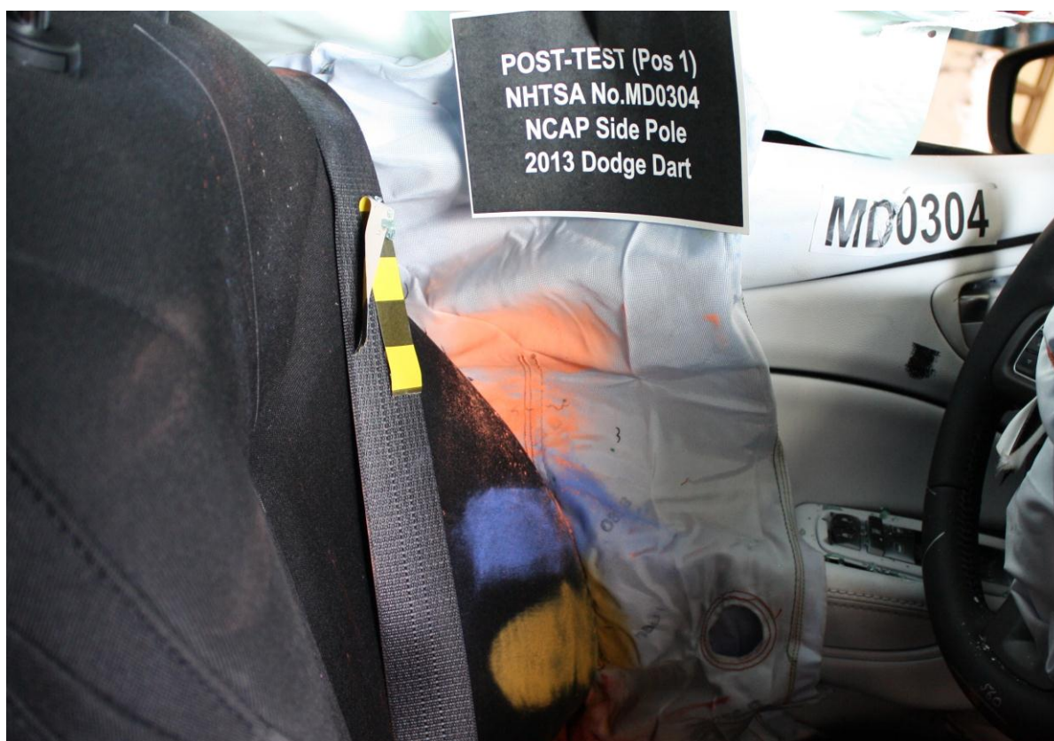
Figure A-48: Post-Test Dummy Close-Up Torso Contact with Vehicle Interior View
