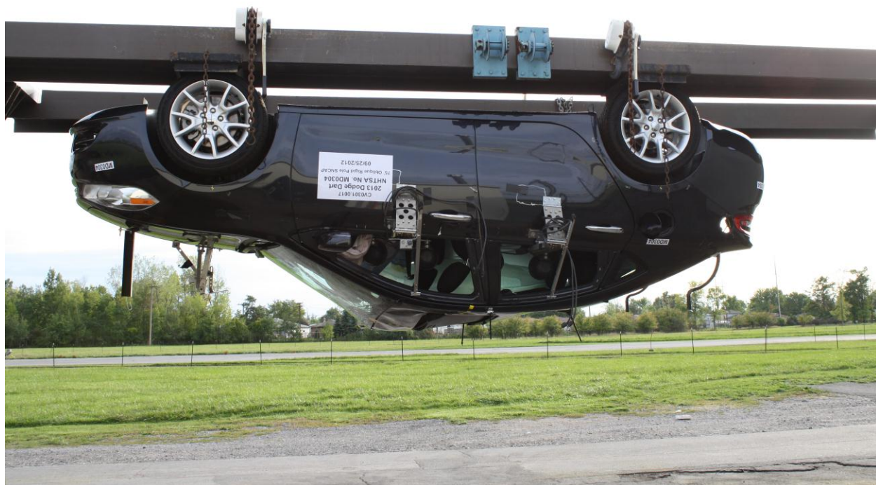
Figure A-65: FMVSS No. 301 Static Rollover 180 Degrees
