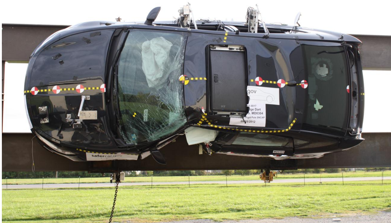
Figure A-66: FMVSS No. 301 Static Rollover 270 Degrees
