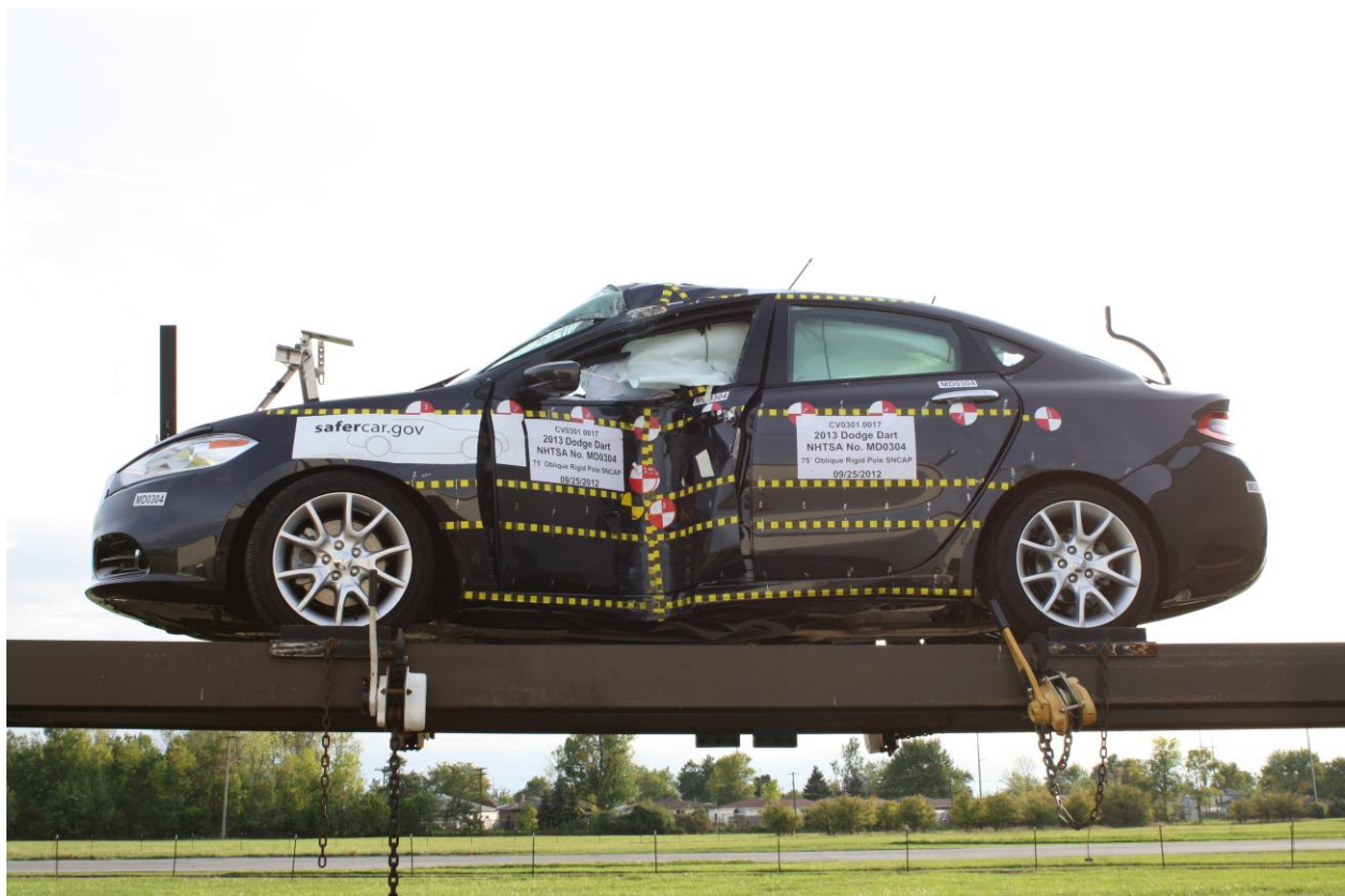
Figure A-67: FMVSS No. 301 Static Rollover 360 Degrees
