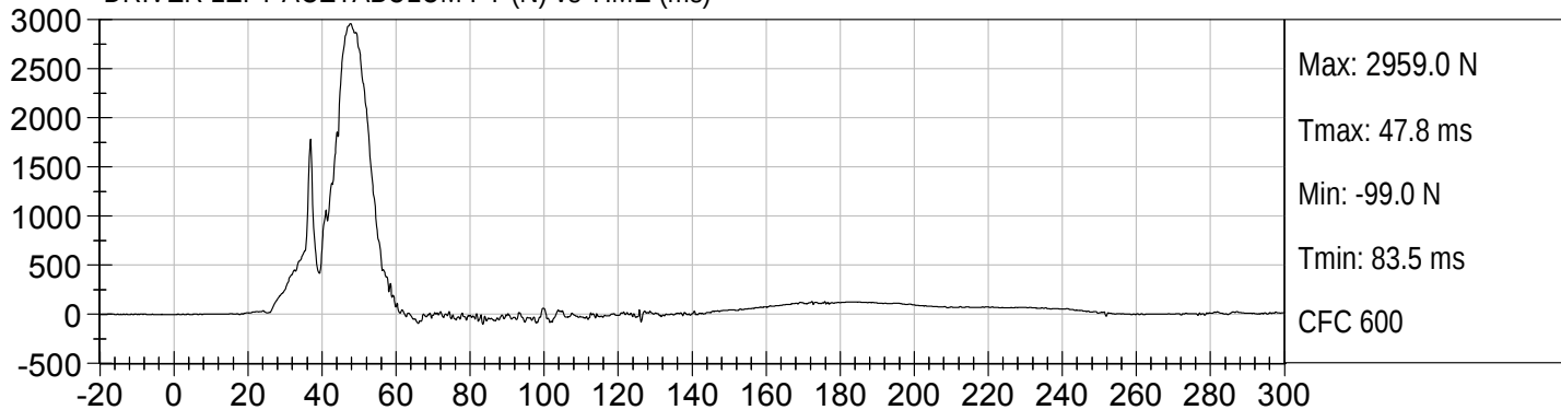
DRIVER LEFT LATERAL PELVIC FORCE (N) vs TIME (ms)
