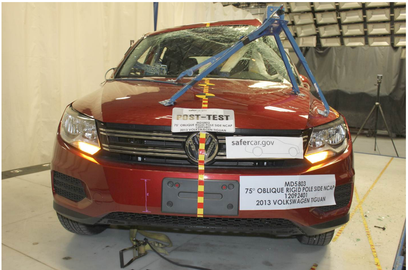
Post-Test Frontal View of Test Vehicle
