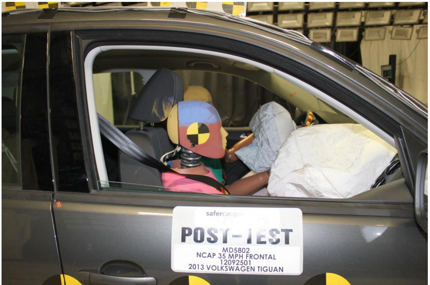
Post-Test Passenger Dummy Window View
