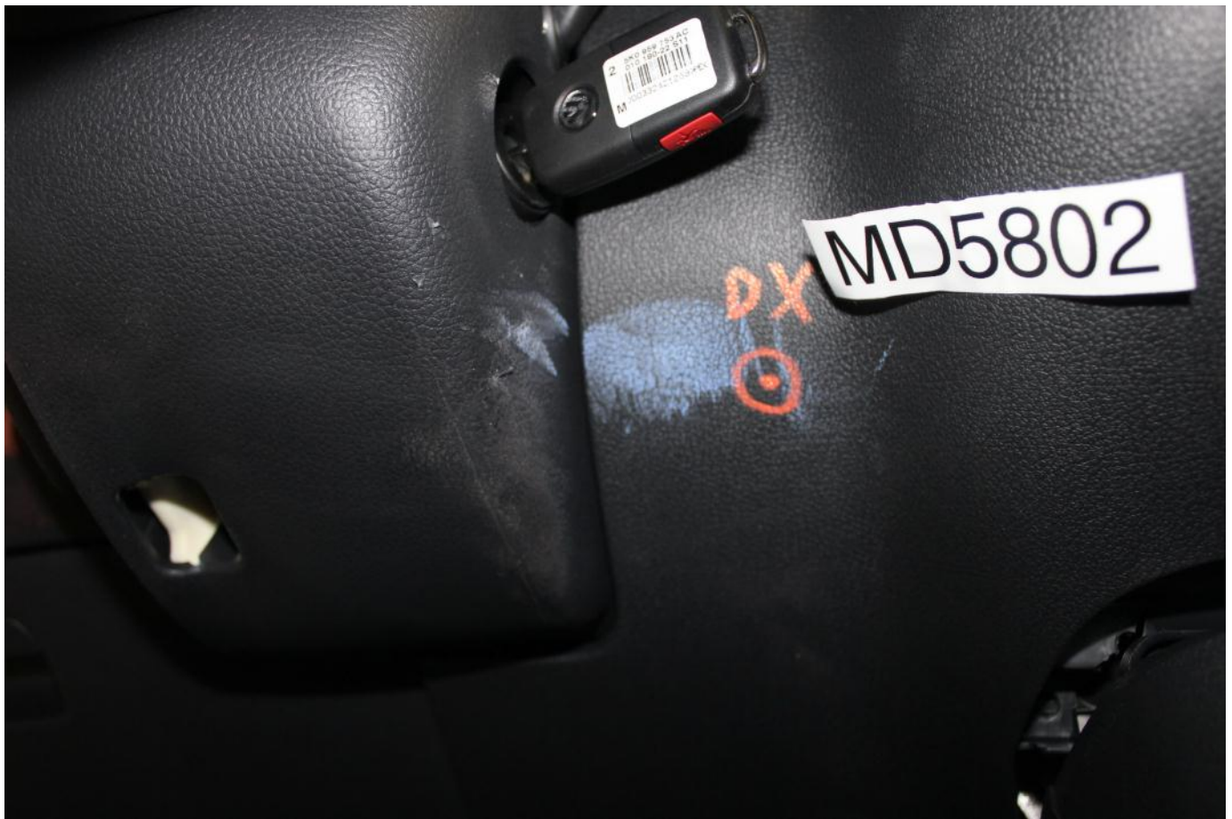
Post-Test Driver Dummy Contact with Steering Column
