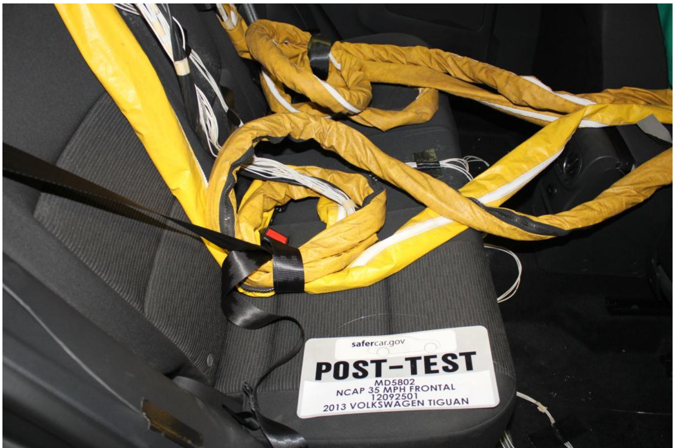
Post-Test Dummy Cable Routing
