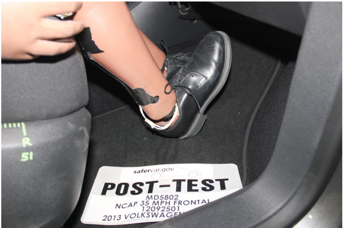
Post-Test Passenger Dummy Feet
