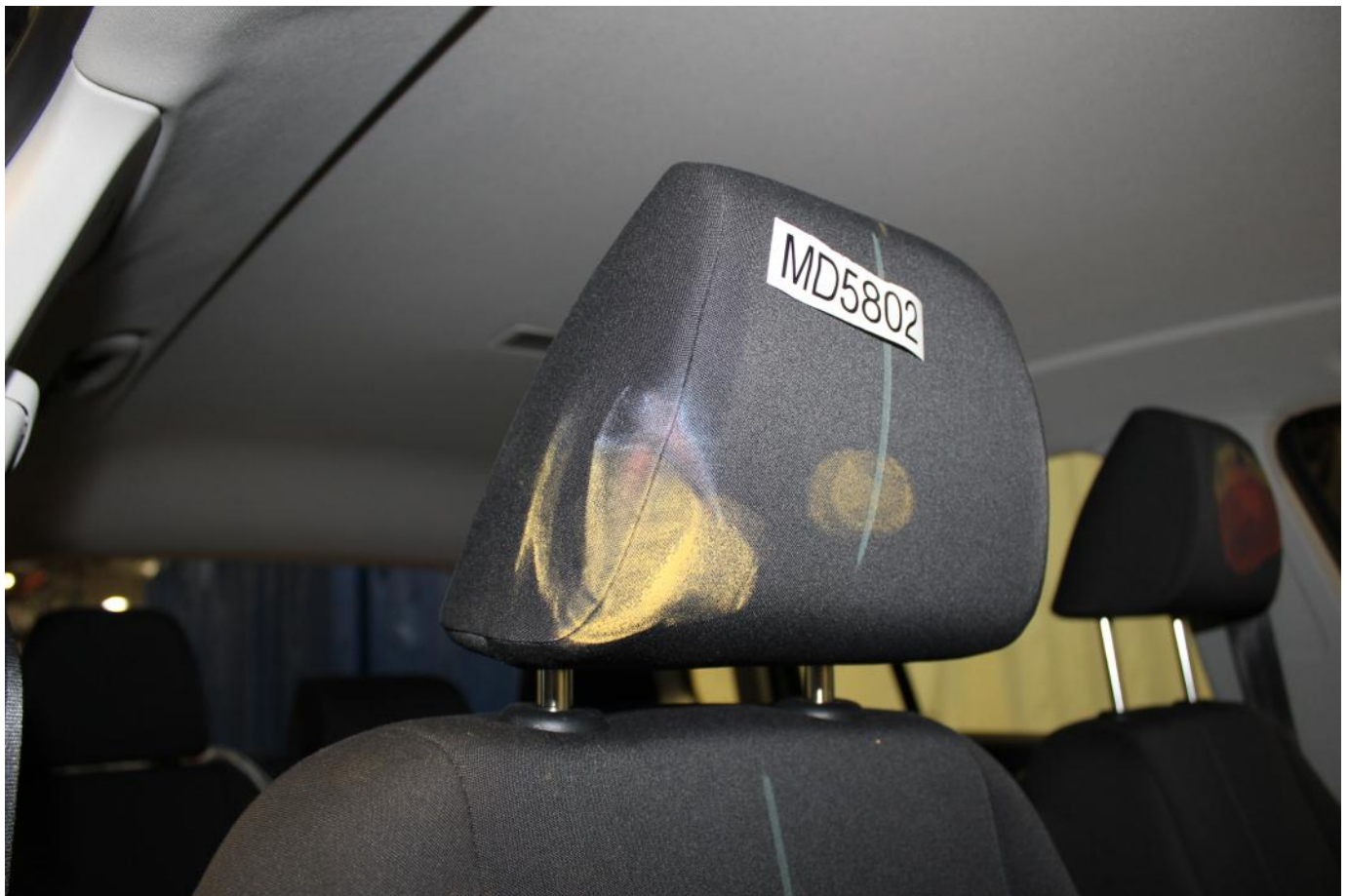
Post-Test Passenger Dummy Contact with Headrest
