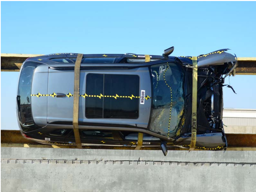
FIGURE 71. Vehicle at 90° on Static Rollover Device
