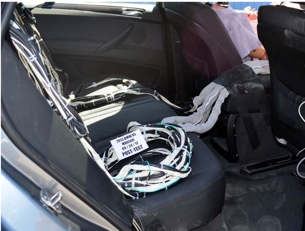
FIGURE 28. Post-Test Dummy Cable Routing
