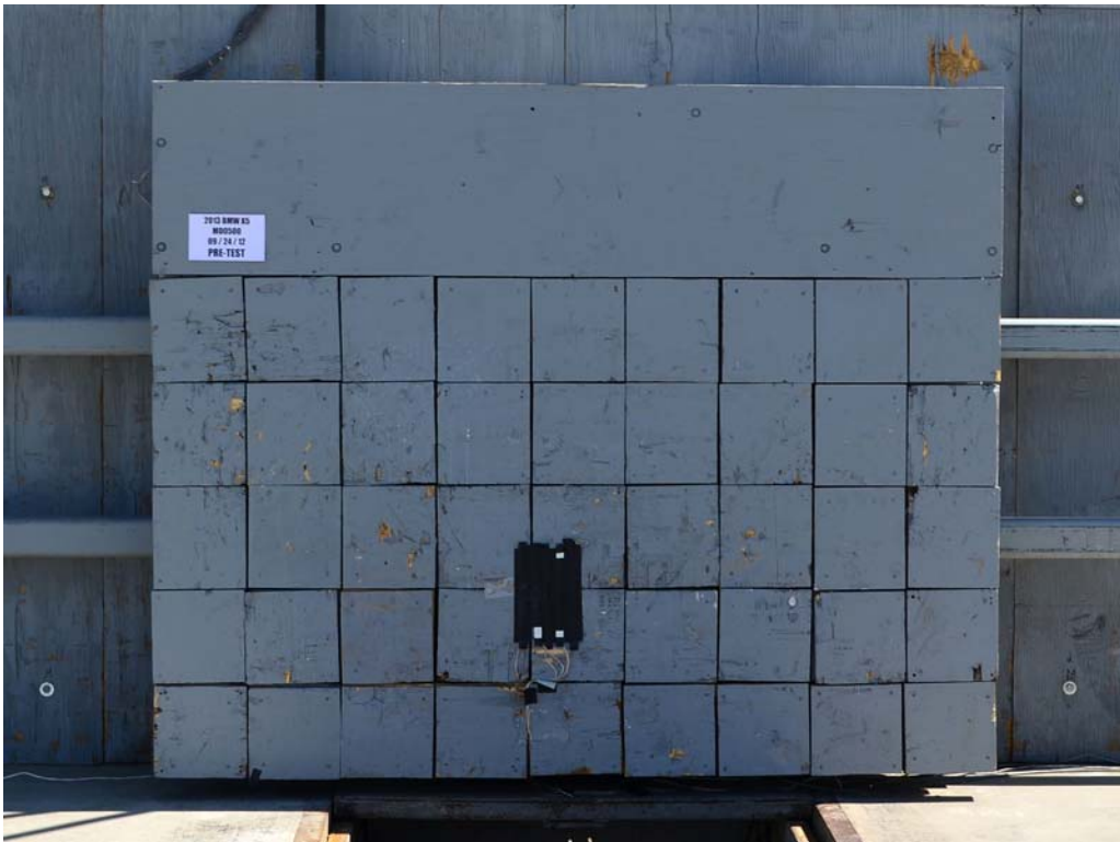
FIGURE 2. Load Cell Wall
