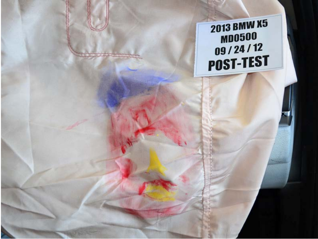
FIGURE 66. Post-Test Passenger Dummy Contact With Airbag
