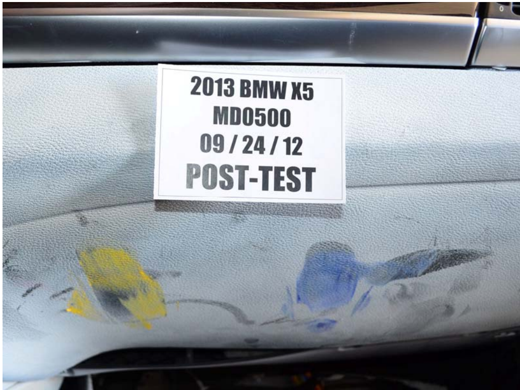
FIGURE 66c. Post-Test Passenger Dummy Contact With Knee Bolster
