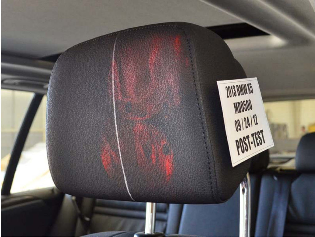
FIGURE 47. Post-Test Driver Dummy Contact With Headrest
