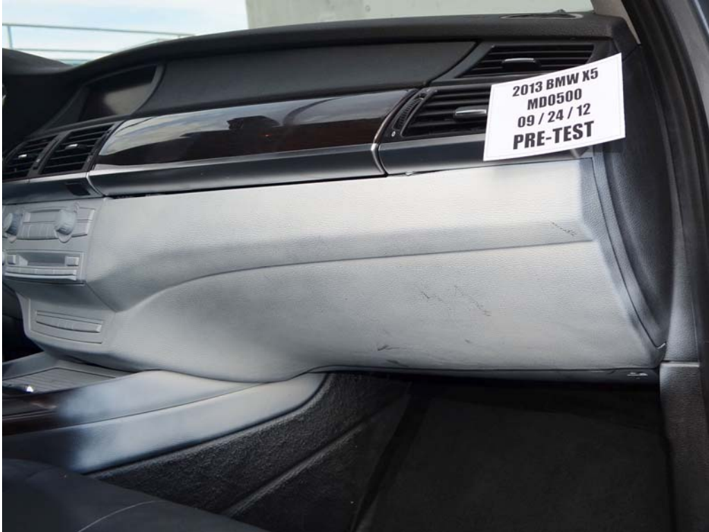
FIGURE 62. Pre-Test Passenger's Side Knee Bolster
