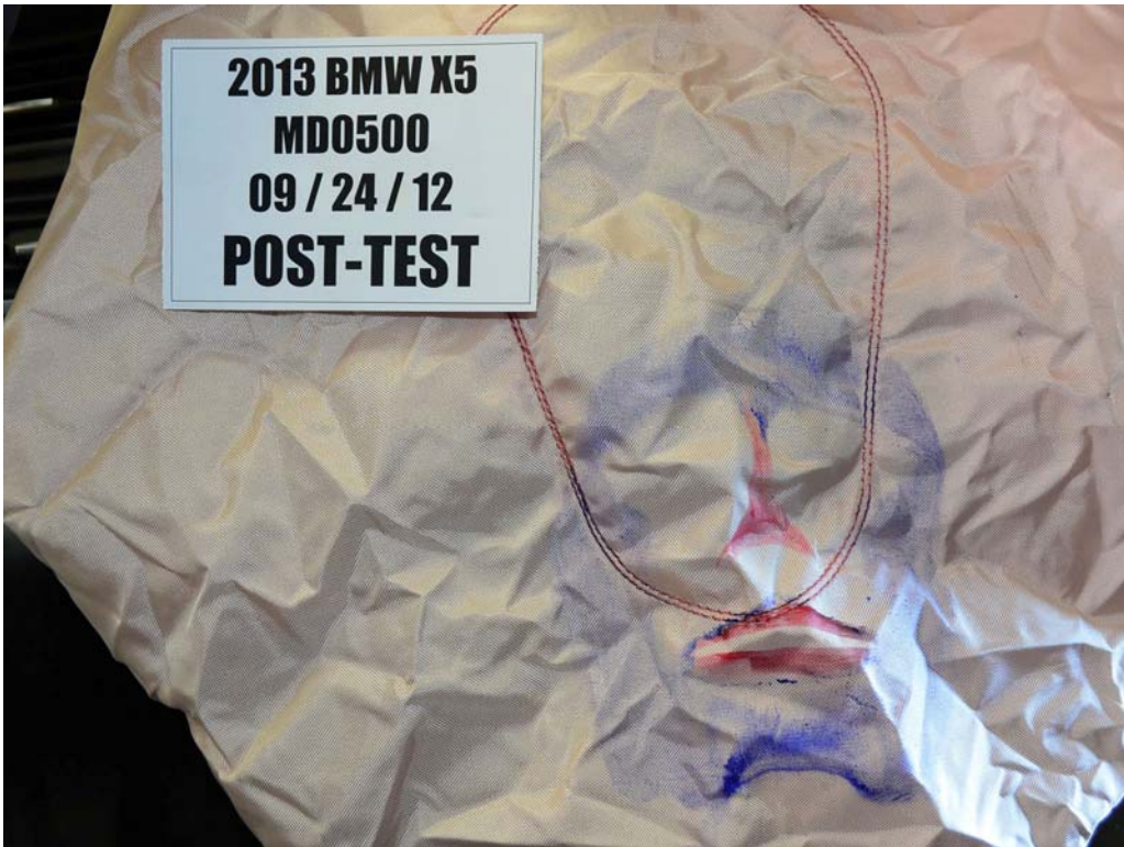
FIGURE 46. Post-Test Driver Dummy Contact With Airbag
