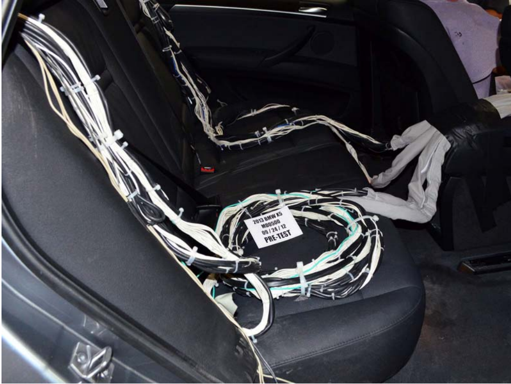
FIGURE 27. Pre-Test Dummy Cable Routing
