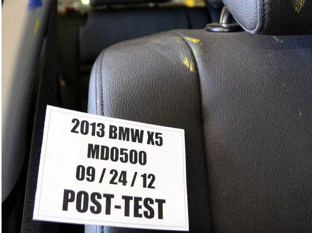
FIGURE 66b. Post-Test Passenger Dummy Contact With Seat Back
