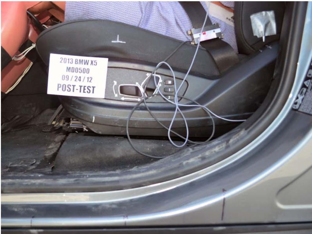
FIGURE 36. Post-Test Driver's Seat Fore-Aft Markings
