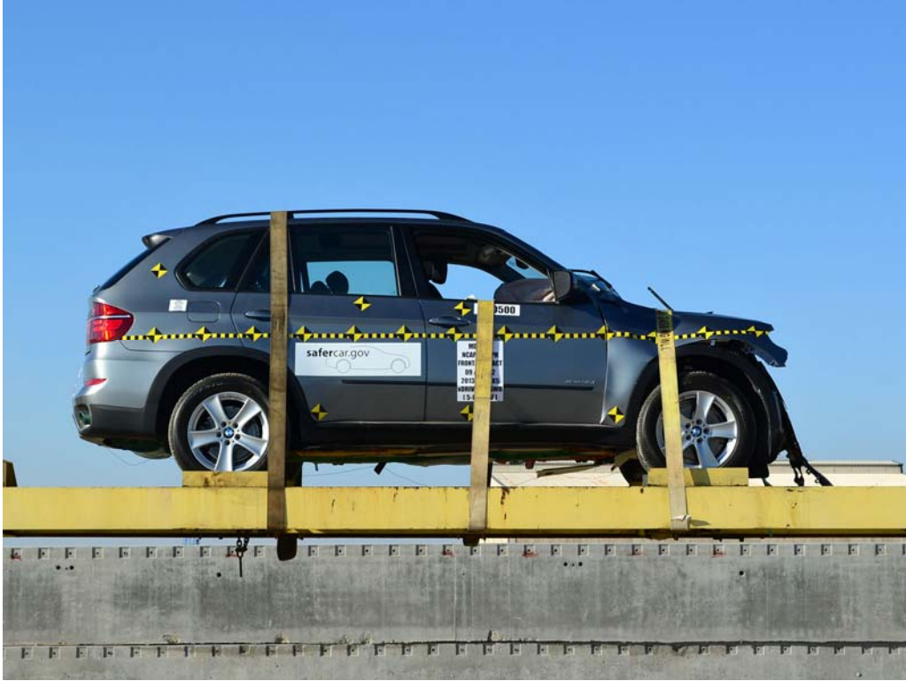
FIGURE 74. Vehicle at 360° on Static Rollover Device
