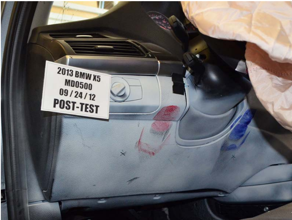
FIGURE 42. Post-Test Driver's Side Knee Bolster
