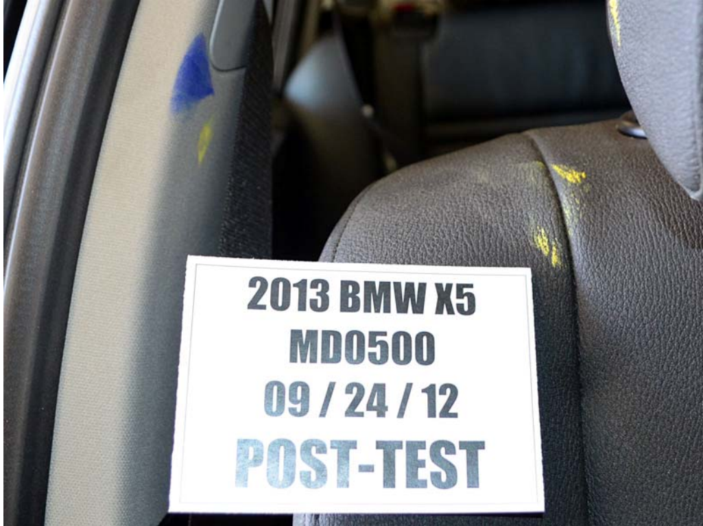
FIGURE 66d. Post-Test Passenger Dummy Contact With B-Pillar
