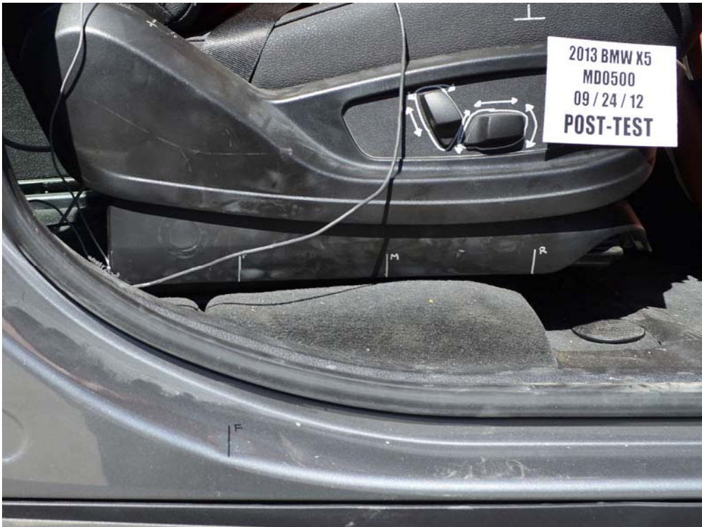
FIGURE 57. Post-Test Passenger's Seat Fore-Aft Markings
