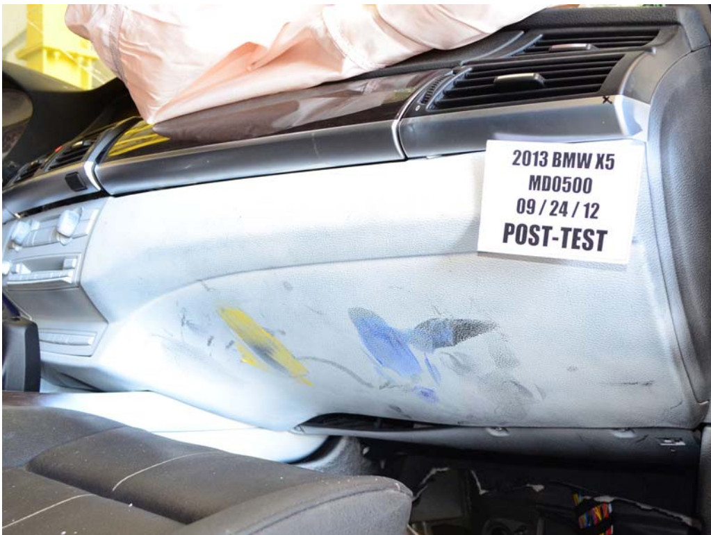
FIGURE 63. Post-Test Passenger's Side Knee Bolster
