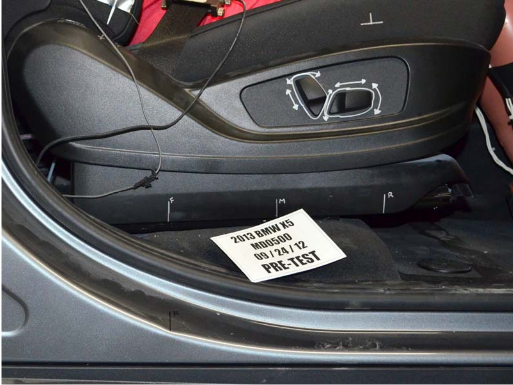
FIGURE 56. Pre-Test Passenger's Seat Fore-Aft Markings
