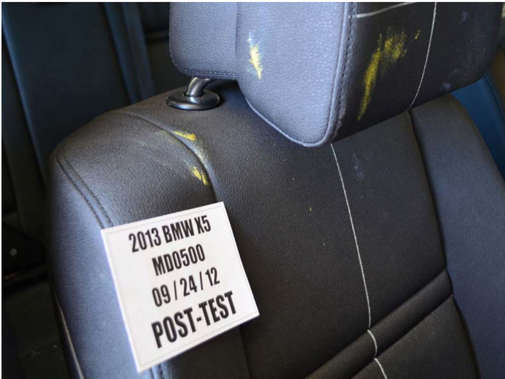
FIGURE 66a. Post-Test Passenger Dummy Contact With Headrest
