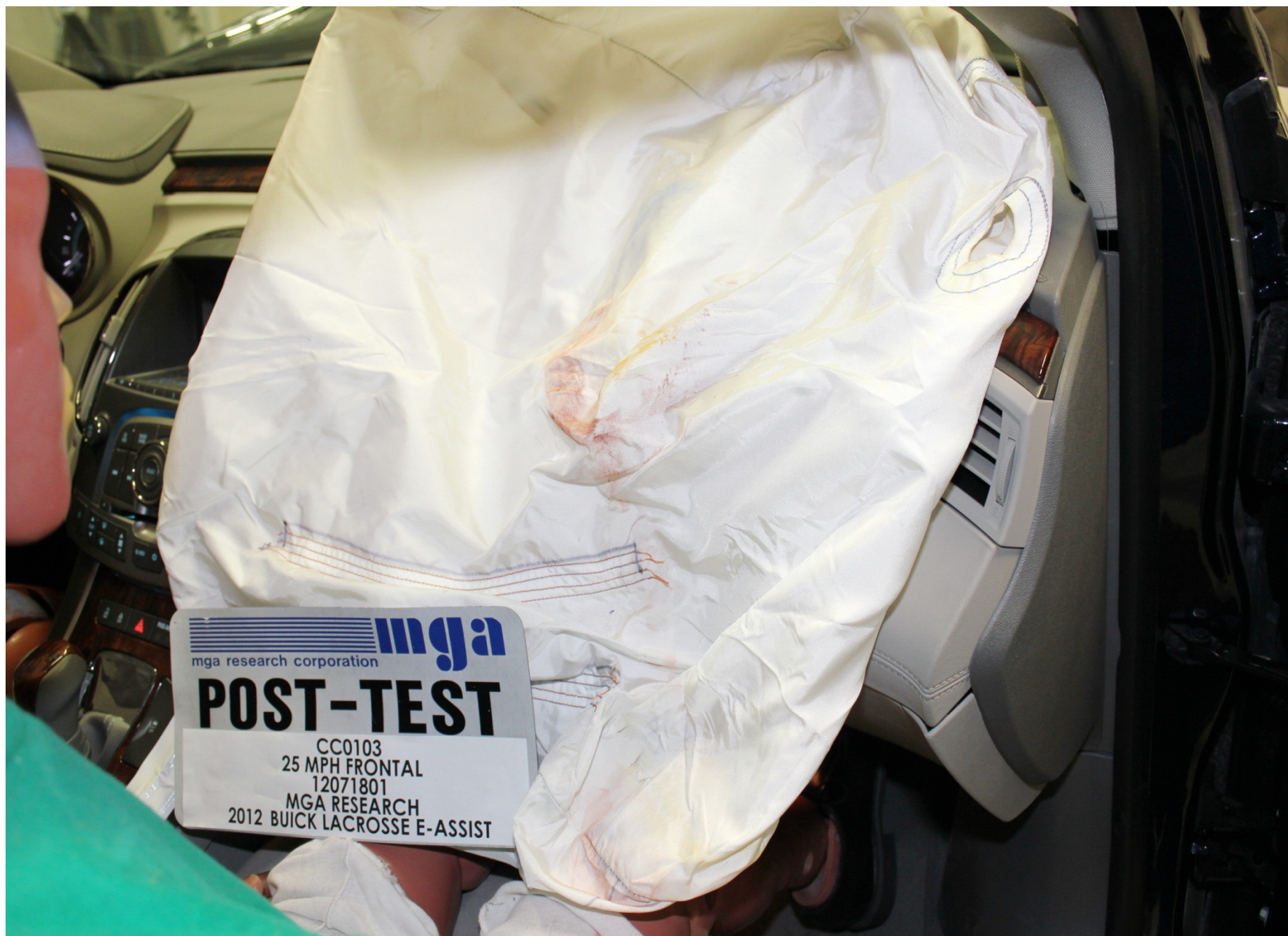
Post-Test Passenger Dummy Airbag Contact
