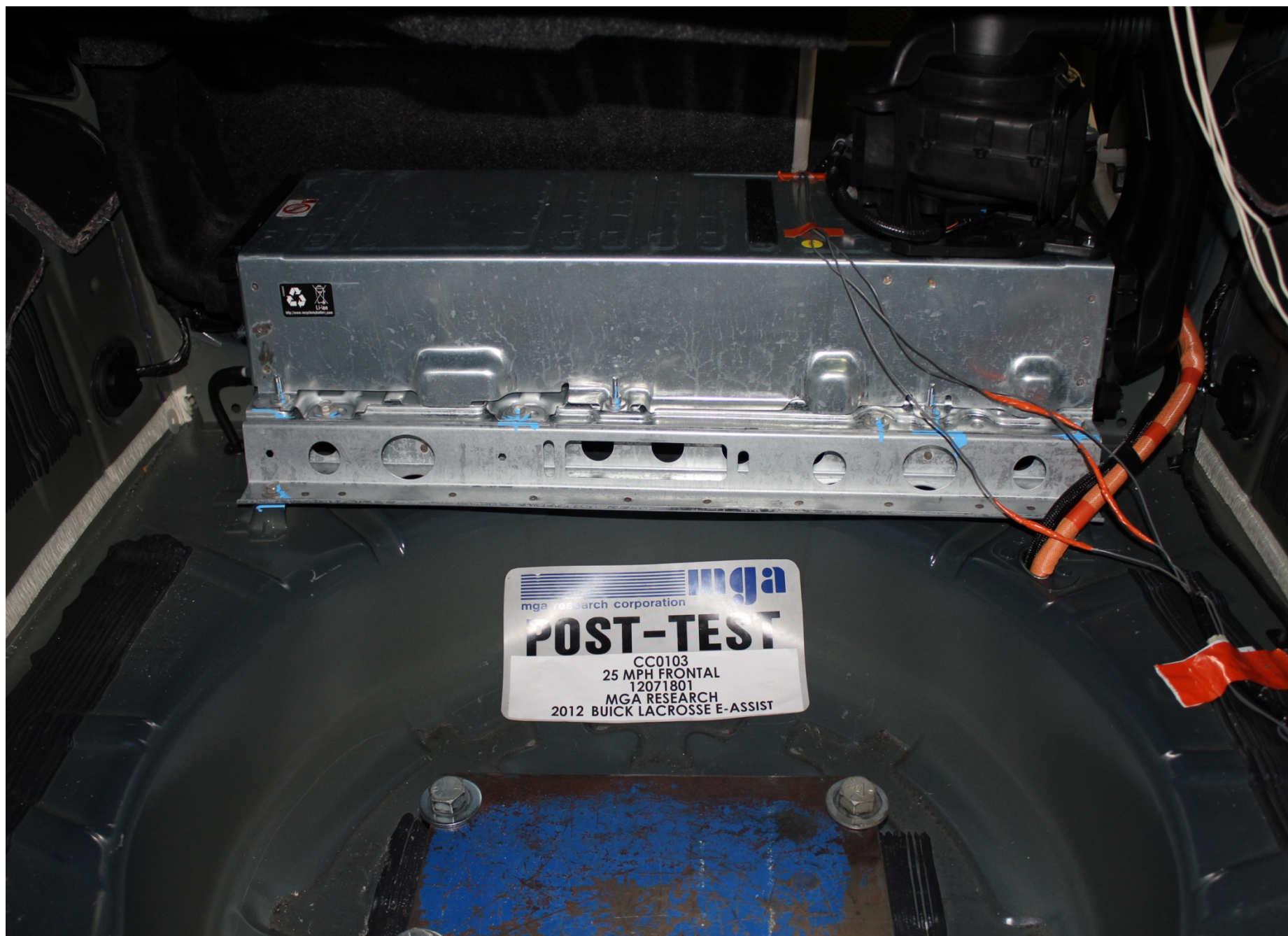
Post-Test Rear View of Electrical Propulsion Battery
