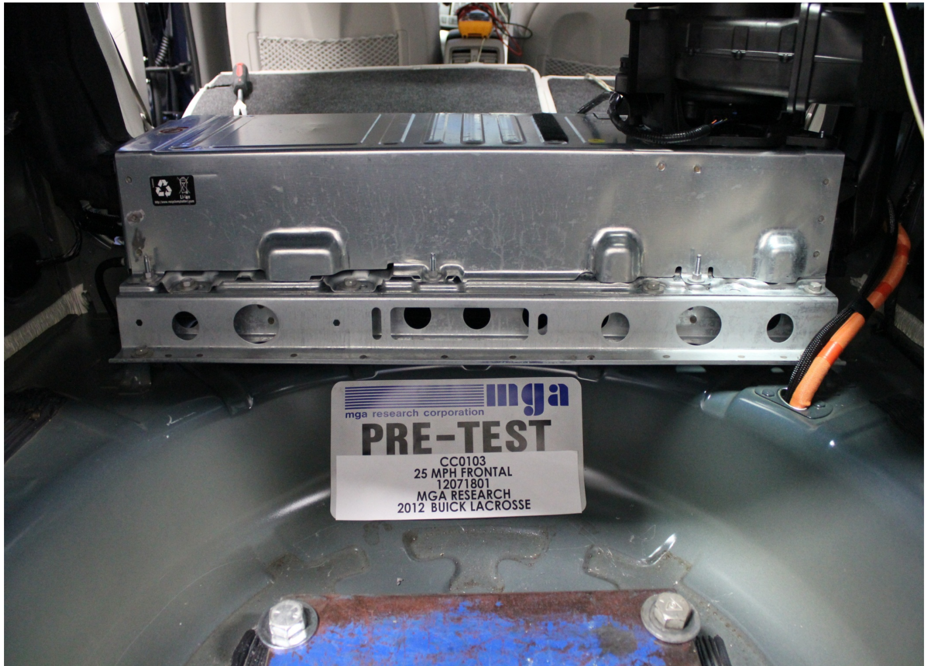
Pre-Test Rear View of Electrical Propulsion Battery
