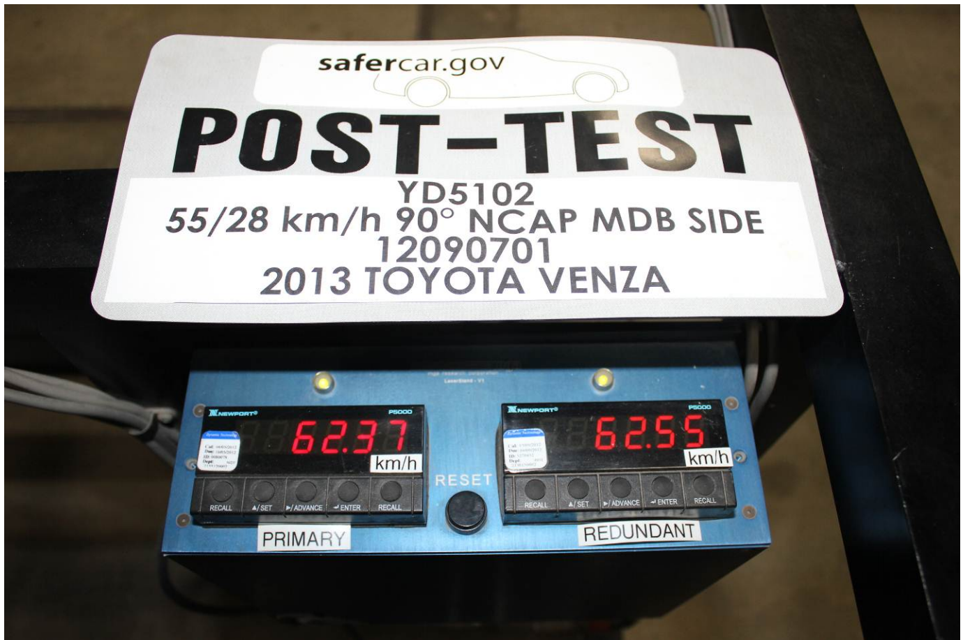
Post-Test Primary and Redundant Speed Trap Read-Out
