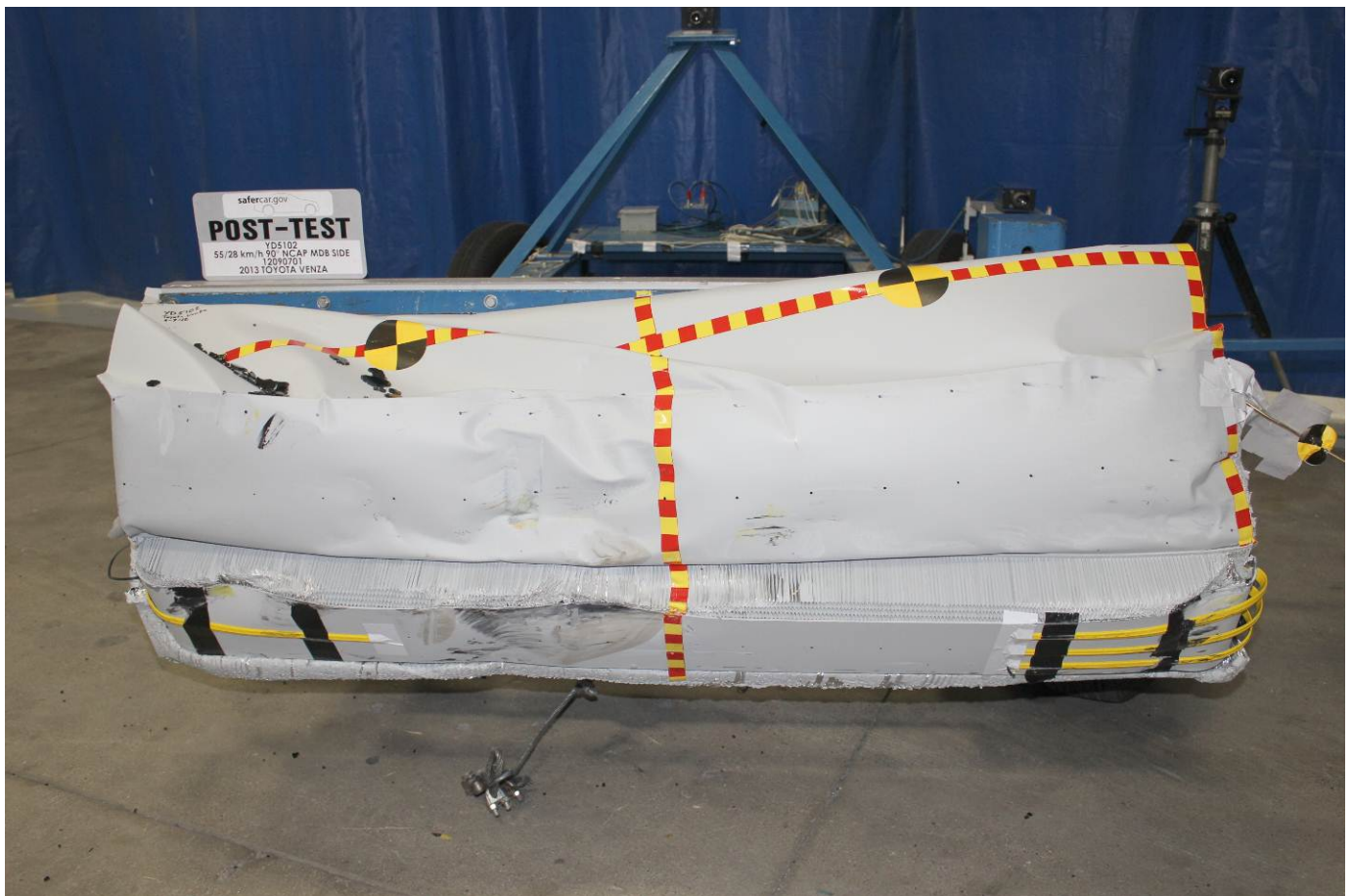
Post-Test Front View of MDB Impactor Face
