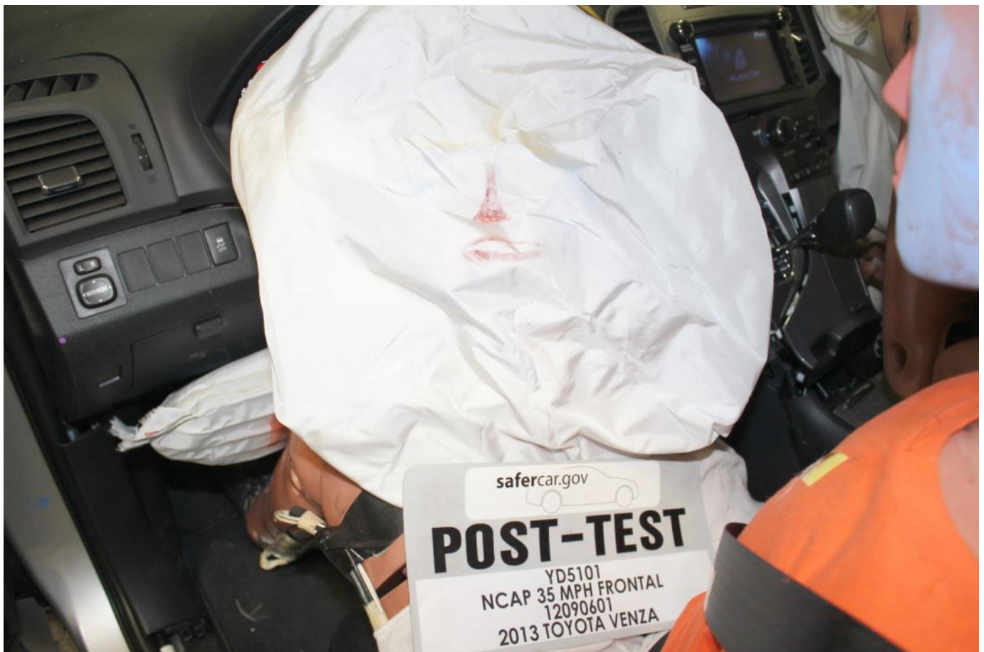
Post-Test Driver Dummy Contact with Airbag
