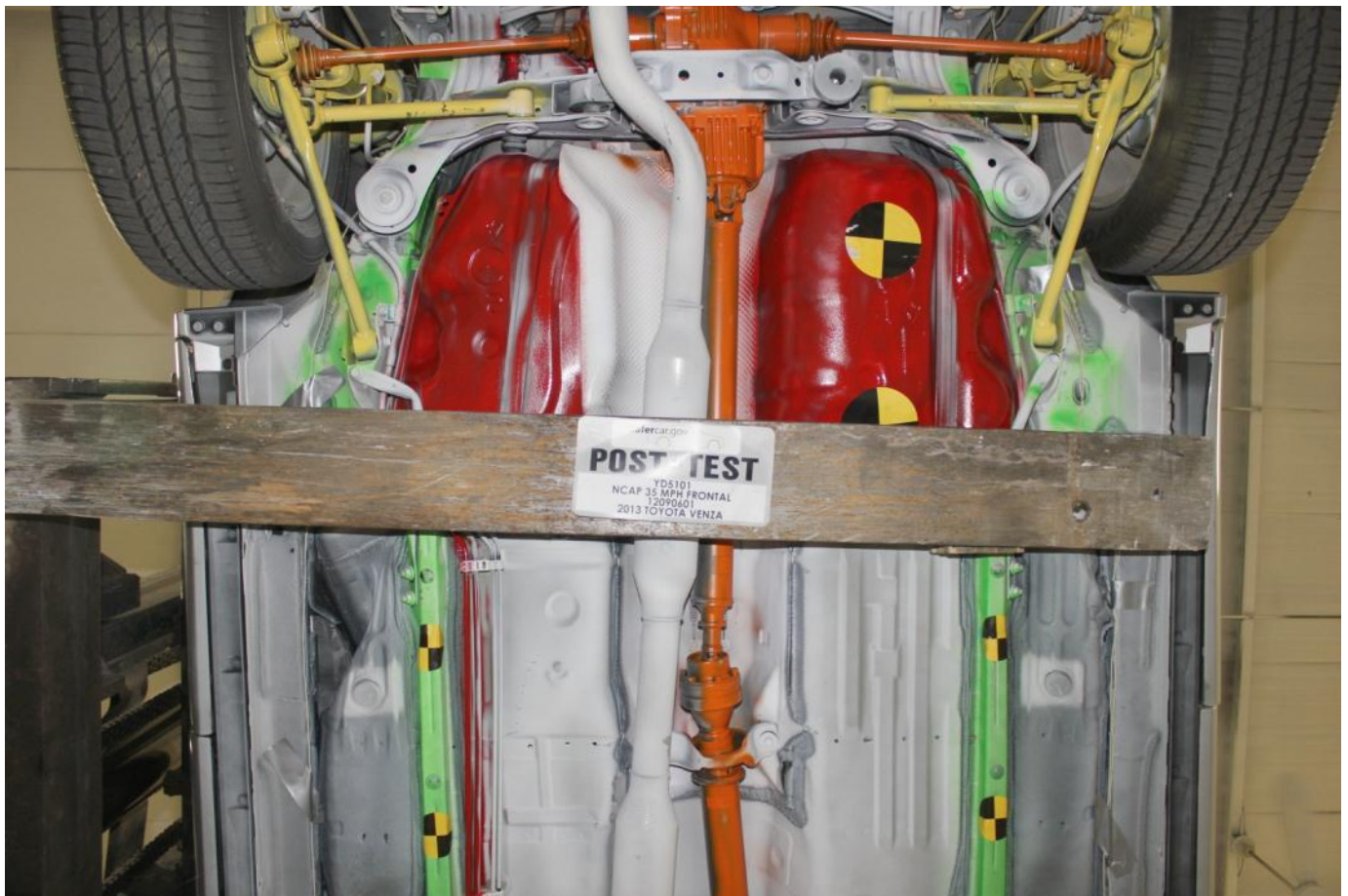
Post-Test Mid Rear Underbody View
