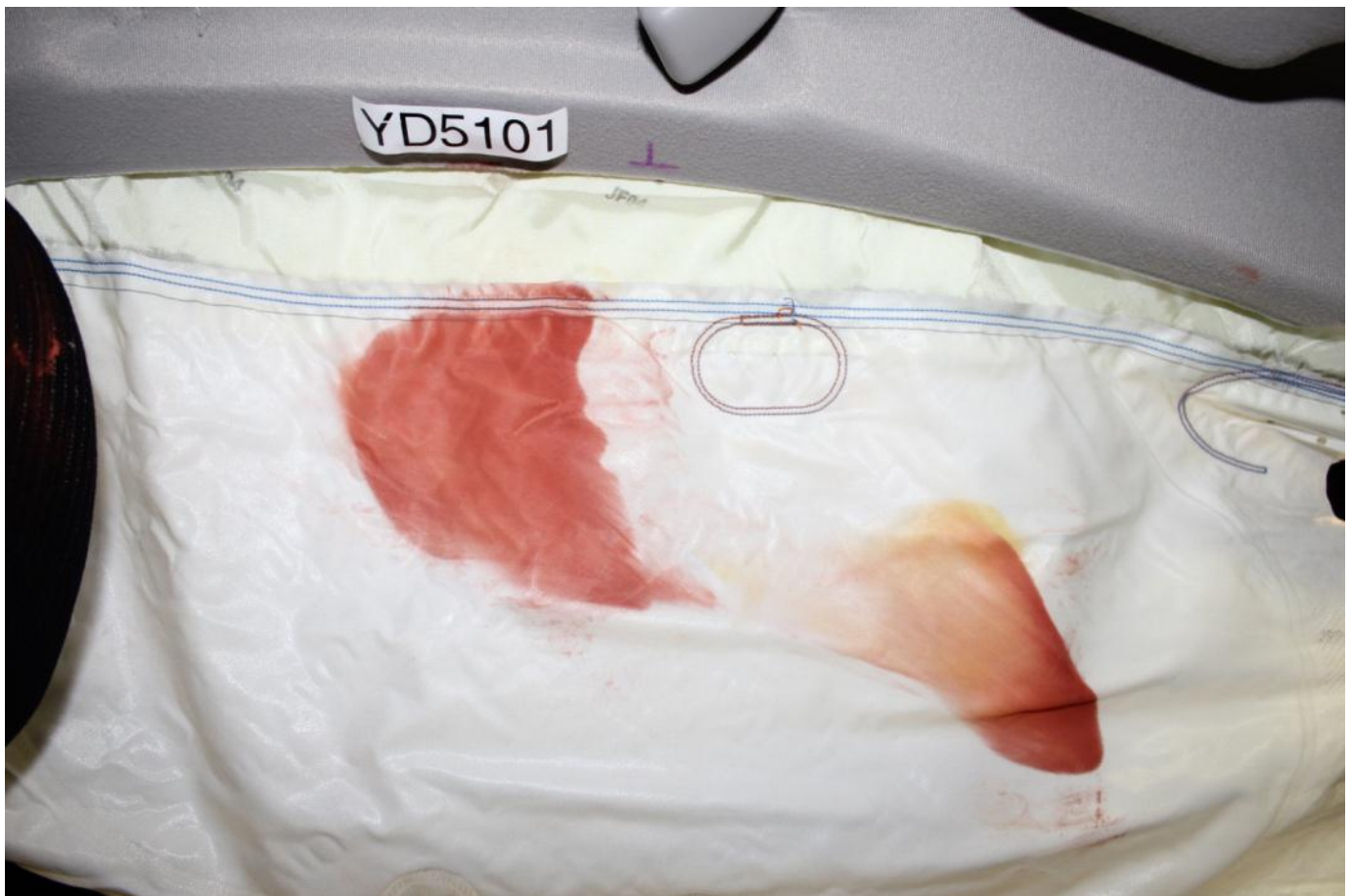
Post-Test Driver Dummy Contact with Curtain Airbag
