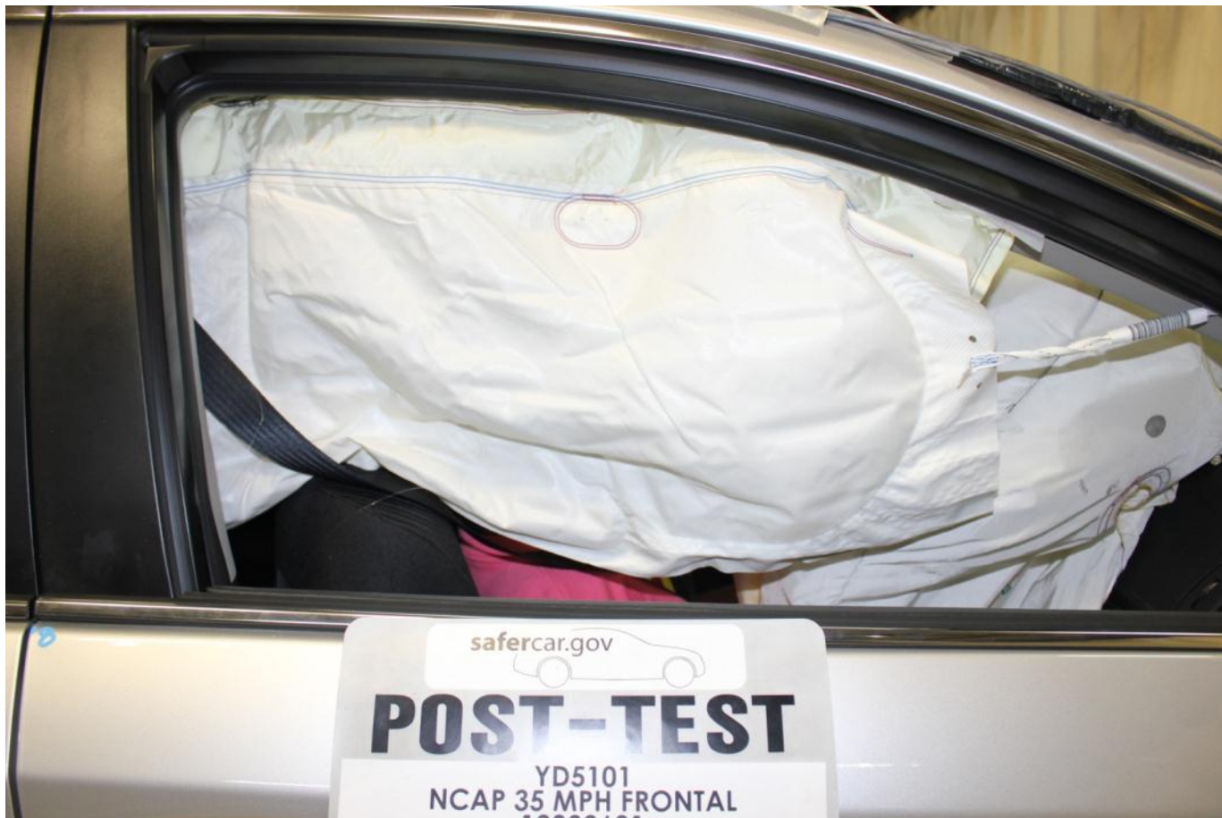
Post-Test Passenger Dummy Window View
