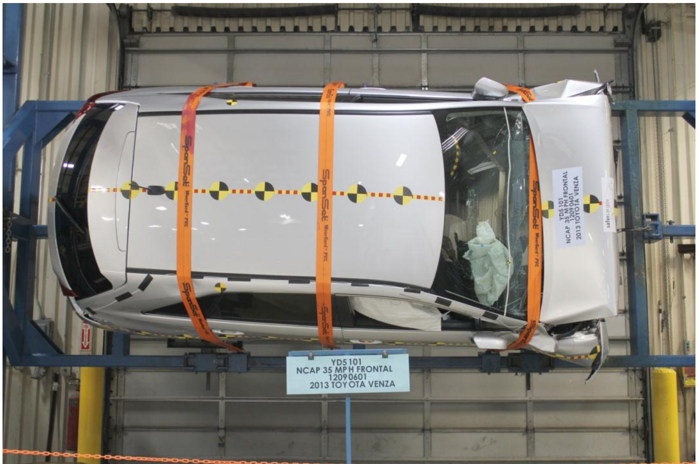
Vehicle at 270° on Static Rollover Device
