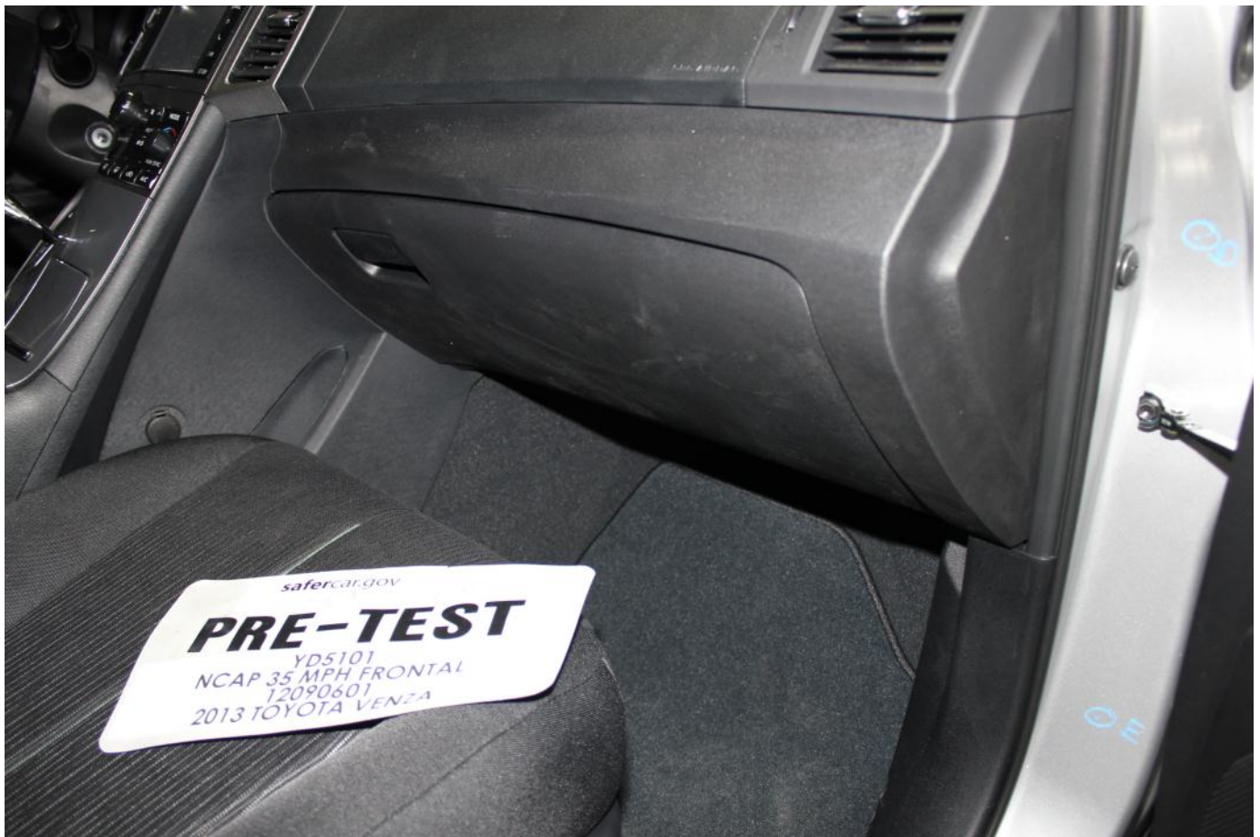
Pre-Test Passenger's Side Knee Bolster (without dummy)
