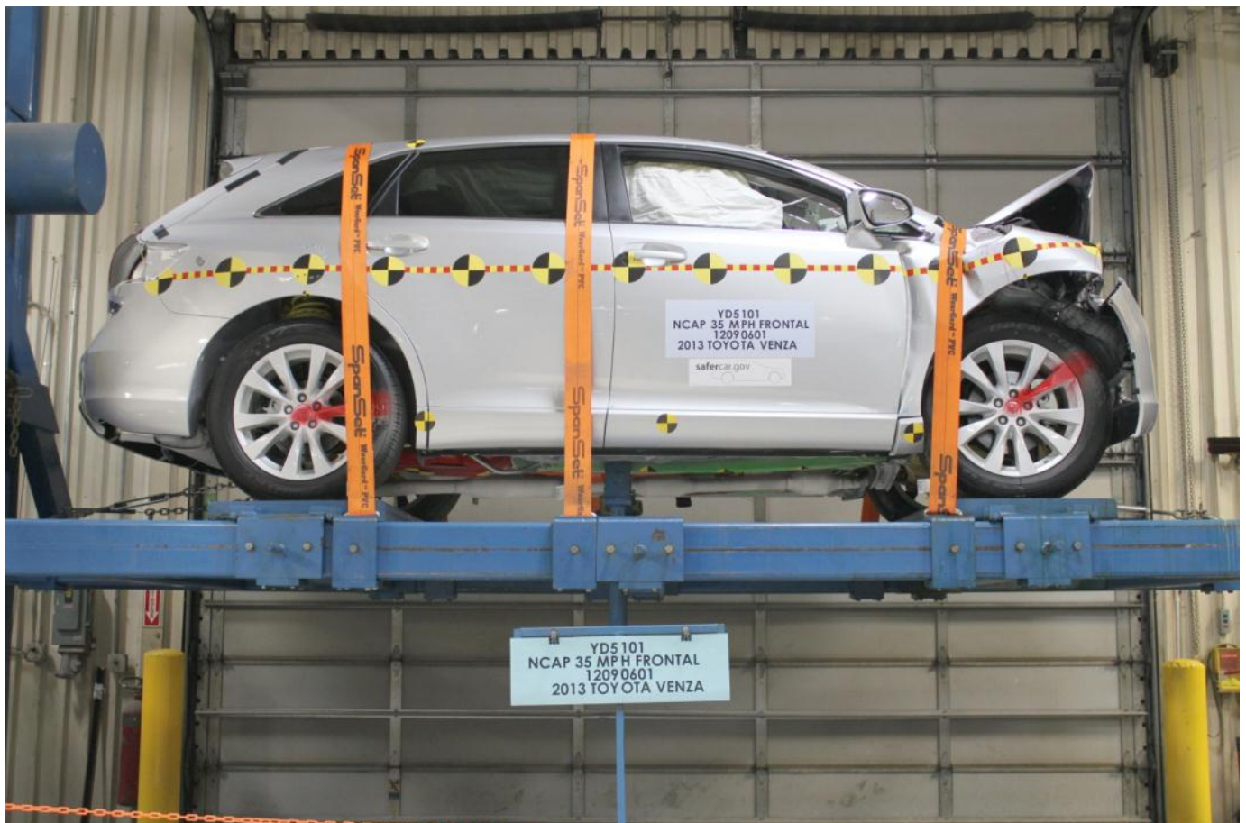
Vehicle at 360° on Static Rollover Device
