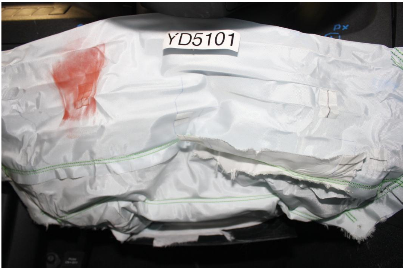
Post-Test Driver Dummy Contact with Knee Airbag
