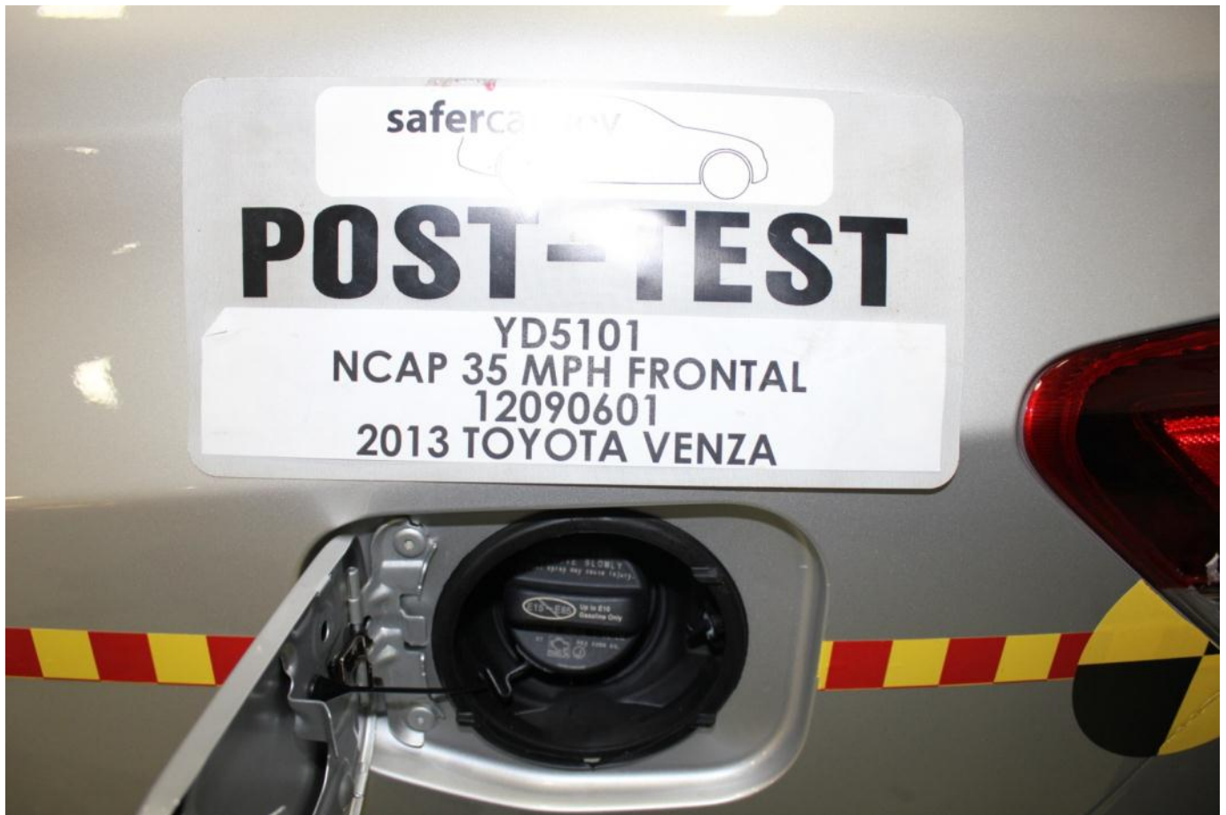
Post-Test Fuel Filler Cap View
