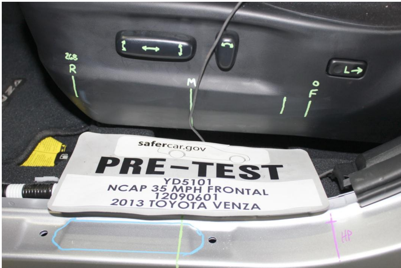
Pre-Test Driver's Seat Fore-Aft Markings
