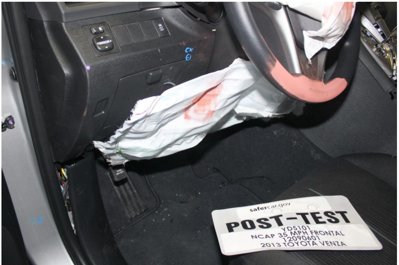
Post-Test Driver Dummy Contact with Steering Column
