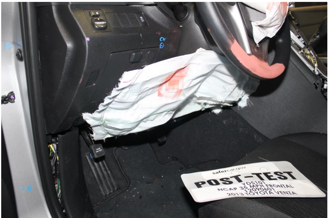
Post-Test Driver's Side Knee Bolster (without dummy)
