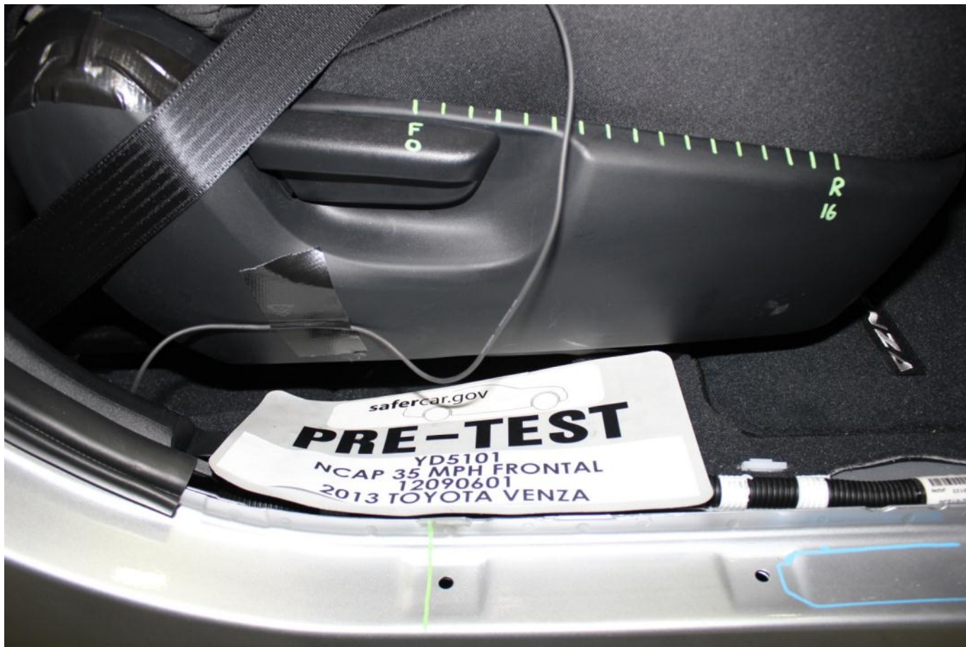
Pre-Test Passenger's Seat Fore-Aft Markings
