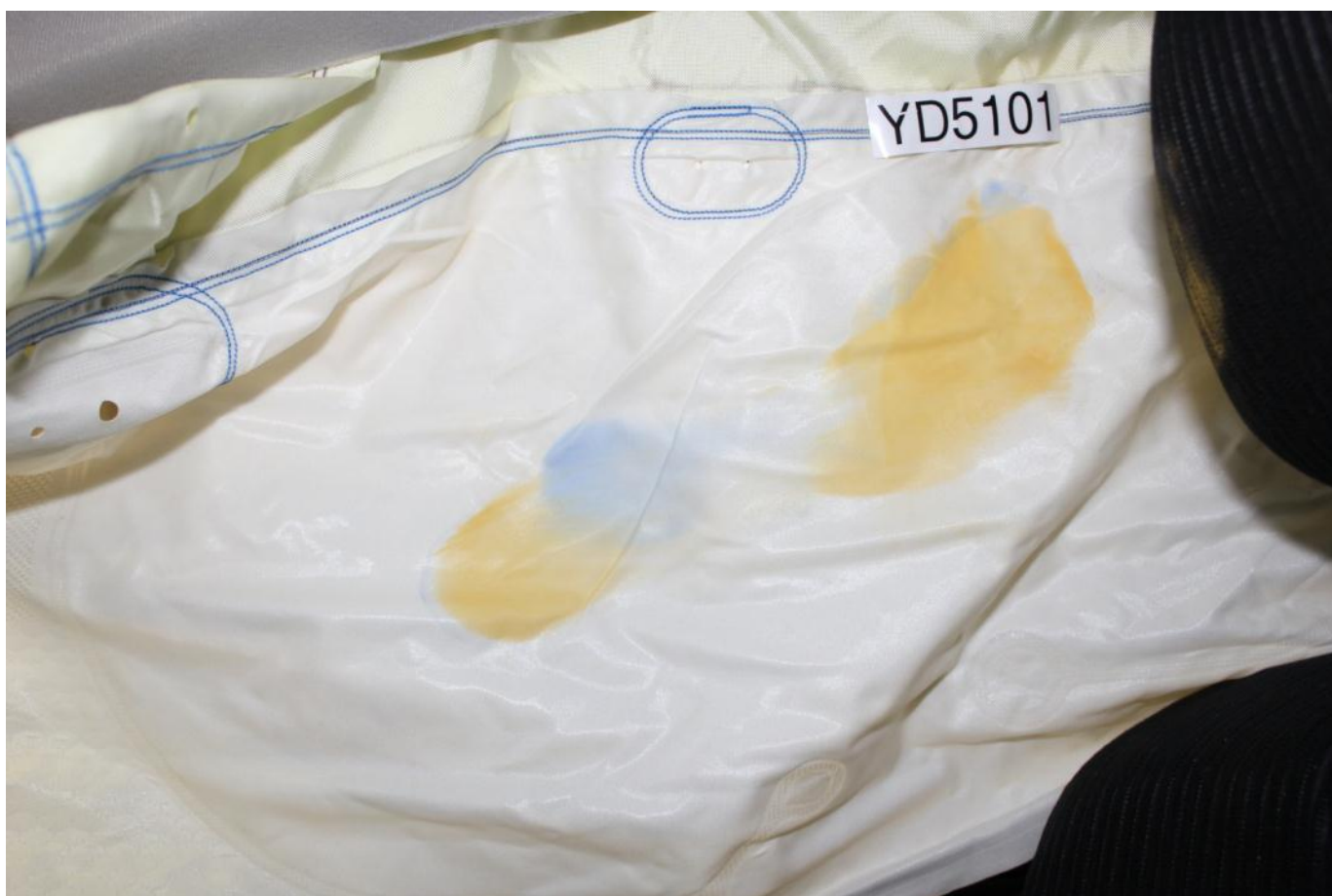
Post-Test Passenger Dummy Contact with Curtain Airbag
