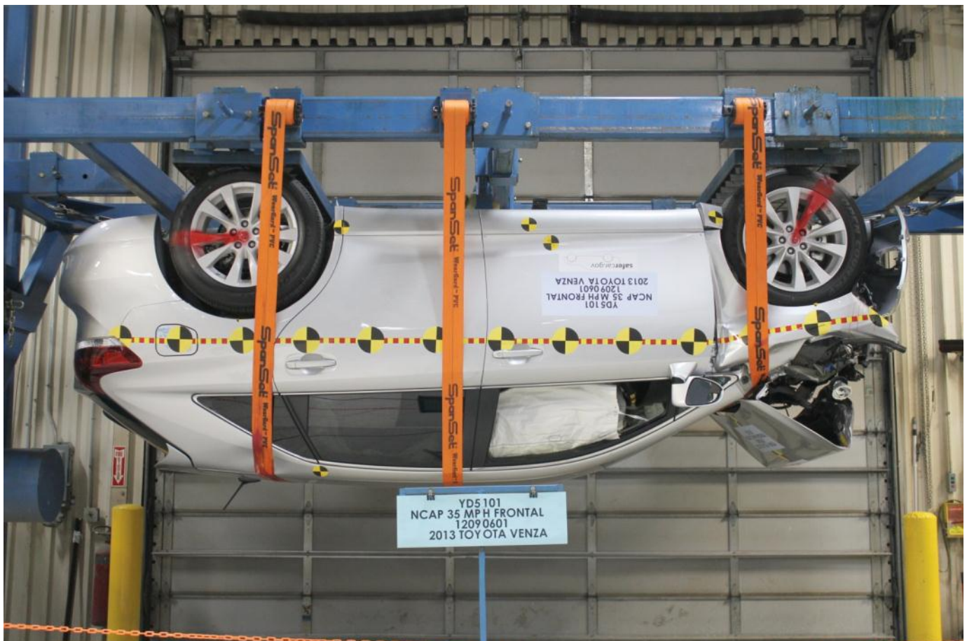
Vehicle at 180° on Static Rollover Device
