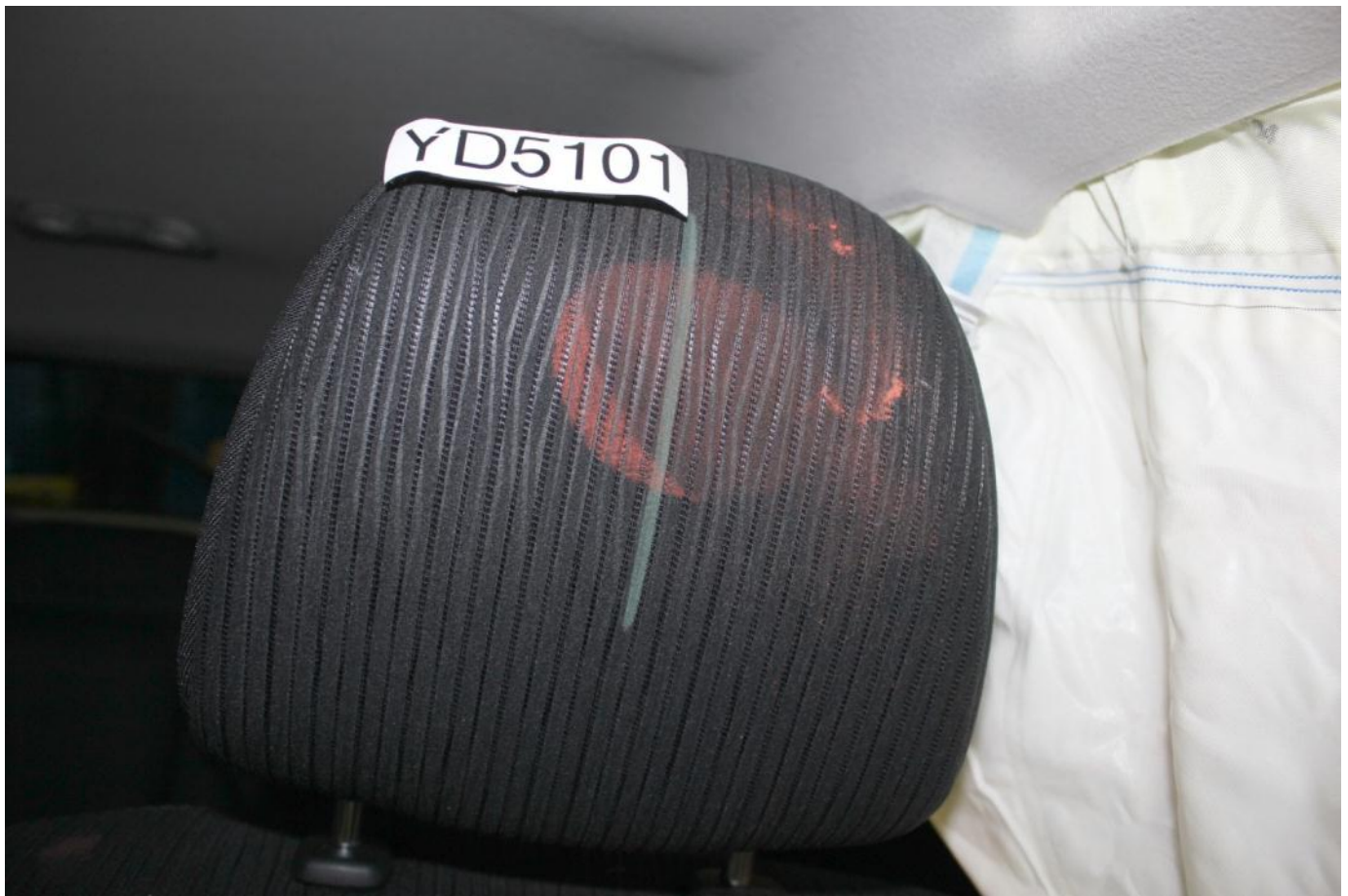
Post-Test Driver Dummy Contact with Headrest
