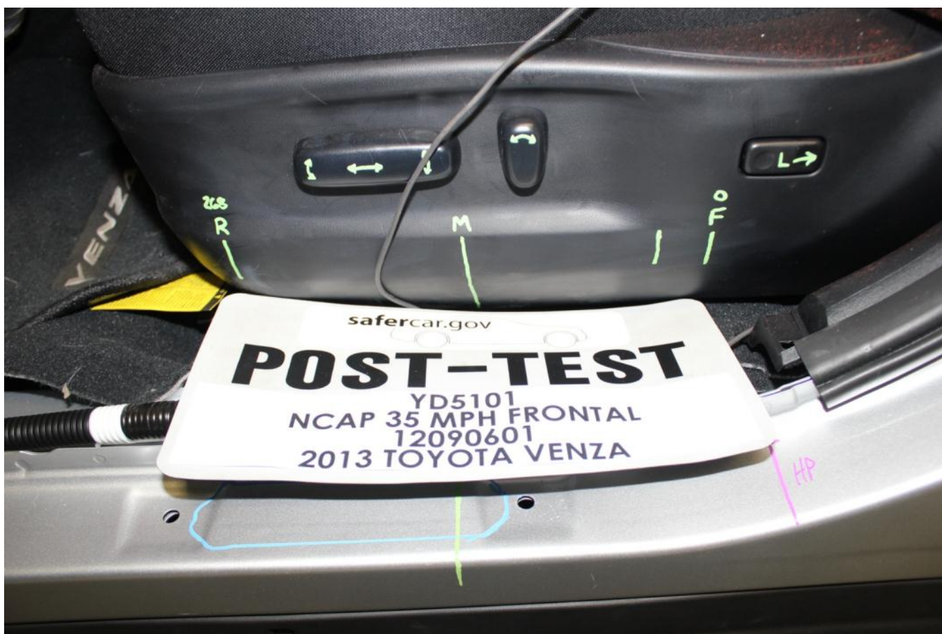
Post-Test Driver's Seat Fore-Aft Markings
