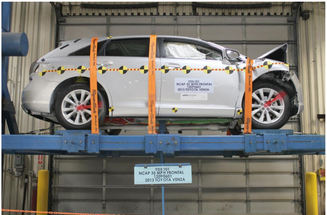
Vehicle at 0° on Static Rollover Device
