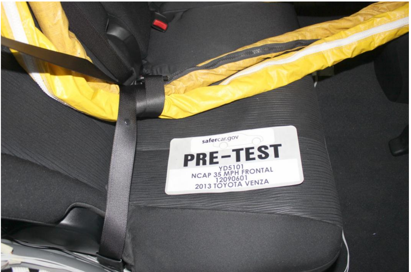
Pre-Test Dummy Cable Routing
