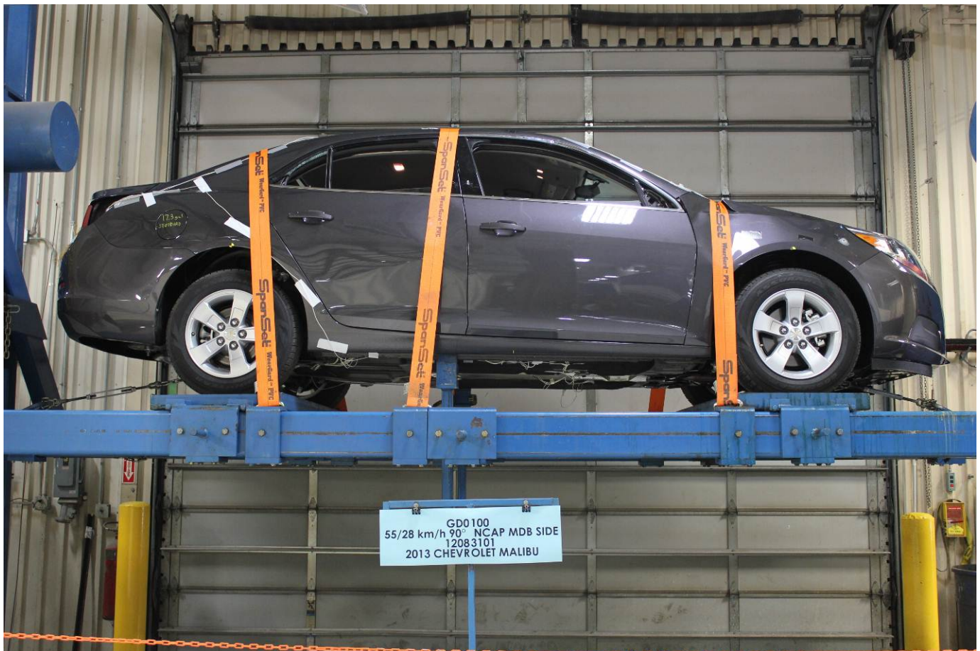
FMVSS No. 301 Static Rollover 360 Degrees
