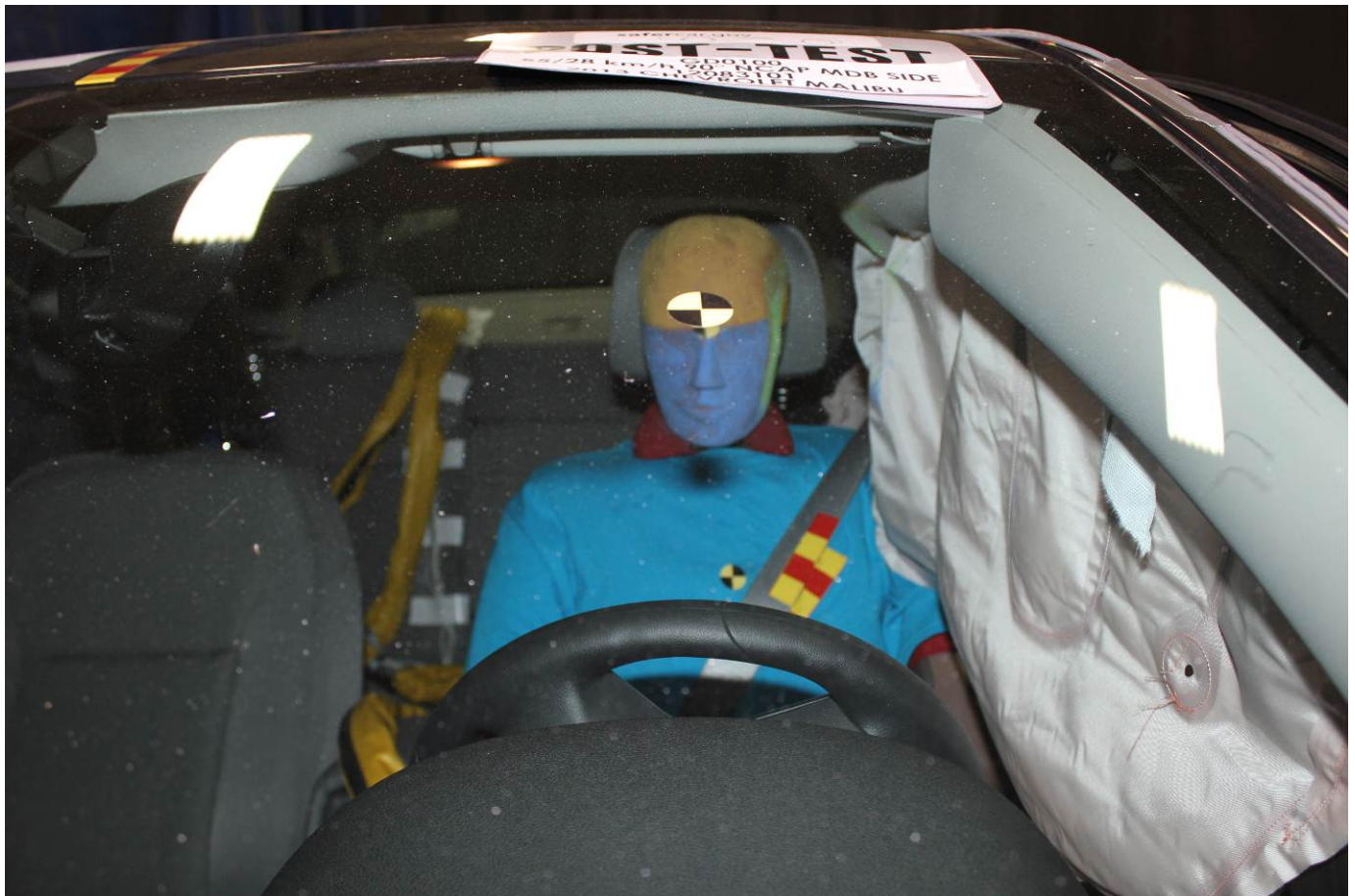
Post-Test Front Close-Up View of Driver Dummy
