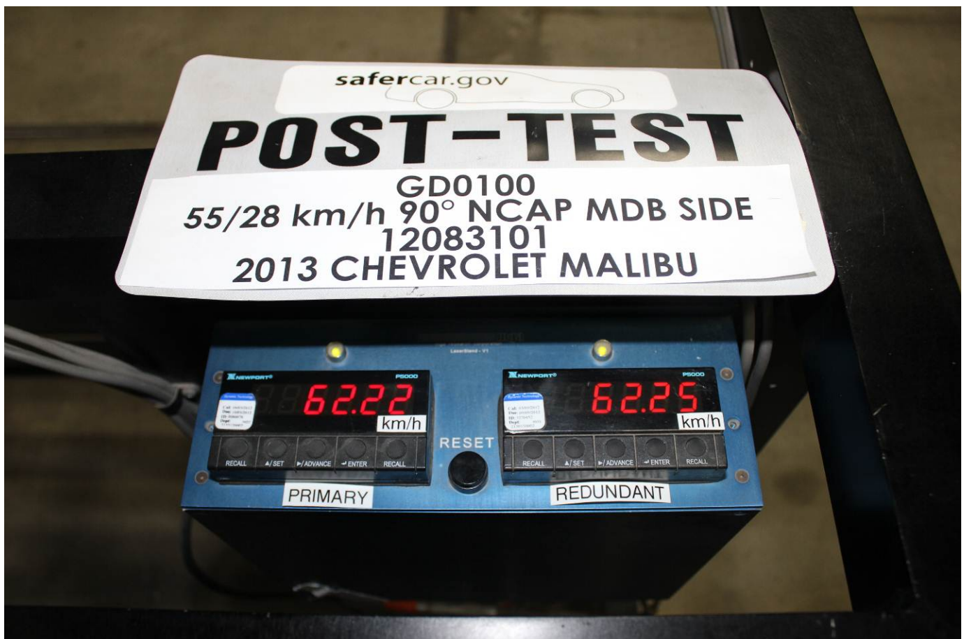
Post-Test Primary and Redundant Speed Trap Read-Out
