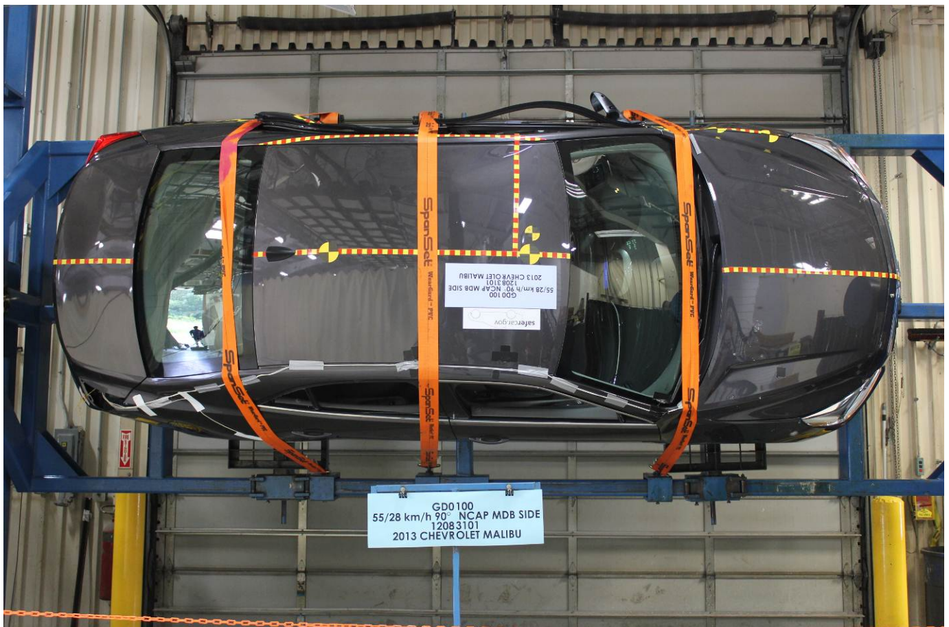
FMVSS No. 301 Static Rollover 90 Degrees
