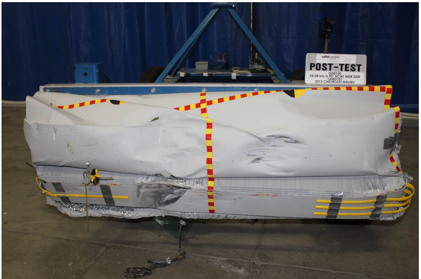
Post-Test Front View of MDB Impactor Face
