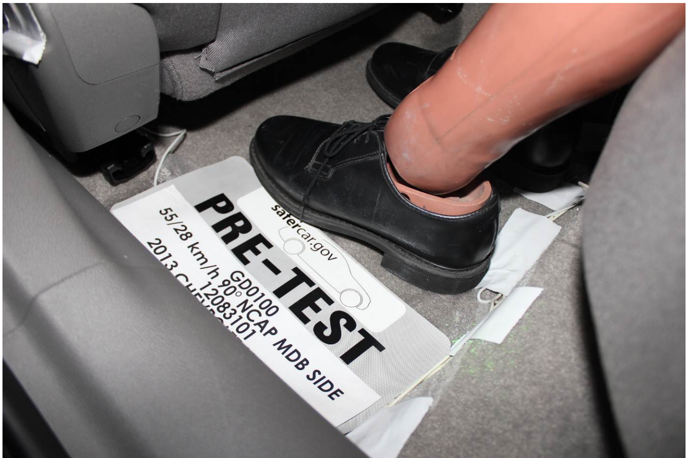
Pre-Test Placement of Rear Passenger Dummy's Feet
