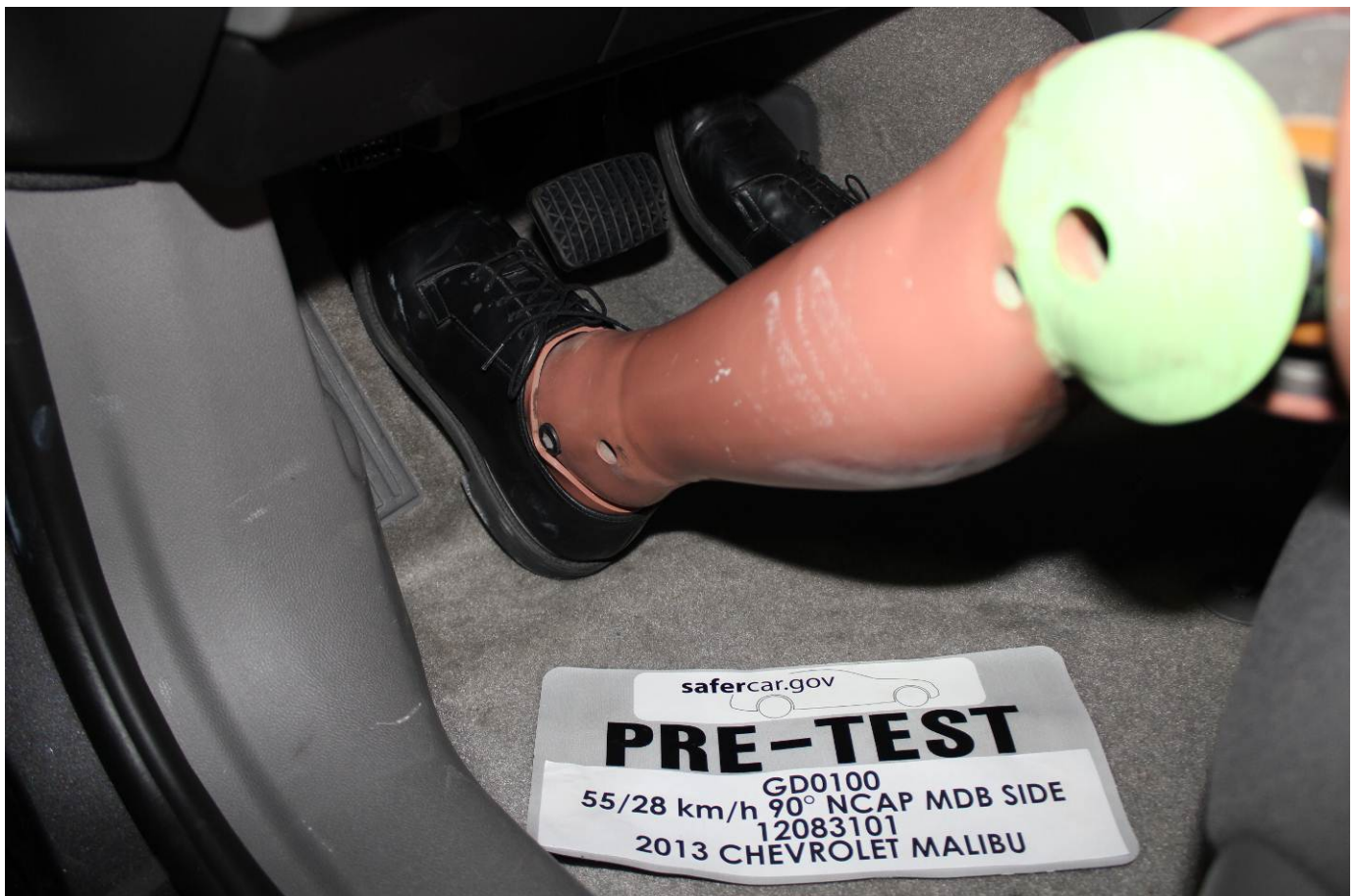
Pre-Test Placement of Driver Dummy's Feet
