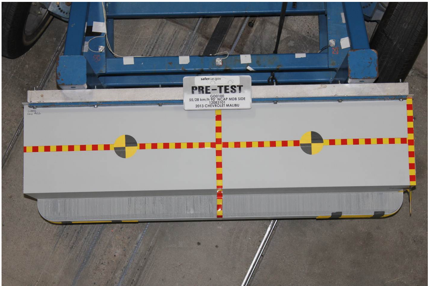
Pre-Test Top View of MDB Impactor Face
