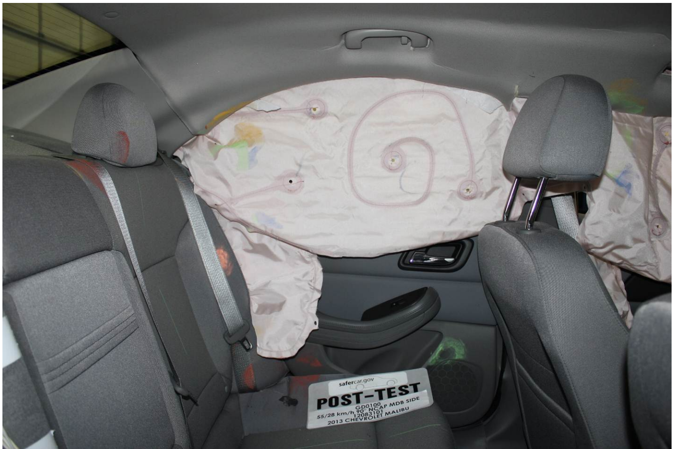
Post-Test Rear Passenger Inner Door Panel View
