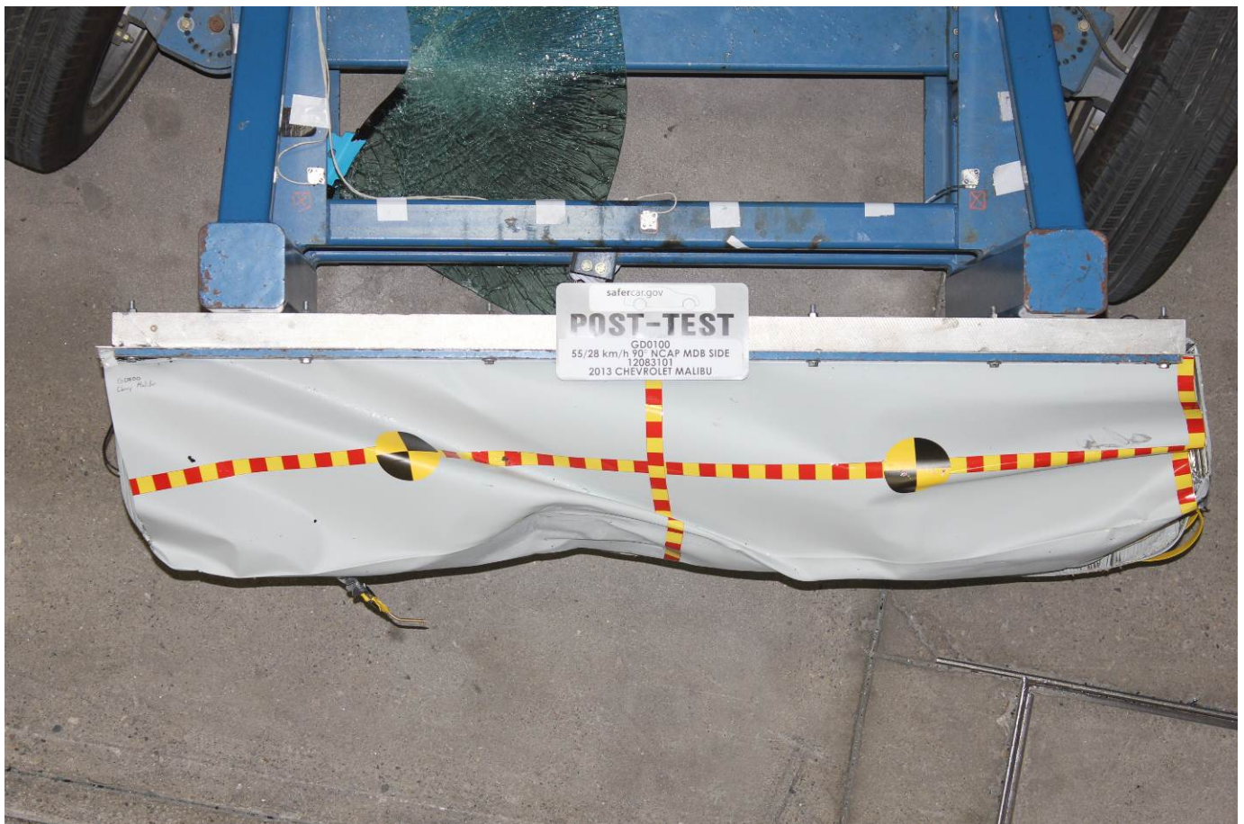
Post-Test Top View of MDB Impactor Face
