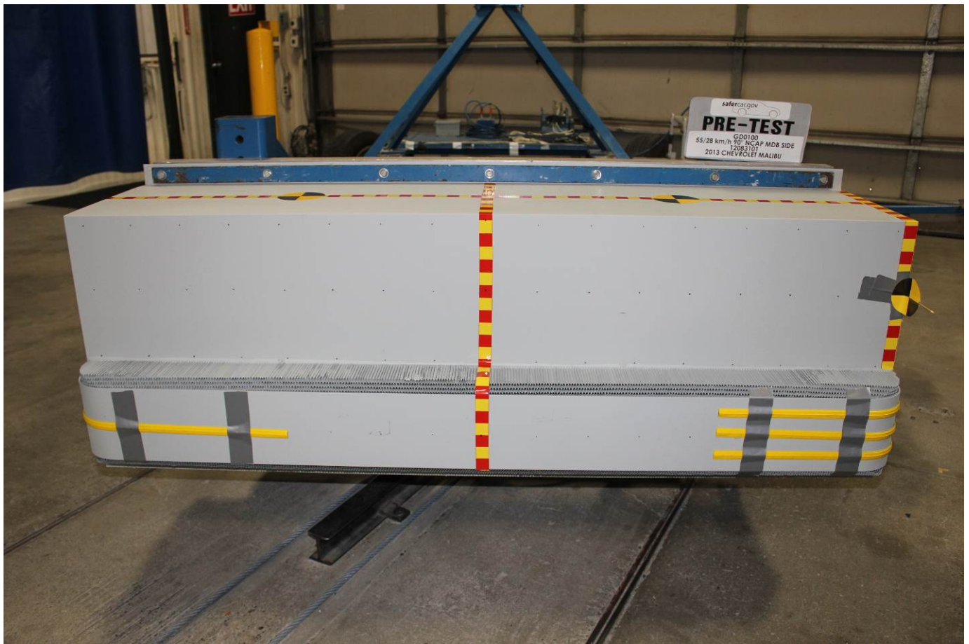
Pre-Test Front View of MDB Impactor Face
