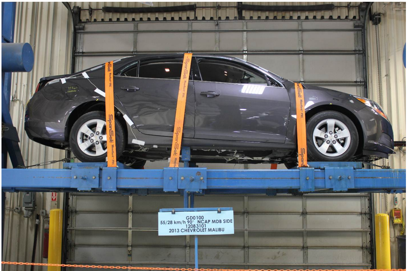
FMVSS No. 301 Static Rollover 0 Degrees
