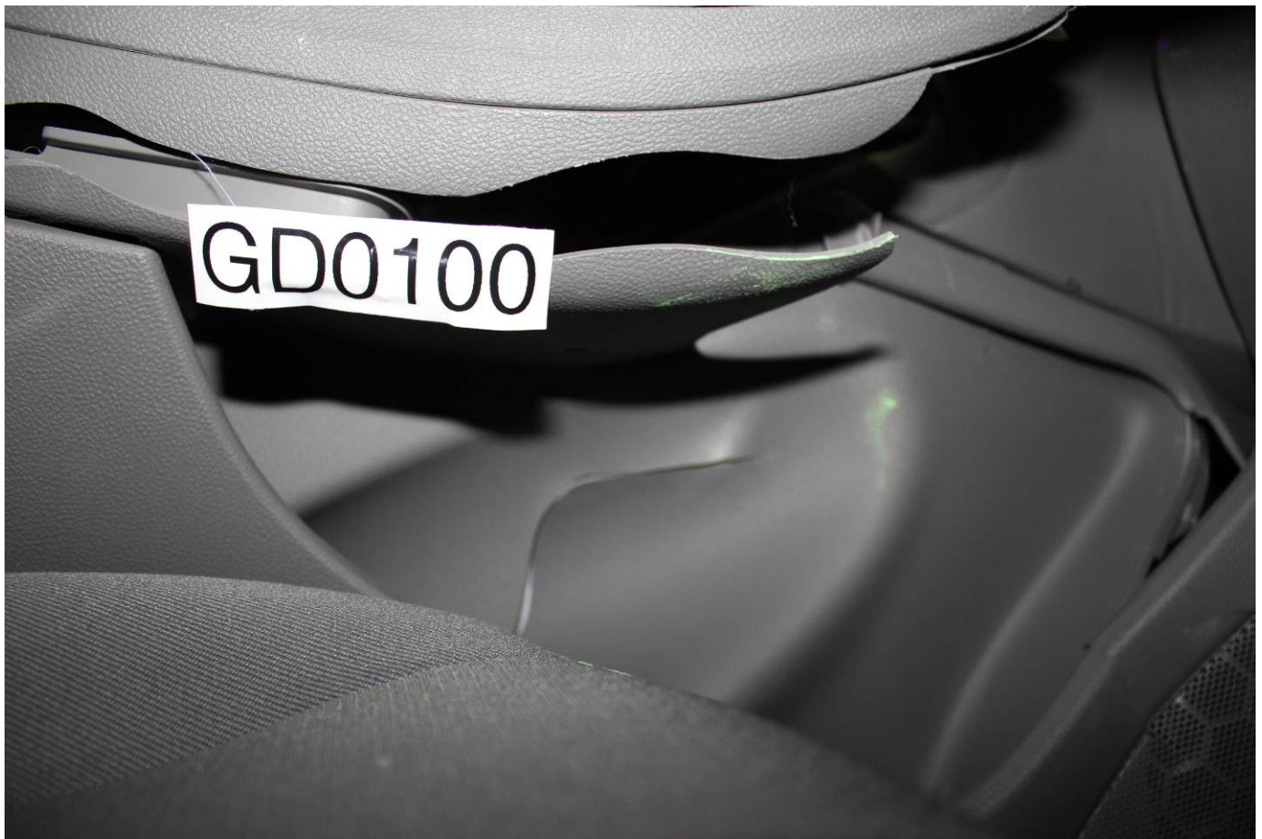
Post-Test Driver Dummy Close-up Knee Contact View
