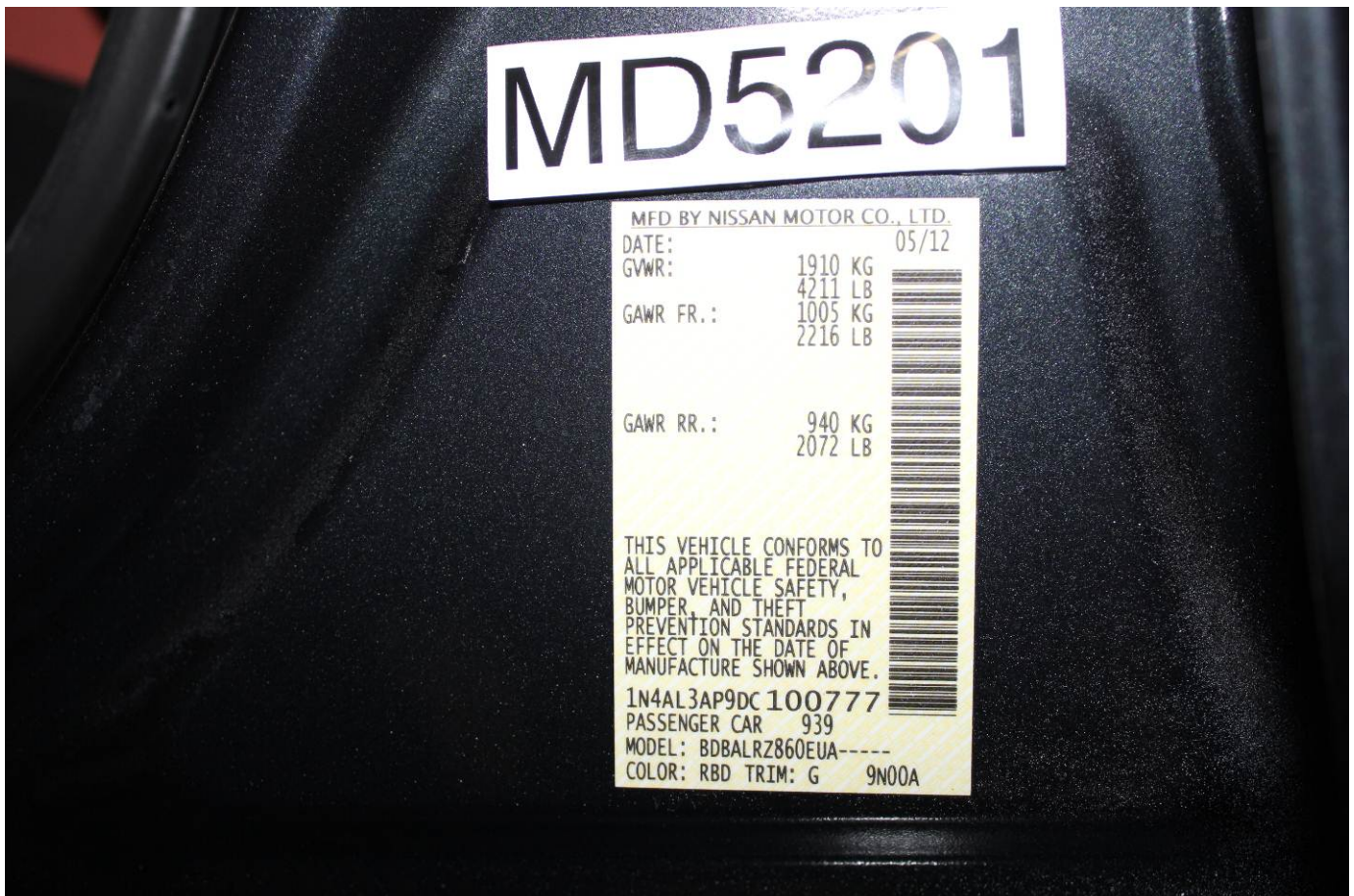
Close-Up View of Vehicle's Certification Label
